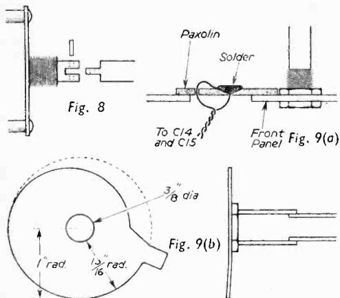
Fig. 8 (above).—Modification to the fine tuner spindle. Fig. 9(a) and (b).—Further fine tuner details.
