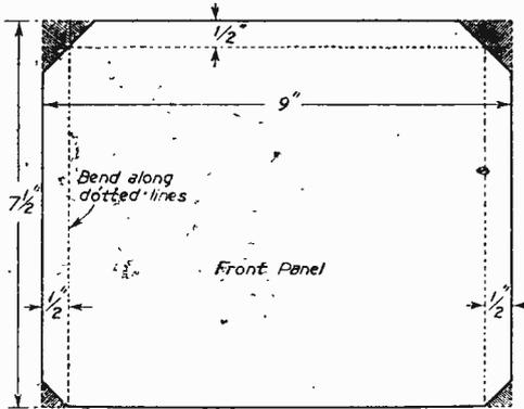
Fig. 8.—The front panel details.
