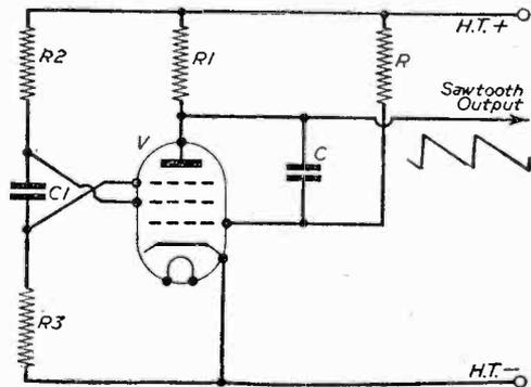
Fig. 26.—Miller transistron sawtooth voltage generator.
