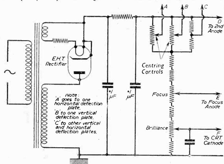
Fig. 11.—An A.C. mains-fed EHT supply.
