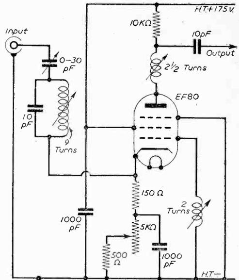
Fig. 7. An alternative circuit.
