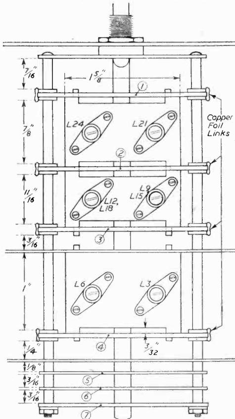
Fig. 7.—Details of the main switching assembly.
