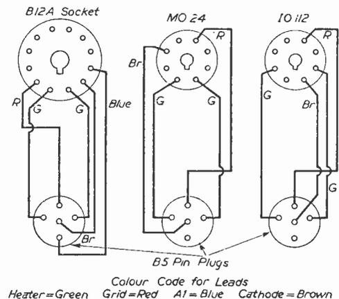
Fig. 9.—Tube base connections.
