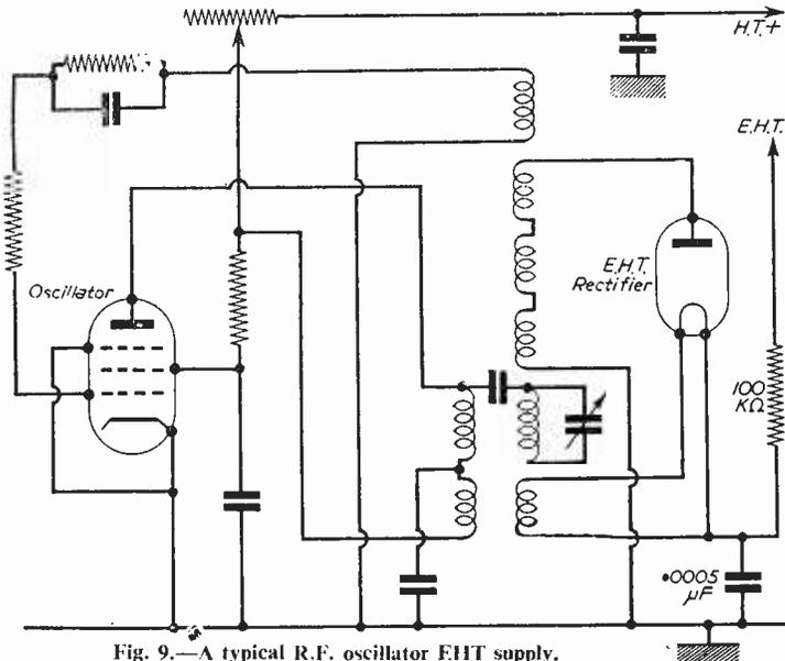
Fig. 9.—A typical R.F. oscillator EHT supply.
