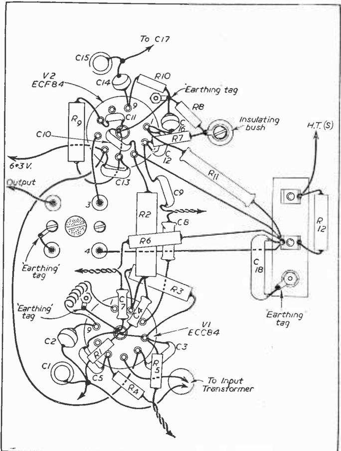
Fig. 4(b).—Wiring diagram of the tuner.
