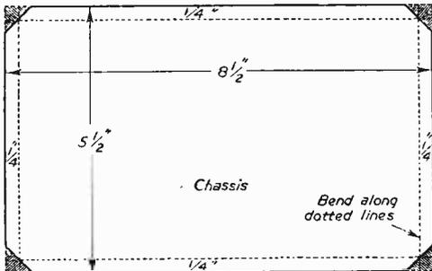
Fig. 3.—Details of the top of chassis.
