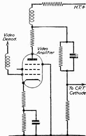
Fig. 44.—A typical video output stage.
