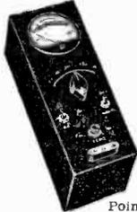
Comprising 2in. moving coil meter, scale calibrated in AC DC volts, ohms and milli-amps. Voltage range AC/DC 0-10, 0-100 and 0-500. Milli-amps 0-10, 0-100. Ohms 0-1,000 and 0-10,000. Front panel, range switch, wire-wound pot (for ohms zero setting), two toggle switches, resistors and metal rectifier. In grey hammer finish case. **19/6** Plus P. & P. 1/6.
