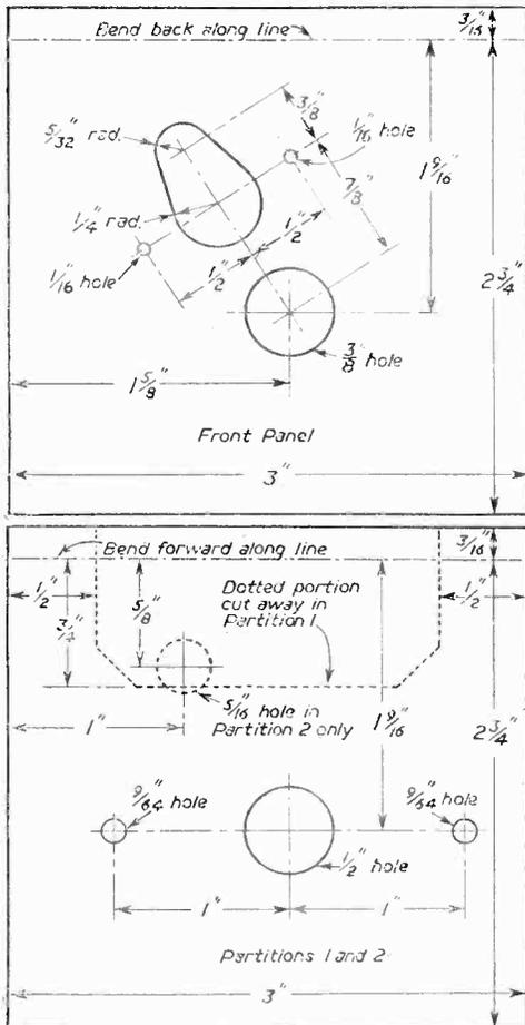
Fig. 5(a) (above), details of the panel, and 5(b) (below), the partitions, two of which are needed.
