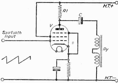
Fig. 25.—Frame scanning output stage for high impedance coils.
