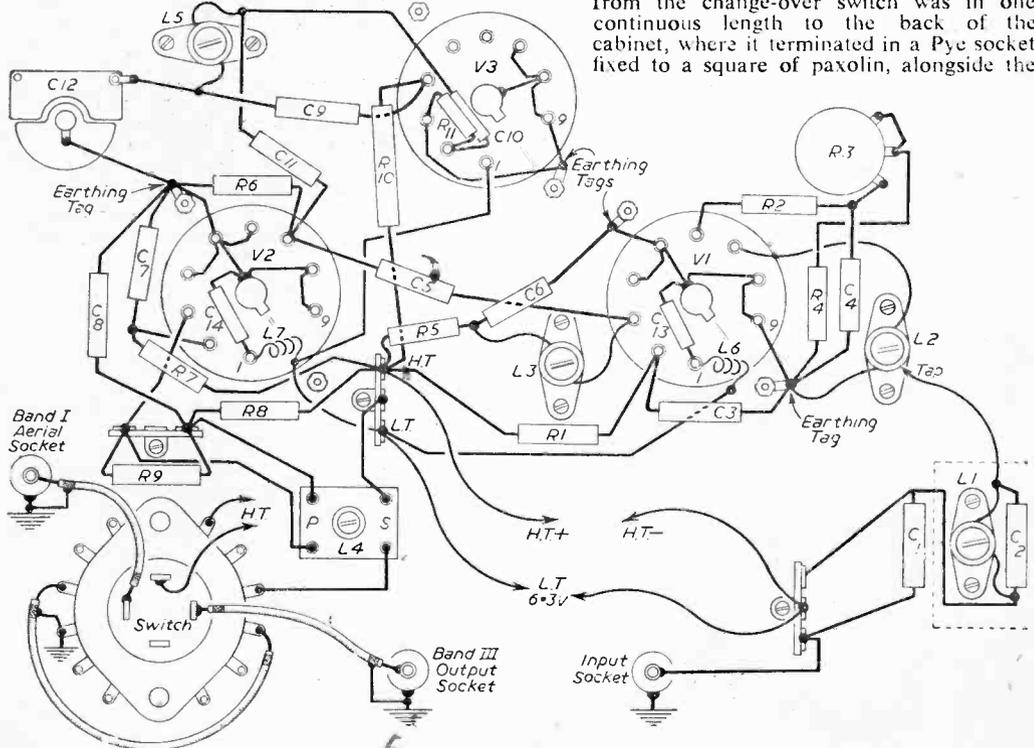
Fig. 8. Wiring diagram of the converter.
