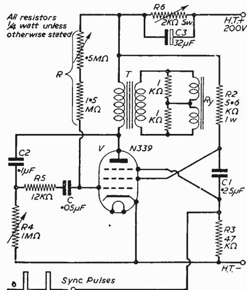
Fig. 28.—Inductive Miller transatron frame scanning circuit.
