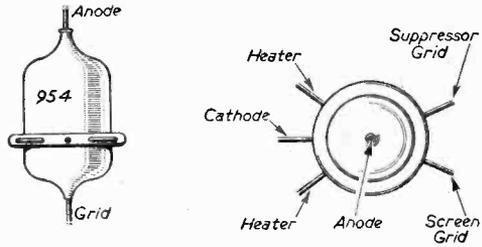
Fig. 1.—Connections for 954 V.H.F. pentode.
