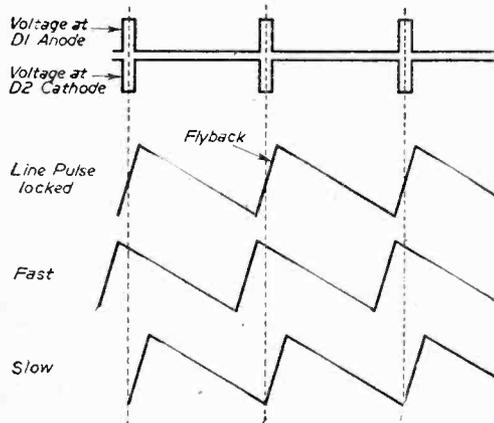
Fig. 2 (b).—Waveforms out of sync. and locked.
