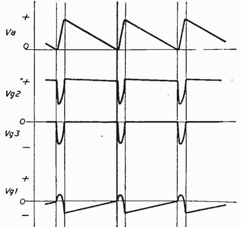
Fig. 27.—Waveforms at the various valve electrodes of the transatron circuit.
