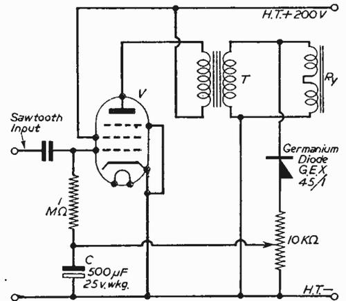
Fig. 29.—Method of obtaining bias supply in a frame scanning output stage.
