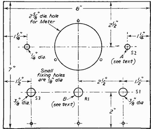
Fig. 2.—Drilling details for the panel.
