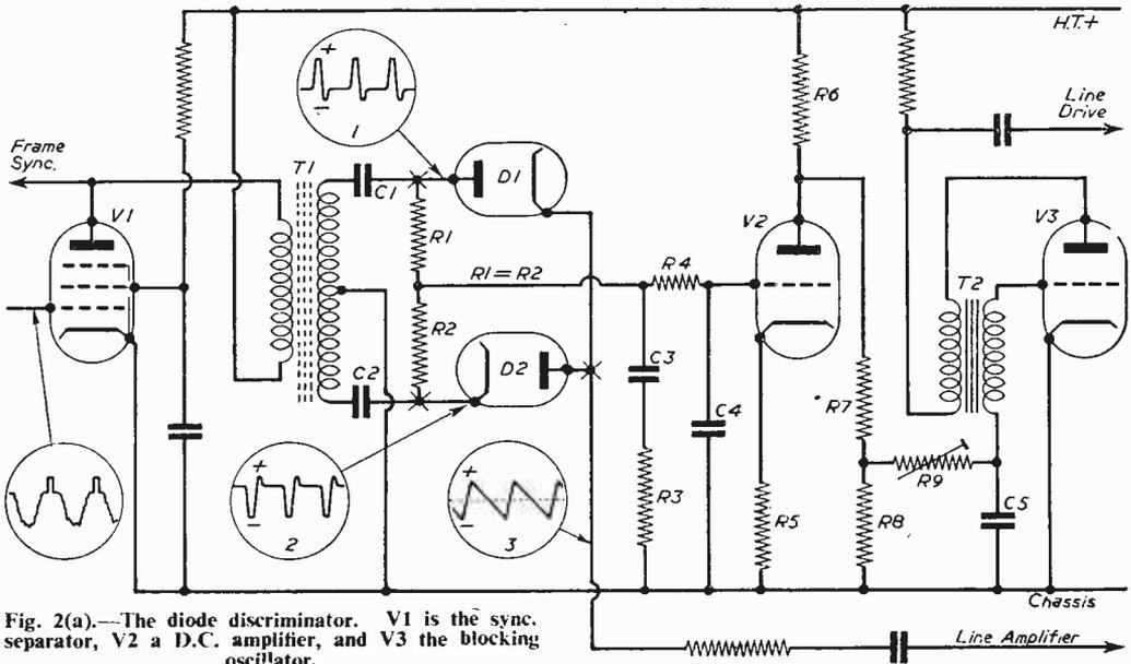
Fig. 2(a).—The diode discriminator. V1 is the sync. separator, V2 a D.C. amplifier, and V3 the blocking oscillator.
