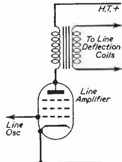
Fig. 10.—A line output stage for use with Fig. 9.
