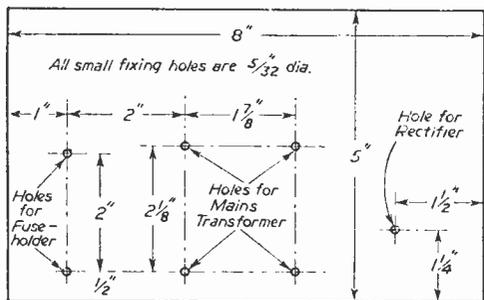
Fig. 4.—Drilling details for the chassis.
