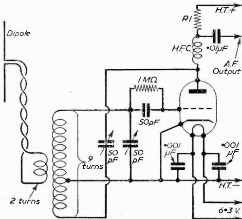
Fig. 3.—The detector circuit.
