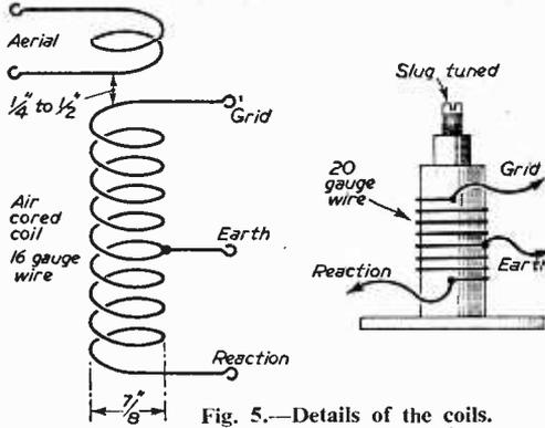
Fig. 5.—Details of the coils.
