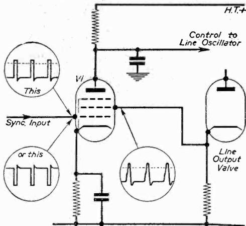
Fig. 3.—A pentode coincidence detector. The screen is tied down to the line output valve cathode.
