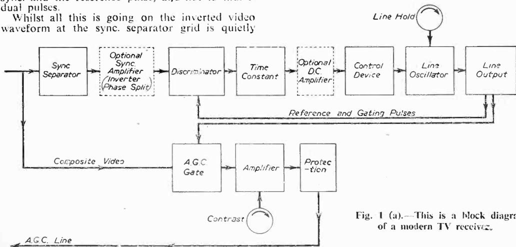
Fig. 1 (a).—This is a block diagram of a modern TV receiver.
