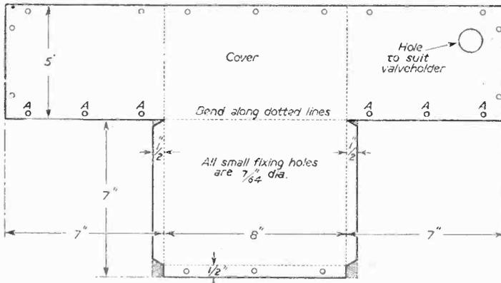
Fig. 6.—Details of the chassis cover.
