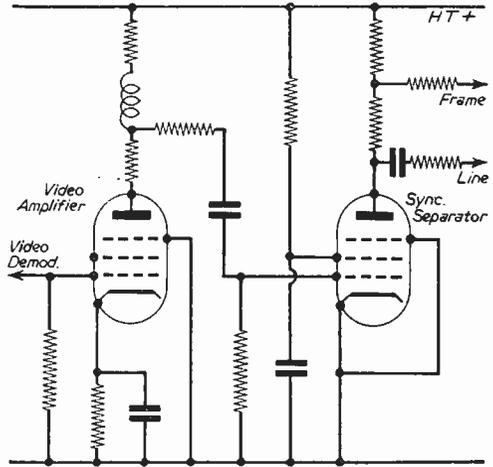
Fig. 12.—Simple sync separator.
