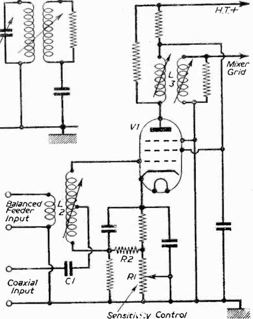
Fig. 2.—Input to the sound and vision R.F. amplifier.
