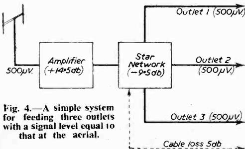
Fig. 4.—A simple system for feeding three outlets with a signal level equal to that at the aerial.
