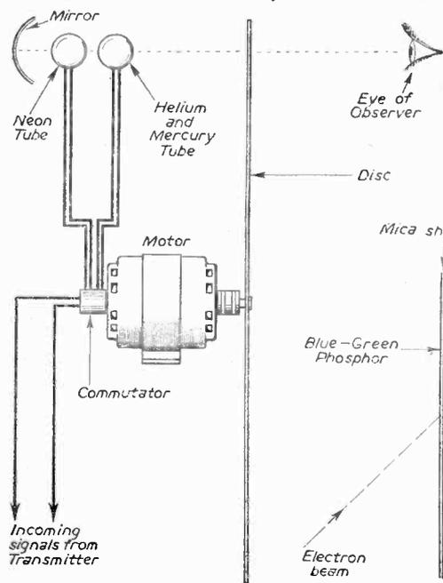
Fig. 11.—1928 system for colour television.
