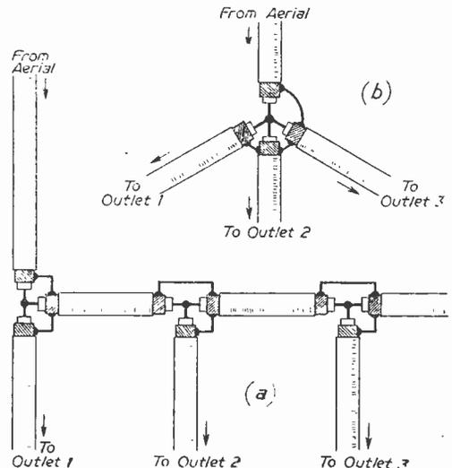
Fig. 1.—Neither of these arrangements should be used for operating more than one receiver from a single aerial.
