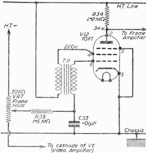
Fig. 1.—Circuit of the frame oscillator of the Baird 164.
