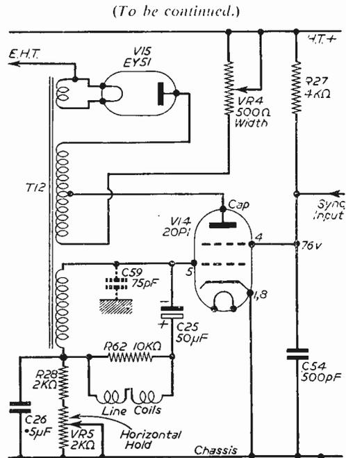
Fig. 3.—A circuit diagram of the line timebase of the Baird 164 series.
