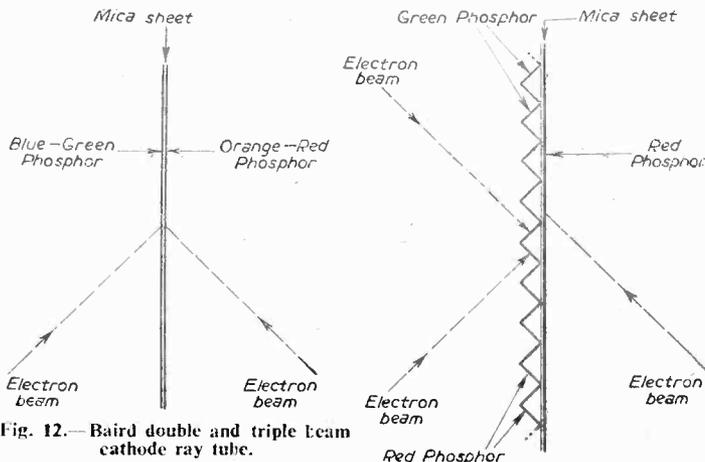
Fig. 12.—Baird double and triple beam cathode ray tube.
