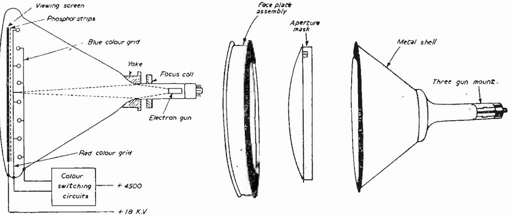
Fig. 8 (Right).—The Chromatron colour tube. (Left) The R.C.A. colour tube dissected.
