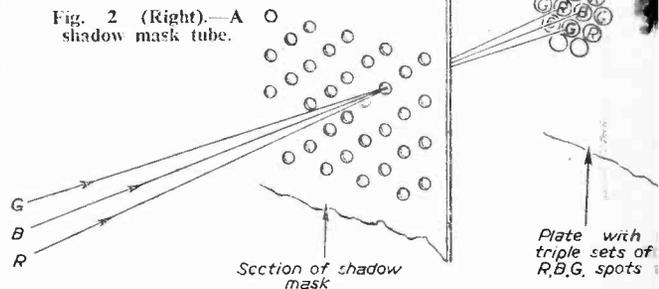
Fig. 2 (Right).—A shadow mask tube.
