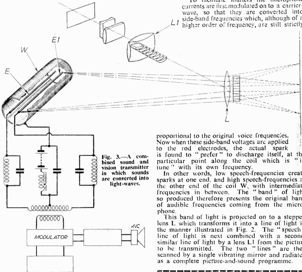
Fig. 3.—A combined sound and vision transmitter in which sounds are converted into light-waves.
