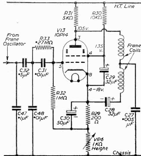
Fig. 2.—Frame amplifier circuit of the Baird 164.
