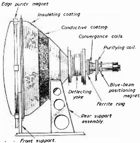
Fig. 9.—A sketch showing a modern colour tube with all the essential parts identified.
