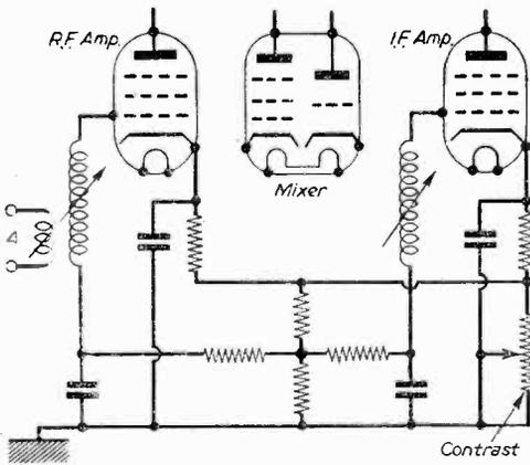
Fig. 3.—Method of controlling the I.F. and R.F. stages by a single control.
