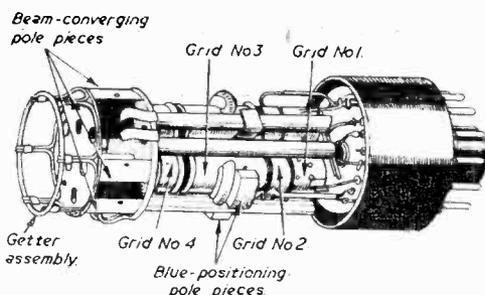
Fig. 10.—A sketch of the "gun" assembly of a modern colour cathode ray tube.
