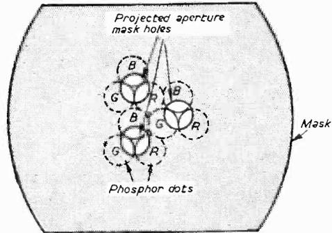
Fig. 3.—The colour grains seen through the shadow mask.
