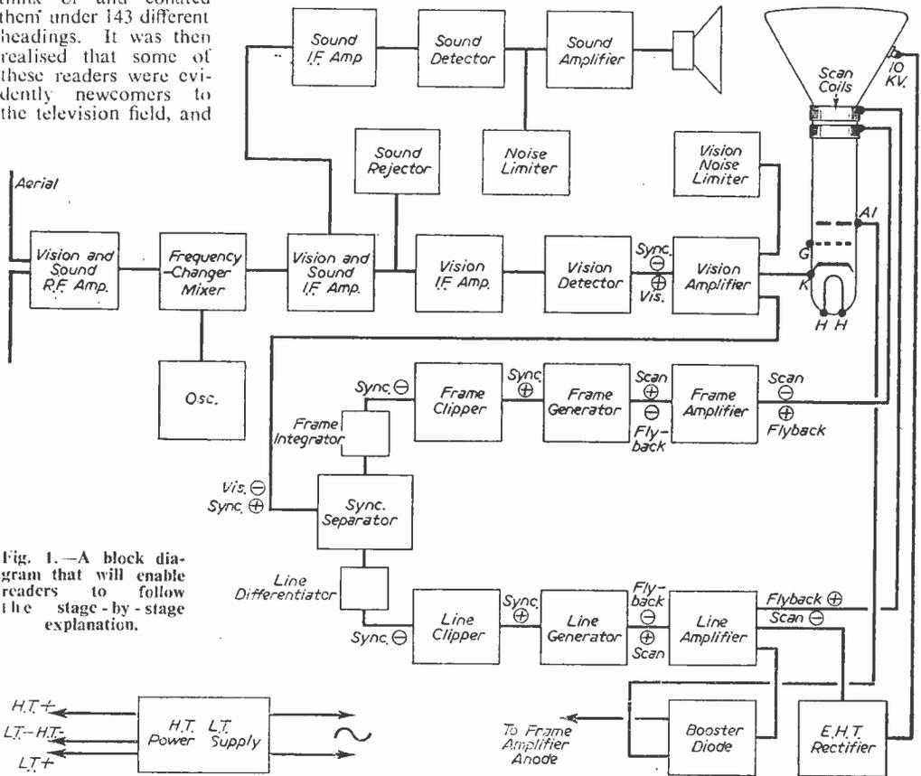
Fig. 1.—A block diagram that will enable readers to follow the stage-by-stage explanation.
