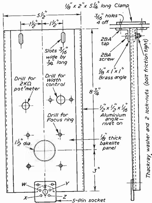
Fig. 16.—Details of the support for the tube neck
