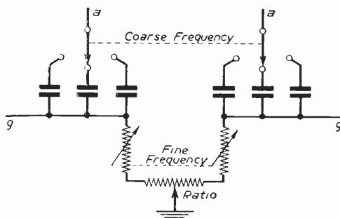
Fig. 4.—Controlling the frequency of the multivibrator.
