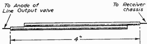
Fig. 3.—A small value capacitor can be produced from a length of twin p.v.c. covered cable. The conductors act as the plates while the p.v.c. covering acts as the dielectric.
