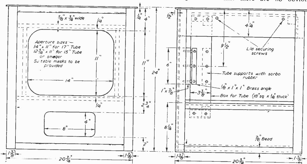
Fig. 15.—Details of the cabinet construction. (Left) front view. (Right) side view.
