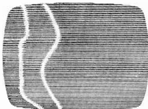
Fig. 1.—Showing how the "windscreen wiper" effect may appear momentarily on the screen.
