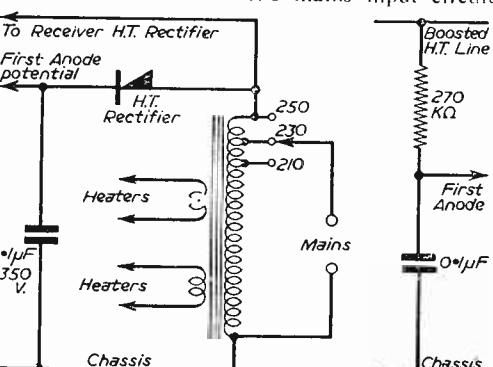
Fig. 4 (Above, left) and Fig. 5 (Above, right) show two methods of obtaining a potential suitable for the first anode of a tetrode.
