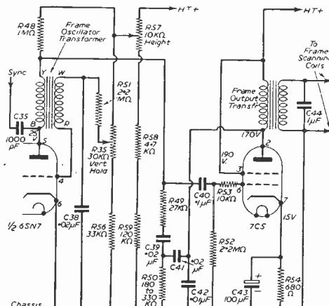
**Fig. 1.—Frame timebase circuit of Cossor Models 916, 917, 920 and 922.**
