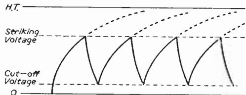
Fig. 2.—Neon timebase waveforms.
