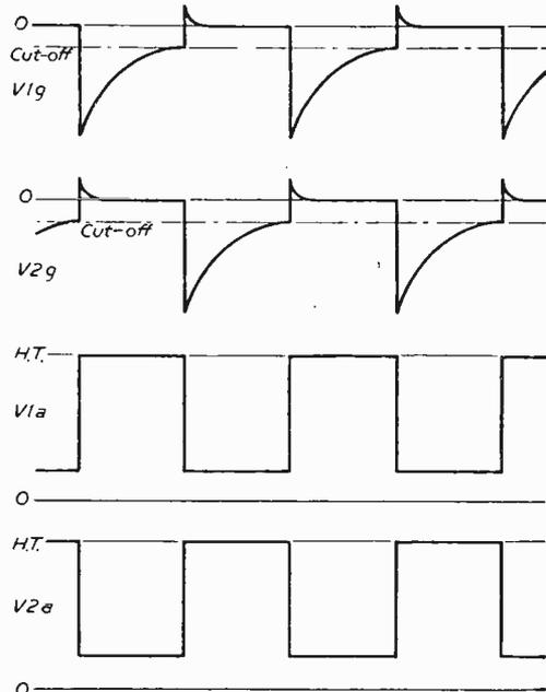
Fig. 5.—Waveforms in the multivibrator.
