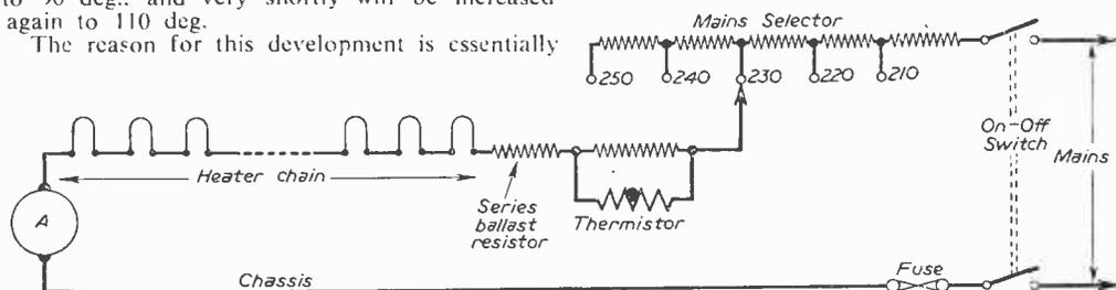
Fig. 1.—Including an A.C. ammeter in the circuit to check the heater current.
