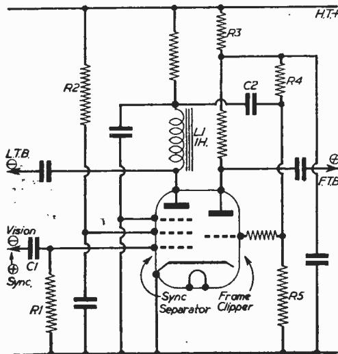
Fig. 16.—The pentode sync separator.
