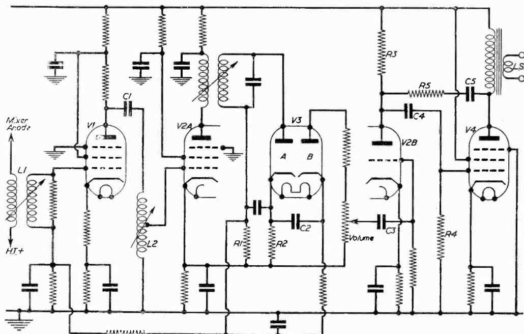
Fig. 15.—The sound circuit.
