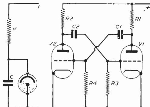
Fig. 1 (Left).—Neon timebase oscillator. Fig. 3 (Right).—A Multivibrator circuit.
