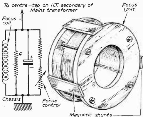
Fig. 6 (Above, left).—The resistor R is used to reduce the current through the focusing coil.
