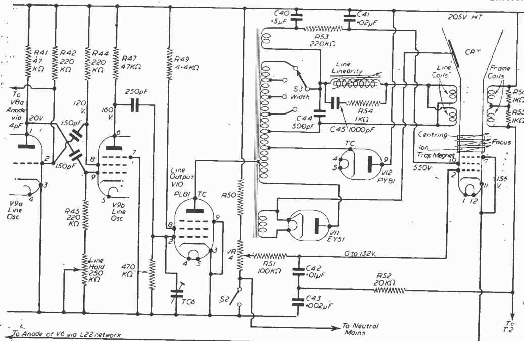
Fig. 1.—Circuit of line oscillator and output stages.
