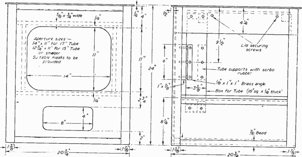
Fig. 15.—Details of the cabinet construction. (Left) front view. (Right) side view.
