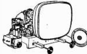
17in. Rectangular Tube on modified chassis. Supplied as single channel chassis covering B.B.C. channels 1-5, or incorporating Turret Tuner which can be added as an extra, at our special price to chassis
