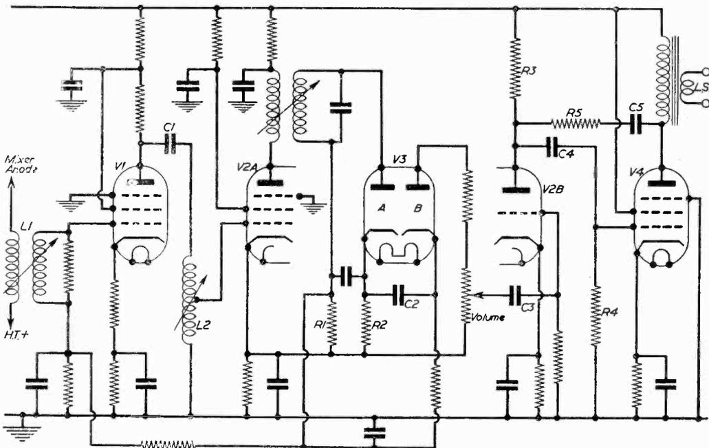
Fig. 15.—The sound circuit.
