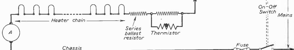
Fig. 1.—Including an A.C. ammeter in the circuit to check the heater current.
