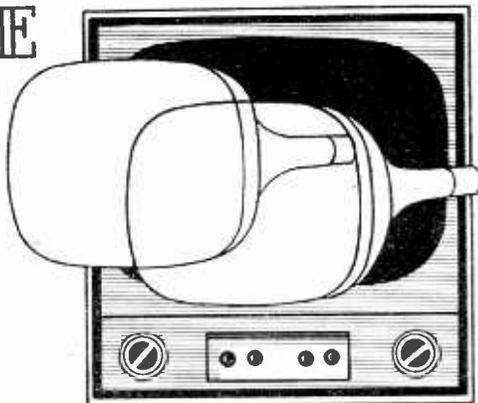
a mechanical one, and is that as the beam is deflected over a greater angle, the length of the tube can be decreased for a given screen size. This means that very slim receivers can be produced without the ugly bulge at the back of the cabinet, which on older receivers houses the tube base and part of the neck.
