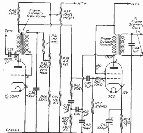
Fig. 1.—Frame timebase circuit of Coscor Models 916, 917, 920 and 923.
