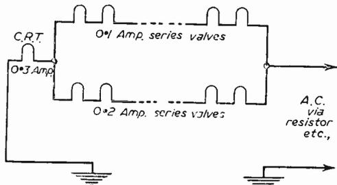
Fig. 2.—An alternative circuit for series connection of valve heaters.
