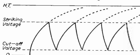
Fig. 2.—Neon timebase waveforms.
