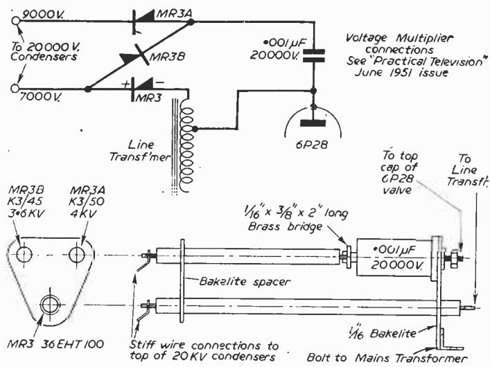
Fig. 13.—The circuit and mounting of the voltage multiplier.
