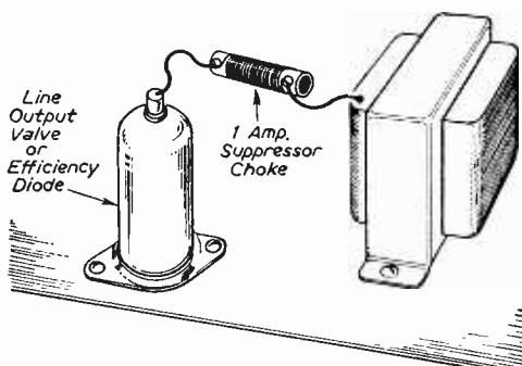
Fig. 2.—The introduction of a small iron-cored suppressor choke is often sufficient to damp the diode switching effect and B-K oscillation.
