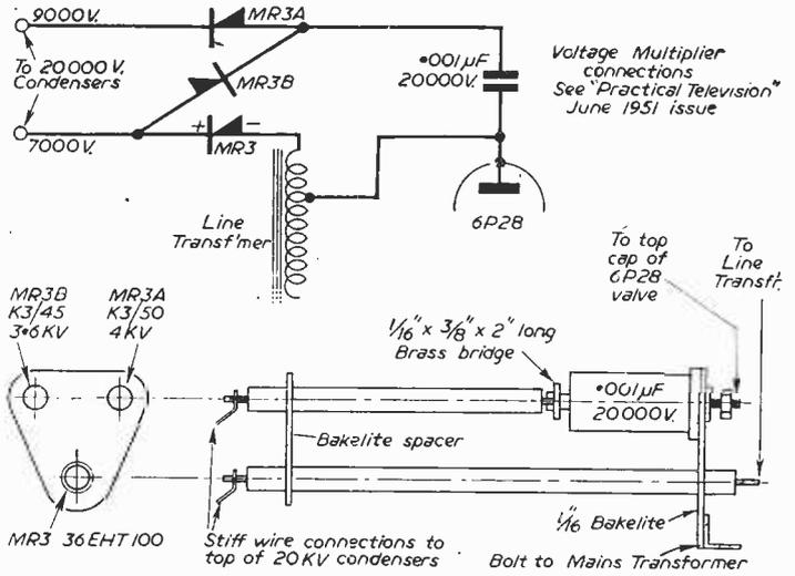
Fig. 13.—The circuit and mounting of the voltage multiplier. Fig. 14 (Below, left).—Construction of the tube mask.
