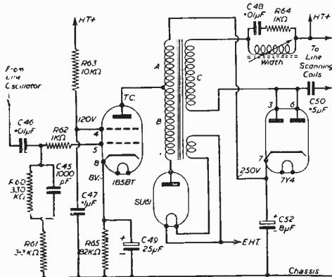
Fig. 2.—The circuit of the line amplifier.
