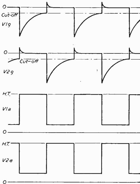
Fig. 5.—Waveforms in the multivibrator.
