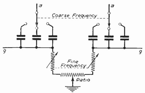
Fig. 4.—Controlling the frequency of the multivibrator.
