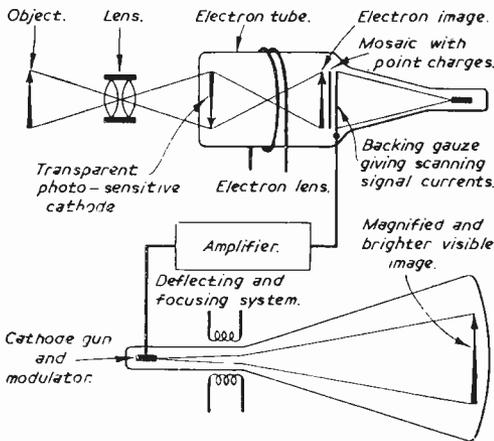
A simple form of industrial television equipment for image magnification.
