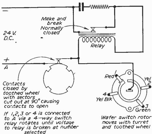
Fig. 2.—Circuit and operation of the impulse relay.
