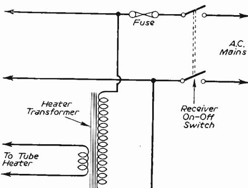
Fig. 3.—Using a separate transformer for the tube heater.
