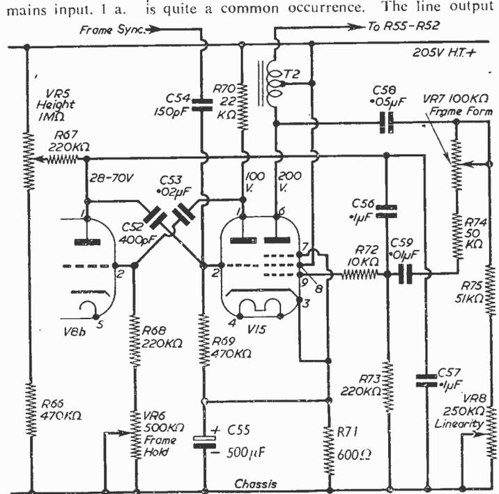
Frame oscillator and output stages.
