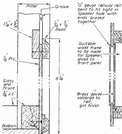
Fig. 18 (Above, left).—Shows the construction of the bottom part of the sides of the cabinet. The loose wooden sides slide into the groove indicated.
