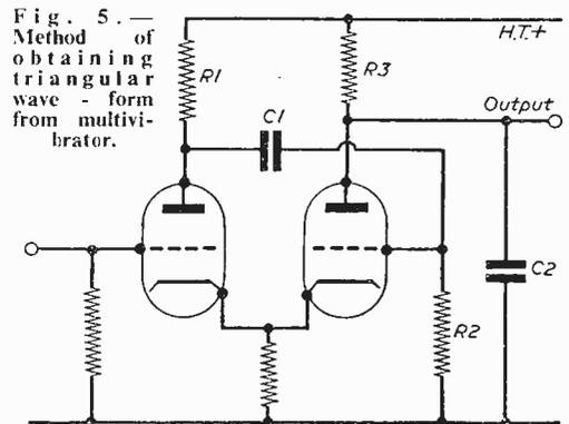
Fig. 5.—Method of obtaining triangular wave form from multivibrator.
