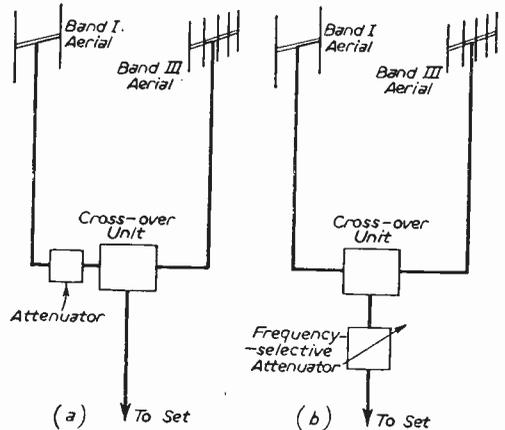
Fig. 2.—Showing at (a) the position for the introduction of an attenuator for eliminating cross-modulation on Band I, and at (b) the position for a frequency-selective attenuator which serves to adjust the level of the Band I signal with respect to the Band III signal, which is hardly affected by the unit. This method is essential where a combined aerial and single down-lead are adopted.
