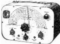
C.W. and mod. switch, variable A.F. output. Incorporating magic-eye as output indicator.
