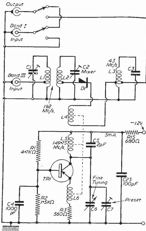
Fig. 2.—A Channel 9 to Channel I Converter.
