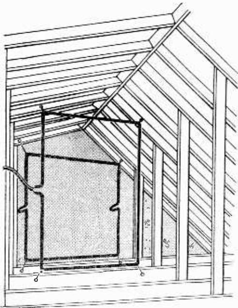
Fig. 1.—A quad aerial positioned parallel to the party wall which is shown shaded.
