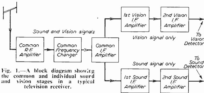
Fig. 1.—A block diagram showing the common and individual sound and vision stages in a typical television receiver.
