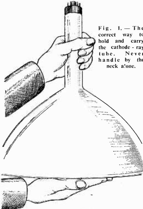
Fig. 1.— The correct way to hold and carry the cathode-ray tube. Never handle by the neck alone.
