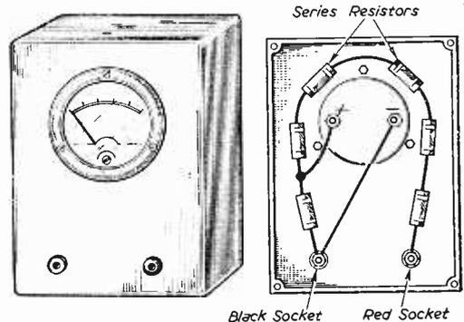
The meter in its case, and a rear view of the panel.
