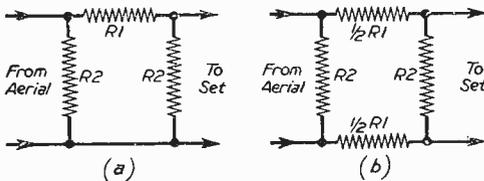
Fig. 3.—Pi-type attenuators (a) for coaxial feeder and (b) for twin feeder.  $R_1 = Z(N^2 - 1)/2N$  and  $R_2 = Z(N+1)N - 1$ , where  $Z$  is the feeder and receiver input impedance, and  $N$  is the ratio of input to output signal voltage (attenuation ratio).
