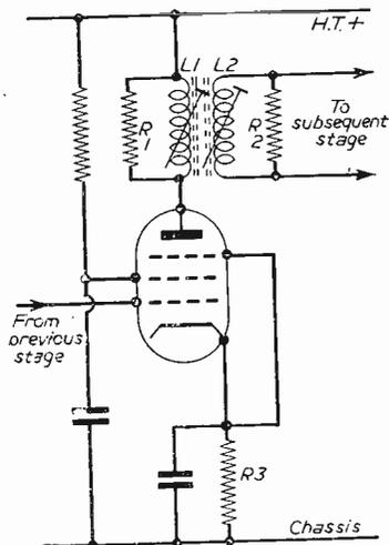
Fig. 2.—Improved gain at the expense of definition can be secured by increasing the value of the damping resistors R1 and R2, or by shunting R3 with a 500 ohm resistor.
