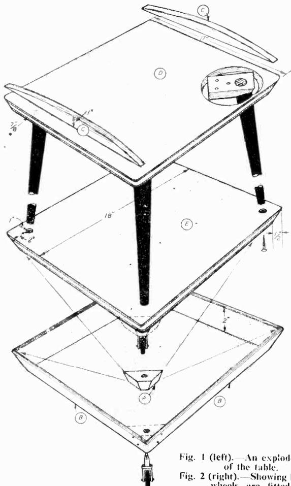
Fig. 1 (left).—An exploded view of the table.
