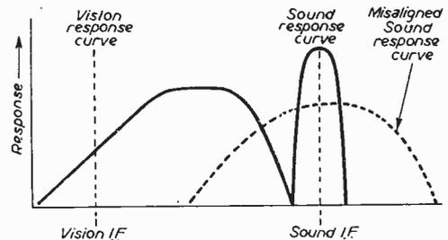
Fig. 4.—Vision-on-sound is often caused by misalignment of the sound I.F. channel. This causes the sound response to spread out and embrace the vision response, as indicated by the broken-line curve.
