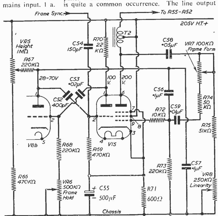
Frame oscillator and output stages.
