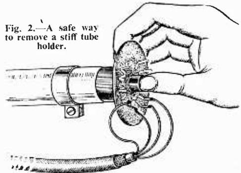
Fig. 2.— A safe way to remove a stiff tube holder.
