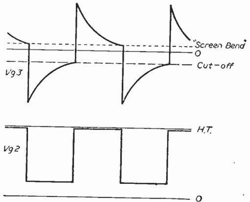
Fig. 2.—Waveforms in the transitron.
