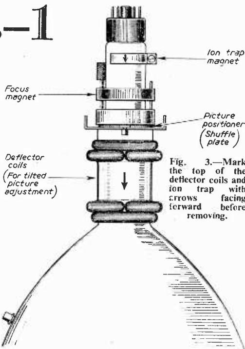
Fig. 3.—Mark the top of the deflector coils and ion trap with arrows facing forward before removing.
