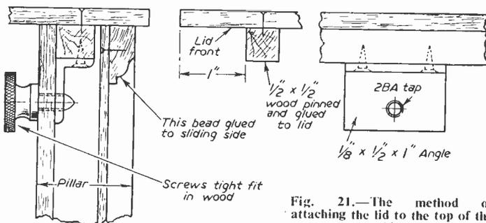
Fig. 21.—The method of attaching the lid to the top of the cabinet.
