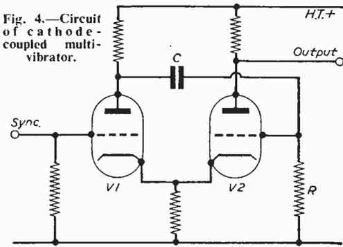
Fig. 4.—Circuit of cathode-coupled multivibrator.
