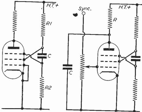
Fig. 1.—(Above, left) Basic circuit of transitron oscillator.
