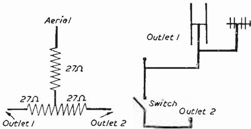
Fig. 1 (Left).—Theoretical circuit for two outlets.
