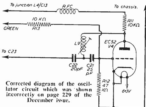
Corrected diagram of the oscillator circuit which was shown incorrectly on page 229 of the December issue.
