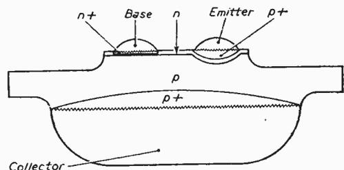
Fig. 1.—Diagrammatic representation of the alloy-diffusion junction transistor.
