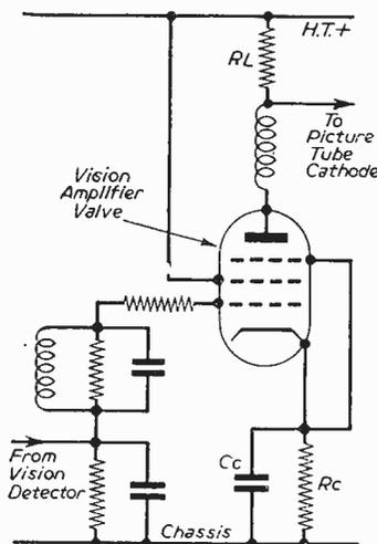
Fig. 1.—Sensitivity increase of the video amplifier can be accomplished either by increasing the value of Cc or RL.
