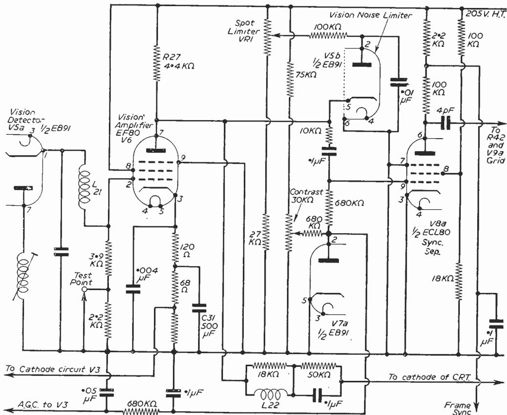
Circuit of the vision detector, amplifier, limiter and sync separator stages.
