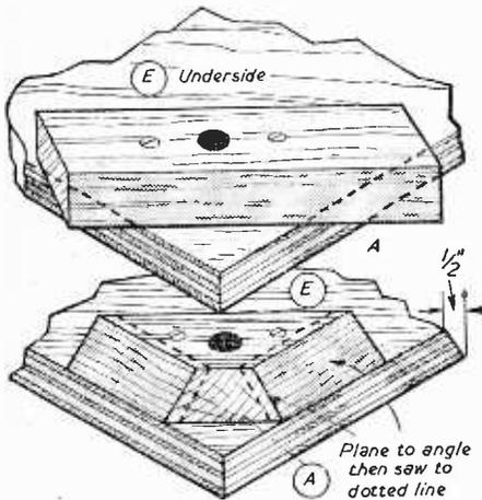
Fig. 3 (above).—Fixing the apron.
