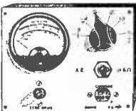
Comprising 2in. moving coil meter scale calibrated in AC/DC volts, ohms and milli-amps. Voltage range AC DC 0-50, 0-100, 0-200, 0-500, milli-amps 0-10, 0-100. Ohms range K-10,000. Front panel, range switch, wire-wound pot (for ohms zero setting), toggle switch, resistors and rectifier. Basic movement 2 mA. In grey hammer finished case.
