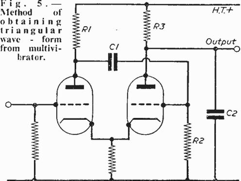
timebase, the multivibrator frequency is made much higher than the required sweep frequency, and the anode load of the output valve is made much higher than usual.
