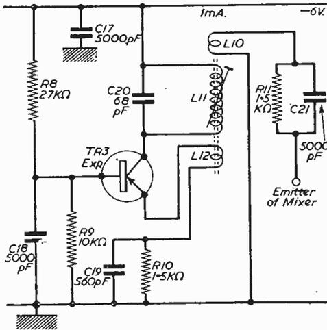
Fig. 4.—The transistorised local oscillator.
