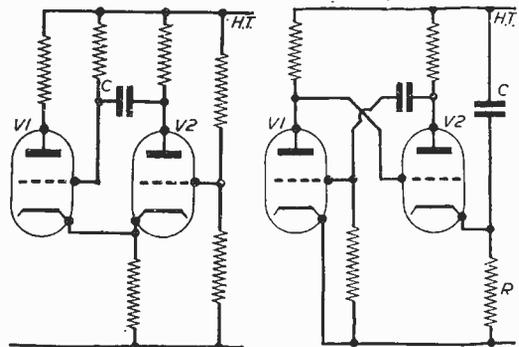
Fig. 2.—(Left) The "flip-flop" circuit.
