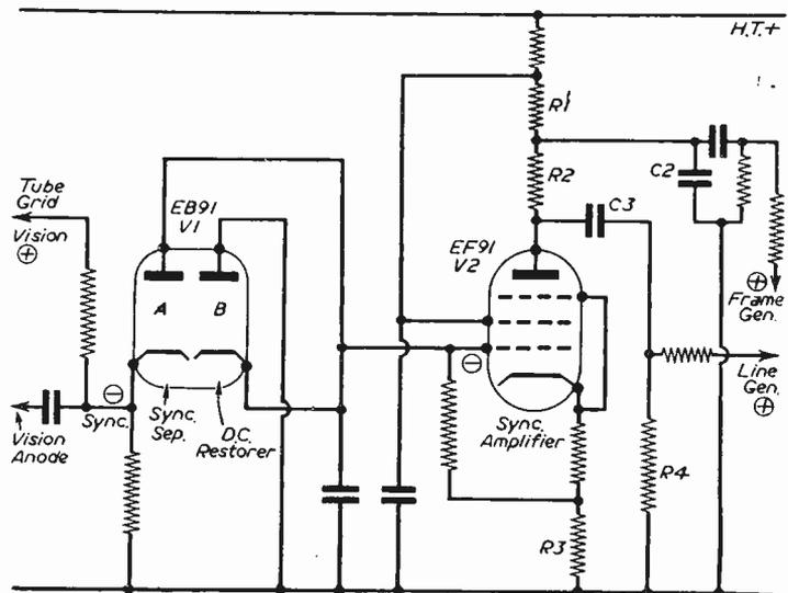
Fig. 20.—Diode type of sync separator.
