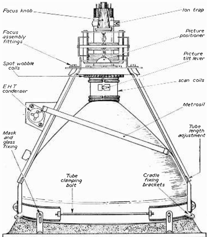
Fig. 4.—Details of the T231 tube cradle assembly.
