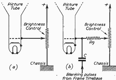
Fig. 3.—In most older receivers the brightness control is arranged as in circuit (a), but where frame-flyback suppression is featured, in more recent models, the circuit in (b) is often used.
