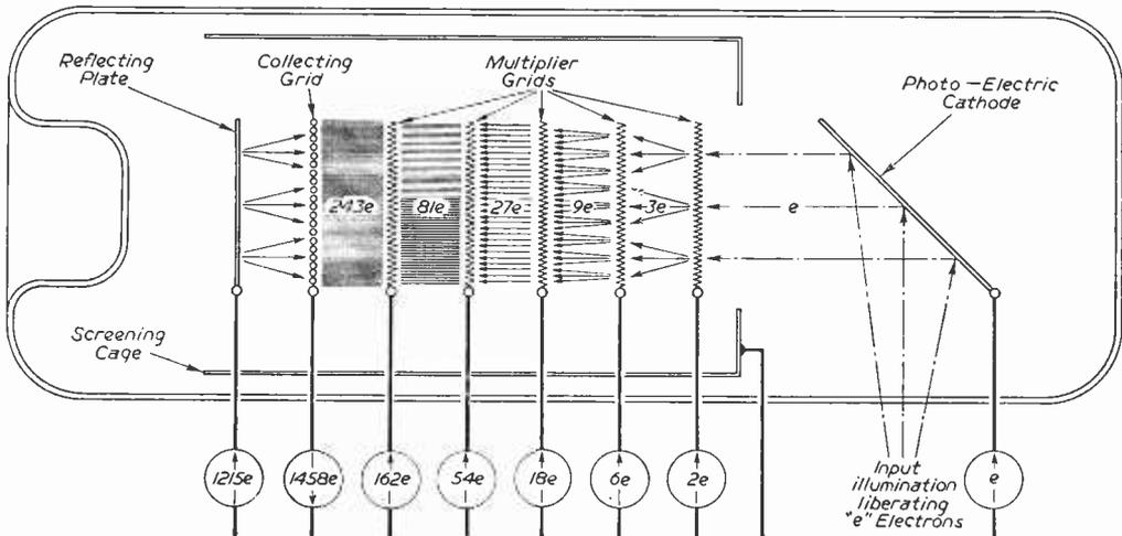
A pictorial representation of a grid cell multiplier.
