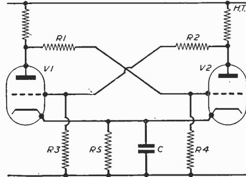
Fig. 1.—Stable multivibrator circuit.
