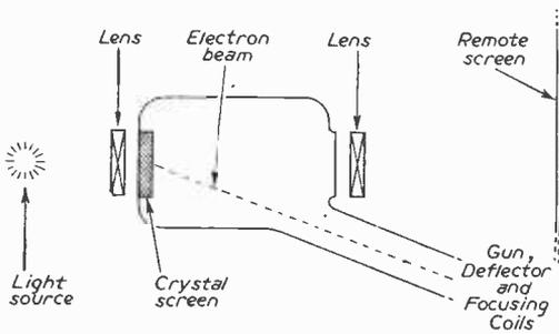
Basic details of a light relay C.R. tube.
