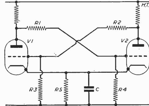
Fig. 1.—Stable multivibrator circuit.
