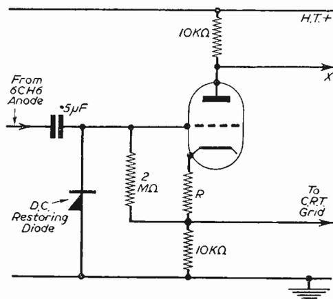
Fig. 2.—Cathode follower for use with grid modulation of C.R.T.
