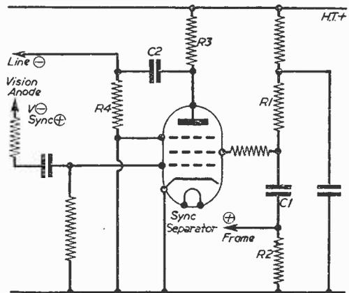
Fig. 18.—Taking off the frame pulses from the screen grid.
