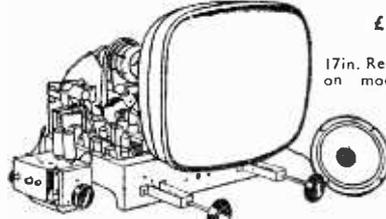
17in. Rectangular Tube on modified chassis.
