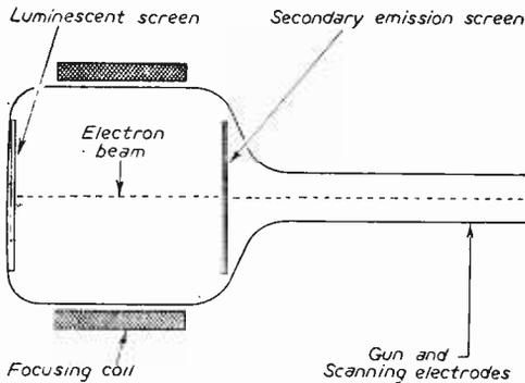
The secondary emission cathode ray tube.
