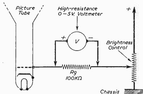
Fig. 4.—The set-up required for checking gas current.
