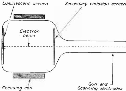
The secondary emission cathode ray tube.
