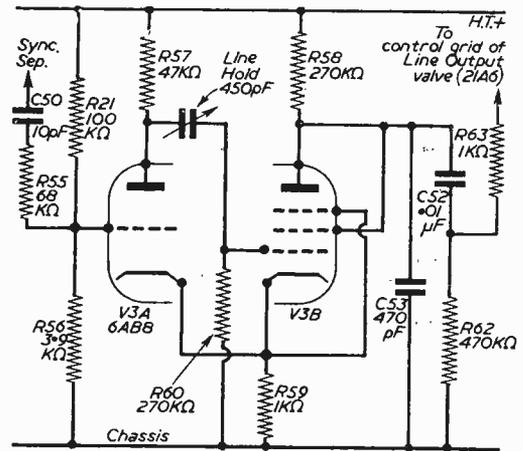
Fig. 2.—Circuit diagram of the line timebase generator.
