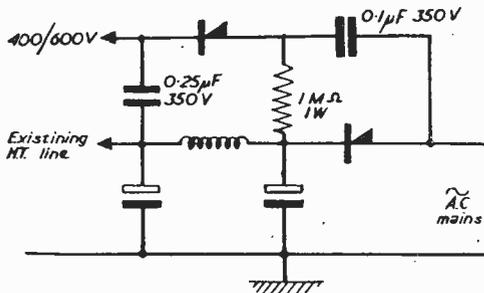
Picture tube substitution. A voltage additive arrangement.
