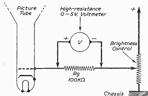
Fig. 4.—The set-up required for checking gas current.
