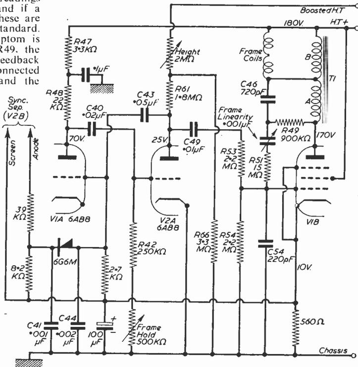
Fig. 1.—Circuit diagram of the frame timebase and interface filter of the Cossor 927 series.
