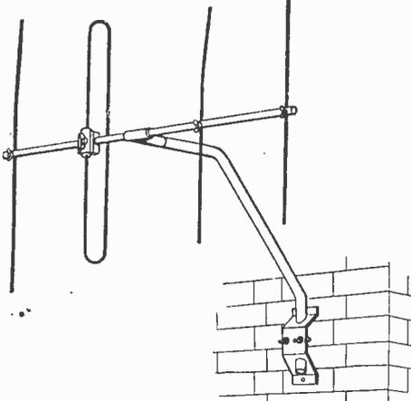
This powerful 4-element, pre-assembled, wide spaced Band III beam Aerial by a leading manufacturer. Supplied complete with cranked pole and wall fixing brackets, can also be loft mounted. Listed at 55/6.
