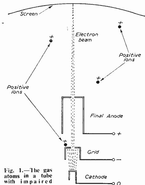
Fig. 1.—The gas atoms in a tube with impaired vacuum are bombarded by the fast-moving beam electrons and themselves lose electrons. This results in the creation of positive ions which drift towards the negatively charged grid, and detract from the tube efficiency.
