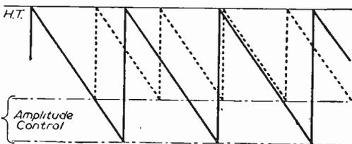
Fig. 6.—Effect of amplitude control on frequency.
