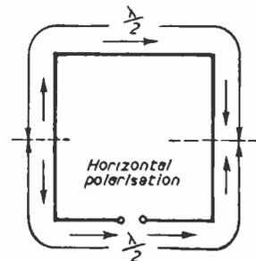
Fig. 4.—Distribution of current in a horizontally polarised aerial—driven member.
