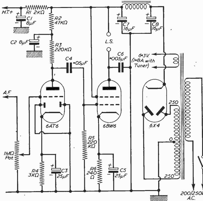
Fig. 4.—Amplifier using miniature valves.
