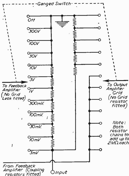
Fig. 5.—Input gain control. Both resistor chains add up to 2 M $\Omega$  each.
