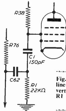
**Fig. 2.**—A modification to improve line lock and prevent bending of the verticals at the top of the picture. R1 and C1 are the extra components required.
