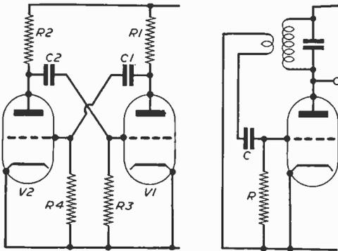
Fig. 1 (Left).—Pulse-producing multivibrator.
