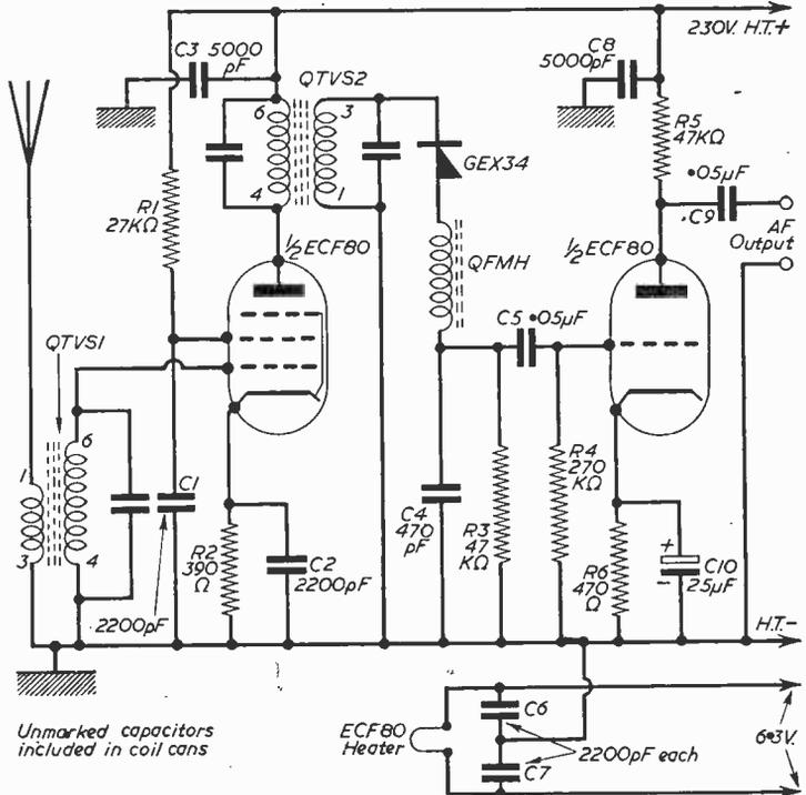
Fig. 1.—The TV tuner circuit.
