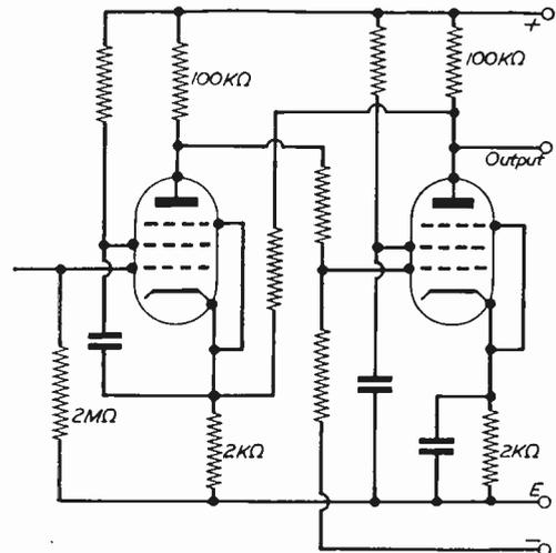
Fig. 4.—Negative feedback amplifier.
