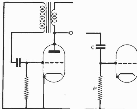
Fig. 3 (Left).—Blocking oscillator.
