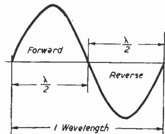
Fig. 3.—The current flow in an aerial.
