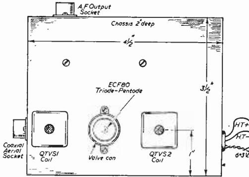
Fig. 2.—Plan view of the chassis.
