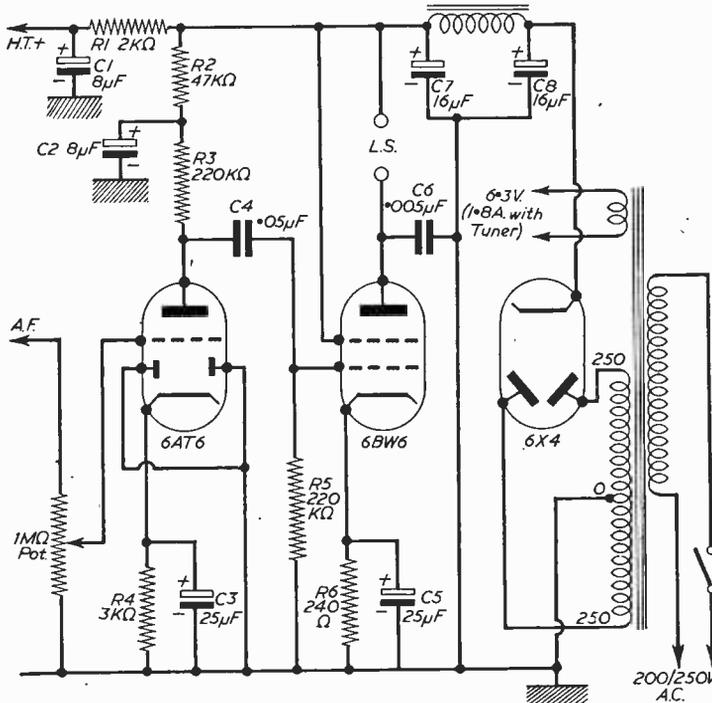
Fig. 4.—Amplifier using miniature valves.
