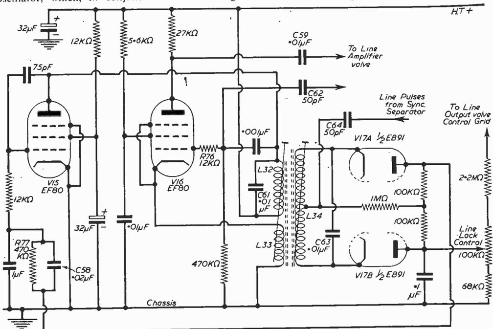
Fig. 1.—Line oscillator, discriminator and reactance stages of the Ferguson 991T series.
