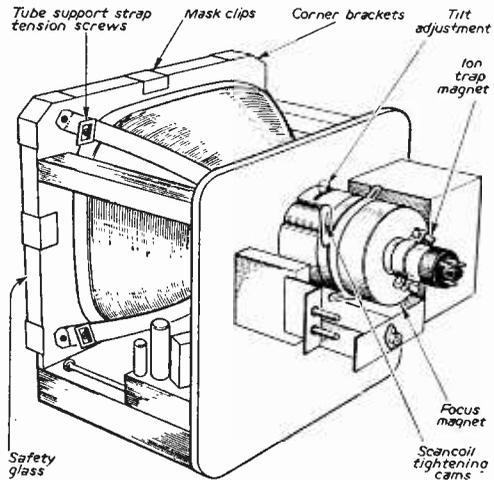
Fig. 11.—Tube and chassis, Pye V14 and V14C.
