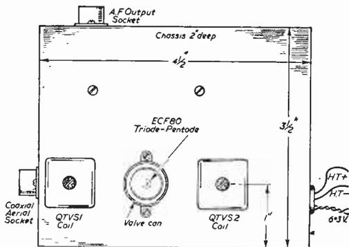
Fig. 2.—Plan view of the chassis.
