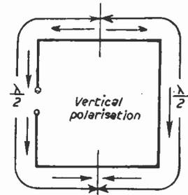
Fig. 2.—Distribution of current in a vertically polarised aerial—driven member.
