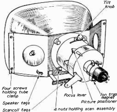
Fig. 8.—Tube and clamp assembly of Pye V4 and VT4.
