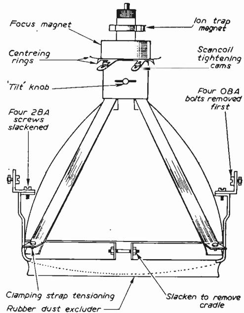
Fig. 7.—Tube and cradle of Pye Continental series with wired chassis.
