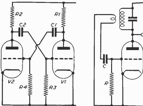
Fig. 1 (Left).—Pulse-producing multivibrator.
