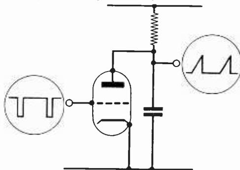
Fig. 7.—Production of triangular pulses.
