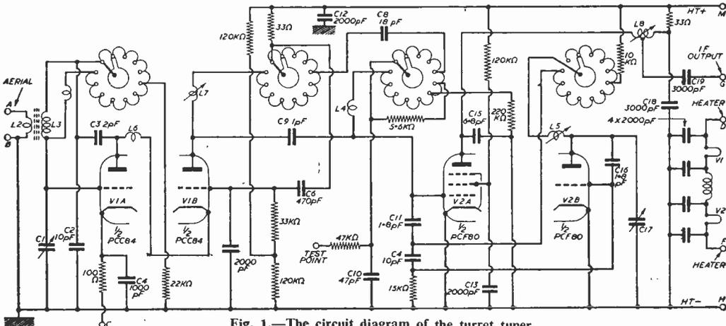
Fig. 1.—The circuit diagram of the turret tuner.
