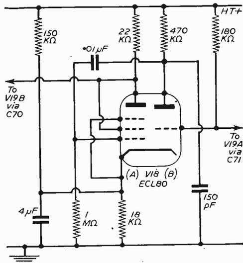
Fig. 4.—Frame interlace filter and clipper section.
