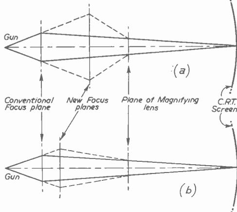
Fig. 15.—Focusing requirements imposed by magnifying lens: Optical Analogy in which the lenses have been replaced by their principal planes. Solid lines represent extremes of beam in conventional tube. Dotted lines show modification imposed by magnifying lens.
