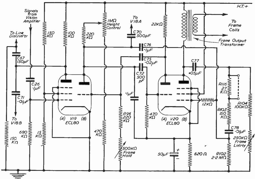
**Fig. 3.**—Frame timebase and sync separator sections.
