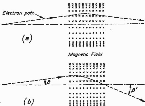
Fig. 12.—Diagrammatic representation of deflection in plane at right-angles to that shown in Fig. 11.
