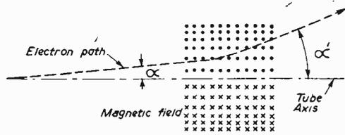
Fig. 11.—Diagrammatic representation of basic scan magnification system.
