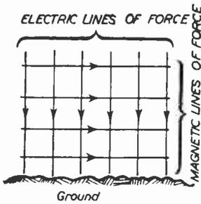
Fig. 1.—The lines of force acting on an aerial.
