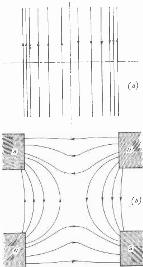
Fig. 13.—Realisation of magnetic field for basic magnification system. (End view of field looking from gun.)
