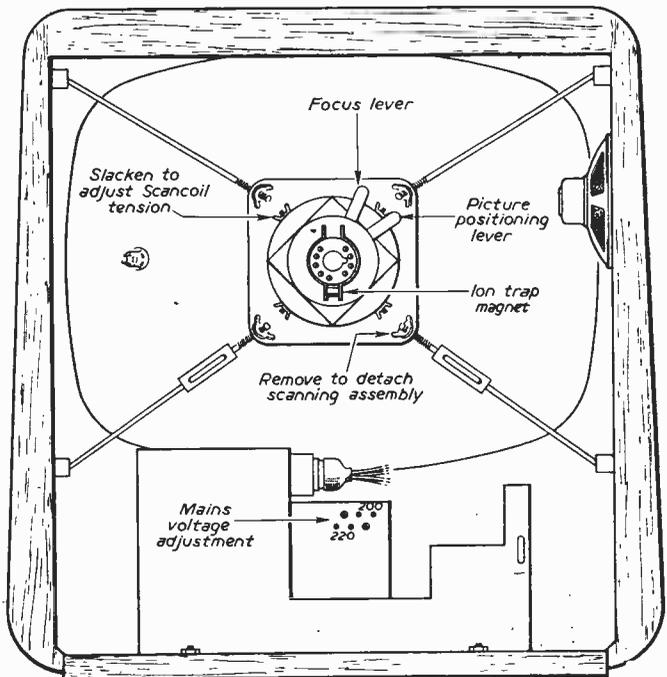
Fig. 9.—Later Continentals, etc., with printed chassis.
