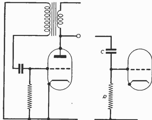
Fig. 3 (Left).—Blocking oscillator.
