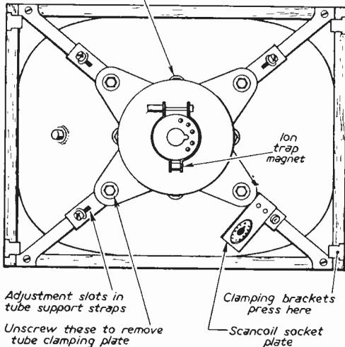
Fig. 10.—Wooden tube cradle assembly Pye VT17 (Luxury 17).
