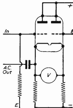
Fig. 6.—Simple D.C. valve voltmeter with high input impedance.
