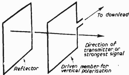
Fig. 5.—How a quad aerial pair should be sited in relation to the transmitter.
