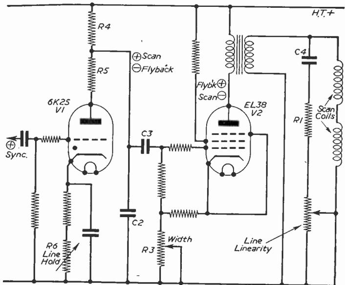
Fig. 24.—A thyratron timebase circuit.
