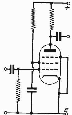
Fig. 7.—Circuit of the sync amplifier.
