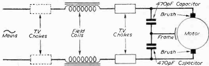
Fig. 1.—Showing how to include the chokes.
