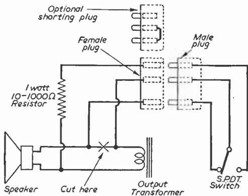
Fig. 1.—The constructional details.
