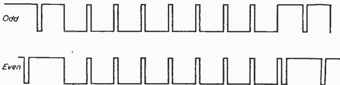
line pulse) than is the case on even frames, the resulting voltage starts off at a somewhat greater value. In other words, the sync voltage for odd frames builds up at a greater rate from a higher initial level; the pulses are slightly different for the two frames, and good interlace cannot be obtained—except perhaps by accident.
