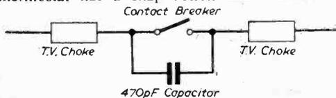
Fig. 2.—A suppressor system for thermostats.
