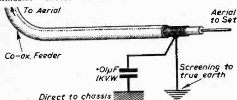
Fig. 3.—The screening of the coaxial lead should be connected direct to earth.
