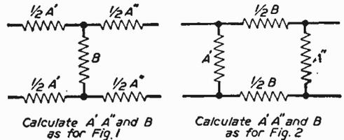
Fig. 6.—Networks for a balanced line.
