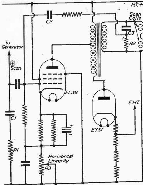
Fig. 25.—Line output stage with feedback network for linearity.
