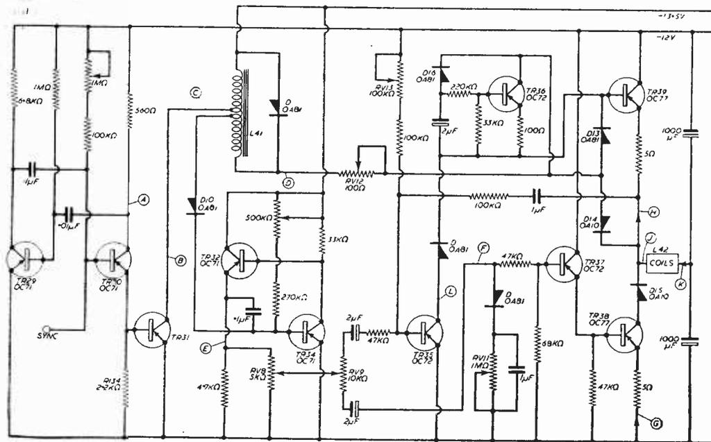
Fig. 25 (b).—The circuit of the field timebase.
