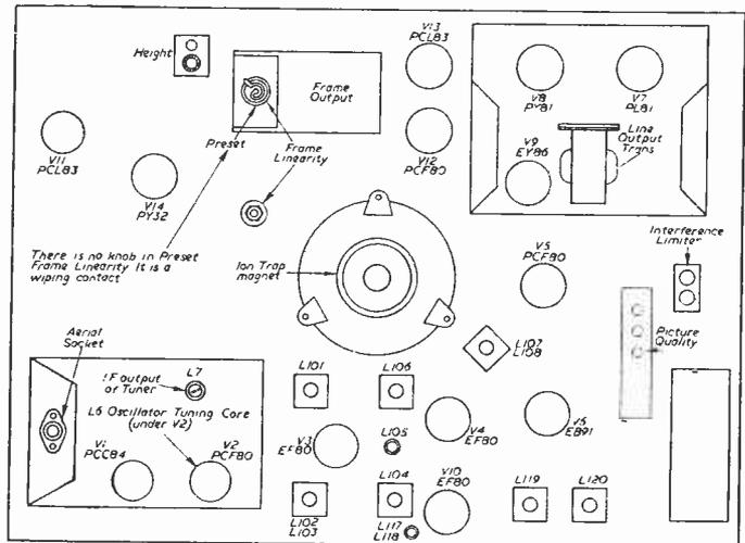
Fig. 1.—Rear view of chassis.
