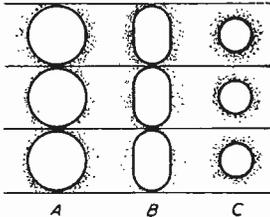
Fig. 2(a).—If the spot is defocused, the gaps disappear, but definition is impaired. (b) Improving horizontal definition. (c) A correctly focused spot leaves gaps.
