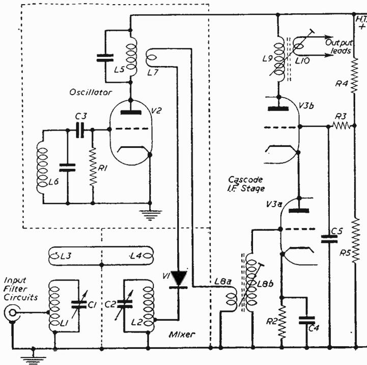
Fig. 1.—Circuit diagram of the converter.
