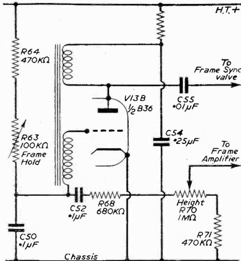
Fig. 2.—The frame oscillator section of the BT2147.
