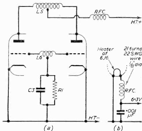
Fig. 2(a) (Left)—Tuned-anode, tuned-grid oscillator circuit.
