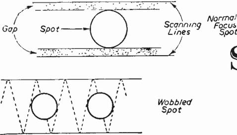
Fig. 1.—With a normally focused spot, there are gaps between the scanning lines. If the spot is “wobbled,” the gaps are filled.
