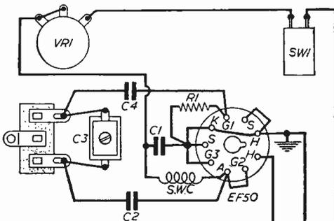
Fig. 4.—Wiring diagram. Note: Earth the valve holder spigot. LT+ HT- H.T. LT- +
