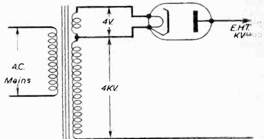
Fig. 29.—Mains driven EHT (negative supply).
