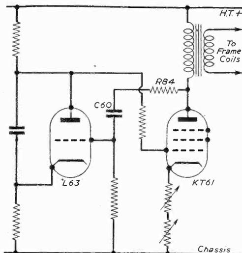
Fig. 1.—Frame timebase of the BT1091. C60 is prone to failure.
