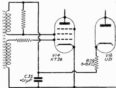
Fig. 3.—Basic circuit of the line amplifier of the BT5145.
