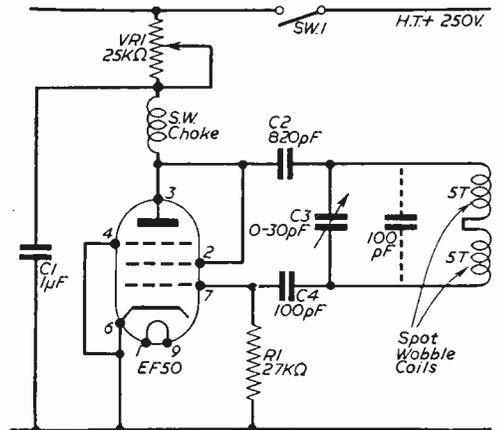
Fig. 3.—Circuit of the oscillator using an EF50.
