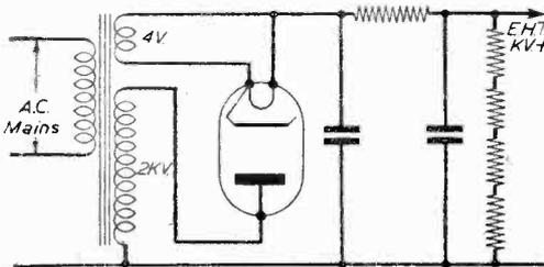
Fig. 28.—Mains driven EHT (positive supply).
