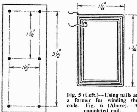
Fig. 5 (Left).—Using nails as a former for winding the coils. Fig. 6 (Above).—A completed coil.
