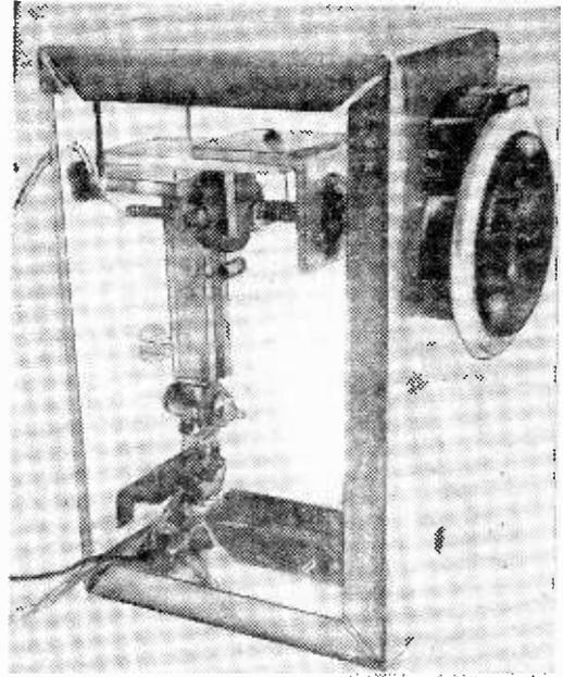
The oscillator works with the cathode choked and, because the heater-cathode capacitance represents only a small impedance at the frequencies covered, the heater is also choked so as to remain at the same R.F. potential as the cathode. The inclusion of chokes in these leads also has
