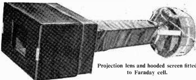
Projection lens and hooded screen fitted to Faraday cell.
