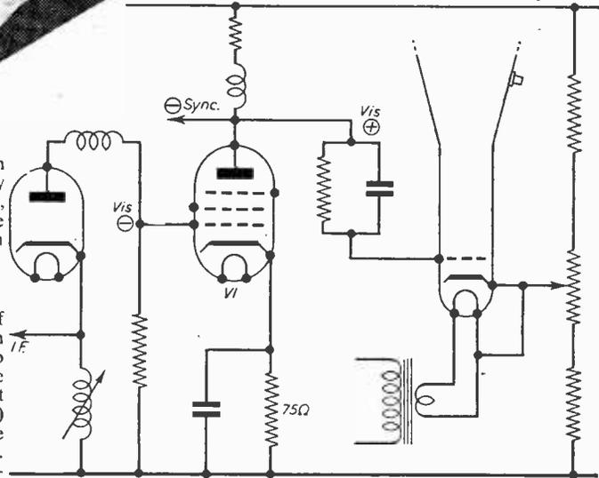
Fig. 36—Grid modulation (and the use of an isolating heater transformer).
