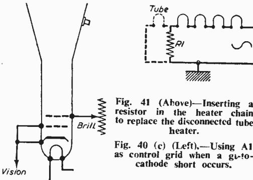
Fig. 41 (Above)—Inserting a resistor in the heater chain to replace the disconnected tube heater.
