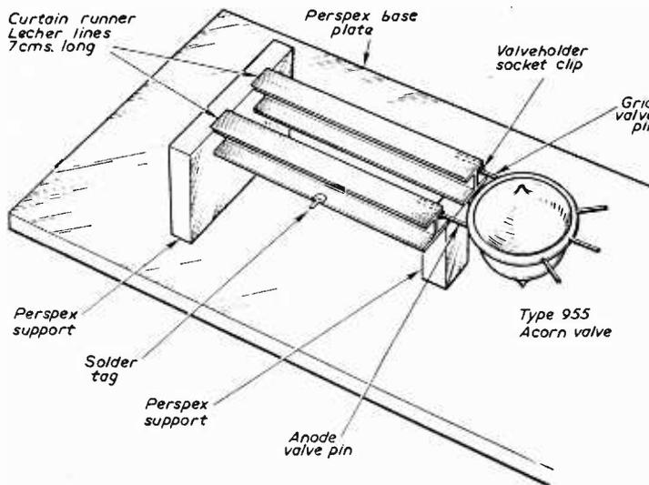
Fig. 3.—Mounting the Lecher lines and valve on the Perspex baseplate.
