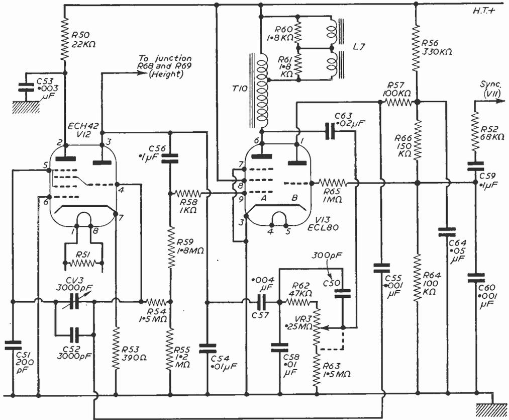
Fig. 4.—Frame oscillator and output stages.
