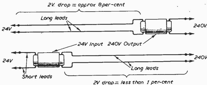
Fig. 1.—With low voltages, voltage drop is particularly serious.
