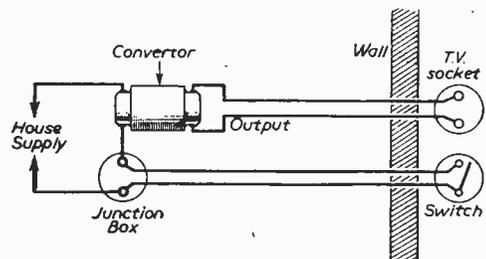
Fig. 2.—Connecting an input switch.
