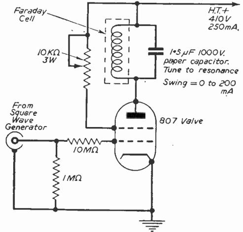
Fig. 7.—Circuit of the Faraday cell driver unit.
