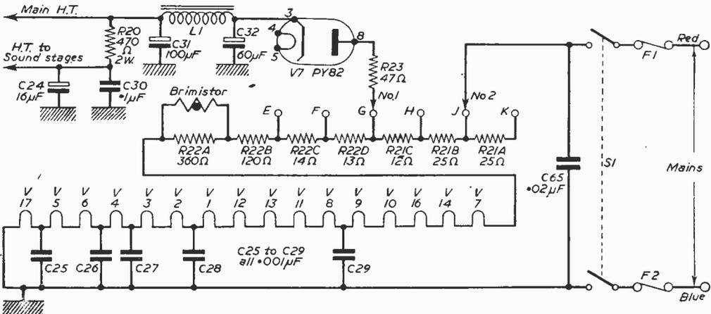
Fig. 3.—Heater wiring and the H.T. supply.
