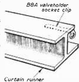
Fig. 2.—Fitting the valveholder sockets to the Lecher lines.
