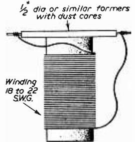
Fig. 4.—Small suppressor chokes.
