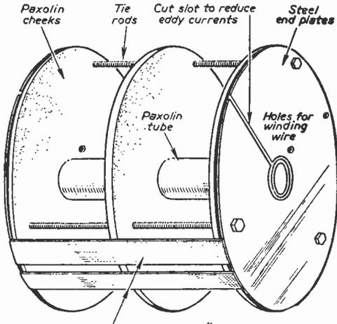
Tinned steel strips 1" wide with  $\frac{1}{8}$ " gap between should make good contact with end plates. Bind on with insulating tape
