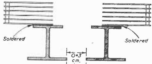
Fig. 4.—The "butterfly" stator plates are soldered to the Lecher lines.
