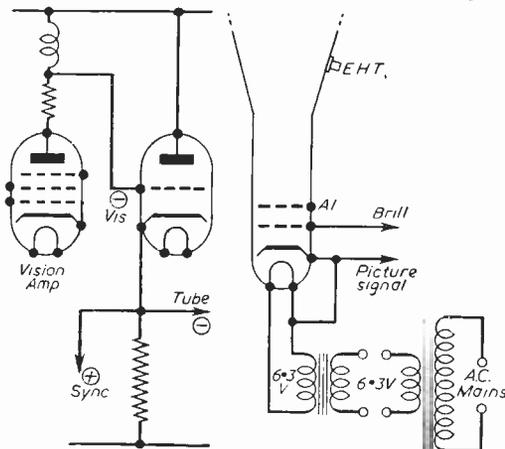
Fig. 38 (Left)—Feeding the cathode follower direct from the anode of the video amplifier.
