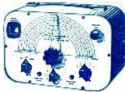
£6.19.6 or 25/- deposit and 6 monthly payments of 21/6. P. & P. 5/- extra. Coverage 100 Kc/s-100 Mc/s on fundamentals and 100 Mc/s to 200 Mc/s on harmonics. Metal case 10in. x 6in. x 5in., grey hammer finish. Incorporating three miniature valves and Metal Rectifier, A.C. Mains 200/250. Internal Modulation of 40% c.p.s. to a depth of 30%; modulated or unmodulated R.F. output continuously variable. 100 milli-volts.
