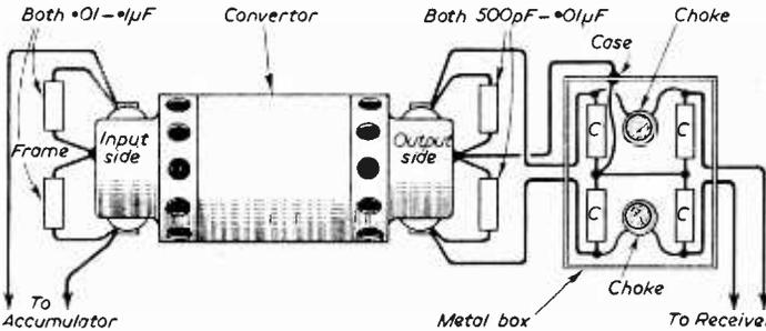
Fig. 3.—Wiring-in suppressor condensers and chokes.
