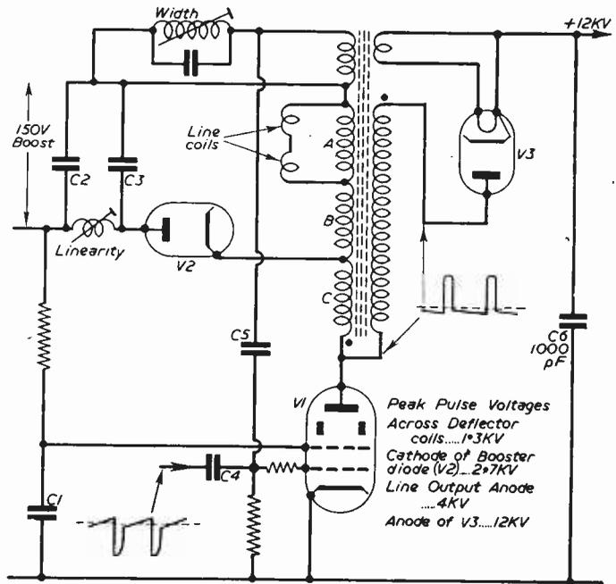
Fig. 7.—Line output stage for 17in. tube.
