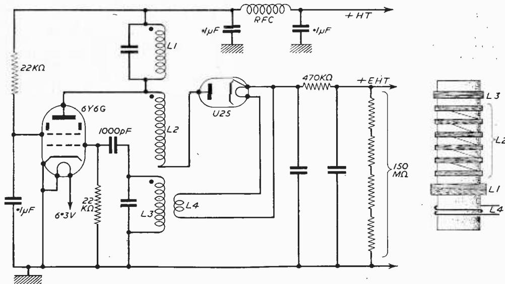
Fig. 6.—Positive R.F. EHT supply for a picture tube.
