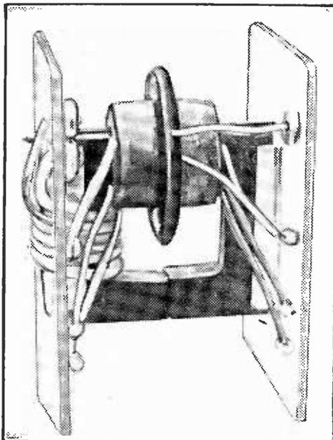
A home-constructed line-output transformer.
