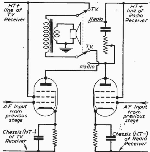
Fig. 1.—Changeover switching for feeding output transformer from TV or radio.
