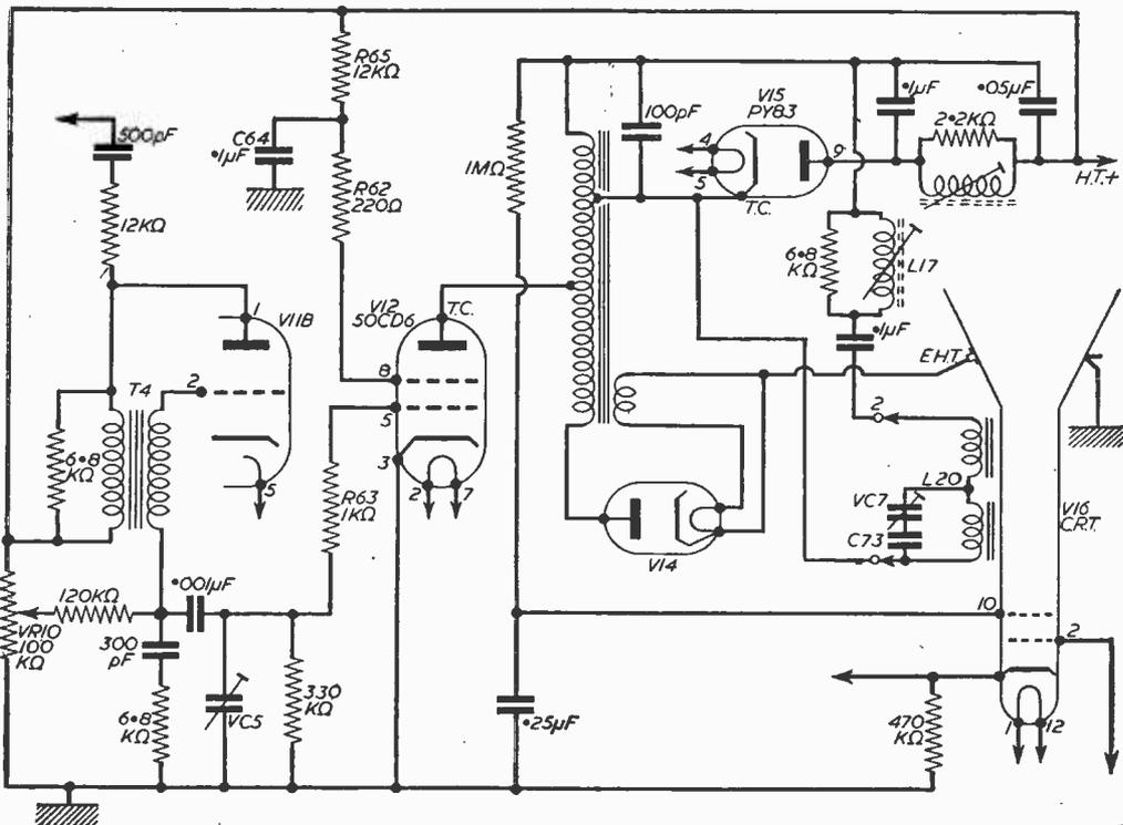
Fig. 3.—Line timebase circuit.
