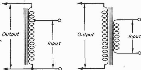
Fig. 1.—Auto and two-winding transformers.
