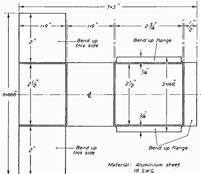
Fig. 3.—Making the chassis.
