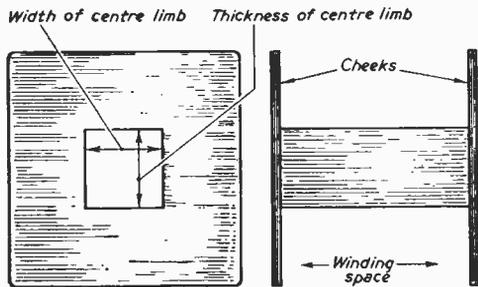
Fig. 2.—Bobbin and core size.
