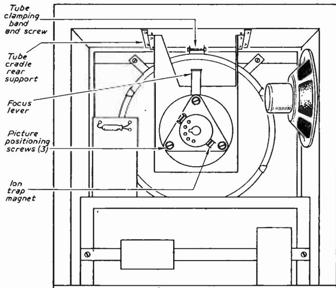
Fig. 4.—Cosor 927; rear view of cabinet and chassis.
