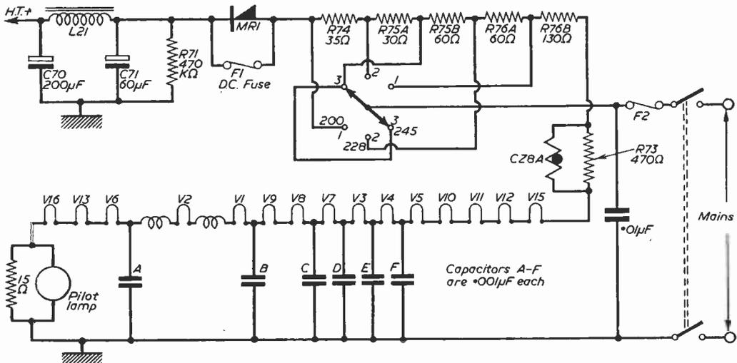
Fig. 1.—H.T. and heater circuits (V16 is the C.R. tube).
