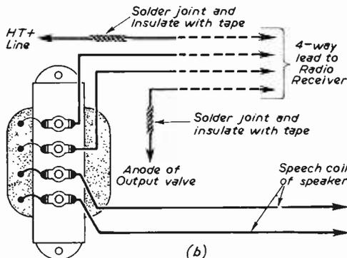
Fig. 3b.—Connections after modification. Note that in some output transformers, the position of the various tags may differ from the above (see text for identification).
