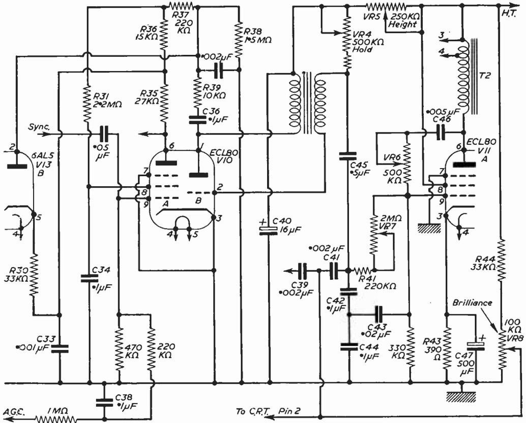
Fig. 4.—Frame timebase circuit.
