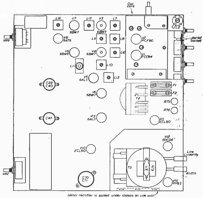
Fig. 2.—Plan view of chassis.
