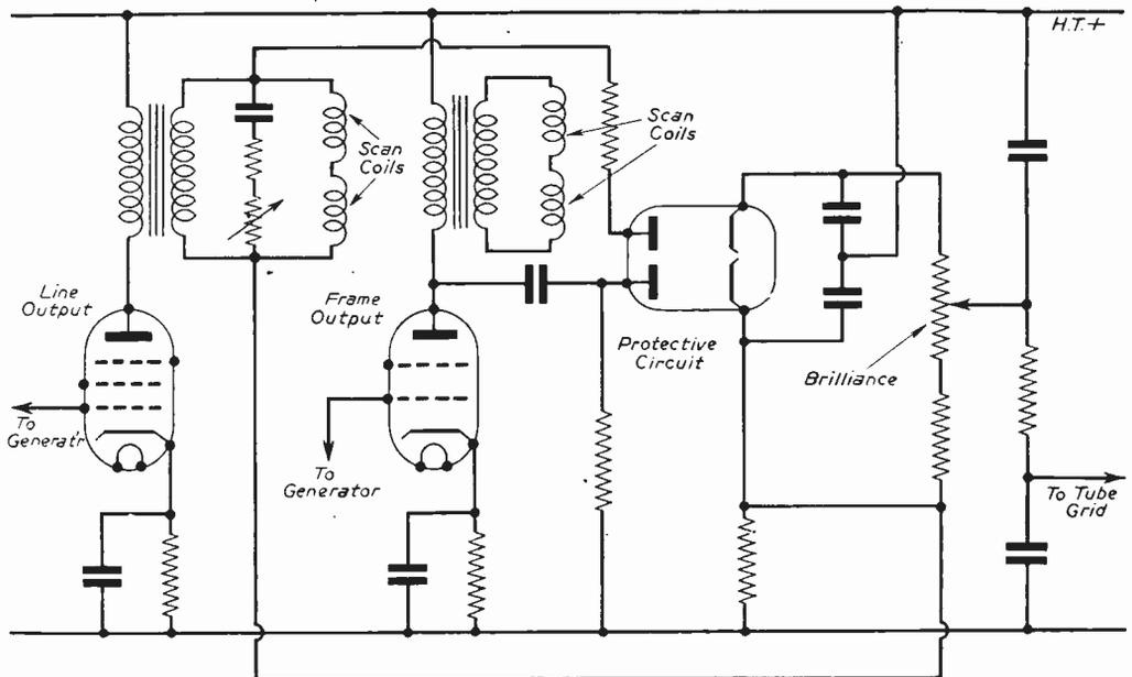
Fig. 49.—Projection tube protection circuit.
