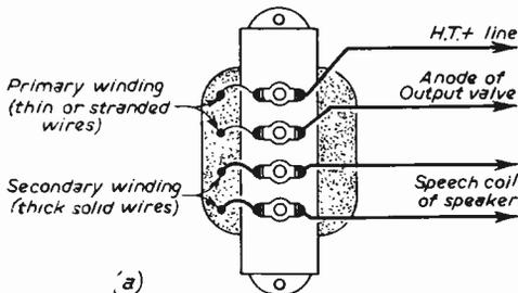
Fig. 3a.—Connections to output transformer before modification.
