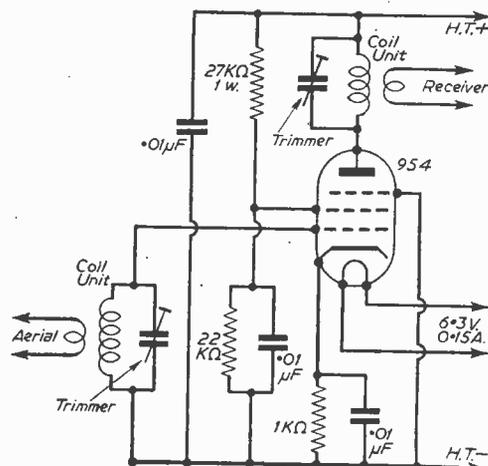
Fig. 1.—The circuit diagram. Power is obtained from the H.T. and L.T. supplies of the receiver.
