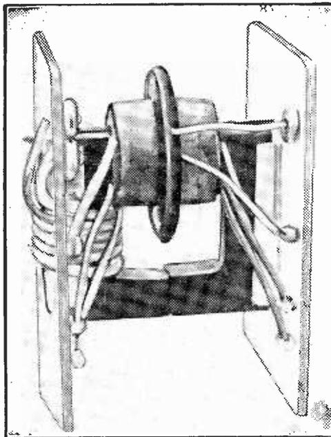
A home-constructed line-output transformer.
