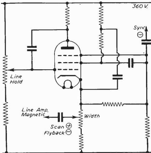
Fig. 52.—Miller transitron timebase.
