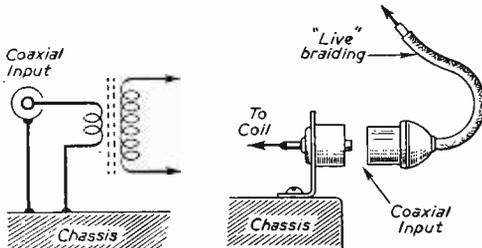
Fig. 3.—How the aerial connection may be "live".
