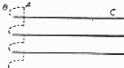
Fig. 1.—Section of raster showing foldover on line.
