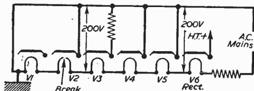
Fig. 59.—An open-circuit heater chain.
