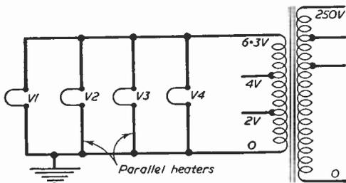
Fig. 55.—Parallel heater circuit.
