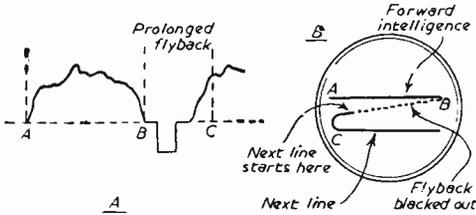
Fig. 4.—Waveform when flyback is late.
