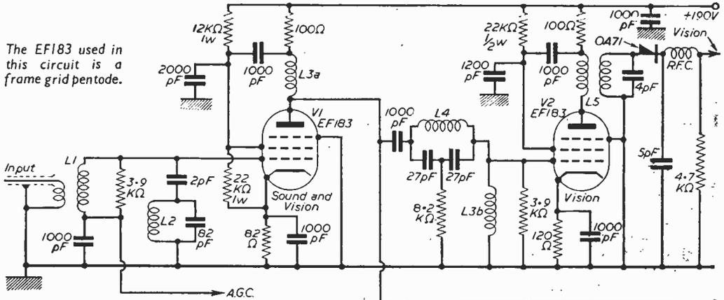
The EF183 used in this circuit is a frame grid pentode.
