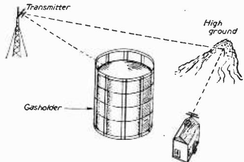
Fig. 3.—If there is an obstacle between the transmitter and the receiving aerial, a reflected signal can sometimes be utilised.
