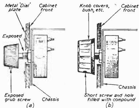
Fig. 2.—The danger of exposed metal parts.
