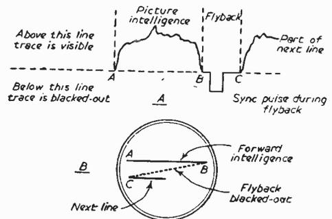
Fig. 3.—Waveform for one line.
