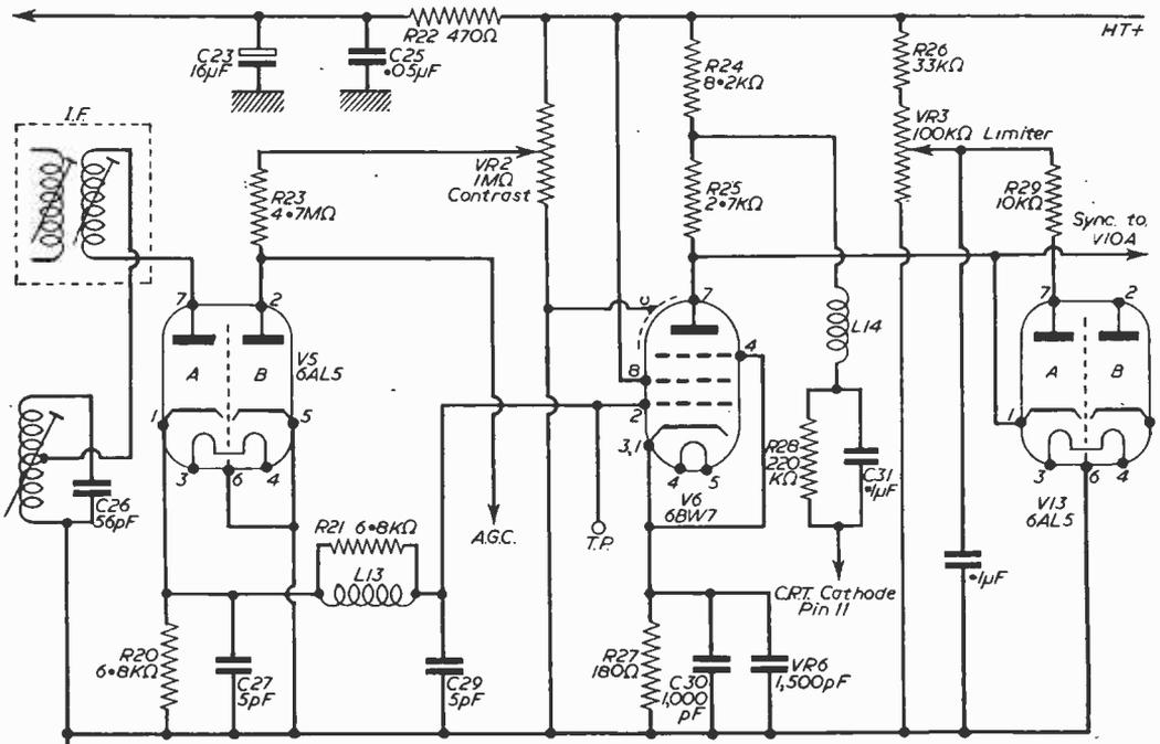
Fig. 1. — Vision detector, AGC diode, video amplifier, vision limiter and H.T. feed (via R22) to early stages.
