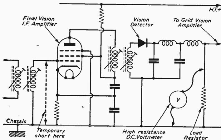
Fig. 2.—Instability may show as a constant voltage across the vision detector load resistor with the aerial disconnected from the set. This is proved by the voltage collapsing when a short is applied to the control grid of the final vision I.F. valve.
