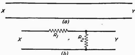
Fig. 1.—Diagram illustrating characteristic resistance of lines.
