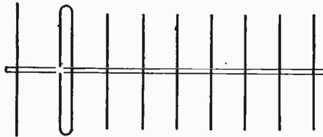
Fig. 2.— Typical multi-element aerial array. These arrays are often used indiscriminately in areas of poor signal strength; the most complicated array is not necessarily the optimum for a given location as much depends on the effects of reflections.
