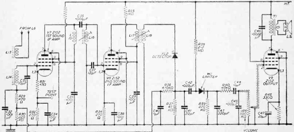
Fig. 6.—Circuit of the sound strip.
