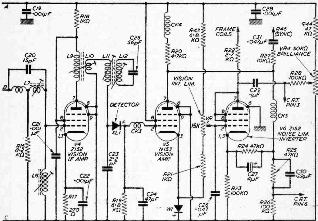
in a lack of voltage at the screen or anode and of course in the case of R13 the sound will also be almost entirely absent. These resistors often burn out as a result of a shorted  $0.001\mu\text{F}$  decoupling capacitor or an internal short in a Z152 valve. Thus when a short is recorded at pin 8, before disconnecting the  $0.001\mu\text{F}$ , always remove the Z152 to see if this is responsible after all.
