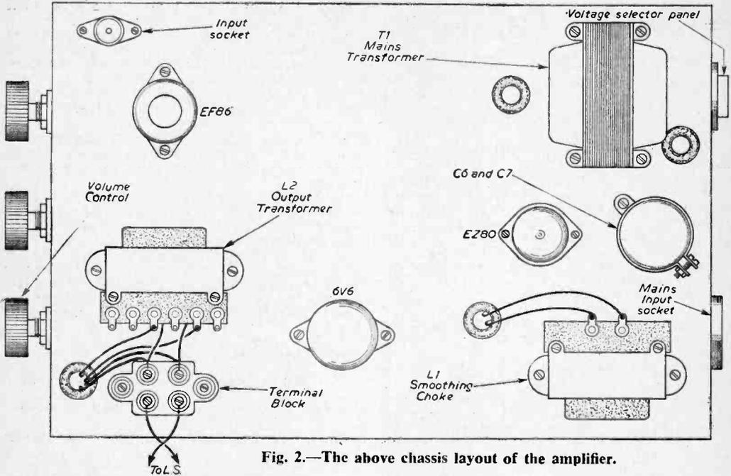
Fig. 2.—The above chassis layout of the amplifier.
