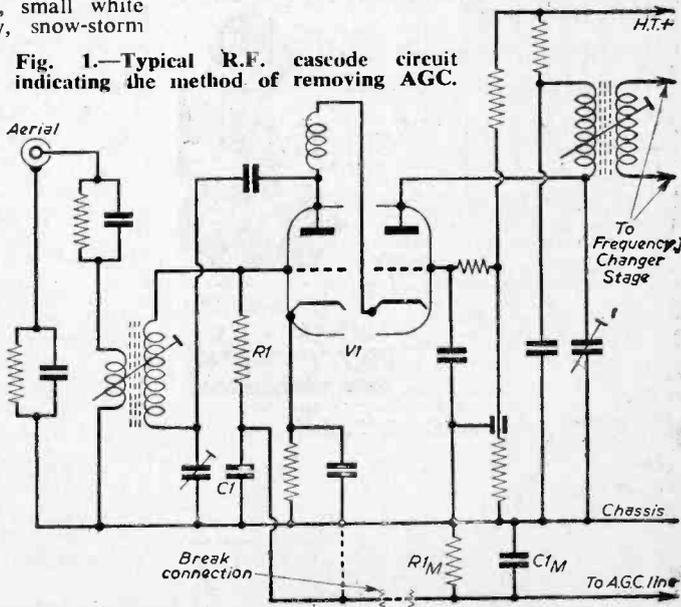
Fig. 1.—Typical R.F. cascode circuit indicating the method of removing AGC.
