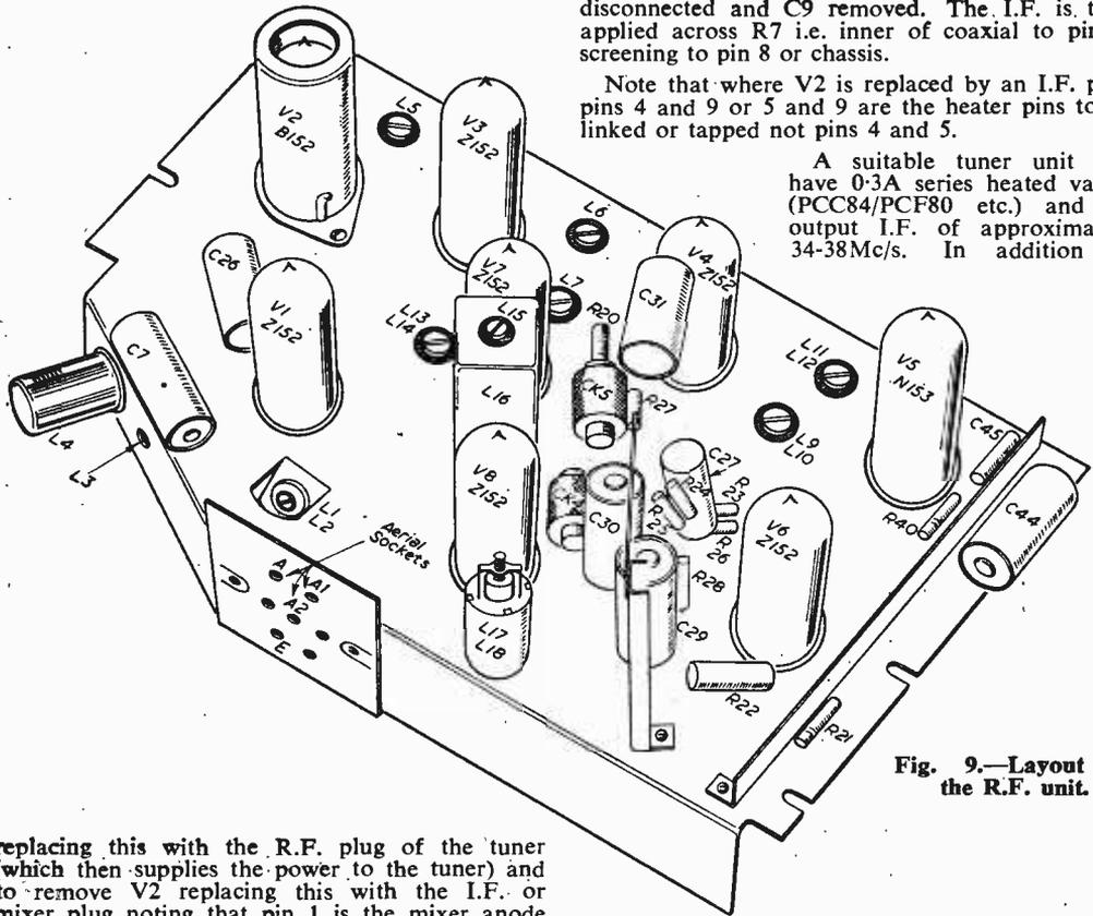
Fig. 9.—Layout of the R.F. unit.
