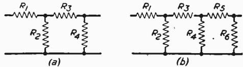
Fig. 2.—Rearrangement of line characteristic resistances.
