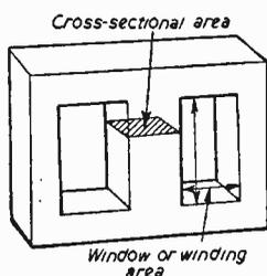
Fig. 2.—A typical transformer core, showing the cross-sectional and window areas.
