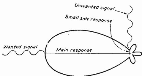
**Fig. 8.**—An aerial response pattern as shown may well be necessary to obtain maximum discrimination between the wanted and unwanted signals.
