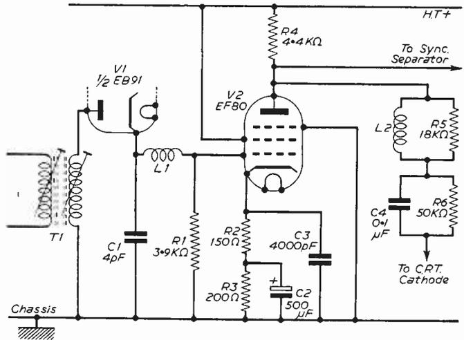
Fig. 2.—Typical vision detector and video amplifier stages. Note the direct coupling from the detector to the amplifier.
