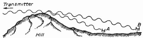
**Fig. 6.—**Owing to the greater diffraction of Band I signals than Band III signals, a receiver at "A" at the foot of the hill may obtain Band I signals only, while at "B" both Band I and Band III signals would be received.
