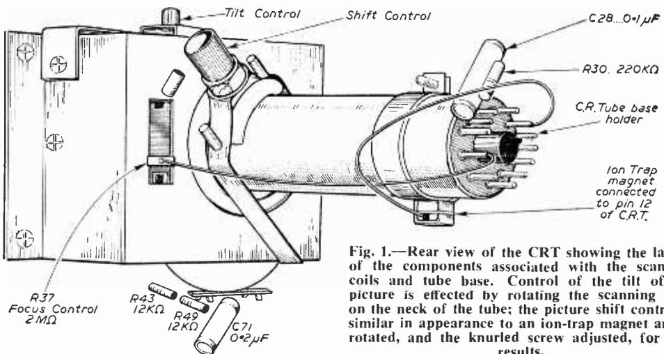
Fig. 1.—Rear view of the CRT showing the layout of the components associated with the scanning coils and tube base. Control of the tilt of the picture is effected by rotating the scanning coils on the neck of the tube; the picture shift control is similar in appearance to an ion-trap magnet and is rotated, and the knurled screw adjusted, for best results.
