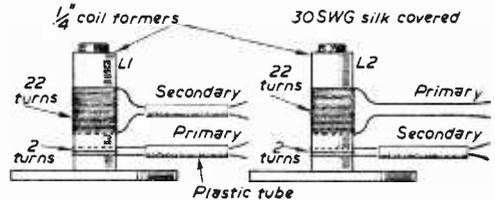
Fig. 3.—The I.F. coil details.
