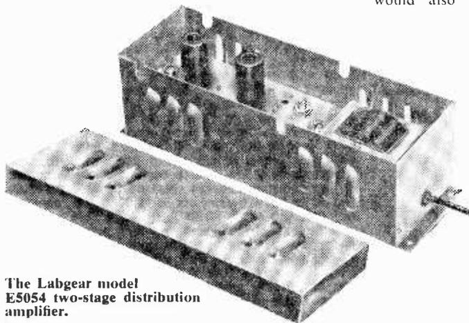
**The Labgear model E5054 two-stage distribution amplifier.**
