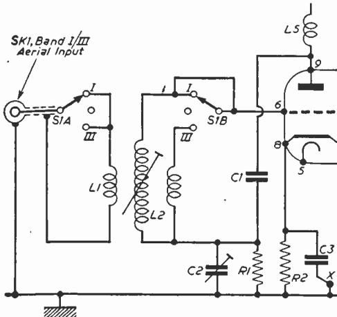
Fig. 1.—The alternative input circuit.
