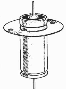
Fig. 5.—Lead-through condenser.
