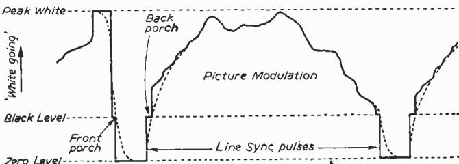
Fig. 1.—One line of a television signal between two line sync pulses. The dotted line shows the distortion of the theoretically ideal wave-shape which results from too great a rise-time in the amplifier.
