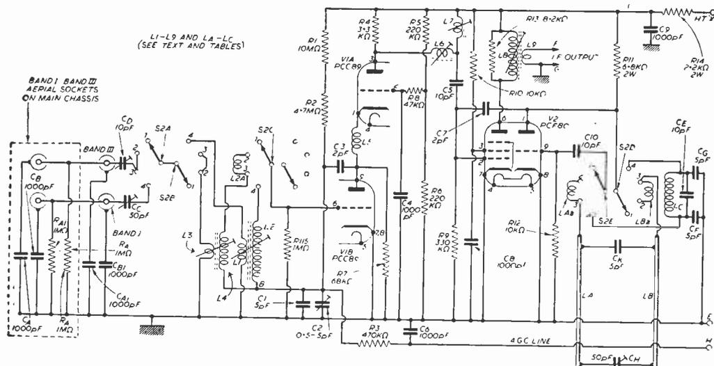
Fig. 1.—The circuit diagram of the tuner unit. (The cathode of the input triode—V1B—may be decoupled by C67, as on the blueprint, if necessary. Condensers C10 and C5 are N750K.)
