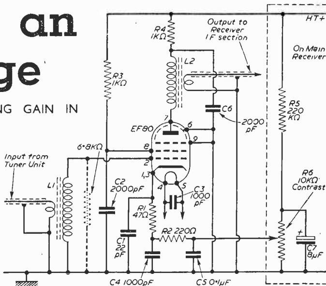
Fig. 1.—The circuit diagram.
