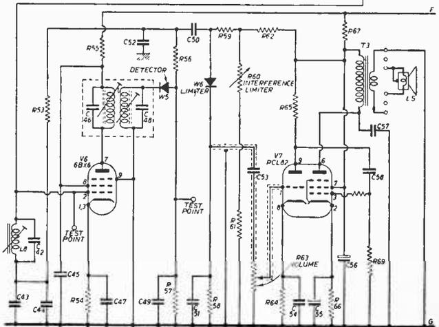
Fig. 3 (a) and, opposite, (b).—Circuit diagram of the Cossor 948 receiver.
