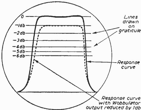
Fig. 7.—Calibrating the C.R.T. graticule using an attenuator.
