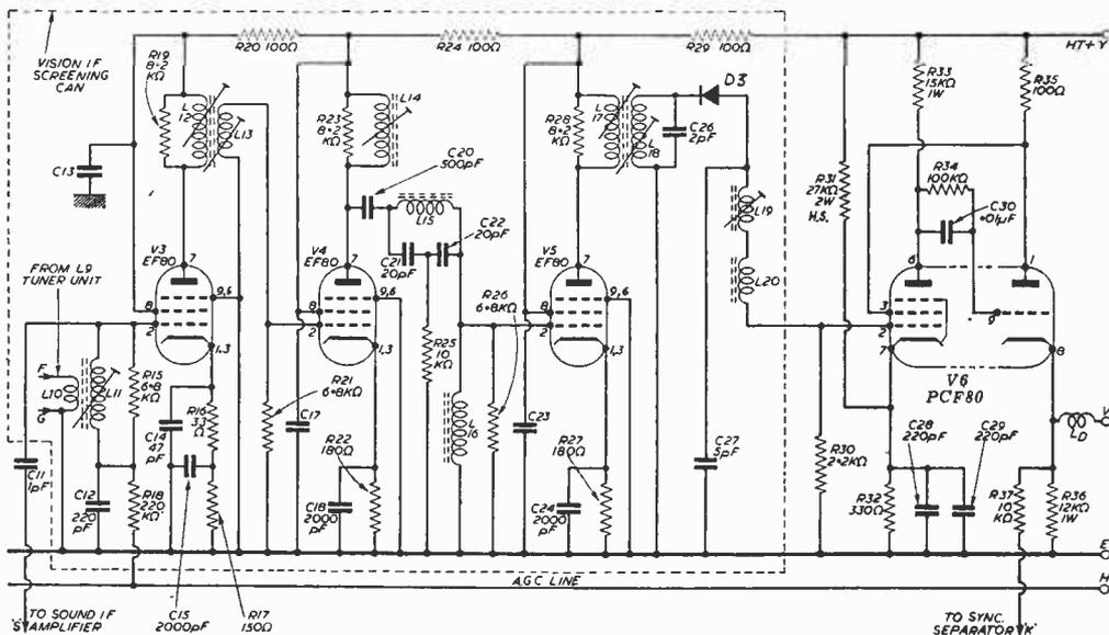
Fig. 2.—Vision I.F. circuits. (Notes: Condensers C21 and C22 are  $\pm 5$  per cent; C21, C22 and C26 are all silver-mica. R31 is a High Stability component. Condensers C13, C17 and C23 consist of two 2000pF components in parallel. Components C26 and D3 are included in the can of L17/18 and therefore do not appear on the blueprint.)
