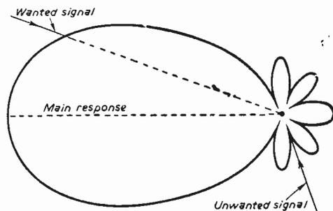
**Fig. 10.**—If there is one major interfering signal, an aerial with a relatively wide forward lobe may be orientated to give maximum rejection of the interfering signal without unduly affecting the pickup of the wanted signal.
