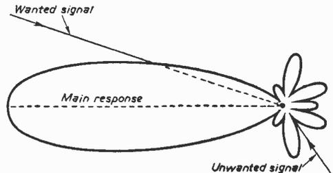
Fig. 11.—This diagram shows how the response to the wanted signal could be severely reduced if an aerial with a narrow forward lobe were orientated to reduce the response to an interfering signal coming in towards the rear. Nevertheless, an aerial with a narrow forward lobe may be required to reduce interference coming in from a variety of directions.
