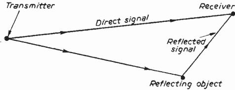
**Fig. 4.—**The extra distance over which a reflected signal may travel, in relation to the direct signal, can be determined by the displacement of the resulting ghost from the main image.
