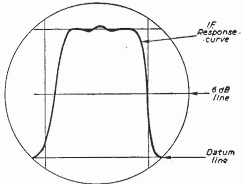
Fig. 5.—Assessing relative amplitudes within the display.
