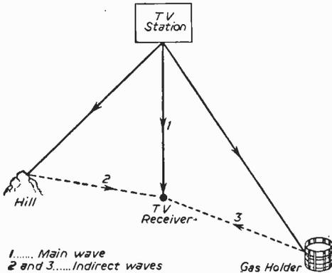
Fig. 1.—Reflected and direct signals.
