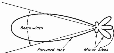
**Fig. 9.**—As more elements are added to an aerial to provide a narrow forward lobe and extra high gain with small beam, width, subsidiary minor lobes tend to develop, as shown.
