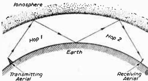
**Fig. 1.**—Reflection from the ionosphere enables signals to travel long distances. (This does not happen with signals about 30Mc/s.)
