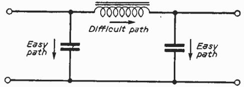
Fig. 3.—Behaviour of filter circuit at low frequencies.
