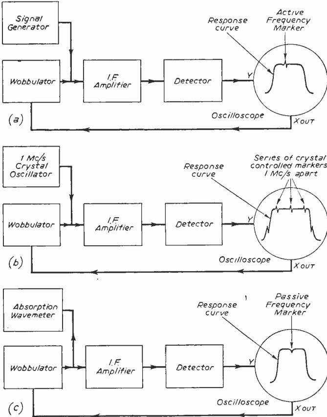
Fig. 6.—Three types of frequency marker.
