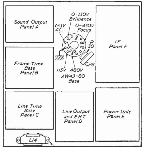
Fig. 2 (Right).—Layout of the printed panels, viewed from the rear.
