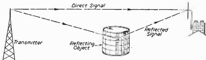
Fig. 3.—Reflections of the transmitted signal may cause "ghosts" on the picture. This effect may be confused with "ringing" intentionally introduced in the video amplifier.
