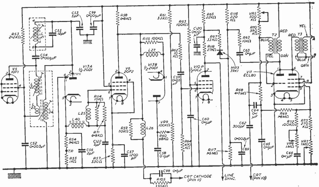
Fig. 1.—The video amplifier, sync separator and frame timebase circuits.
