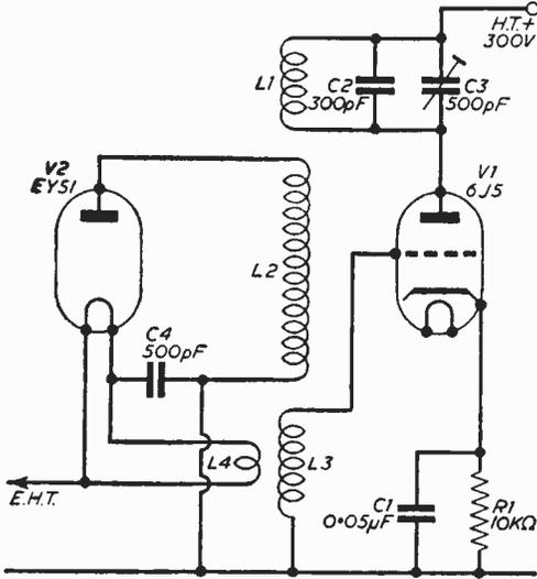
Fig. 3.—Circuit of the R.F. oscillator EHT unit.
