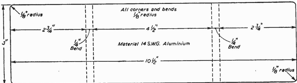
Fig. 8.—Dimensions of the chassis of the tuner and inter-stage screen.
