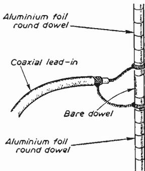
Fig. 2.—The method of making the elements from aluminium foil.
