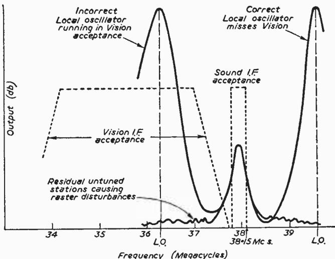
Fig. 4.—Correct and incorrect local oscillator settings.
