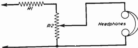
Fig. 3.—Low impedance circuit with volume control.
