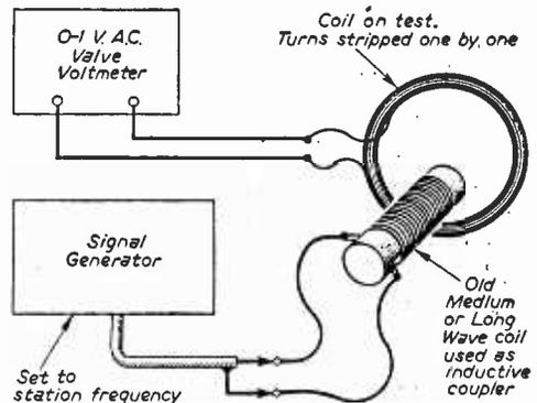
Fig. 3.—Pre-tuning the coils.
