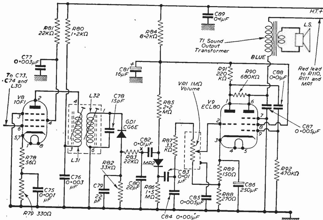
Fig. 4.—The sound detector, limiter and A.F. output stage circuits. ('X' marks a test-point)
