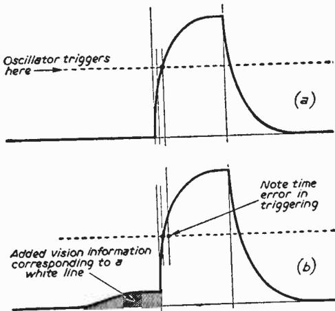
Fig. 8a—Normal line sync pulse.
