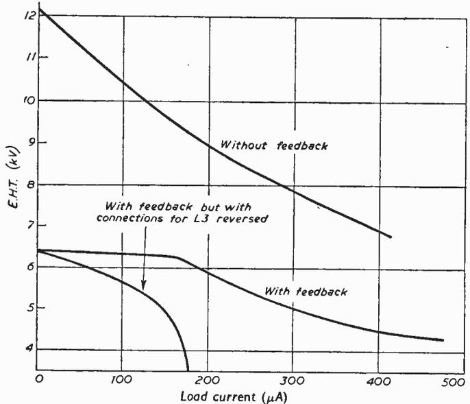
**Fig. 6.—Regulation of ringing choke system.**
