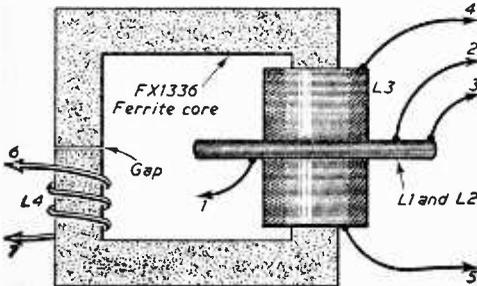
**Fig. 7.—Construction of the transformer.**
