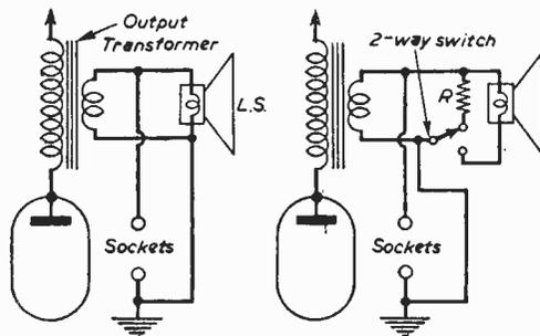
Fig. 1.—Connections for a receiver with an earthed chassis.
