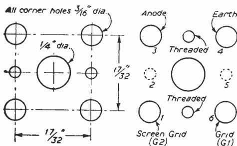
Fig. 4.—(left) Chassis drilling details for the I.F. transformers, and (right) the coil connections.
