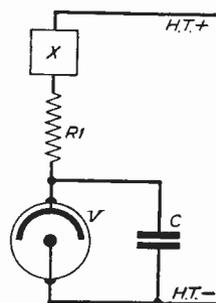
Fig. 1.—Simple neon tester for capacitors.
