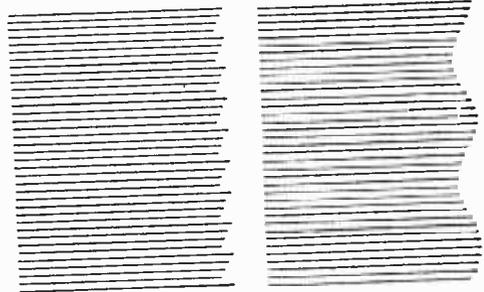
Fig. 9 (left)—A form of poor sync which may occur when a capacitor is used in series with the deflection coils.
