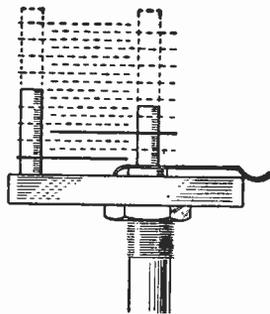
Fig. 5.—Modifications to the tuning condenser to leave one moving and one fixed vane.
