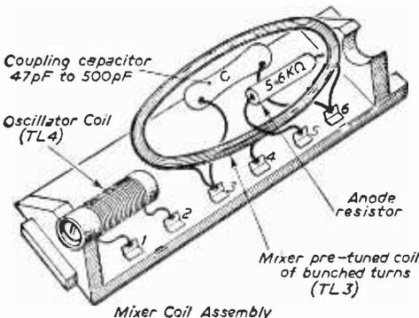
Fig. 2.—Mixer coil assembly.
