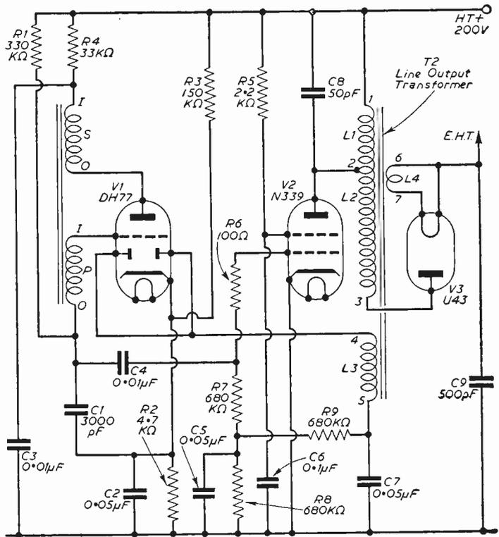
**Fig. 5.—Ringing choke circuit.**
