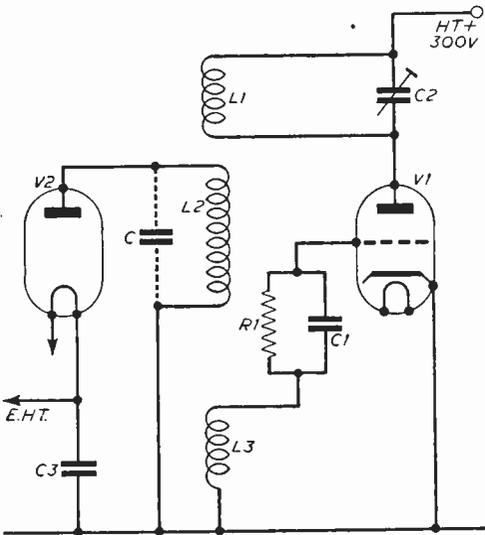
Fig. 1.—R.F. oscillator circuit (grid-leak bias).
