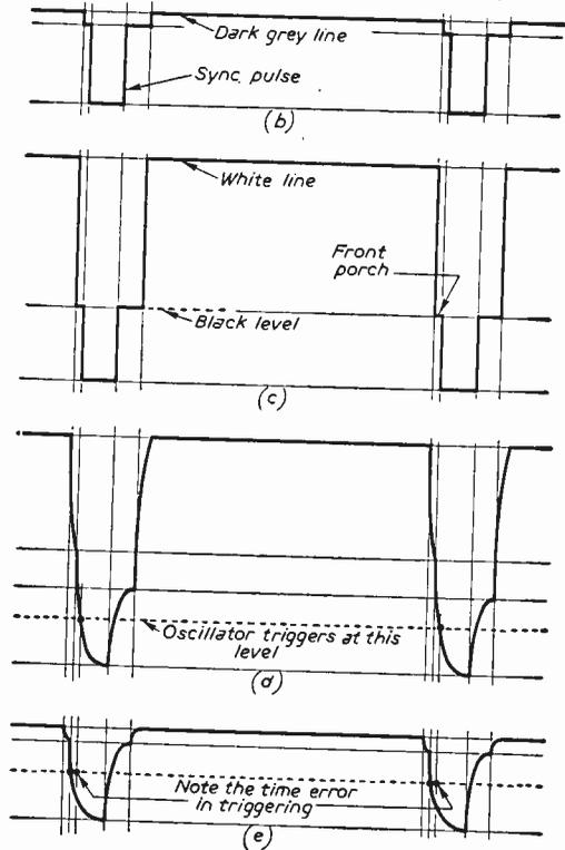
**Fig. 7b—Ideal signal waveform corresponding to the dark grey lines of Fig. 7a.**
