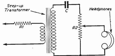
Fig. 4.—Impedance matching and top-boost circuit.
