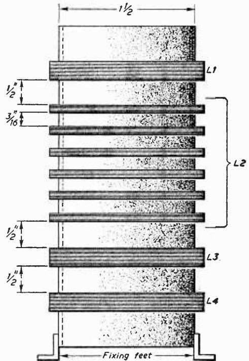
Fig. 4.—R.F. oscillator coil construction.
