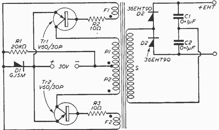
Fig. 8.—A practical circuit to provide 5kV.
