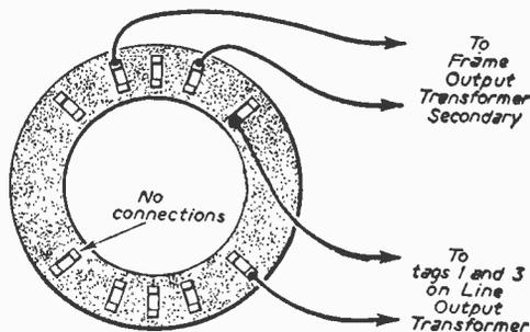
Fig. 20.—The scanning coil connections.
