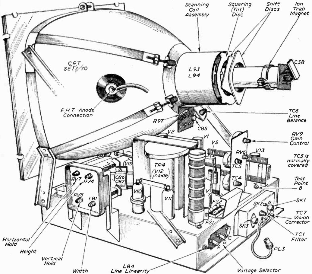
Fig. 7.—A view showing the CRT position of the HMV 1854.
