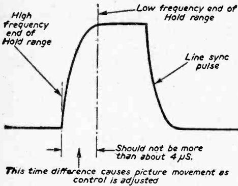
Fig. 19.—Sloping sync pulses cause picture movement when the hold control is adjusted.
