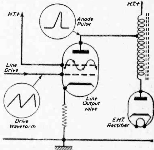
Fig. 2 (above).—The basic circuit of a line output stage and its waveforms. The sinuous arrow traces the path of the electrons.
