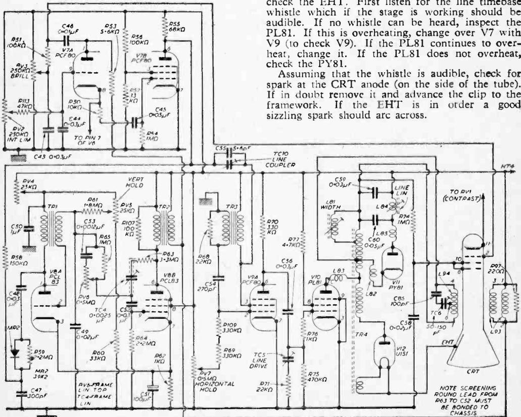
Fig. 6.—The timebase circuit.
