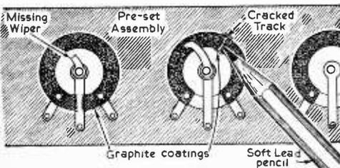
Fig. 2.—Repairing broken pre-sets.
