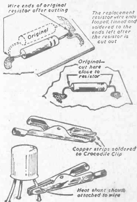
Fig. 2.—Making heat shunts for removing transistors.
