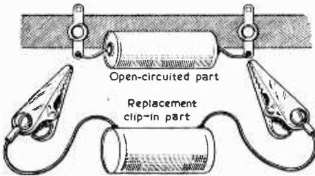
Fig. 1.—Bridging an open-circuit component in a restricted position.
