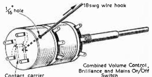
Fig. 3.—Loosening welded mains contacts.
