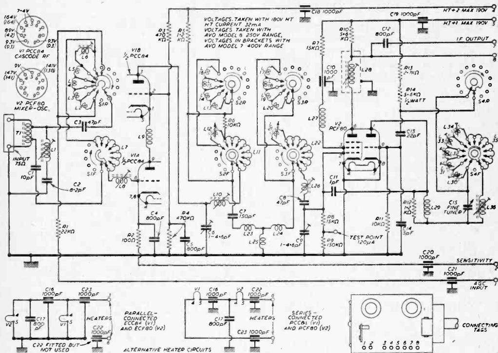
Fig. 6.—The circuit diagram of a switch tuner.
