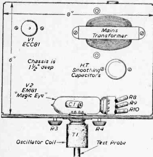
Fig. 3 (above)—An above-chassis view.
