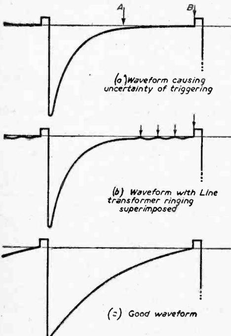
Fig. 20.—Grid waveforms and their effect on synchronization.
