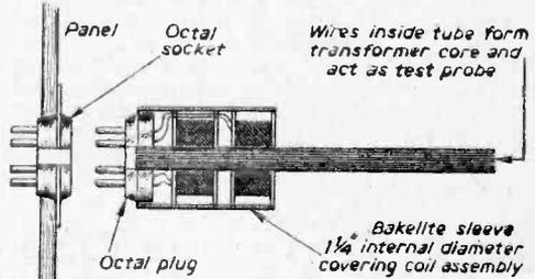
Fig. 6.—The completed probe, with the octal plug attached (the core is formed from iron wires).
