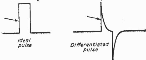
Fig. 17.—(above) Sync pulses with steep leading edges.
