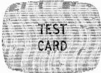
Fig. 10. (above left).—R.F. interference gives moving patterns on the screen rather like moiré silk.
