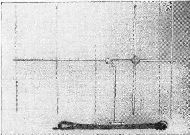
A complete Band III aerial which can be made from a Ben Nevis kit.
