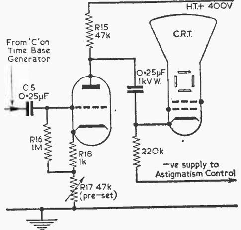
Fig. 10 (above).—The cathode connection to the CRT, with flyback blanking.
