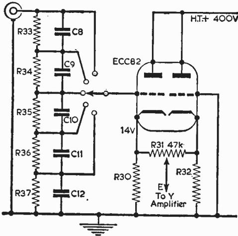
Fig. 12.—The input attenuator and cathode-follower input to the Y-amplifier. R30 and R32 are equal in value (2.2k) and should be matched.
