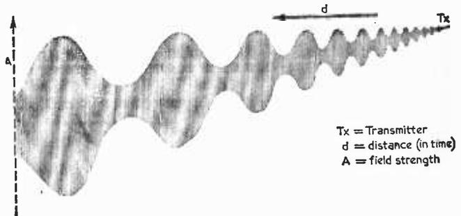
Fig. 1.—The well known representation of an amplitude modulated carrier wave.
