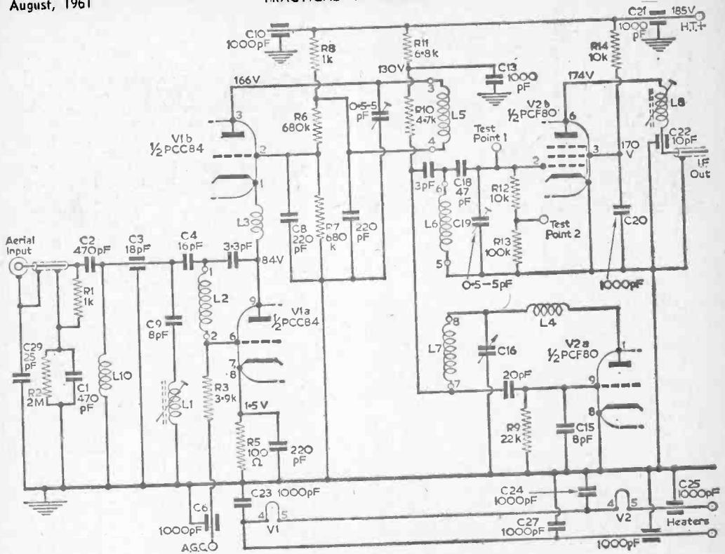
Fig. 3.—The circuit of the tuner.
