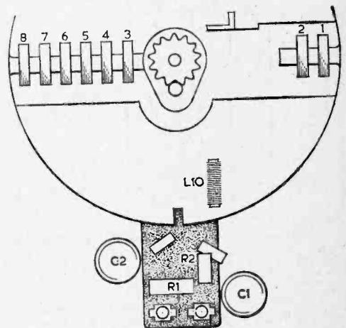
Fig. 4 (right).—The rear of the tuner with the disc removed to show the contacts and the star wheel.
