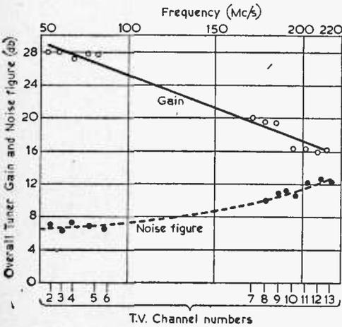
Fig. 2.—The gain and noise figures of the tuner shown in Fig. 1.
