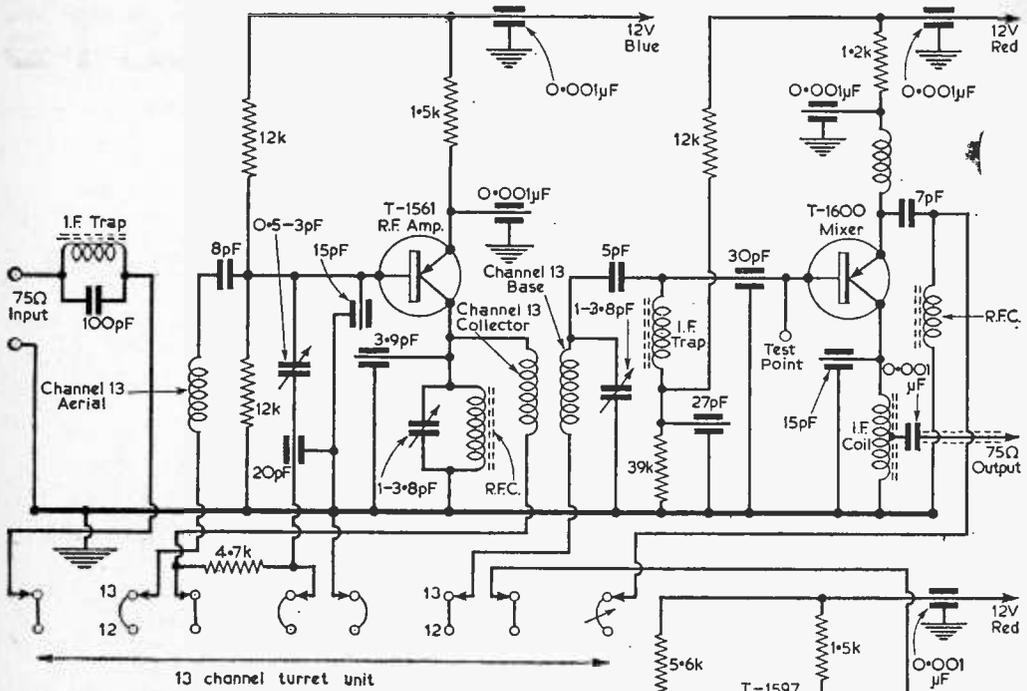
Fig. 3.—The circuit of the Sickles Mark 6T VHF tuner.
