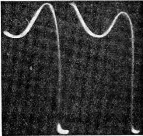
The oscilloscope trace of a screen pulse (for fly-back blanking) :  $f=100kc/s$ .
