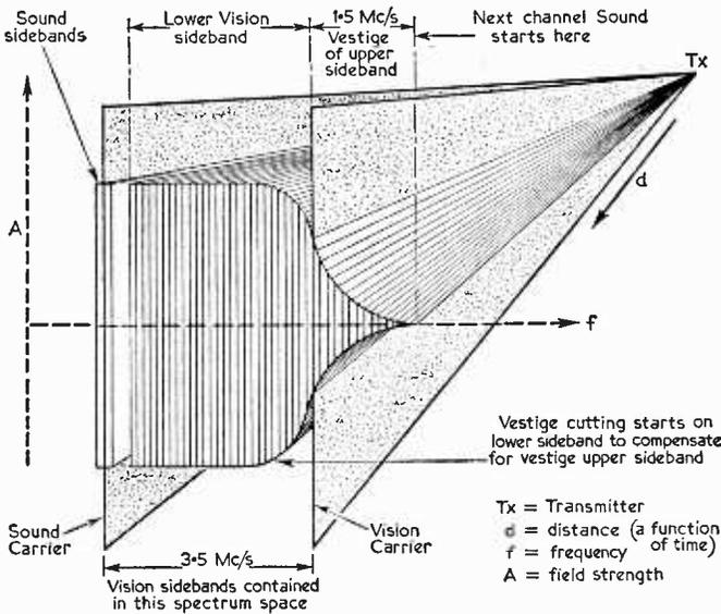
Fig. 3.—A "picture" of a television channel with equal vision/sound power ratio.
