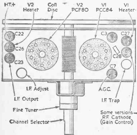
Fig. 1.—The top view of the original Fireball tuner. The shaded components are lead-through decoupling capacitors.
