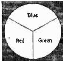
Fig. 8 (right).—A primary colour separation filter for use with a single lens—it consists of three equal sectors mounted in a frame.
