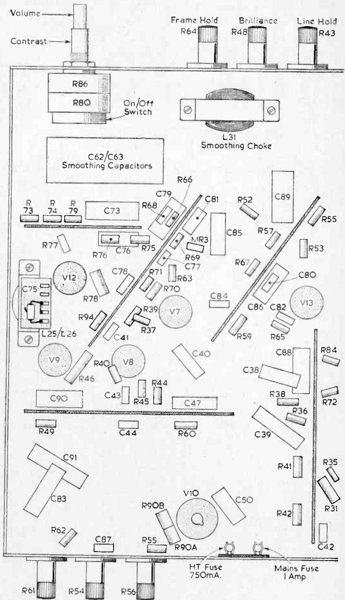
Fig. 6.—The underchassis view of the receiver.
