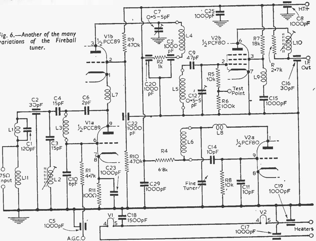
V2 are ever accidentally transposed and subsequent reception is nil or poor after the mistake has been rectified, check R5 (pins 7 and 8 of V1 to chassis) and R8 (H.T. feed to V1).
