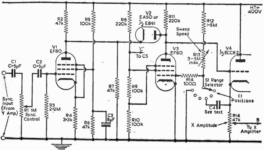
Fig. 9.—The circuit of the Timebase generator.
