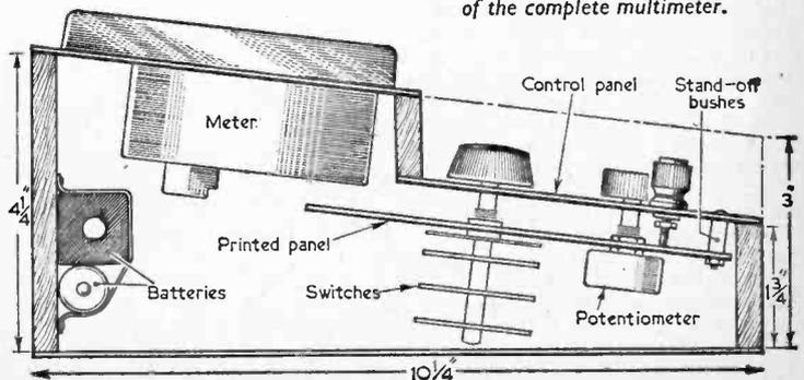
and printed circuit board, can best be obtained new, or as off-cuts, from a "do-it-yourself" shop. They are both  $\frac{1}{8}$  in. thick and  $6\frac{7}{8}$  in. wide, but the control panel is  $5\frac{1}{4}$  in. in length and the meter panel  $5\frac{1}{2}$  in. in length.
