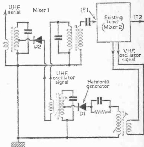
Fig. 1.—The components of this UHF segment are mounted on a biscuit moulding. The oscillator signal is increased in frequency by D1, and this is mixed with the UHF signal in D2 to give I.F.1.
