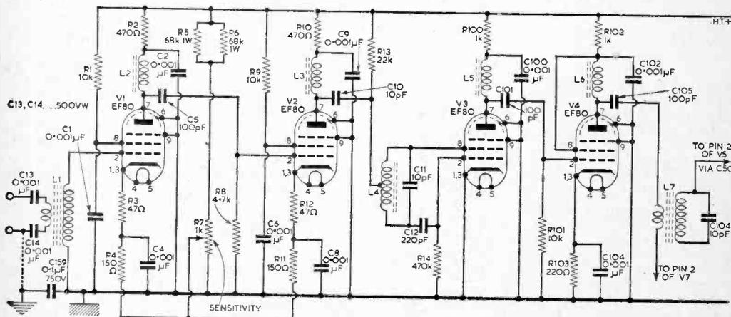
Fig. 1.—The circuit of the R.F. frequency-changer and vision I.F. stages.
