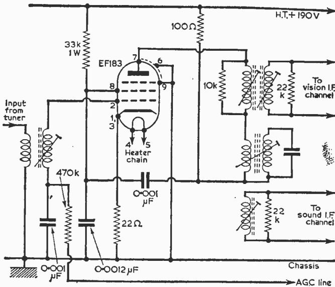
Fig. 2.—The circuit of Fig. 1 rearranged for use with an EF183 frame grid variable- $\mu$  pentode. This circuit gives an effective gm of about 12mA/V.
