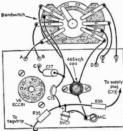
Fig. 13 (above)—R.F. oscillator coil switching.
