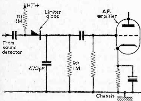
Fig. 8.—A germanium diode used in a sound noise limiter circuit.
