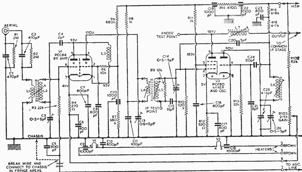
Fig. 1.—The circuit diagram of a typical turret tuner. The components making up this tuner are described in detail in the text.
