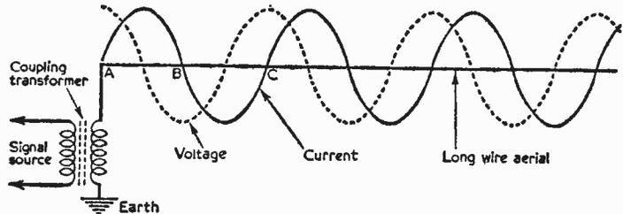
Fig. 1.—The current and voltage distribution in a long-wire aerial.
