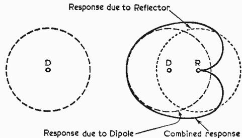
Fig. 4(a).—The polar response of a simple dipole, and (b), the directional response produced by adding a reflector. Further directivity and gain is produced by adding directors.
