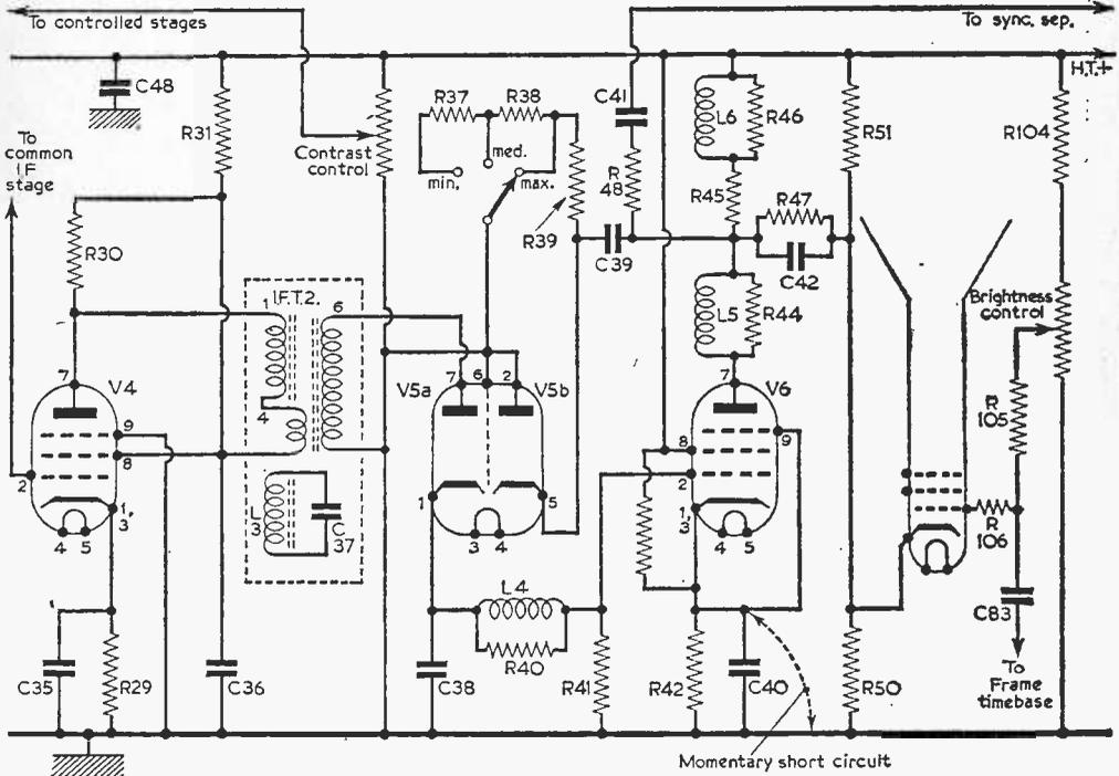
Fig. 5.—The vision I.F., detector, vision amplifier, and picture tube biasing circuit.
