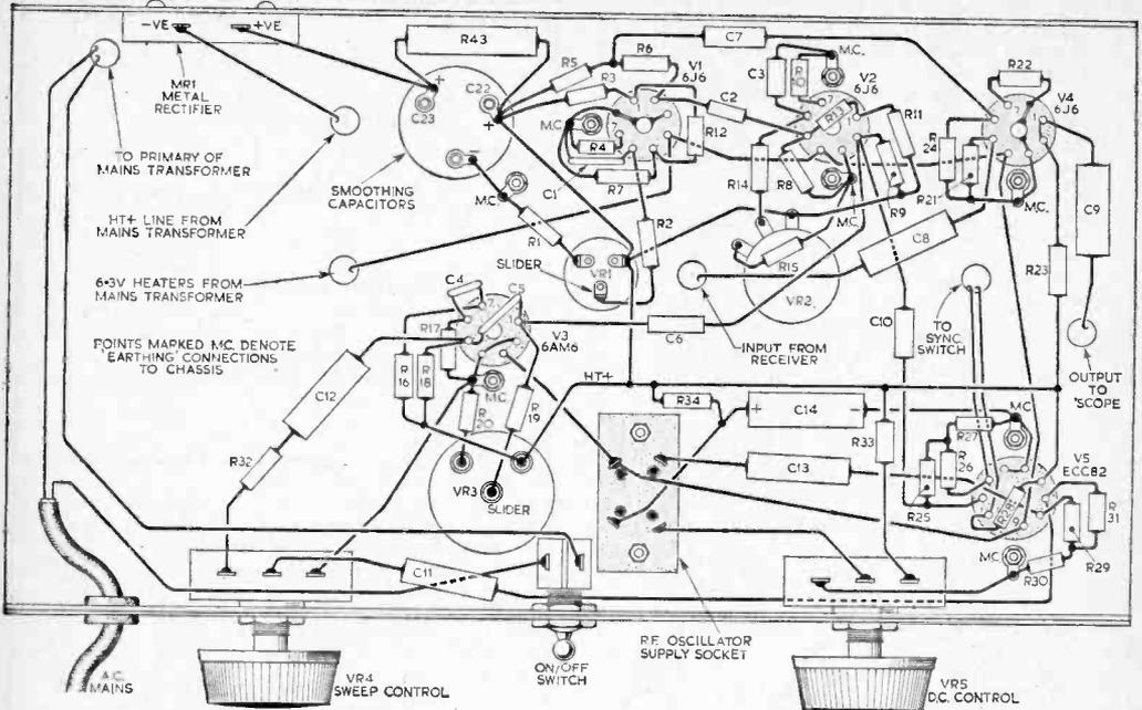
Fig. 11.—The underchassis wiring diagram.
