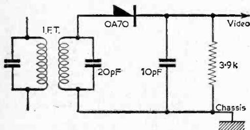
Fig. 7—A vision detector circuit, using a medium impedance diode.
