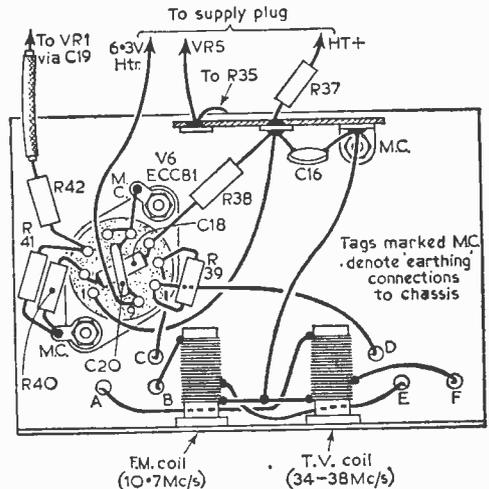
Fig. 10.—The wiring details of the oscillator circuit.
