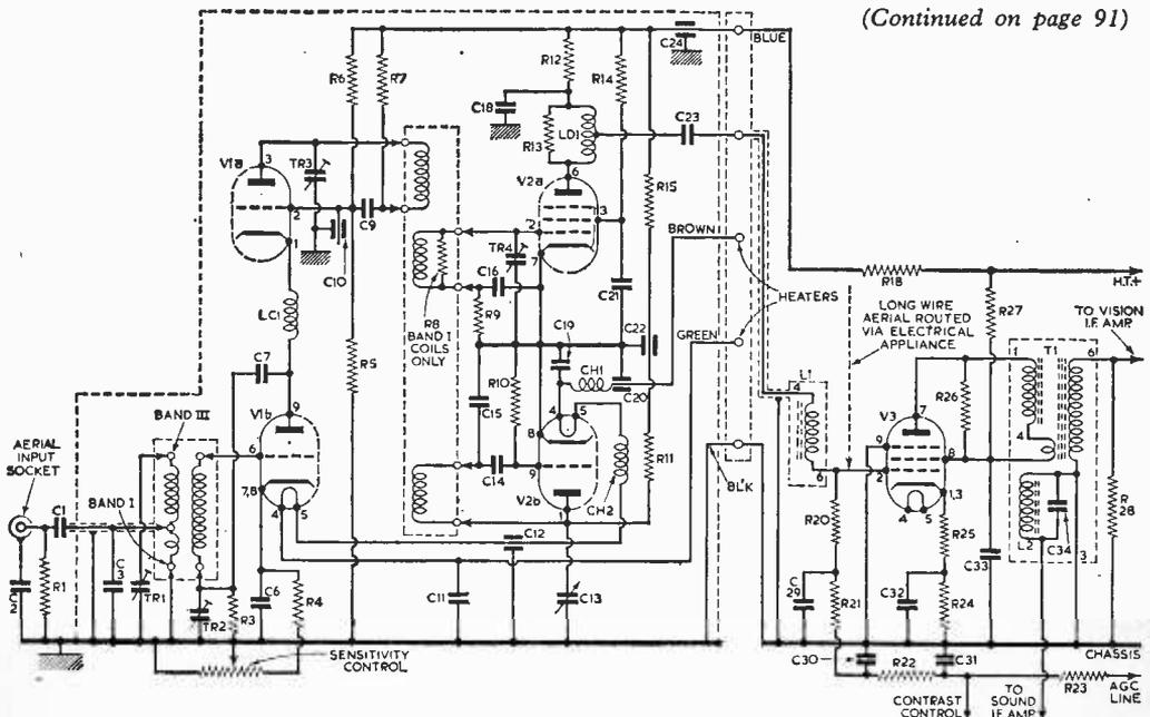
Fig. 4.—The tuner and common I.F. stages (stages 3 and 4 in Fig. 1 on page 616 of the September issue).
