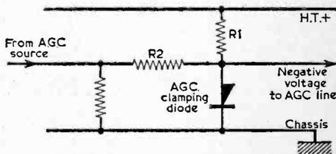
Fig. 9.—A diode clamping circuit which may also be used to provide AGC delay to one or more controlled stages.
