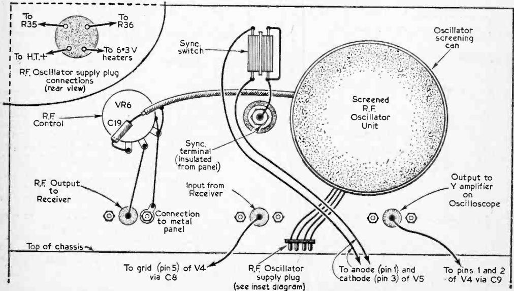
Fig. 12.—The connections to the rear of the front panel (inset: the plug connections for the R.F. oscillator).
