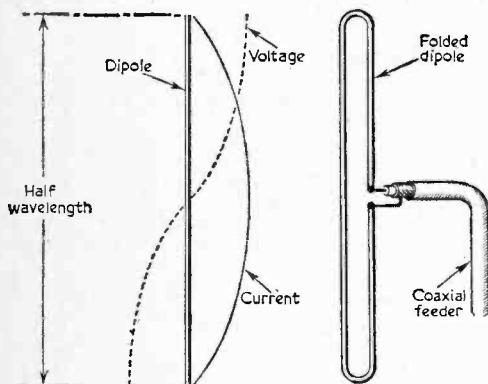
Fig. 3 (left).—The current and voltage distribution in a tuned half-wave aerial.
