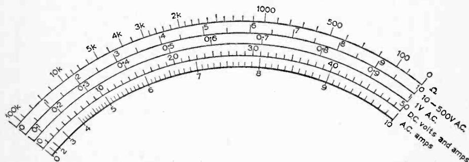
Fig. 4.—An example of the type of scale produced in calibrating the multimeter—in fact, this scale may be used on the completed instrument.
