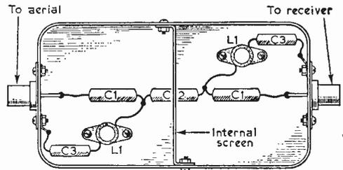
Fig. 17—A suggested construction for the filter of Fig. 15.
