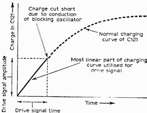
Fig. 5—The charge in C121 (Fig. 4) is cut short within the linear part of the charging curve by conduction of the line blocking oscillator.
