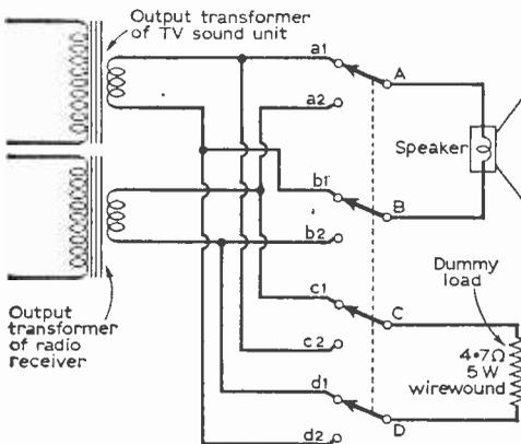
Fig. 3 (above)—The circuit switching to provide change-over of loudspeaker from the TV unit to radio output and dummy loading of the channel not in use.
