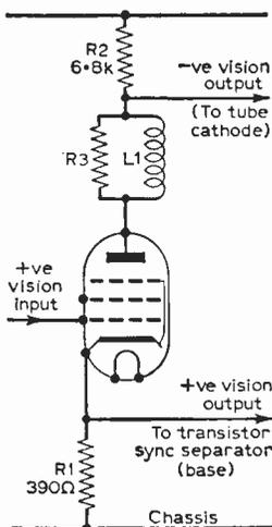
signal input conditions, the line pulses being positive-going and the frame pulses negative-going. Coupling to the appropriate generators should be by way of a capacitor—about 47pF for line and 680pF for frame are suitable. With multivibrator types of generator, the sync pulses are best injected into the cathode circuit rather than the grid.
