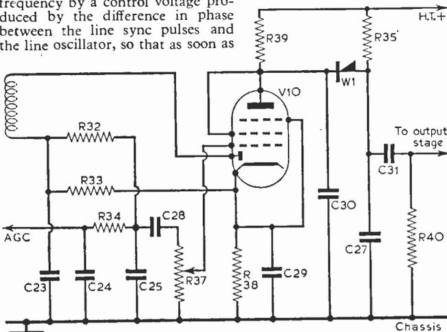
Fig. 5—A circuit for improving the sound interference suppression in Ferguson Models 941T and 951T.
