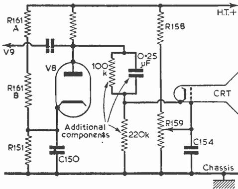
Fig. 7—Reducing the D.C. component of the vision signal in English Electric T40 series. This modification reduces random changes in brightness.
