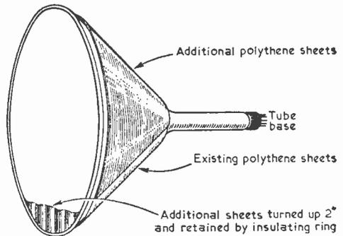
Fig. 8—Eliminating corona on 21in. English Electric models C45 and C46.
