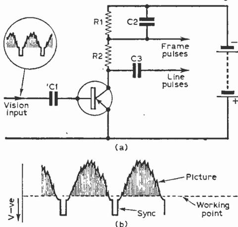
Fig. 1—The basic transistor sync separator circuit.
