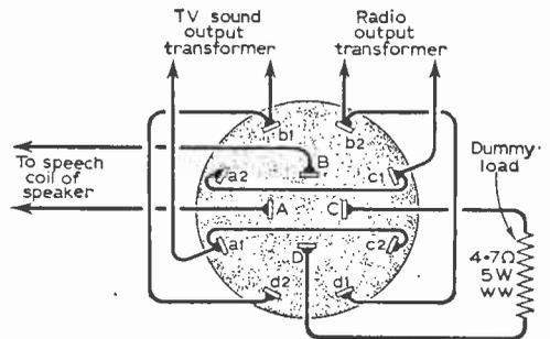
Short and direct wiring is of course essential, and the principle of "single point earthing" of screen and cathode decoupling and biasing components, as shown in the circuit diagram, is very important. Soldering tags are mounted on the valvoholder fixing bolts as shown in Fig. 5, to facilitate this, and the wiring of the H.T. supply is made easy by the use of a tagstrip.
