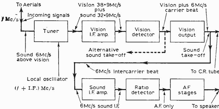
since upon it is superimposed the original frequency-modulation of the sound signal. In some sets it is passed along with the video signal through the video output stage and is extracted at the output and then applied to a separate 6Mc/s sound I.F. amplifier, as shown in the diagram.
