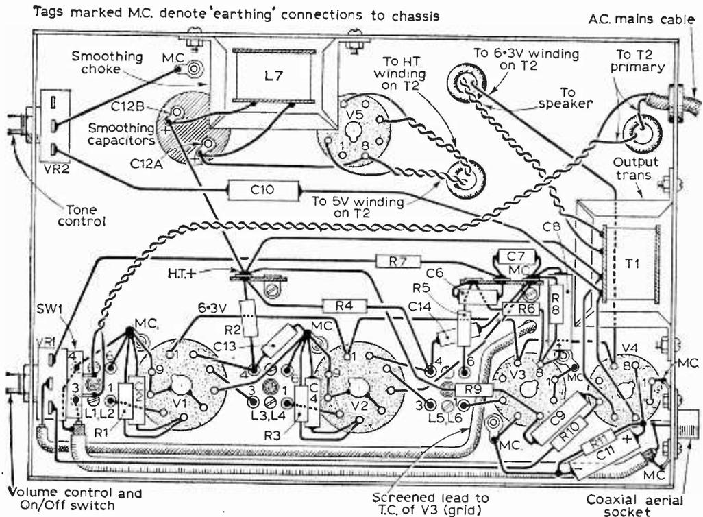
Fig. 5—The underchassis wiring.
