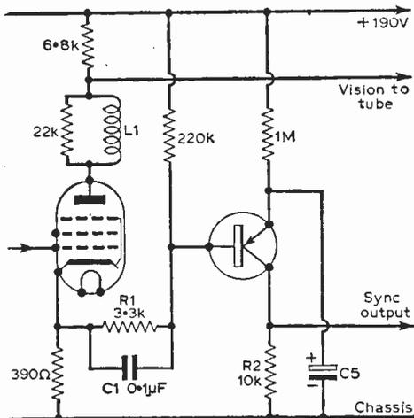
Fig. 4—The transistor sync separator as used in recent commercial receivers.
