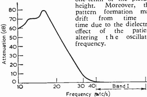
Fig. 16—The frequency/attenuation characteristics of the high-pass filter of Fig. 15.
