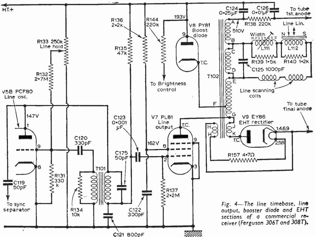
Fig. 4—The line timebase, line output, booster diode and EHT sections of a commercial receiver (Ferguson 306T and 308T).
