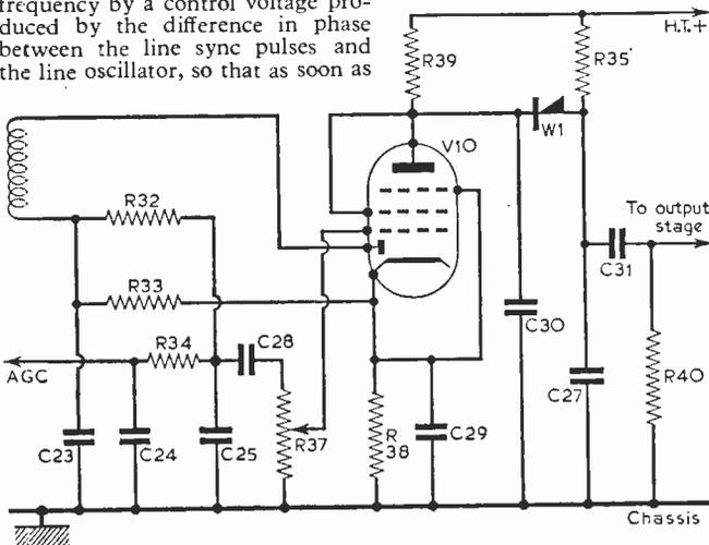
Fig. 5—A circuit for improving the sound interference suppression in Ferguson Models 941T and 951T.
