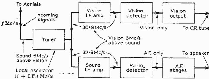
Fig. 2 (above)—The system of Fig. 1 altered to suit the CCIR standards.
