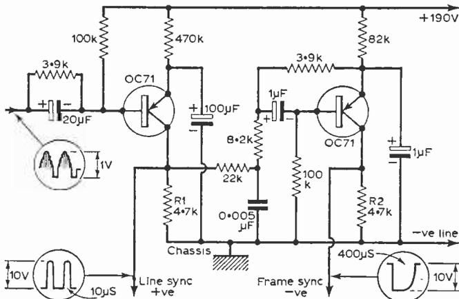
Fig. 2 (above)—The Mullard circuit using two transistors.
