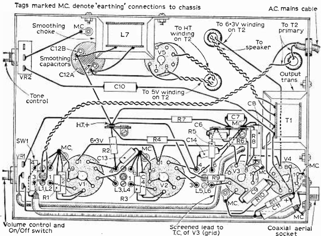
Fig. 5—The underchassis wiring.
