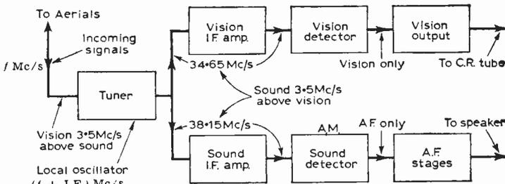
Fig. 1—A block diagram showing the standards adopted in the existing 405-line television system.
