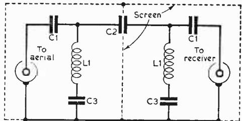
Fig. 15—The circuit of a practical high-pass two-stage filter. This is designed for 75Ω coaxial cable and to provide the characteristics of Fig. 16, the components should have the following values: C1, 68pF; C2, 33pF; C3, 500pF; L1, 0.24μH (produced by 7 turns of 16s.w.g. tinned copper wire on 2in. former).
