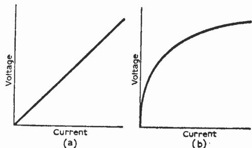
Fig. 2—The resistance of a normal resistor remains constant with variations in the voltage present across it; thus, the voltage/current characteristic is linear as shown in (a). With a voltage-dependent resistor, however, the resistance is not constant, but falls as the voltage across it increases. This gives a non-linear voltage/current characteristic shown in (b).
