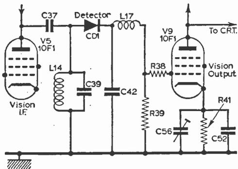
Fig. 28—Intermittent vision in the Ekco T217 series is often caused by a dry-soldered joint developing in L17, the vision coupling inductor. Check by probing with an insulated tool, and resolder if necessary.
