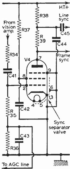
Fig. 31—Improved vision channel gain and better control of contrast is sometimes possible by shunting R36 with a resistor of about 15k.
