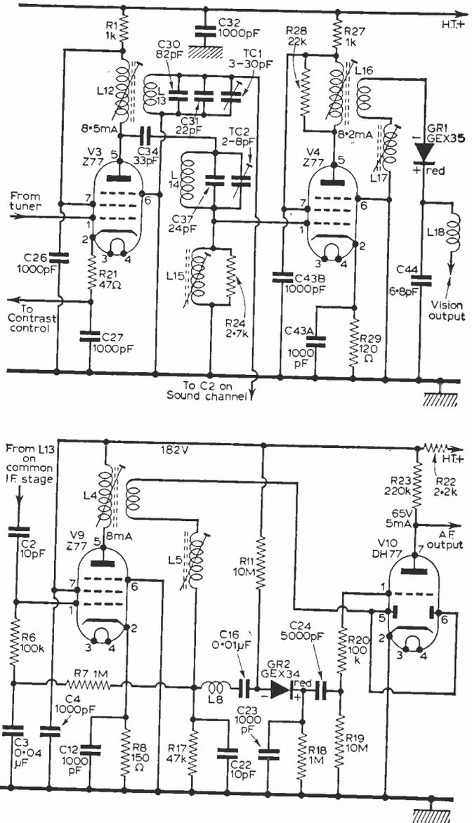
Fig. 3—This circuit shows how the sound and vision I.F. signals are separated after the common I.F. amplifier state V3. Here, V4 is the vision I.F. amplifier valve fed via C34 and V9 is the sound I.F. amplifier valve fed via L13 and C2.
