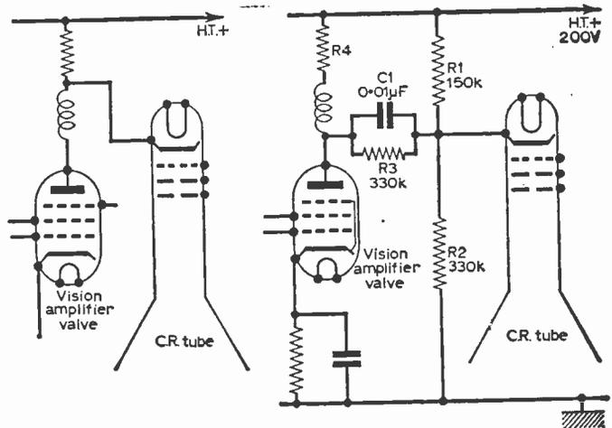
Fig. 6 (left)—Direct coupling was used on most early sets from the anode of the video amplifier valve to the cathode of the picture tube, but this was found to aggravate aircraft flutter and similar effects.
