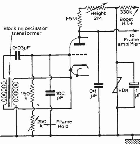
Fig. 4—In this circuit, a VDR is used to stabilise a frame blocking oscillator.
