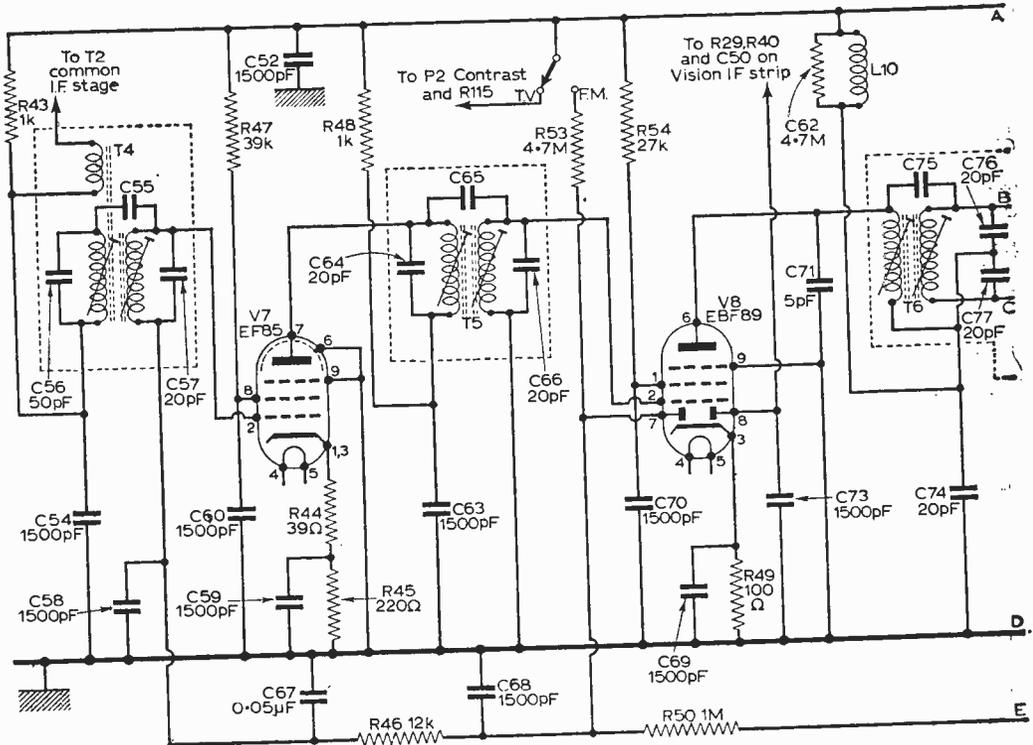
Fig. 8a—The circuit of the sound I.F. stages.
