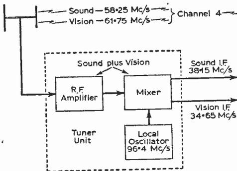
Fig. 1—A block diagram of the first two stages in a television receiver common to both sound and vision. The standard I.F.'s (e.g., sound at 38.15Mc/s and vision at 34.65Mc/s) are produced by the local oscillator operating above the signal frequencies, causing the sound I.F. to be higher than the vision I.F.
