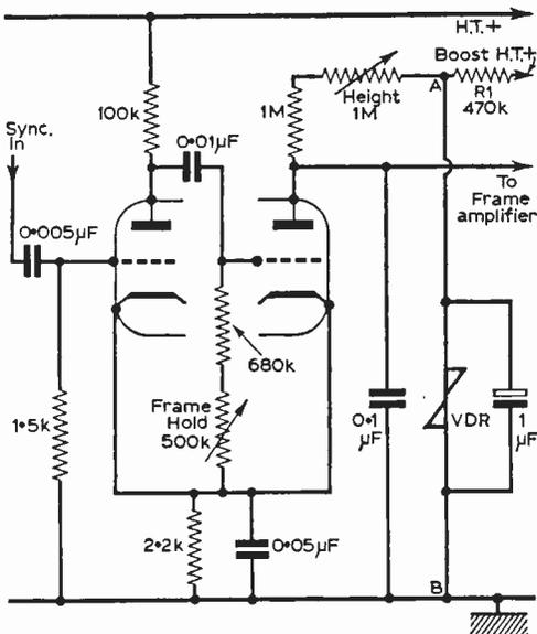
Fig. 3—A circuit showing how a multivibrator frame generator can be stabilised with a voltage-dependent resistor.
