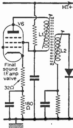
Fig. 29—Sound channel instability often results in the early versions of the Masteradio TE4T and TE7T models. This can be caused either by defective decoupling in the sound I.F. stages or excessive gain in the final stage shown. The trouble can be countered either by de-tuning L2 slightly, or by including a 32  $\Omega$  resistor in the cathode circuit, as shown. A too peaky sound channel response impairs the operation of the sound interference limiter.
