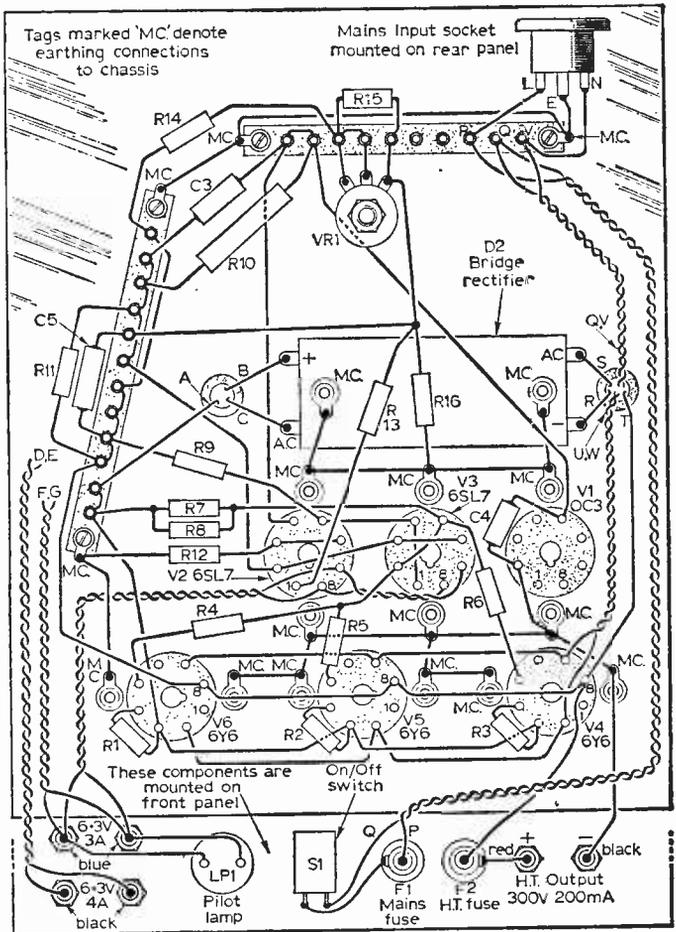
Fig. 4—The underchassis wiring diagram.
