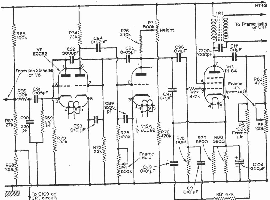
Fig. 5—Circuit of the sync separator and frame timebase stages.
