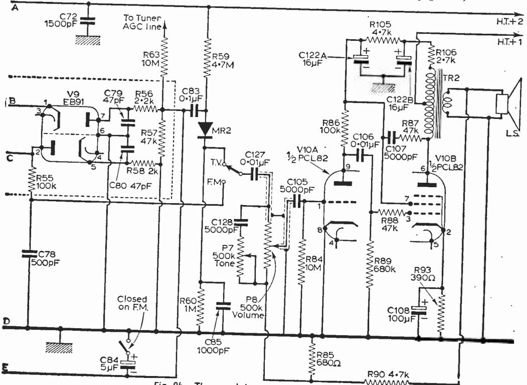
Fig. 8b—The sound detector and output stages.
