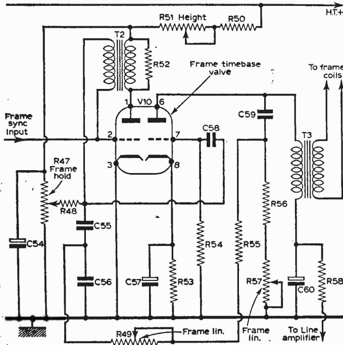
Fig. 30—Extra height can be obtained in the Masteradio series by (a) including R52— $47k$  and (b) increasing C56 from  $0.03\mu F$  to  $0.04\mu F$  by adding an extra  $0.01\mu F$  in parallel.
