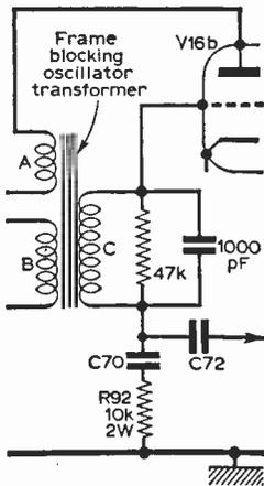
Fig. 32—For frame collapse in the Philips 1446 and 1746 series, check R92 for open-circuit. For frame judder, check the 47k resistor for open-circuit or value increase.
