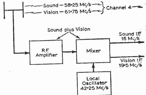
Fig. 2—In early TV sets, the sound I.F. was often lower than the vision I.F., since the local oscillator was arranged to operate below the incoming frequencies, as this diagram shows. An example using such a combination is the Ultra 72 series of receivers.
