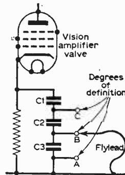
Fig. 10—A plug and socket arrangement is sometimes used instead of the pre-set capacitor shown in Fig. 9.
