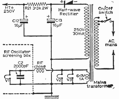
Fig. 4—The circuit of a suitable power-pack for the meter.
