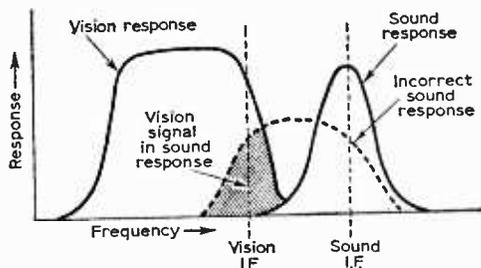
Fig. 4—This diagram shows that when the sound I.F. stages are aligned correctly, the sound response curve is well out of range of the vision signals, but due to misalignment (as shown by the broken-line curve), the sound response will almost certainly embrace the vision response and cause vision-on-sound.
