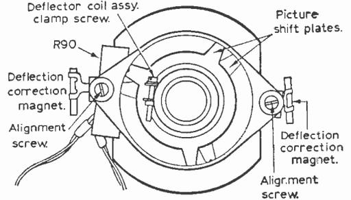
Fig. 8(c)—Picture adjustments provided on some Bush receivers.
