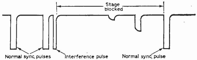
Now on a negatively-modulated signal interference pulses "look" to the valve like extra large sync pulses and thus cause the grid capacitor to charge to a higher than normal value. This means that the valve is held at cut-off for a longer than normal period, depending upon the time-constant of the grid capacitor and resistor combination, so that subsequent to a burst of impulsive interference the valve is "blocked" until the extra charge of the capacitor is exhausted.
