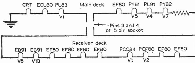
Fig. 1a (left)—The heater system of the TV24C before conversion in a series chain. Valves requiring replacement are given their original circuit reference. The rectifier V7 (PY82) is removed.
