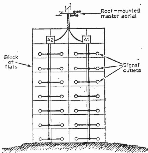
**Fig. 35—Flat system.** Here the master aerials are mounted on the roof and the signals are divided between two amplifiers A1 and A2. Each amplifier feeds its own main cable which is tapped for signal at each dwelling. In some systems a single amplifier system is used and the two main cables are then fed through a circuit splitter (see Fig. 36).
