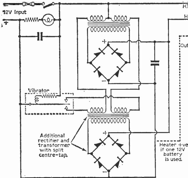
Fig. 3—The modification of a Type No. 9 vibratory power unit by the addition of an extra transformer and rectifier.
