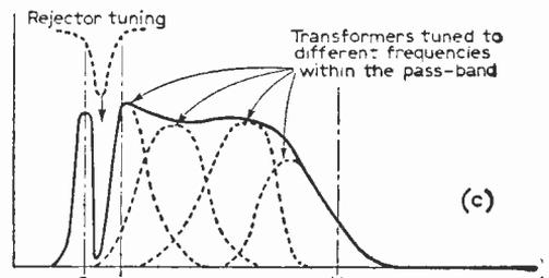
Fig. 1—Vision receiver i.f. response characteristics, as discussed in the text.
