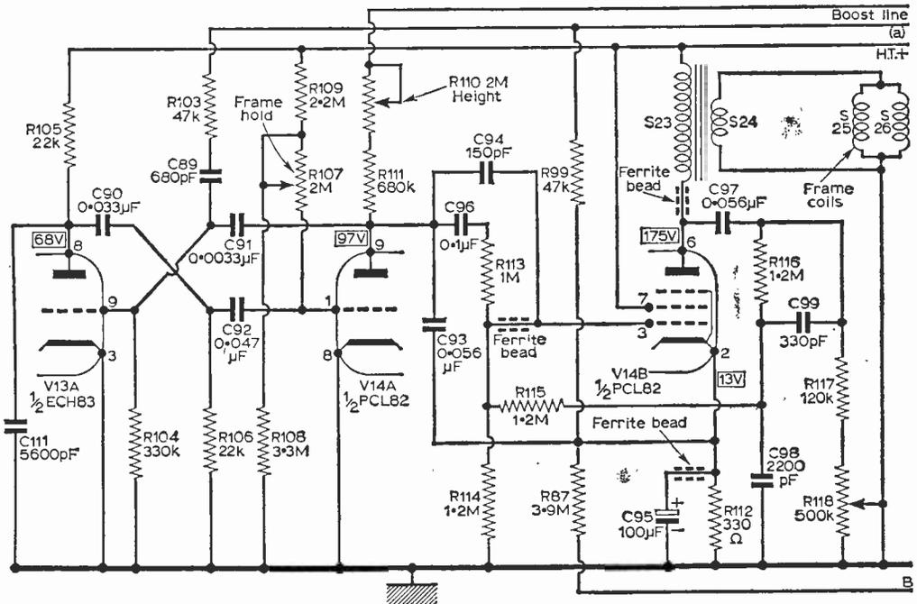
Fig. 7—The frame timebase stage.
