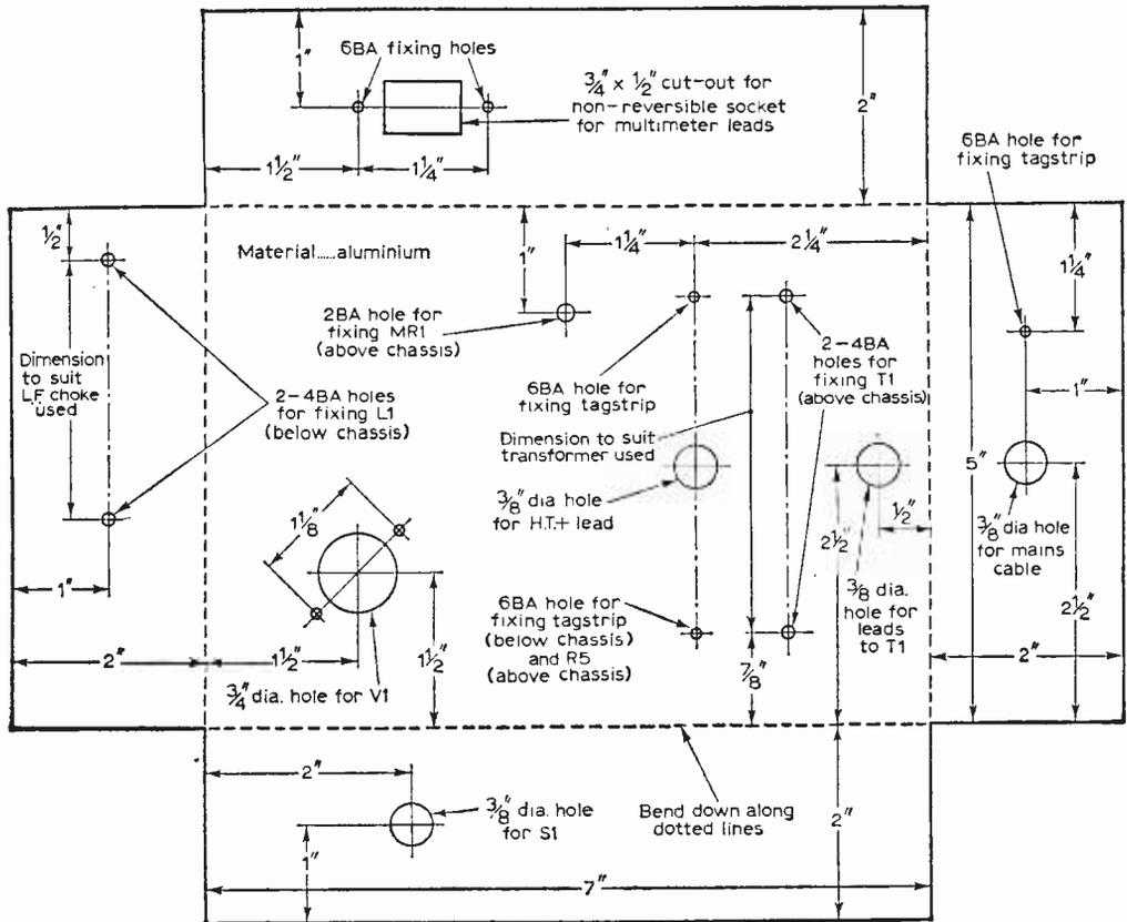
Fig. 2—The chassis drilling.
