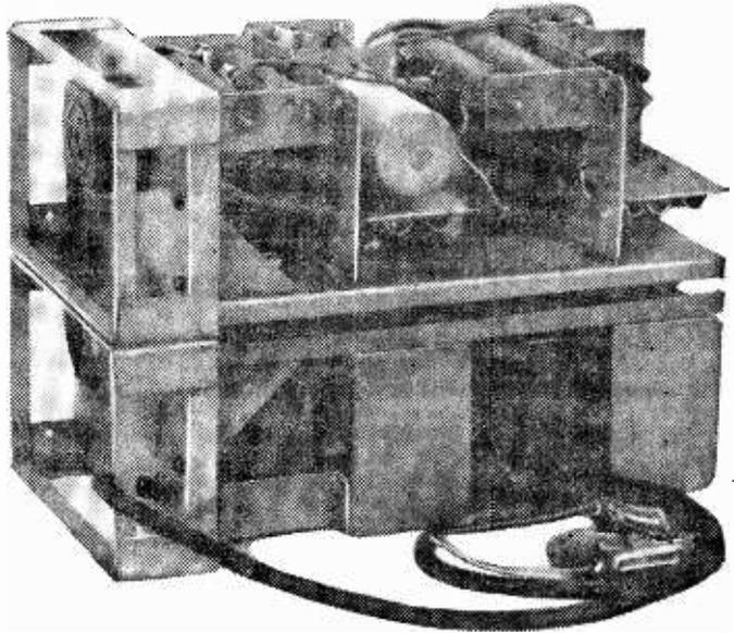
**T**O those who have not access to a mains electricity supply, a battery operated television receiver has certain attractions. The successful conversion of a mains receiver to run from 12V batteries presents an interesting problem, which the writer attempted, working on Bush TV22 and TV24C receivers. The following notes apply specifically to these two sets, but the general principles could be applied to most receivers.
