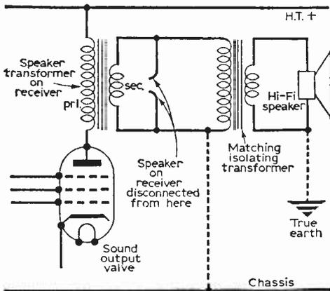
Fig. 1—Showing how a transformer is used between the set's speaker transformer and the extension speaker for matching and isolation (see text).
