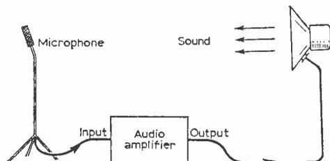
Fig. 1—Showing basic microphony. A feedback path is established partly acoustically from microphone to loudspeaker and partly electrically from the input to the output of the amplifier.
