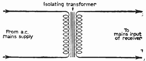
Fig. 2—The use of a mains isolating transformer. This method is necessary for the feed of Fig. 4 when the set is a.c./d.c. See text. The transformer should withstand the power loading of the set.
