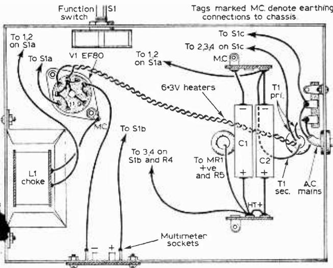
Fig. 5—The underchassis wiring diagram and component layout.
