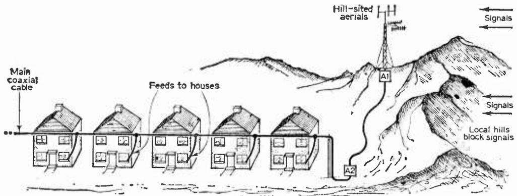
Fig. 34—Small shared aerial system. Signals picked up by the hill-sited aerials are fed into the shielded area through coaxial cable after first being amplified at the aerial by A1 and by A2 at the start of distribution. Feeds to houses are taken through resistive taps as described last month.
