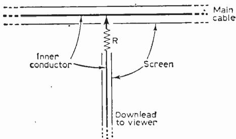
Fig. 37—Simple resistive tap for signal take-off from coaxial spur or main cable. The value of R determines the amount of signal taken from the line and the amount of loss introduced to it. Practical values range from about 180Ω to 2700Ω.
