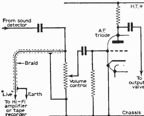
Fig. 3—A method for extracting good quality sound from across the volume control to drive a hi-fi amplifier or for recording. Mains isolation must be used if set of the a.c./d.c. type.
