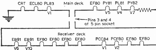
Fig. 1a (left)—The heater system of the TV24C before conversion in a series chain. Valves requiring replacement are given their original circuit reference. The rectifier V7 (PY82) is removed.
