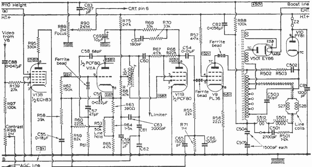
Fig. 6—The line timebase circuit.
