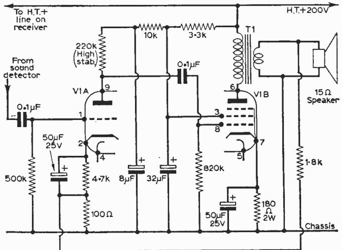
Fig. 4—Experimental audio stage for giving improved sound in conjunction with a good quality extension speaker system. V1 Mullard PCL86; T1 primary impedance 7kΩ, primary inductance 10H, primary resistance 350Ω. All resistors 1/4W and capacitors 300V working unless otherwise stated. Extension loudspeaker isolation must be adopted as described in the text.
