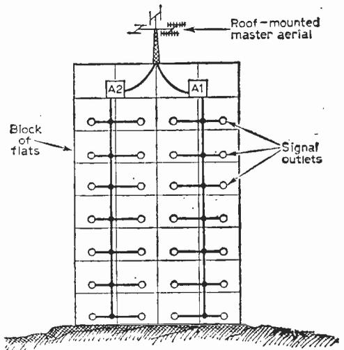
**Fig. 35—Flat system.** Here the master aerials are mounted on the roof and the signals are divided between two amplifiers A1 and A2. Each amplifier feeds its own main cable which is tapped for signal at each dwelling. In some systems a single amplifier system is used and the two main cables are then fed through a circuit splitter (see Fig. 36).
