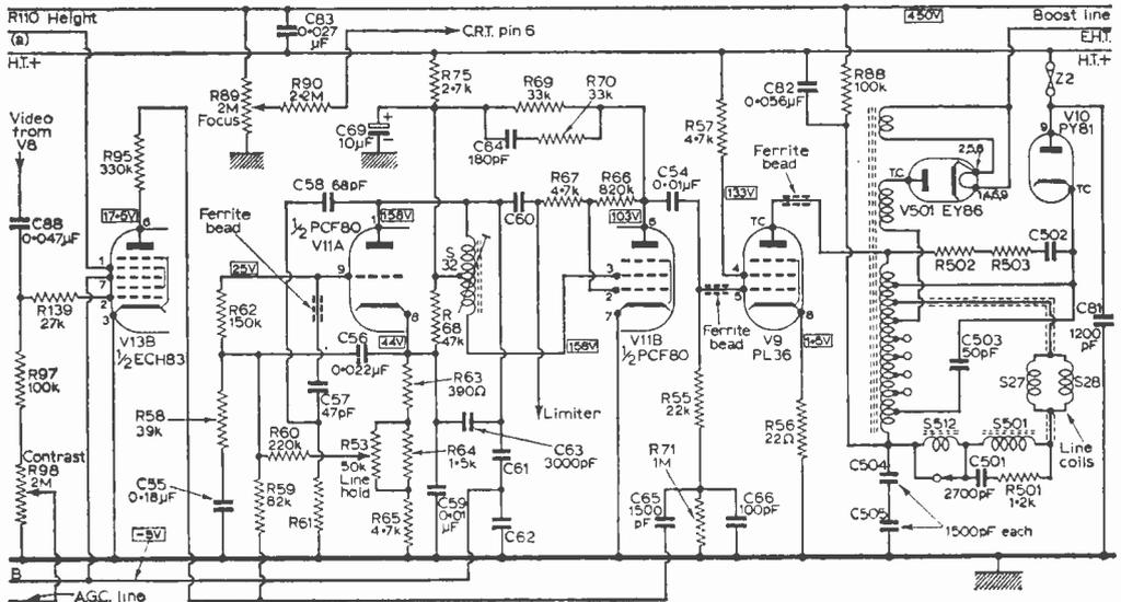
Fig. 6—The line timebase circuit.
