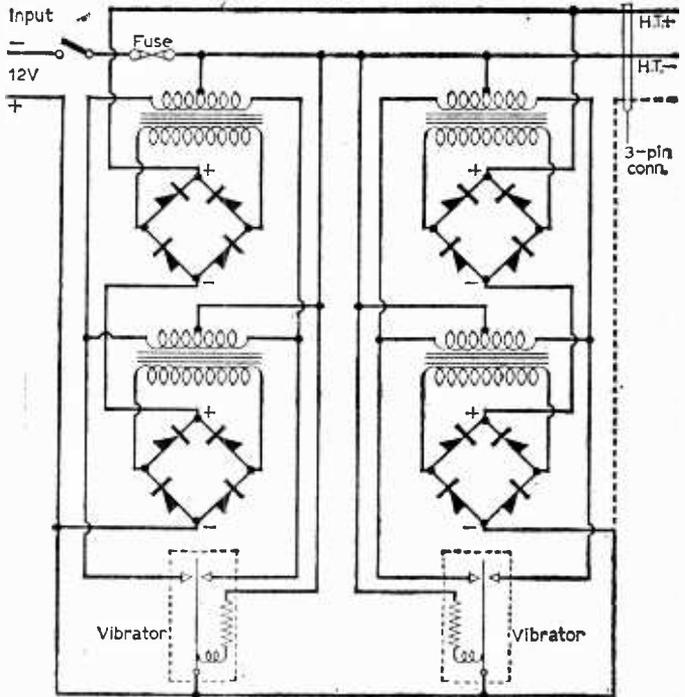
Fig. 2—12V vibratory power unit—part of ZA21531, Power Supply and Amplifier Unit No. 1. The chokes and capacitors are not shown. A photograph of the converted unit is shown in the heading.
