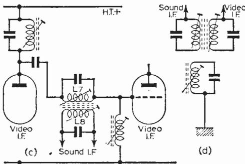
Figs. 2c and d—Absorption sound take-off circuits.
