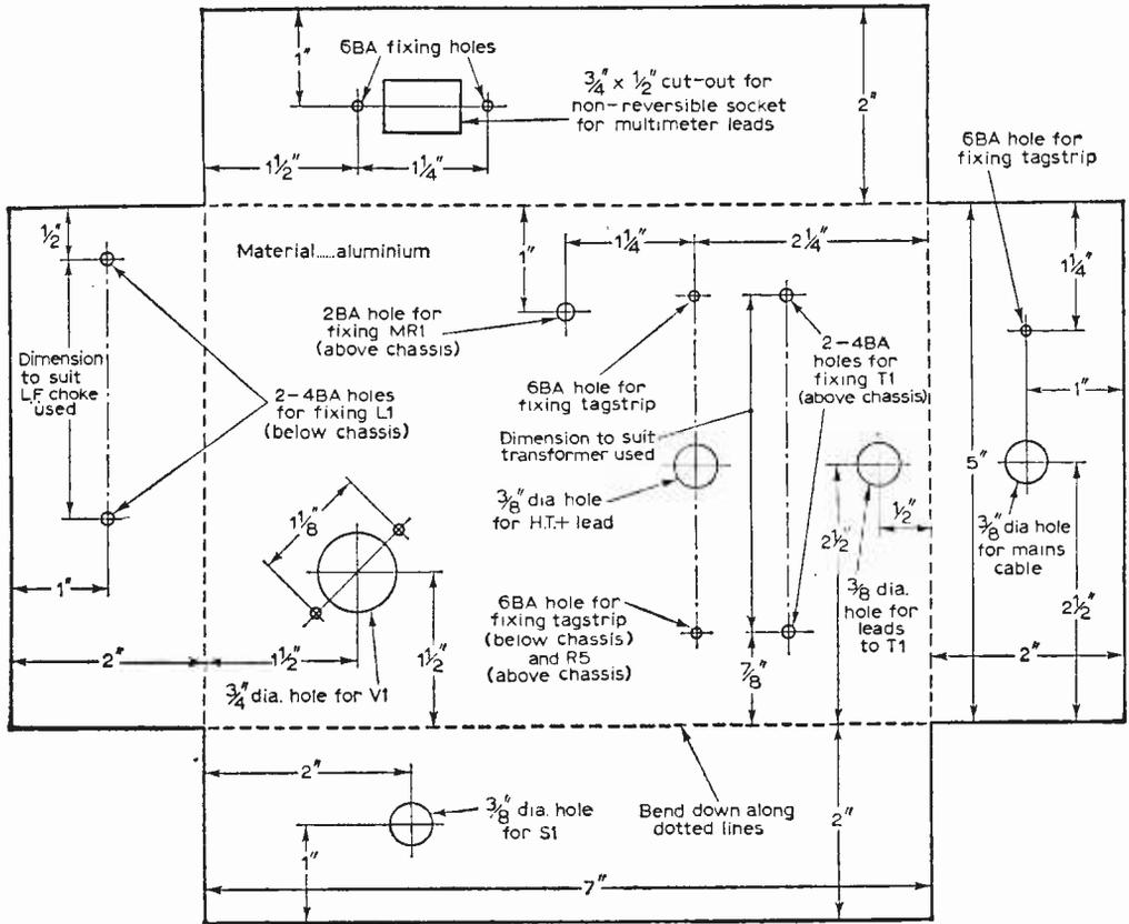
Fig. 2—The chassis drilling.
