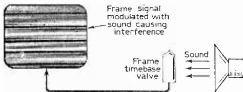
Fig. 2—Showing how the sound-on-vision interference symptom is produced by a microphonic frame timebase valve.
