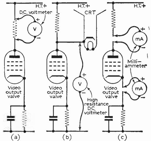
Fig. 3—Alternative methods of obtaining video output indications.
