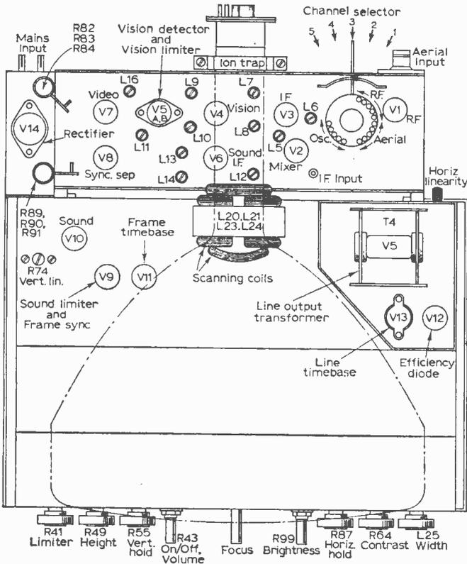
Fig. 2—An example of stage and valve layout (Ferranti 1473 series).
