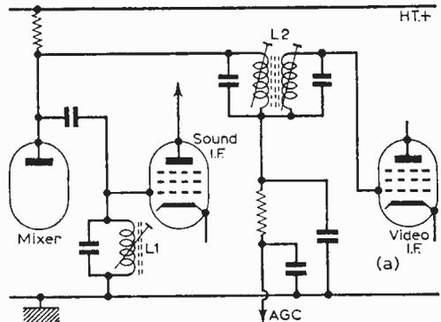
Fig. 2a (above)—Capacitive sound take-off circuit.
