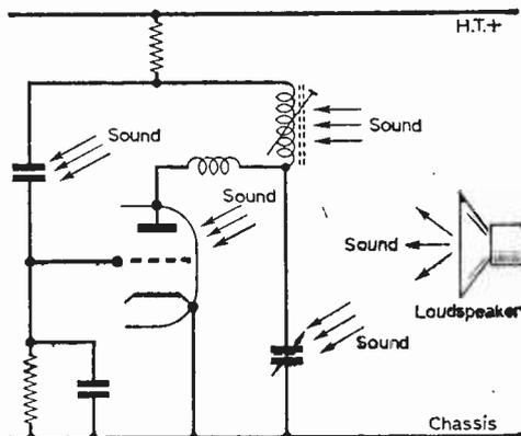
Fig. 4—Microphony symptoms can arise from the exciting vibrations modulating the local oscillator in the tuner. This occurs mainly from the sound causing a change in one of the components used for frequency control of the oscillator in the tuner, as this diagram shows.
