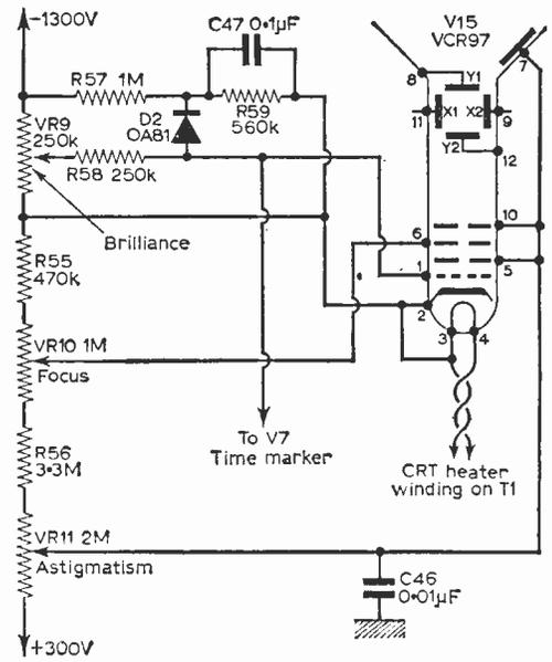
Fig. 6—C.R.T. power supply network.
