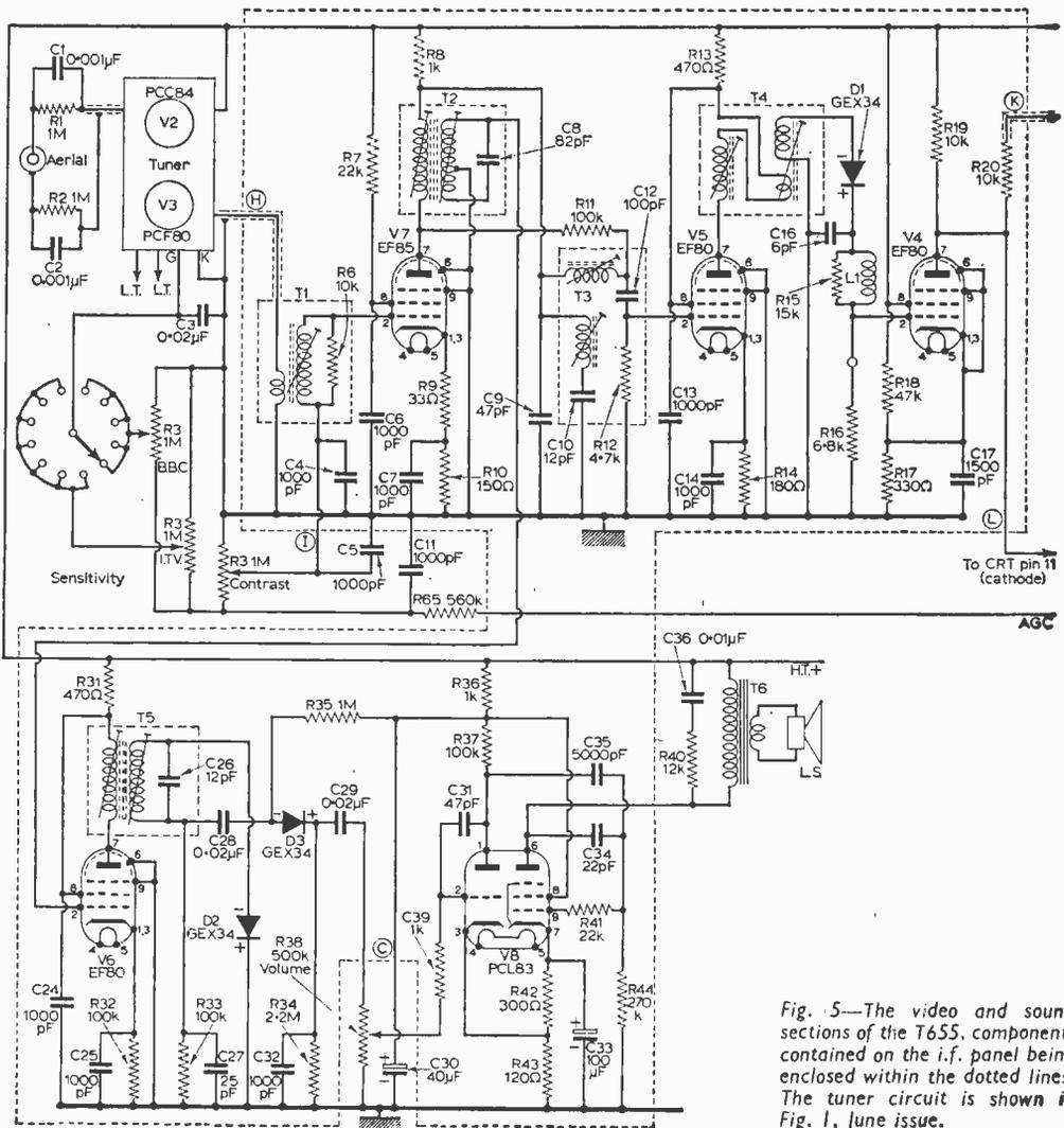
Fig. 5.—The video and sound sections of the T655, components contained on the i.f. panel being enclosed within the dotted lines. The tuner circuit is shown in Fig. 1, June issue.
