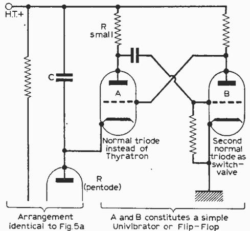
heavily, so that its anode is well below h.t., and so is, therefore, the grid of triode A. This represents heavy cut-off bias on triode A even when C has slightly charged and the cathode of triode A falls progressively below h.t. However, there will ultimately come a point where C has charged so far that the cathode of triode A has fallen below h.t. to an extent to enable anode current to start, i.e. the difference between triode A cathode and triode B anode has become less than the grid-base.
