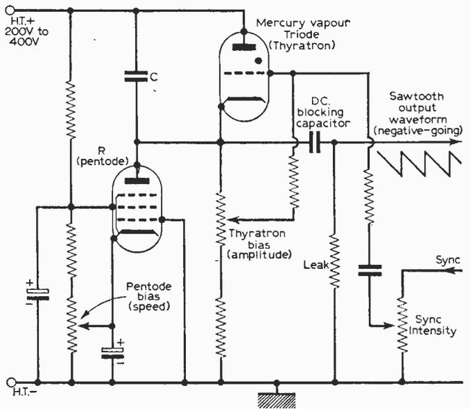
Fig. 5(a) (above)—A practical form of a pentode-controlled thyatron timebase.
