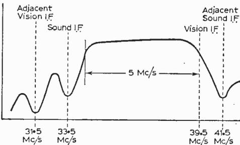
Fig. 3—The overall i.f. response of a 625-line receiver suitable for British standards—i.e. sound/vision carrier spacing 6Mc/s.
