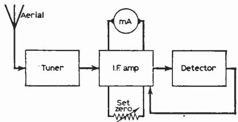
Fig. 1—Block diagram of commercial signal strength meter. The operation of the instrument is explained in the text.
