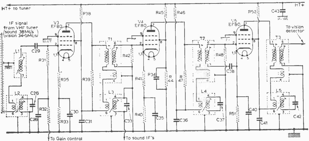
Fig. 1.—The i.f. stages of a typical 405-line receiver of the type which is considered for 625-line conversion in this article.
