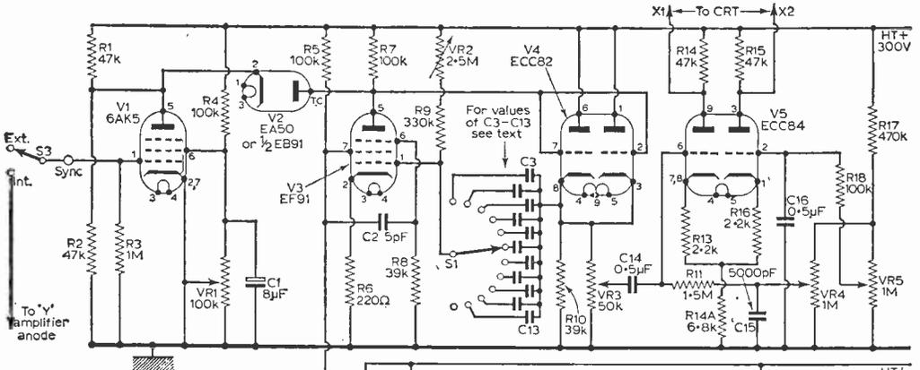
Fig. 2—Timebase generator and amplifier; sync amplifier and time marker.
