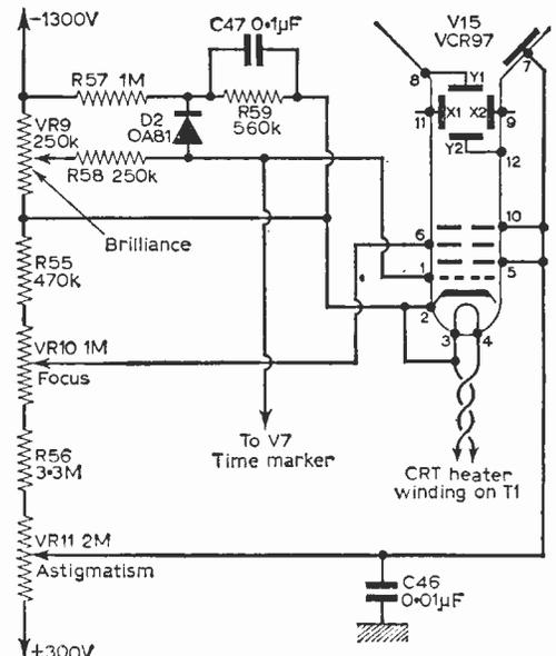
Fig. 6—C.R.T. power supply network.
