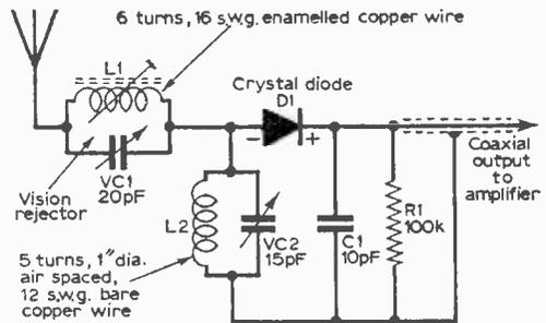
Fig. 1—The circuit and coil winding details.
