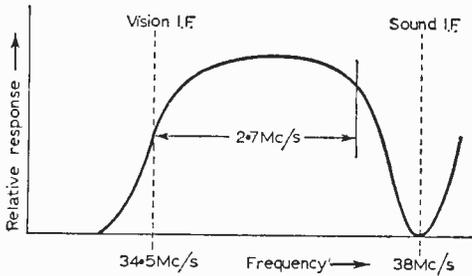
Fig. 2—The vision i.f. response of the circuit in Fig. 1.
