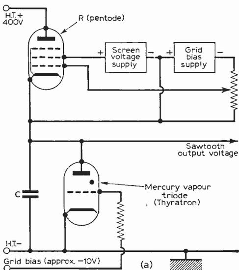
Fig. 4(a) (left)—Use of a pentode valve in place of a charging resistance to improve linearity.
