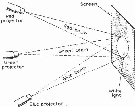
Fig. 1—If lights of the three primary colours are projected on to a common screen, white light is produced. Note that colours are mixed additively in this way, as distinct from colour filters interposed between a white light and the eye, when a colour is subtracted from white light.
