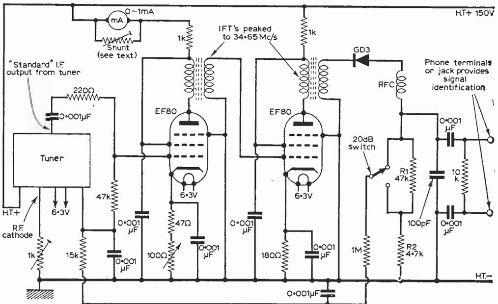
Fig. 3—Circuit diagram of signal strength meter for comparative tests. The milliammeter may be calibrated direct in millivolts and microvolts or a graph may be produced giving signal volts against meter reading. For u.h.f. signals in Bands IV and V, the tuner would tune over the u.h.f. channels and the a.g.c. control would be removed from that section.
