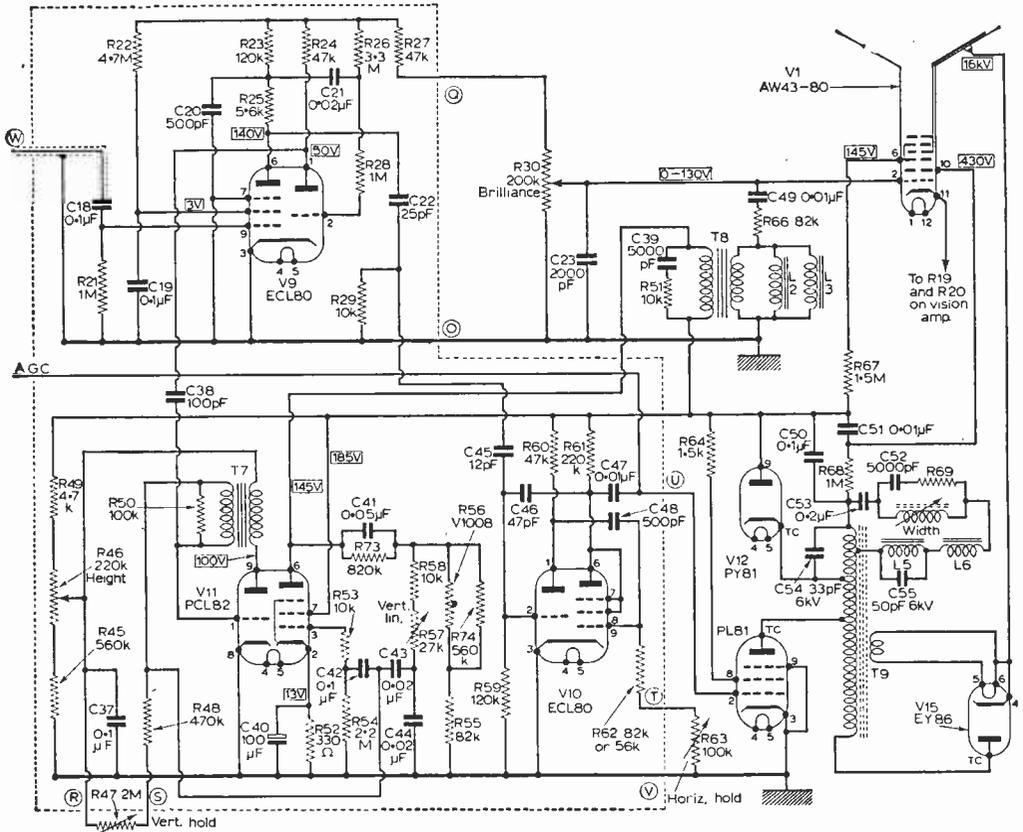
Fig. 6—The sync separator and timebase circuitry, components contained within the dotted lines being contained on the timebase panel.
