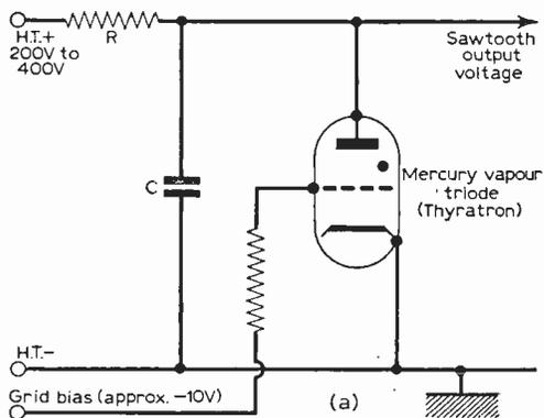
Fig. 3(a) (above)—The basic Thyatron timebase, with the output waveform shown in (b) (below).
