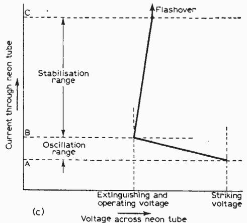
Fig. 2(a)—The simple flashing neon timebase. (b)—The output waveform of the neon-timebase. (c)—The anode characteristics (idealised) of a typical neon tube.
