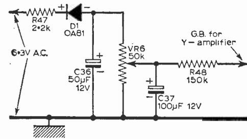
Fig. 4 (above)—Grid bias supplies for the Y amplifier.
