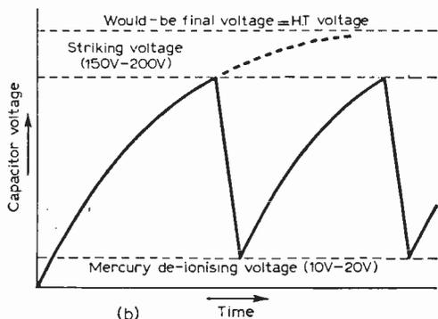
their product. C cannot be less than the circuit and tube stray capacities, and we have seen that R cannot be less than a value raising current above point B in Fig. 2(c). Thus there is a definite upper limit above which frequency the circuit will not oscillate. This, taking also the delaying-effects of the ionising and de-ionising of the neon gas into account, usually lies at around 10kc/s, and is far too low for modern high-speed oscilloscopes for pulse-observations.
