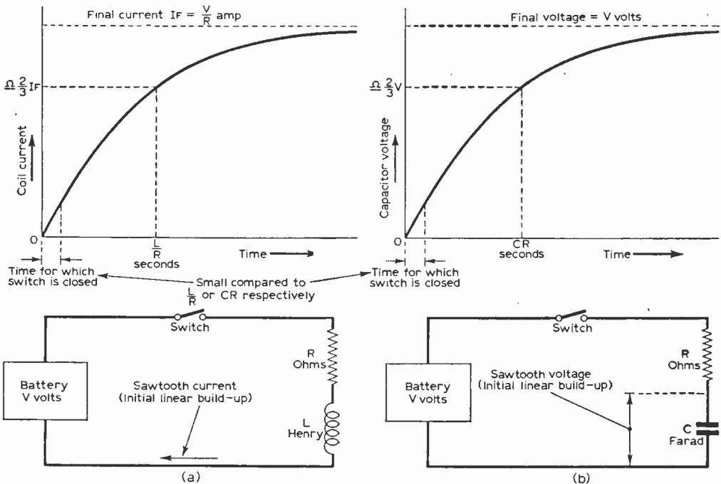
Fig. 1(a)—Showing the exponential build-up of current in an inductance: (b)—showing the exponential build-up of voltage on a charging capacitor. These arrangements form the basis of all timebase circuits for magnetic deflection and electrostatic deflection c.r.t.'s, respectively.
