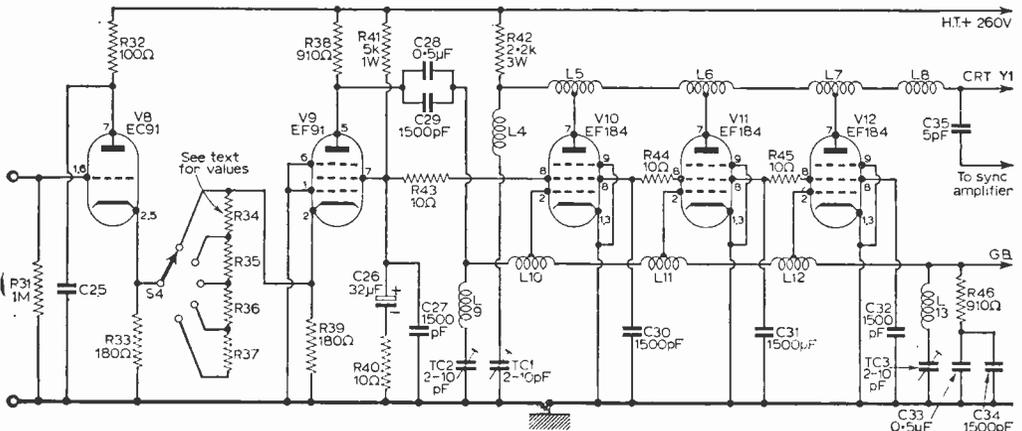
Fig. 3—Attenuator and Y amplifier. Note that C25 is a 16μF electrolytic capacitor.
