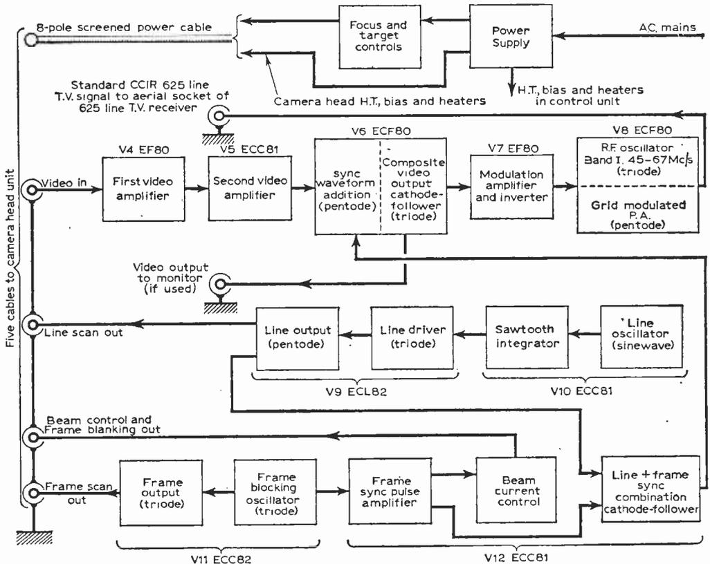
Fig. 3—Basic arrangement of CCTV Control Unit giving 625-line output on CCIR standard, for direct feed to aerial socket of domestic TV receiver. The final article of this series will give full constructional details, including information for obtaining 405-line BBC standard operation if desired.
