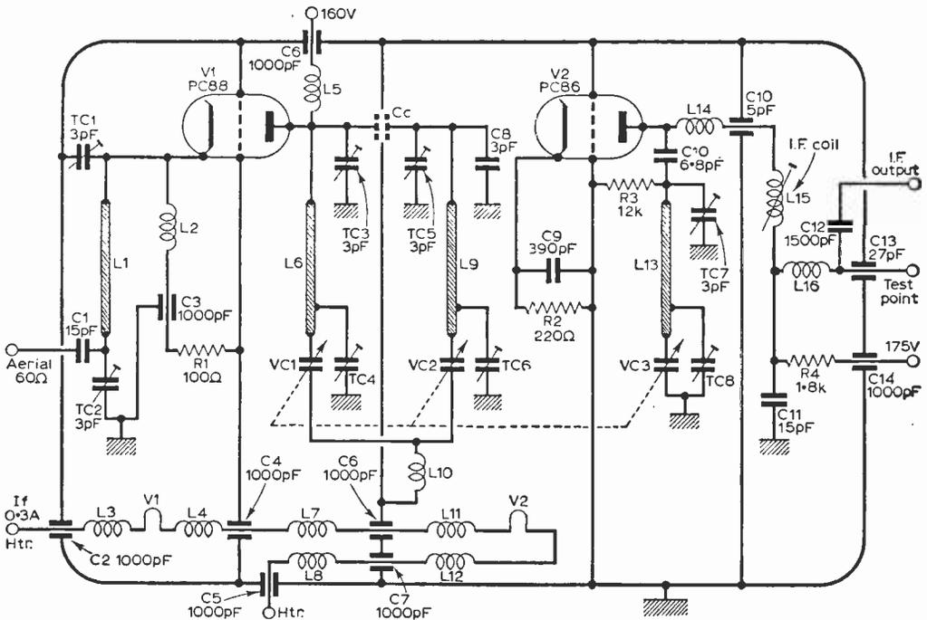
Fig. 14—The circuit of a u.f. tuner, designed by Mullard Limited.
