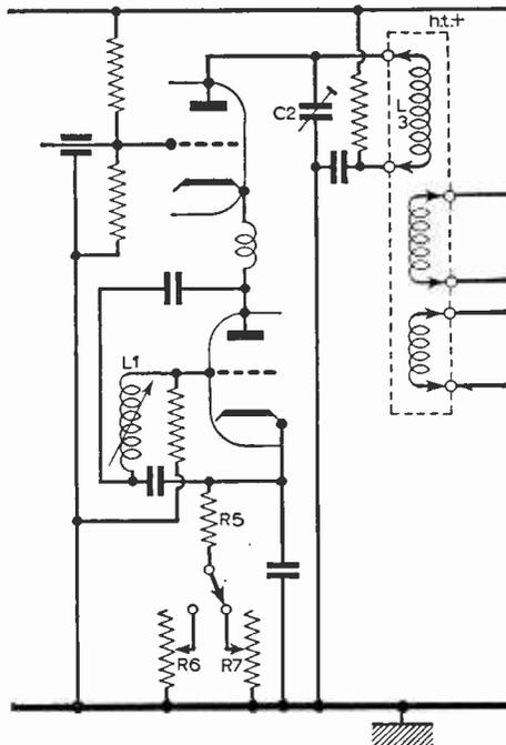
Fig. 1—The basic circuit of a cascode r.f. amplifier.
