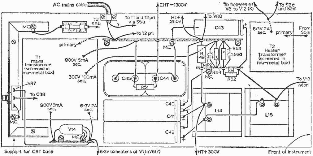
Fig. 20—The wiring of the power deck (see Fig. 13 for the dimensions).
