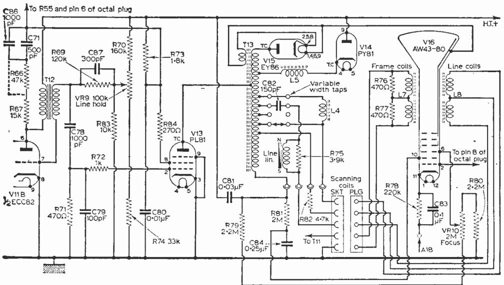
Fig. 2—The line timebase and c.r.t. circuit.
