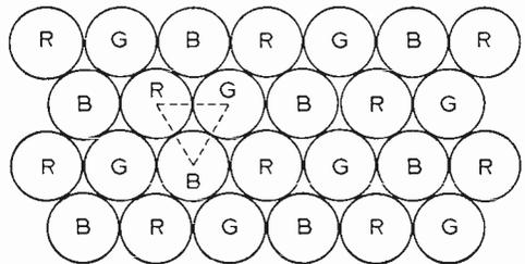
spurious display of other colours—and likewise with blue and green signals. Owing to shortcomings in the manufacture of the tube and the close tolerances that are essential for correct operation, any standard tube without some form of correction would not produce pure colours as described above. On a red only signal, for example, there would be displayed on the screen a red raster distorted by other spurious hues, and likewise with displays due to blue and green signals.
