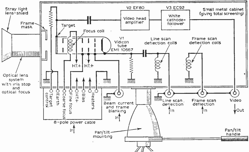
Fig. 2—Basic arrangement of CCTV Camera Head described in this series of articles. The next article will give full constructional details of this head unit. Four coaxial signal cables and one 8-pole screened power cable connect the camera head to the control unit shown in Fig. 3.
