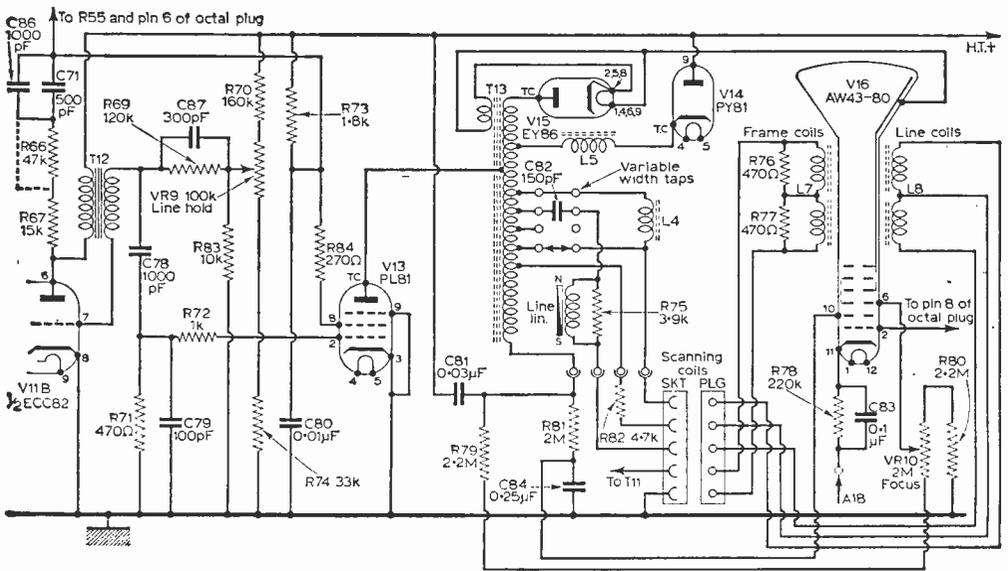
Fig. 2—The line timebase and c.r.t. circuit.
