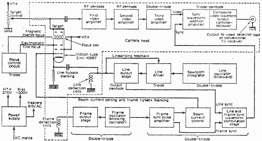
Fig. 1—Basic arrangement of EMI TV-Camera Head for CCTV.
