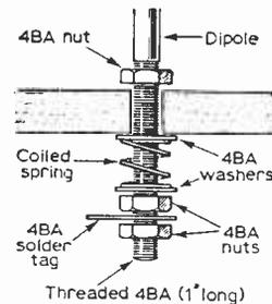
Again, the elements should be connected to the coaxial lead-out cable via 1,000pF isolating capacitors, but there is no need this time to spring-
