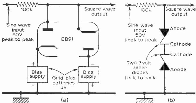
Fig. 10—Methods of producing square waves from arbitrary input signals: a—biased diode clipper pair; b—modern version of a, using backed zener diodes; c (below)—producing square waves by heavy clipping of a sine wave; d (right)—an improved "squarer" using a pentode.
