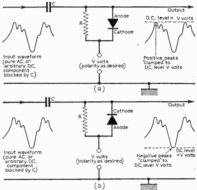
Fig. 11—Clamps or d.c. restorers: a—positive peak clamp or negative d.c. restorer; b—negative peak clamp or positive d.c. restorer.
