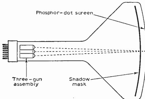
Fig. 19a (above)—Basic structure of the shadow mask colour c.r.t., showing the three-gun assembly. Each tetrode gun is similar to a monochrome counterpart with electrostatic focusing. The three focusing electrodes and final anodes are brought out to common connectors, while the cathodes, grids and first anodes are brought out to separate connectors.
