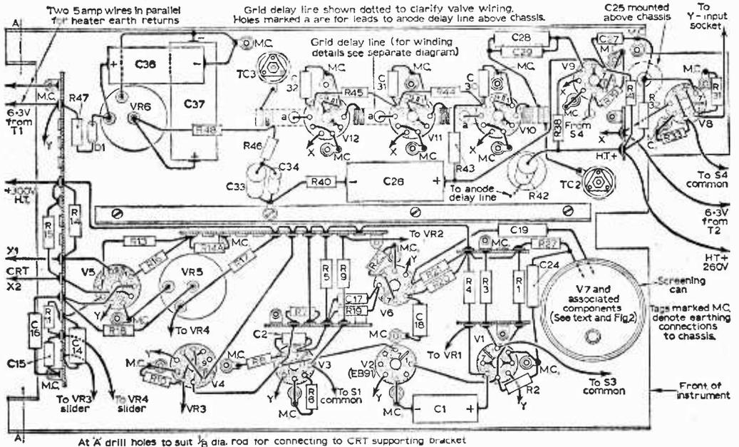
Fig. 19—The top chassis component layout and wiring diagram (for further details of the delay lines see Fig. 9) with overall dimensions also provided.
