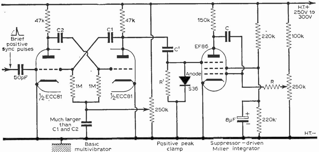
Fig. 13a—Miller integrator timebase with fully external drive from a basic multivibrator. Notes on this diagram should be co-ordinated with the relative text.
