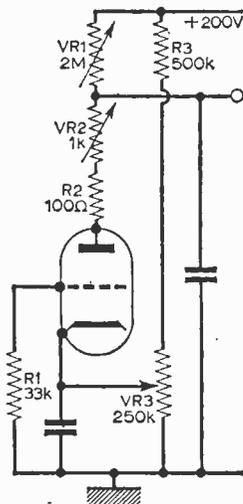
Fig. 21—A substitute for the pulse generator.
