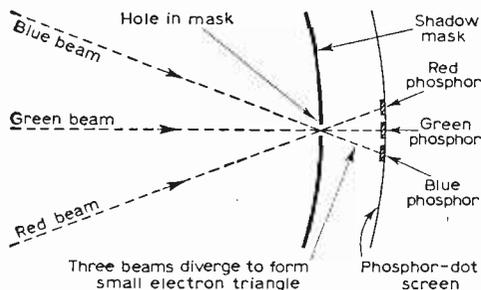
shadow mask. This, of course, means that the tube is running well below maximum efficiency and is one of the shortcomings sometimes levied against the shadow mask technique.
