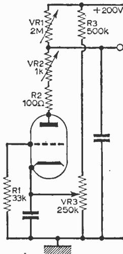
Fig. 21—A substitute for the pulse generator.
