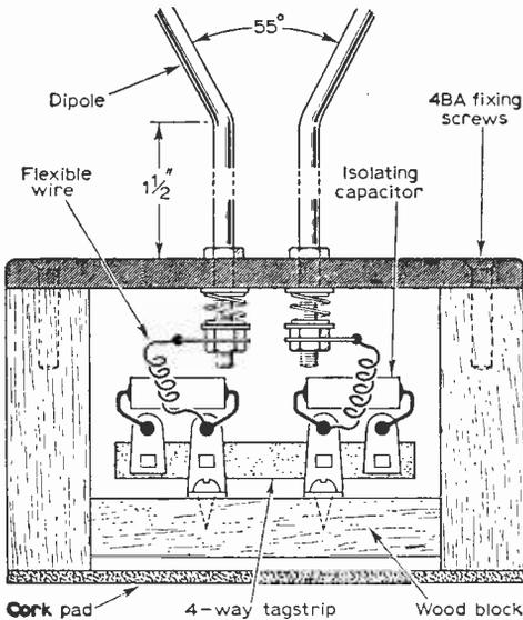
Fig. 1—The basic construction of the "rabbit ears" aerial.
