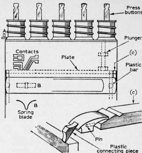
Fig. 7—S.T.C. PC80 push-button tuner.
