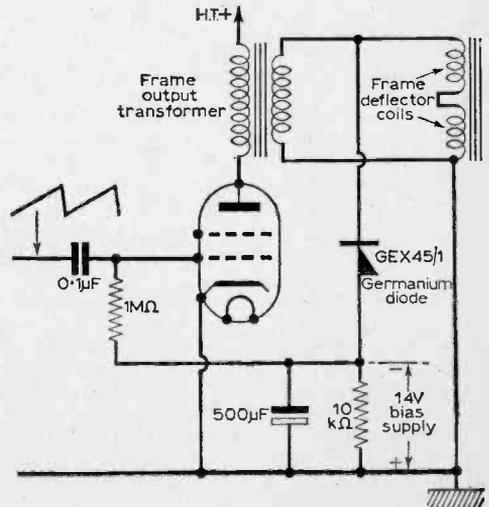
of the sawtooth waveform existing across the line or frame output transformer and by rectifying this provide the necessary bias potential required. Circuit details are shown in Fig. 8. Since very little current is drawn from this bias source no damping will occur across the frame circuit. For the same reason a small germanium diode can serve as the rectifier.
