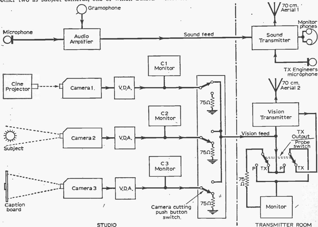
Fig. 1—Block diagram of the station equipment.
