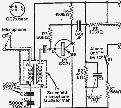
Fig. 2—Circuit of the baby alarm amplifier. The OC71 transistor is powered from the h.t. line of the receiver via potential-divider R1 and R2. Extra smoothing is given by C1. For double safety, two isolating capacitors C2 and C3 are used in the microphone circuit. These must be no larger than 5,000pF and rated at 330V a.c.
