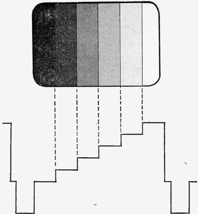
Fig. 11—The top diagram shows the monitor display; the bottom diagram shows the line frequency waveform.
