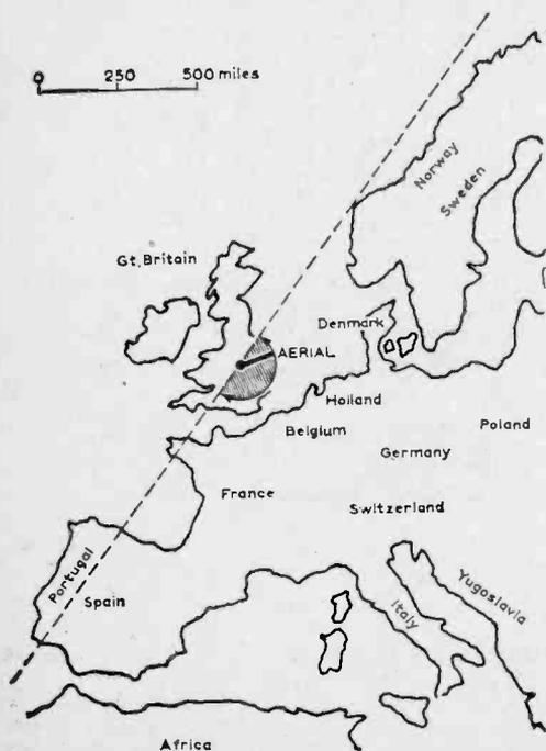
Fig. 1—Showing how a swing through 180° enables the aerial to line up on transmitters all over the continent.
