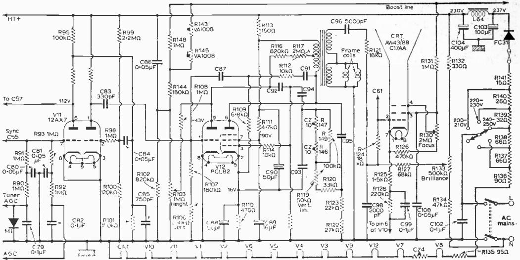
Fig. 5—The sync separator, frame timebase, c.r.t. and power stages.
