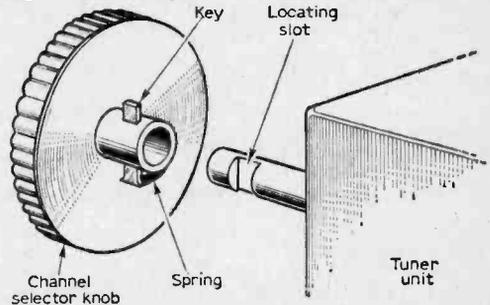
Fig. 3—The channel selector knob of the T380 group of receivers. The key should be pressed down with a knife blade to release the knob.
