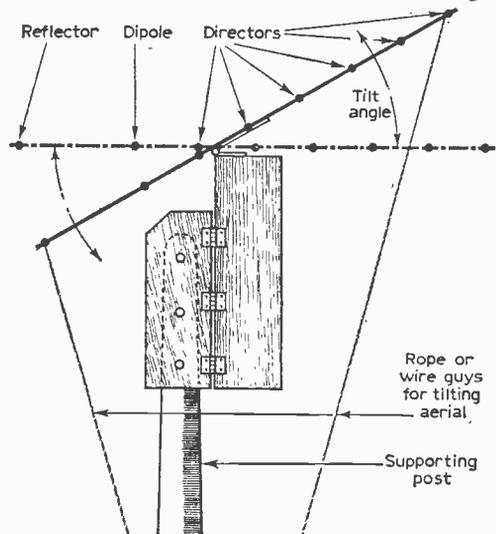
Fig. 2—Illustrating how the aerial tilts up and down on its axis.
