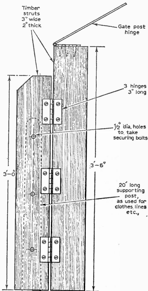
Fig. 3a (above)—A front elevation of the aerial support.
