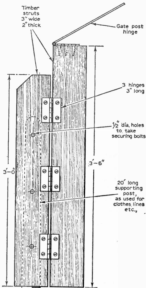
Fig. 3a (above)—A front elevation of the aerial support.
