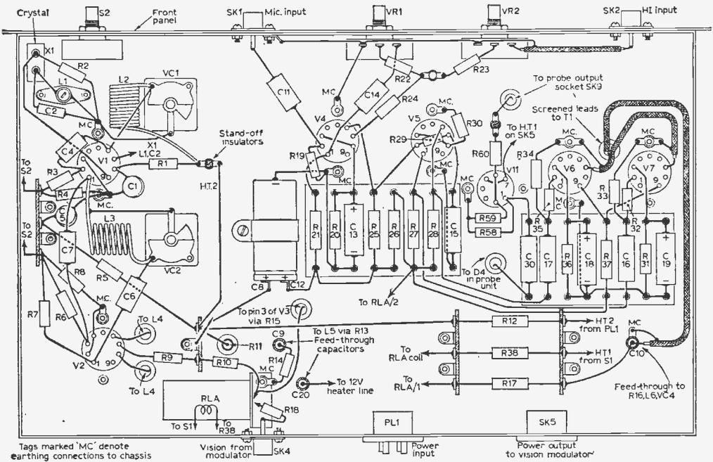
Fig. 9—Underside view of the r.f. and sound modulator unit showing components and major wiring. Note that wiring relating to the following circuits is not shown, or only in part: valve heaters; relay; switches S1 and S2; power supplies; PL1; SK5.
