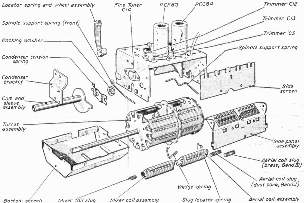
Fig. 1—The construction of a typical turret tuner.
