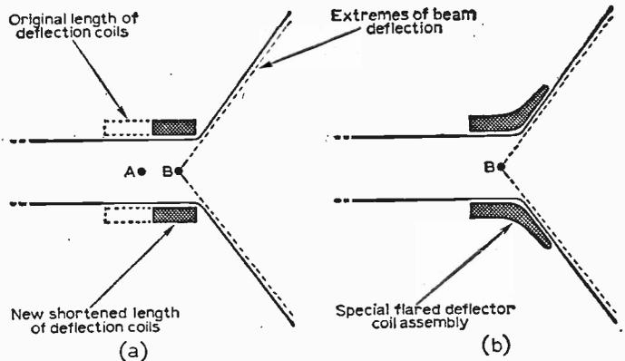
shortened (Fig. 10a) or the deflection coils can be flared to take them further up the neck of the cathode ray tube (Fig. 10b).
