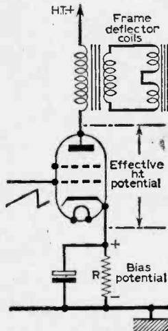
Fig. 7 (left)—The normal bias arrangements of the frame output circuit.
