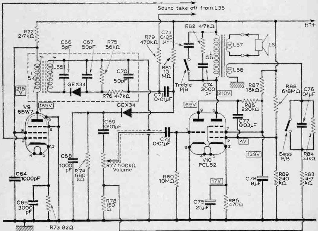
Fig. 4—The sound i.f. and audio stages of the models QV30/1 and QV70.
