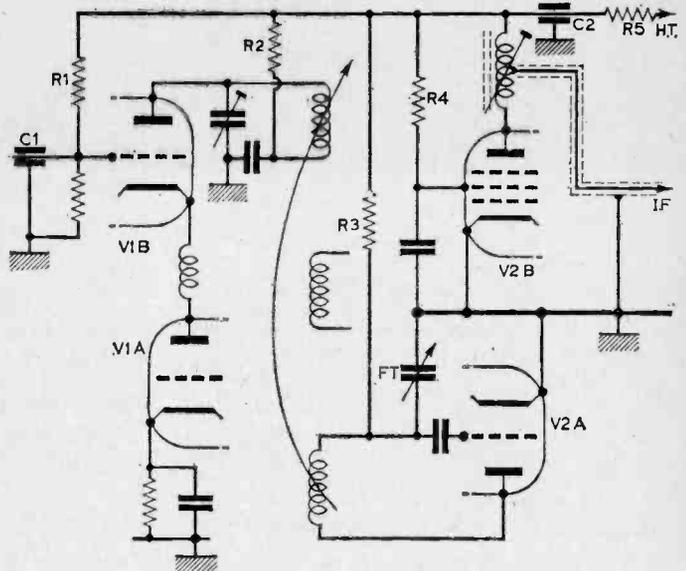
Fig. 3—Faults in the oscillator circuit.
