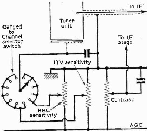
Fig. 4—Contrast and sensitivity arrangement.
