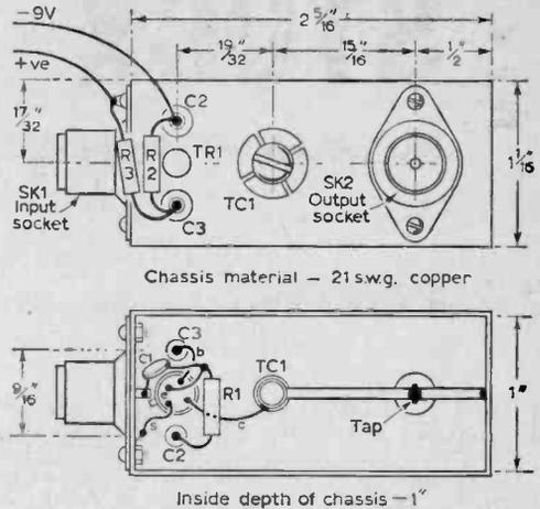
Fig. 2—Top and underside views showing the wiring details.
