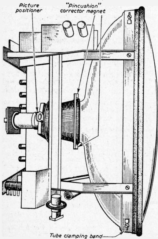
Fig. 3—Sketch showing the layout and chassis assembly of the Regentone Ten 17.
