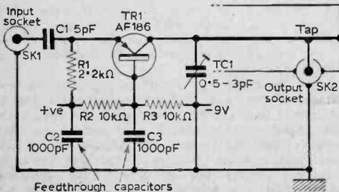
Fig. 1—Circuit diagram of the u.h.f. preamplifier.
