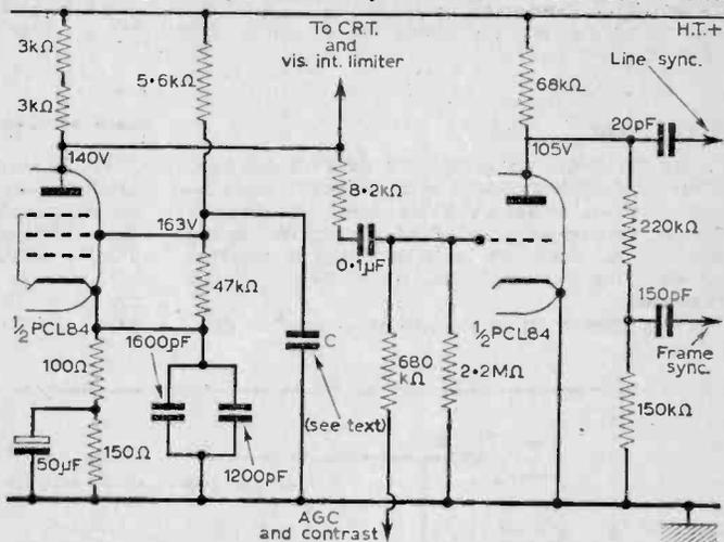
Fig. 28—Ferguson 506T, etc., video output and sync separator circuit, using a single PCL84 valve.
