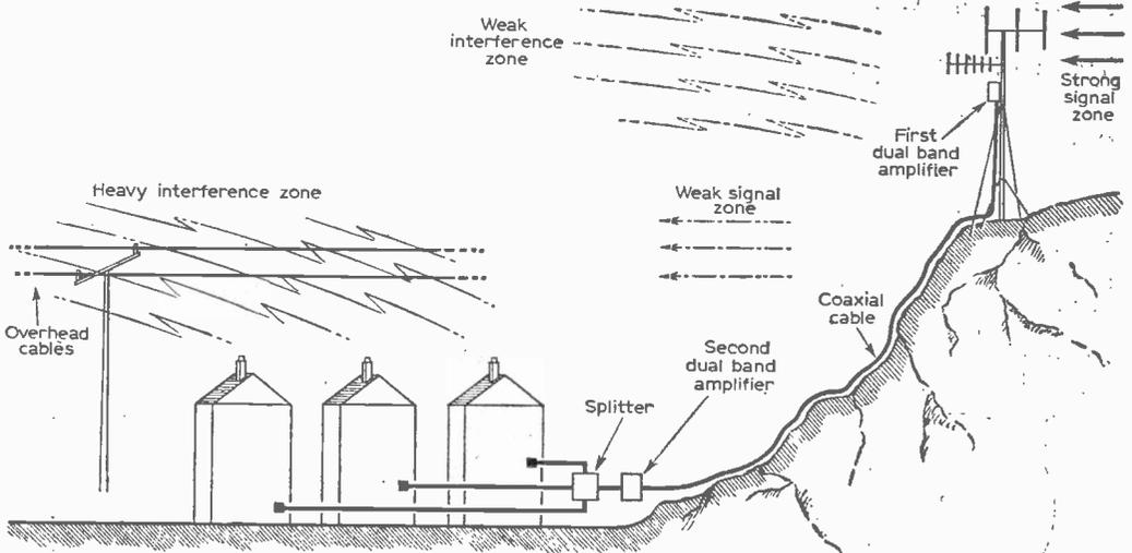
Fig. 1—Example of a hill-mounted aerial to improve the signal/interference ratio. By the use of amplifiers and a splitter a number of viewers may be fed from the one aerial, thereby reducing costs. The masthead amplifier could be powered from a small unit at the set end of the coaxial cable; using the cable to feed power to the amplifier as well as to feed signal to the sets.
