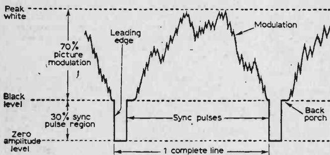
Fig. 24a—Signal waveform, showing relative positions of synchronising pulses, zero, black and peak white amplitude levels.
