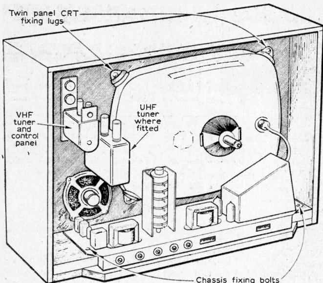
Fig. 2: Back view of the K-B Model WV20, showing location of major components.
