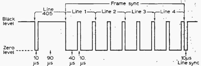
Fig. 25—Train of pulses at commencement of frame. The frame pulse is integrated from the eight half-line pulses of the first four lines of the picture. Each half-line pulse is separated by an approximate 10μs interval, to trigger the line timebase correctly during the frame period.
