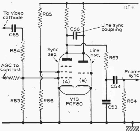
Fig. 26—Pye V200 sync separator. Component values: C65, 0.1μF; R84, 10kΩ; R83, 2.2MΩ; R85, 47kΩ; R86, 22kΩ; C66, 15pF, 750V; R63, 220kΩ; C53, 220pF; C54, 0.01μF, R64, 150kΩ.
