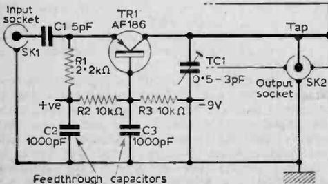
Fig. 1—Circuit diagram of the u.h.f. preamplifier.
