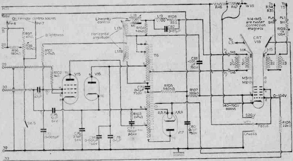
Fig. 6—Line output stage, e.h.t. rectifier and cathode ray tube.
