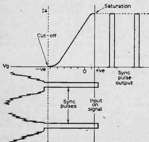
Fig. 24b— $V_g/I_a$  curve for saturated pentode type of sync separator, with input as Fig. 24a. Polarity of applied signal is arranged to drive the valve rapidly from cut-off to saturation when the sync pulse arrives. Anode current drops rapidly again when the sync pulse ceases. Duration of sync pulse is approximately 10 $\mu$ s, occurring at 100 $\mu$ s intervals.
