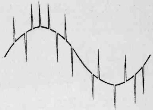
Fig. 3—Showing spikes of impulsive interference superimposed upon a signal waveform.
