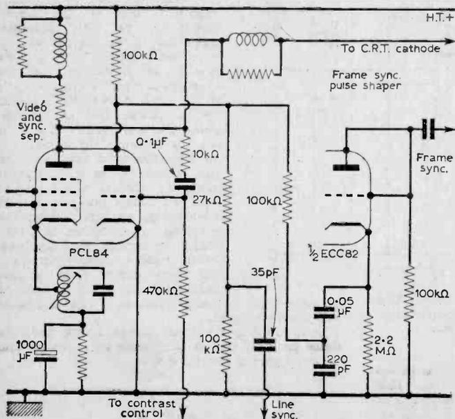
Fig. 27—McMichael MPI8, etc., video, sync separator and frame pulse shaper circuit.
