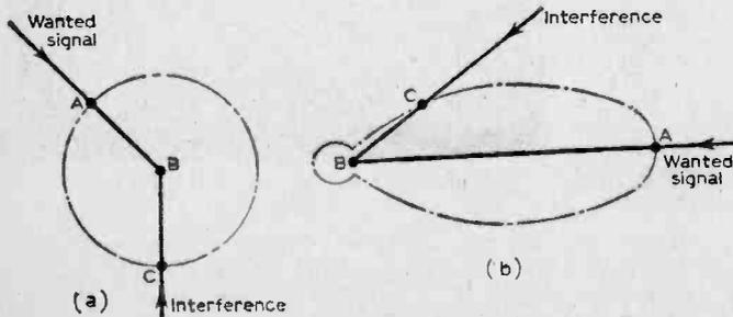
Fig. 2—An omnidirectional aerial at (a) gives response to interference equal to that of the required signal. B-C equals B-A. A directional aerial, however, can be orientated for the best ratio between the signal and the interference. Here the response B-A is greater than the response B-C.
