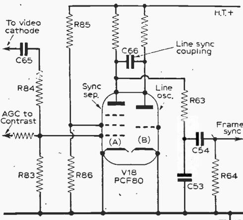
Fig. 26—Pye V200 sync separator. Component values: C65, 0.1μF; R84, 10kΩ; R83, 2.2MΩ; R85, 47kΩ; R86, 22kΩ; C66, 15pF, 750V; R63, 220kΩ; C53, 220pF; C54, 0.01μF, R64, 150kΩ.
