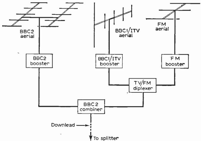
Fig. 7—BBC-2 signals nearly always require separate amplification before combining, as shown here.
