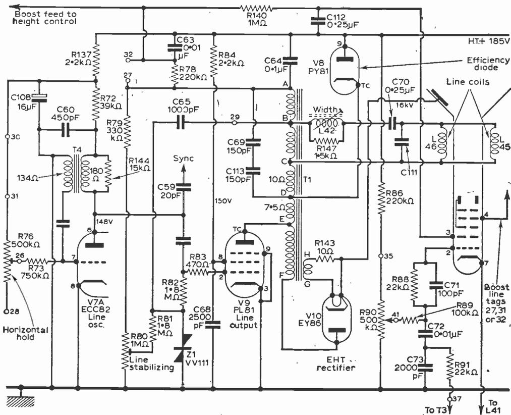
Fig. 5—The line timebase of the schedule C versions of the receivers.
