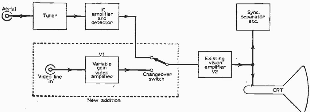
Fig. 1—A simplified block diagram of a television receiver, indicating the additional sections.
