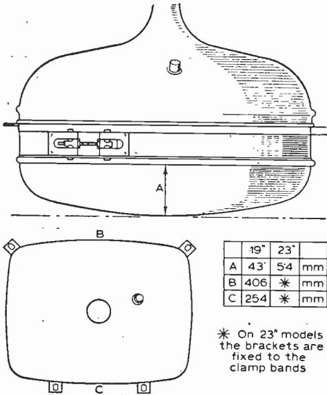
Fig. 2—Critical measurements to be observed with the 19TG111A series.
