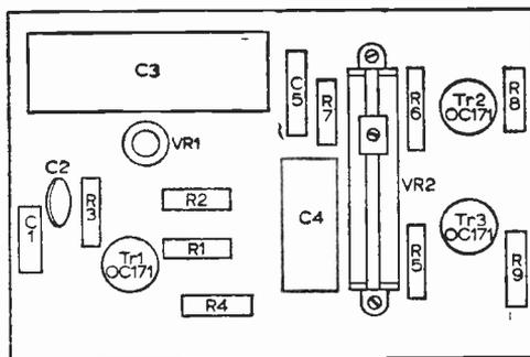
Fig. 6—A suggested layout for the distribution amplifier, for either printed circuit or conventional wiring.
