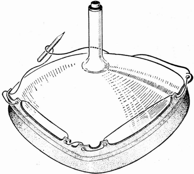
Fig. 3—Refitting the Cornehl safety hood to the latest type of tube.
