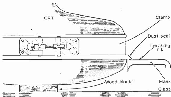
Fig. 1—Tube replacement diagram for the 17TG100U. The wood block fitted to ensure correct spacing between the c.r.t. and the glass should be 7mm thick.
