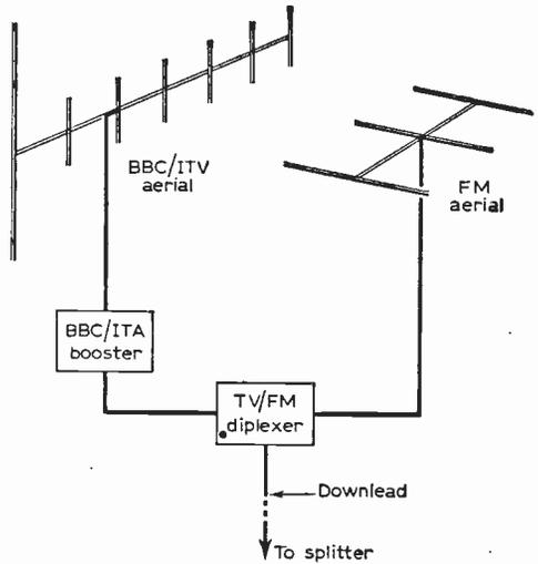
Fig. 6—Here is shown how f.m. is added to a master aerial system. If the f.m. signal is weak, a boost can be supplied with a separate f.m. booster.
