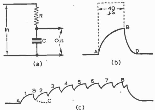
Fig. 37—Integration of the frame pulses: (a) basic integrator circuit, (b) output from an integrator when a square pulse is applied, (c) effective waveform produced from a chain of integrated pulses.
