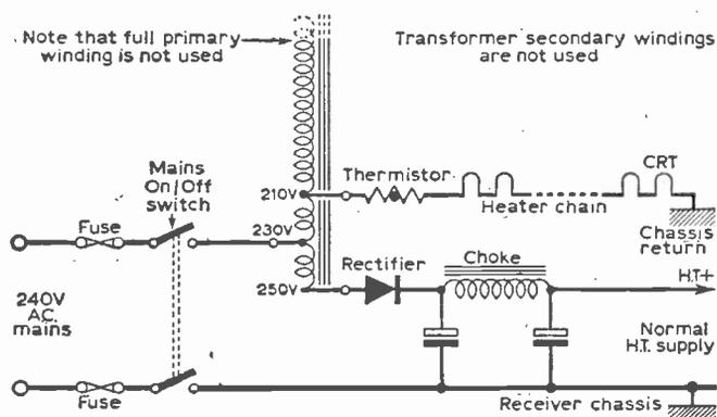
Above—The circuit arrangement evolved by Mr. Amor from his experiments to eliminate the mains dropper in television receivers. The modification makes use of part of an old mains transformer.
