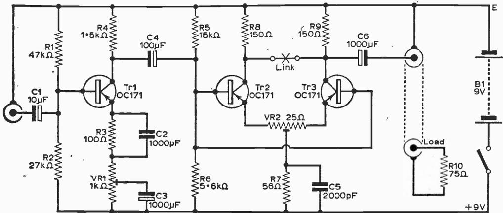
Fig. 4—The circuit of a vision distribution amplifier.
