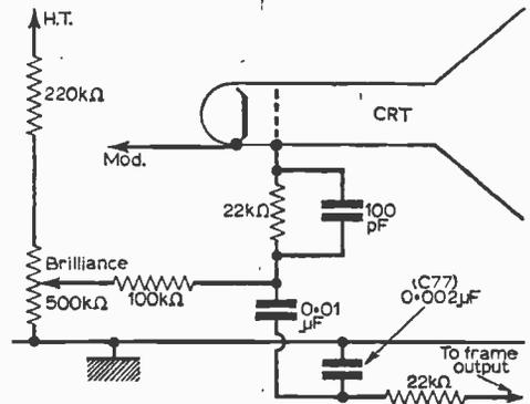
Fig. 42—Marconi method of frame flyback suppression. Open-circuiting of C77 induces vertical hum bars on the raster.
