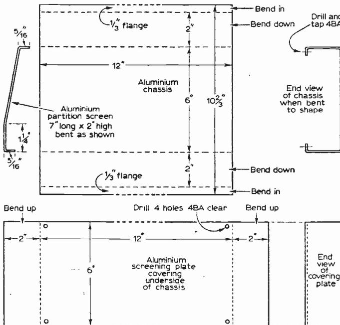
Fig. 7—The sub-chassis covering screens essential to prevent remaining timebase transients reaching the Y-amplifier and interference from direct pick-up of broadcast stations.
