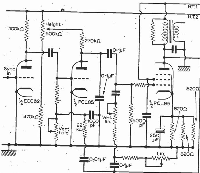
Fig. 38—Sobell T279 frame circuits. Sync pulse shaper, back-coupled triode oscillator and pentode output are typical of many circuits.
