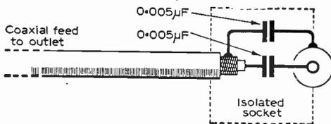
Fig. 8—It is desirable to isolate both the inner and outer conductors at each outlet, as this illustration shows.
