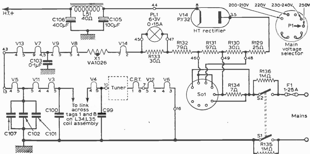
Fig. 4—The power supply and heater circuits.
