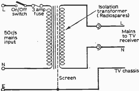
Fig. 3—Making the receiver safe for use as a monitor by the inclusion of an isolation transformer.
