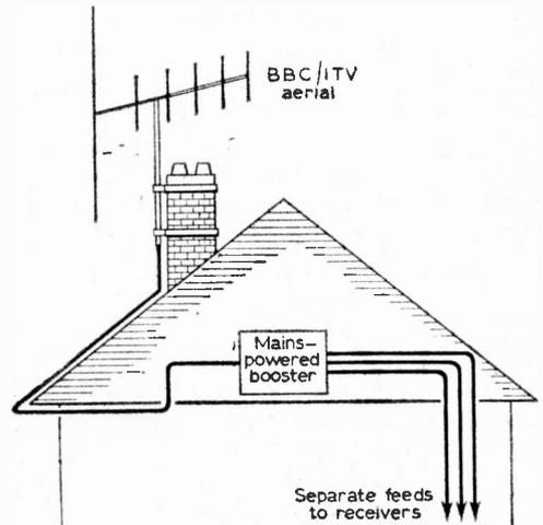
Fig. 4—The mains-powered signal booster can be housed in the roof space. Continuous powering is feasible, for the consumption is very small, amounting to a few pence of electricity per year.
