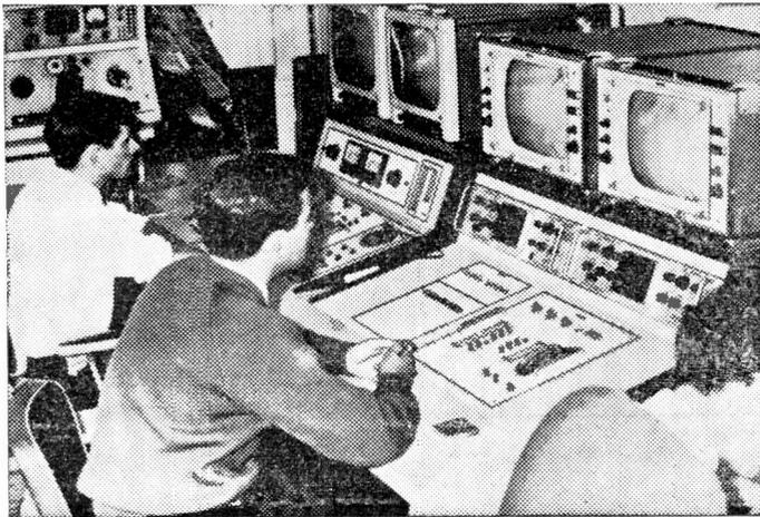
**T**HIS photograph shows presentation switching equipment made and supplied by EMI Electronics Ltd., in service at the Wellington studios of the New Zealand Broadcasting Corporation.
