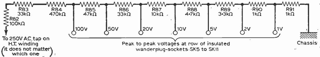
Fig. 5—Y-calibrator circuit. R82 may need reduction or omission, as one half-wave is flattened at the 250V transformer tap, on the conduction-half cycle of the main h.t. rectifier section on this side. This reduces the operative peak-to-peak voltage.
