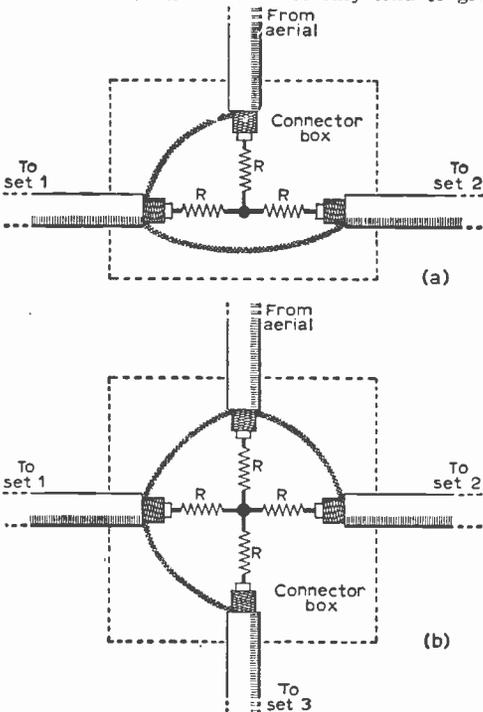
Fig. 2—Connections to more than one set from a common aerial system should always be made through resistors, as shown at (a) for two outlets and at (b) for three outlets. The value for  $R$  can be found by a simple calculation as detailed in the text.
