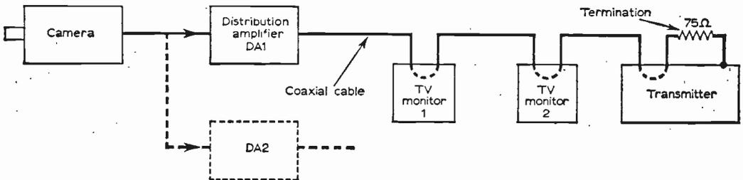
Fig. 5—An amateur television station set-up including a distribution amplifier (DA).
