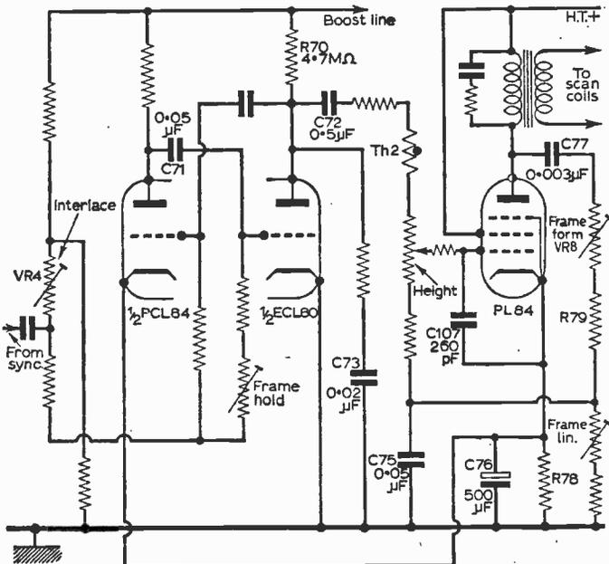
Fig. 39—Decca frame circuit. Note the interacting hold and interlace controls, the series feedback circuitry and the oscillator h.t. feed from the boost line.
