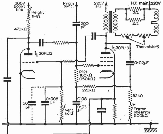
Fig. 41—Ultra frame circuit. A single linearity control is employed and thermistors are fitted in the output transformer secondary circuit to damp flyback pulses and compensate for changing characteristics with heat increase.
