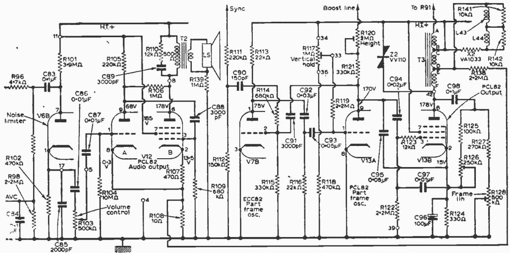
Fig. 6—The sound output and frame timebase stages of the circuit.
