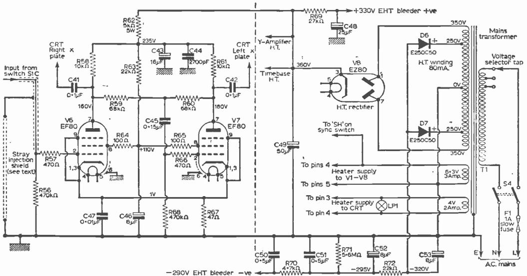
Fig. 4—X-amplifier and the power supplies. Conventional components are used in the power supply, and the X-amplifier can be used with an external signal or with the built-in timebase of Fig. 2 (last month). To avoid h.t. surges, V8 may not be replaced by a metal rectifier.
