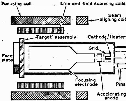
Fig. 1—Cross-section of the vidicon camera tube and its associated control elements.
