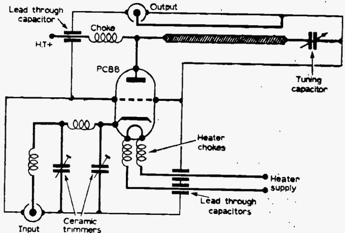
Fig. 5—This is the circuit of the amplifier depicted in Fig. 4.
