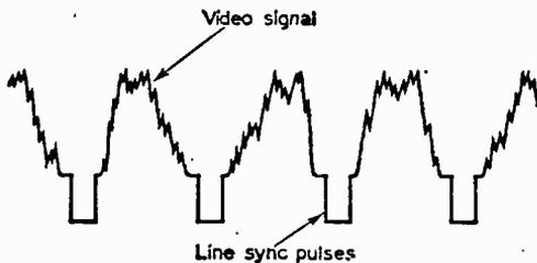
Fig. 5—Here is shown how the sync pulses are added between the lines of picture signal.
