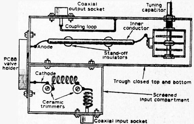
Fig. 4—Here is shown the cross-section of a valve u.h.f. amplifier featuring a transmission line of the nature described in the text.
