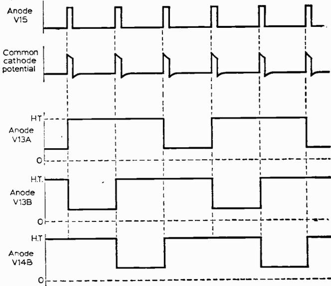
Fig. 5—The ring-of-three counter waveforms.
