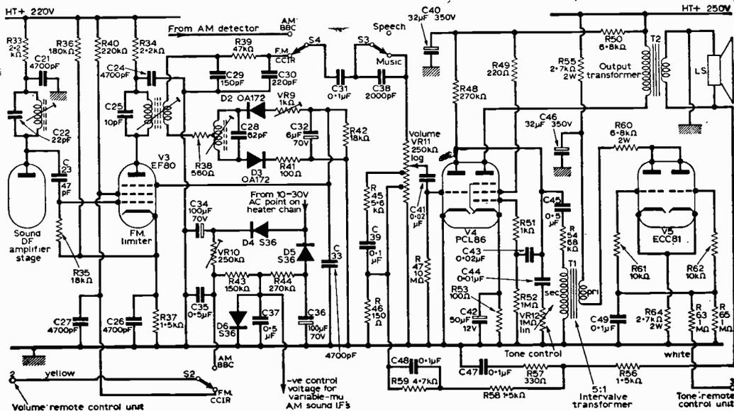
Fig. 4—The audio circuitry of the author's receiver. The f.m. limiter and ratio detector sections for 625-line f.m. sound are included, since these are used for remote volume control on f.m. sound reception.
