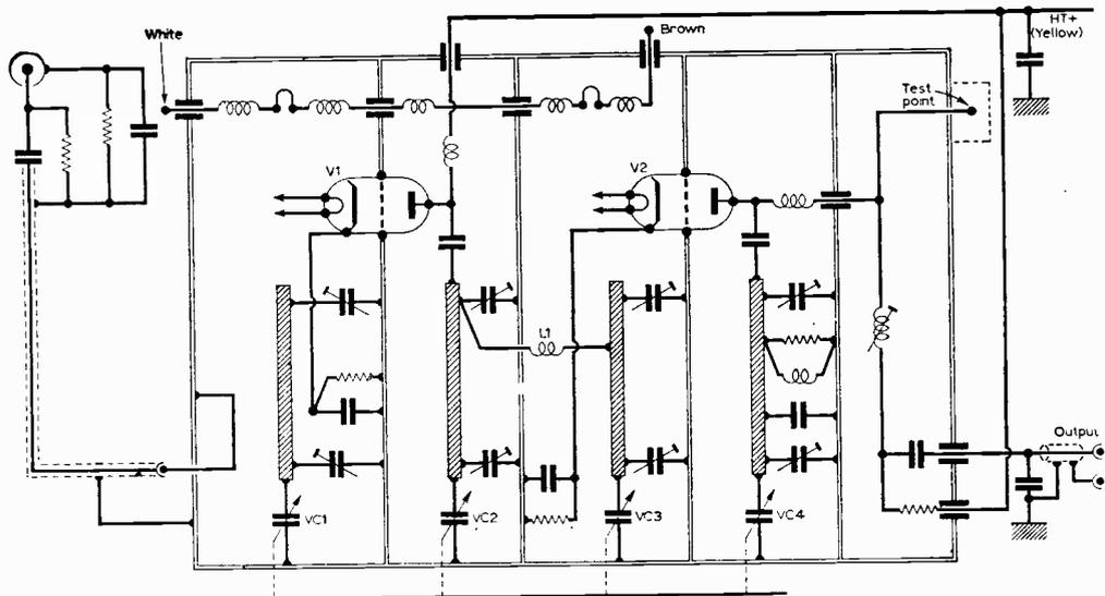
Fig. 7—The complete circuit of a u.h.f. tuner using transmission lines for tuning. This is described in the text.
