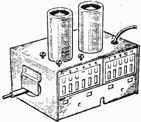
Fig. 3—A typical converter with its side plate removed to show the contacts to the switch banks.
