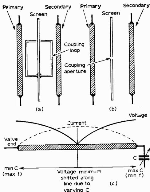
Fig. 6—(a) and (b) show link and aperture coupling between two lines respectively. At (c) it is shown how the minimum voltage point is caused to move along the line by adjusting C. As shown, the circuit is at the centre of its tuning range.
