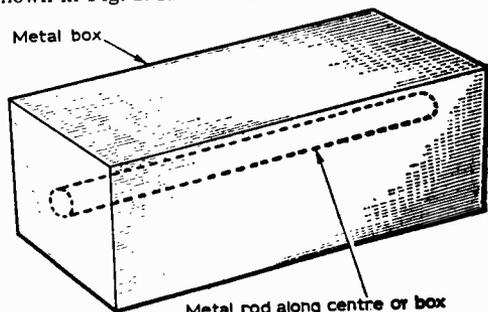
Fig. 2—A simple transmission line consists of a metal rod enclosed by a metal box. It has a characteristic impedance
