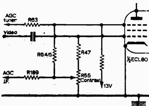
Fig. 7—Simple suppressor-regulated a.g.c. circuit used on later Philips models, with variations. A.G.C. is derived from the sync separator, and delay by suppressor grid biasing.
