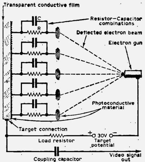
Fig. 3—This diagram shows the basic electronics of the vidicon operation, as detailed in the text.
