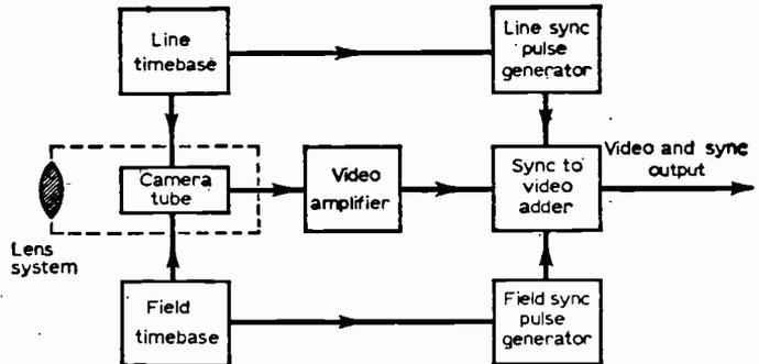
focuses the image of the scene upon the target of the camera tube, that the resulting video signal output is amplified in the video amplifier and then applied to an "adder" which, from the appropriate line and field sync pulse generators, adds the sync pulses to the video signal.
