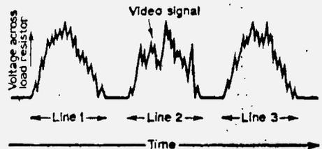
Fig. 4—Three lines of video signal. The spaces between the lines are due to the flyback time of the line timebase.
