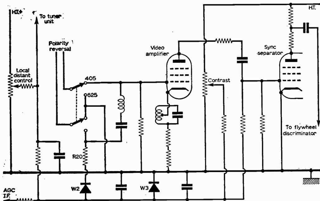
Fig. 8—Thorn 850 a.g.c. circuit, showing additional control necessary when switching to 625-line operation.
