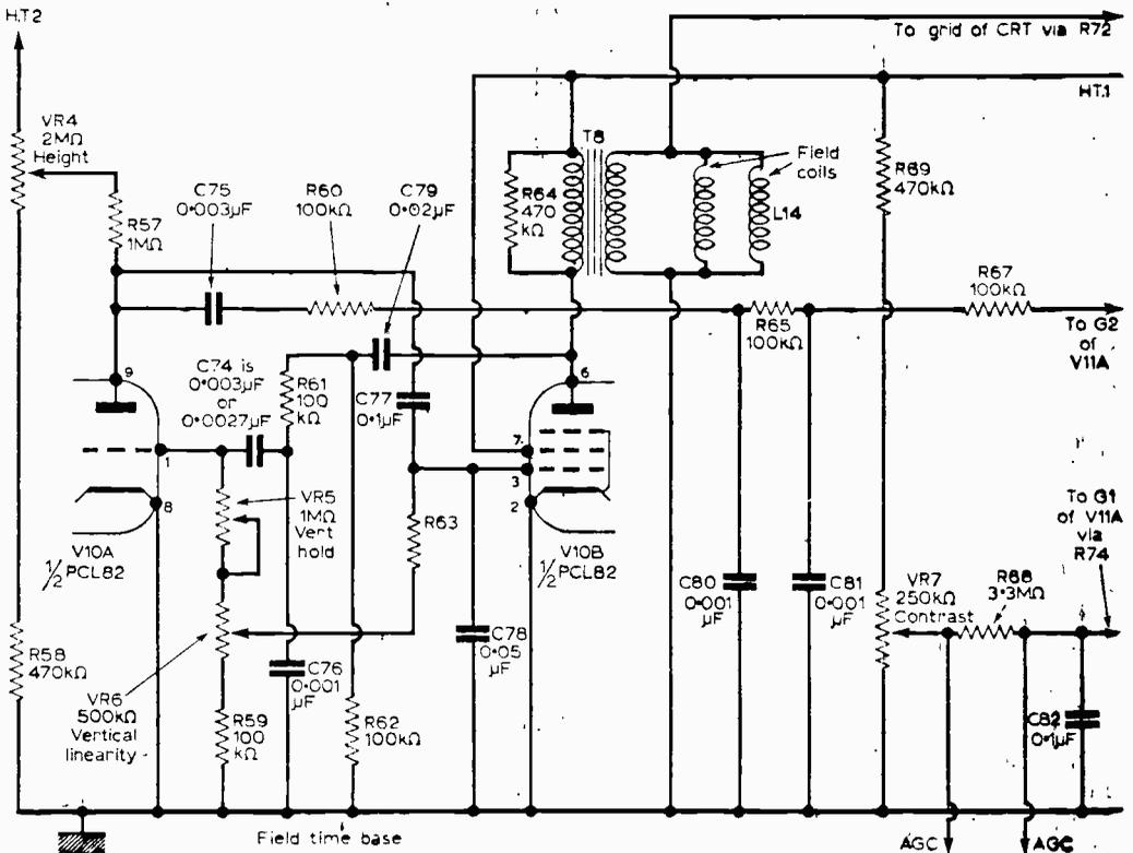
Fig. 1—The field timebase stage of the circuit.
