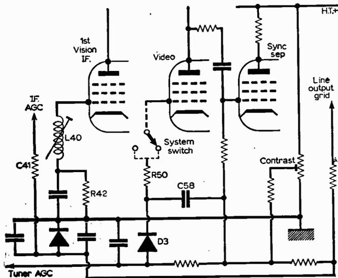
Fig. 9—Kolster-Brandes a.g.c. circuit, as used in the VV series. Protection circuits are incorporated, and delay effected by separate a.g.c. feed lines.
