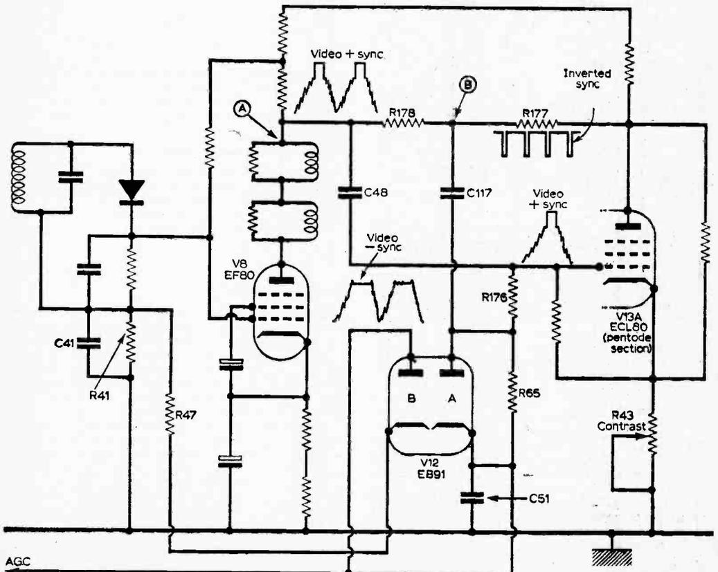
Fig. 6—Earlier Philips type of a.g.c. circuit, with waveforms included. Sync-cancelling system is employed, the resultant of three voltages producing the necessary control.
