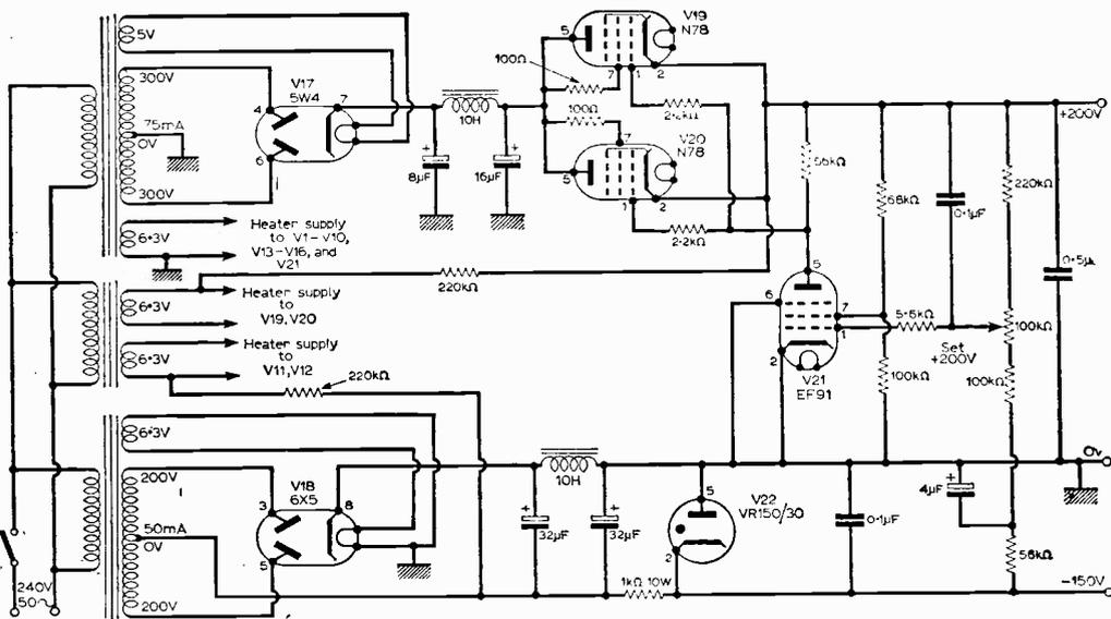
Fig. 6—The power supply circuit, which is entirely conventional.
