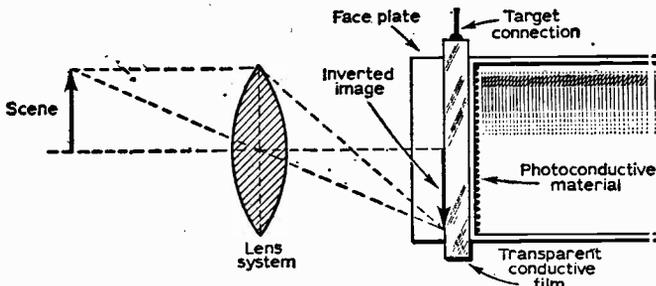
Fig. 2—A detailed view of the target assembly of the vidicon camera tube.
