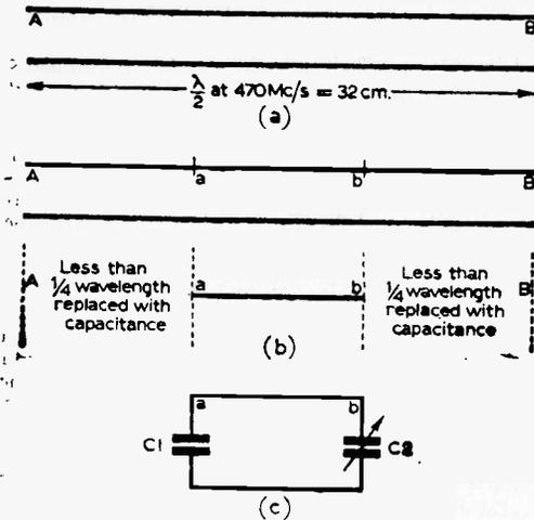
Fig. 3—The length of a half-wave transmission line unloaded is 32cm at 470Mc/s (a). By cutting off a slice of the line at each end and replacing the pieces cut off by capacitance, the line A-B can be reduced in length to (b). The finished configuration is shown at (c) and the line a-b is 5cm.
