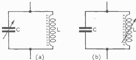
Fig. 1—The resonant frequency of a circuit in which capacitance is connected in parallel with inductance can be altered either by varying capacitance,  $C$  (a) or inductance,  $L$  (b). Increasing either decreases the tuned frequency.
