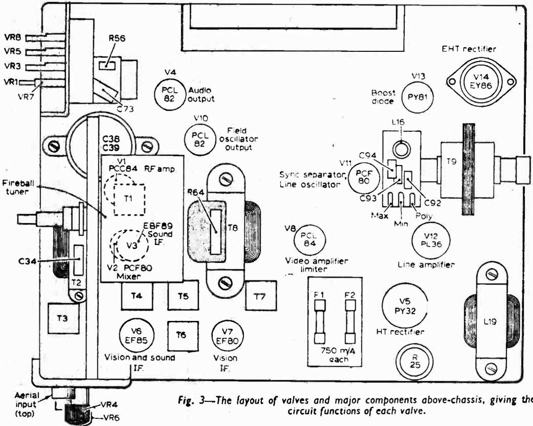
Fig. 3—The layout of valves and major components above-chassis, giving the circuit functions of each valve.
