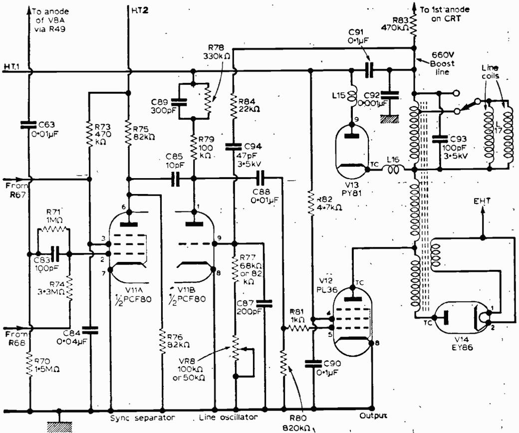
Fig. 2—The line timebase and amplifier and sync separator sections.
