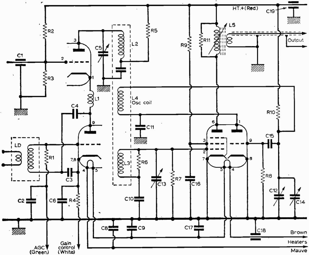
Fig 4.—The circuit of a typical turret tuner.
