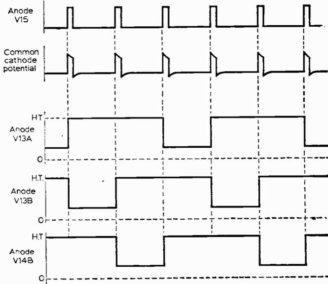
Fig. 5—The ring-of-three counter waveforms.
