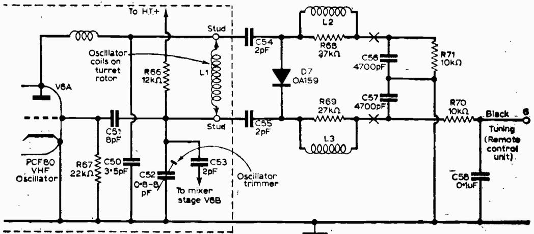
Fig. 5—This circuit shows how a variable capacitance diode D7 may be added to virtually any TV turreted tuner, as a simple means of remote fine tuning.
