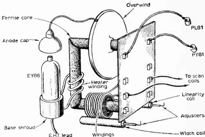
Fig. 6—Typical line output transformer assembly, with mounting brackets, etc., omitted.
