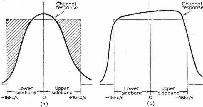
Fig. 8(a): A narrow channel response suppressing the higher frequency ends of the sidebands. On sound this would result in treble attenuation and on vision lack of definition. (b): The whole range of sidebands accepted without attenuation by a suitably wide channel response.
