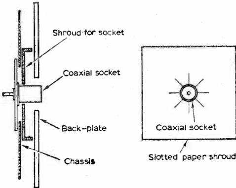
Fig. 5: Insulating the aerial input socket.
