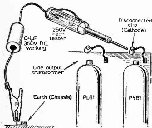
Fig. 5—Voltage tests, using only standard neon tester and capacitor. See text for interpretation.
