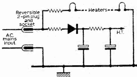
Fig. 1: Mains input-circuitry of a typical a.c./d.c. receiver.
