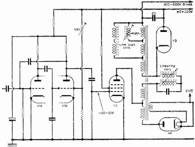
Fig. 4—Typical line oscillator and output section of modern receiver. Multi-vibrator oscillator V1 drives amplifier V2. Speed of oscillation is controlled by VR1. Flyback pulses are rectified by V3 and developed across C1 to produce boost voltage. V4 is E.H.T. rectifier, with heaters powered via a separate winding (see also Fig. 6).
