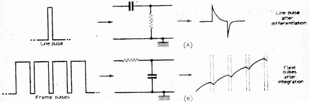
Fig. 3 (A)—Differentiating and (B) integrating [frequency selective circuits and their effect on line and field pulses respectively.]
