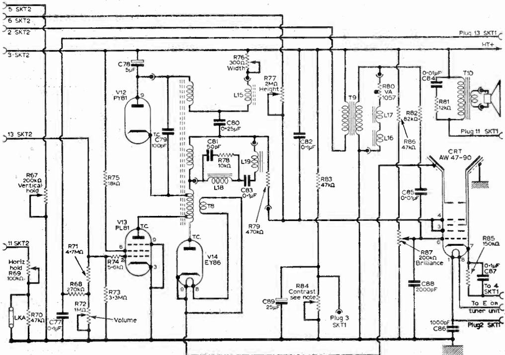
Fig. 3: The line output and c.r.t. circuit.
