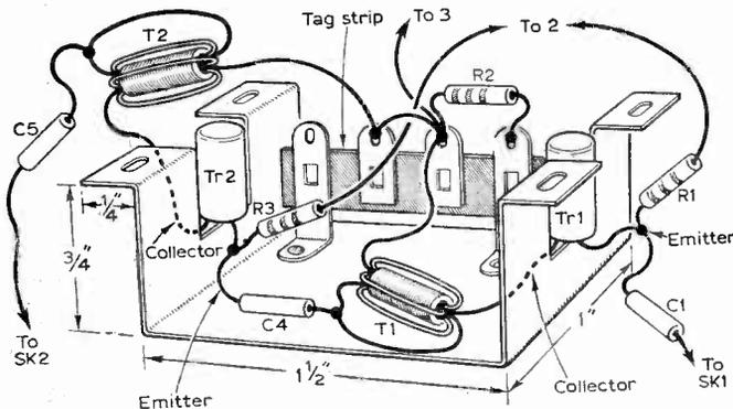
Fig. 5—Point-to-point wiring details of the sub-assembly.
