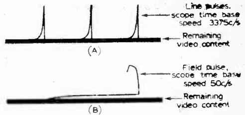
Fig. 2—Synchronising pulses at the anode of the sync separator, as seen on an oscilloscope.
