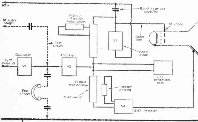
Fig. 3—Principles of flyback-derived E.H.T. system, showing test points and features discussed in the text.
