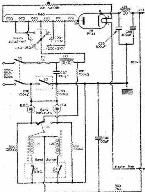
Fig. 1: Mains input stage.
