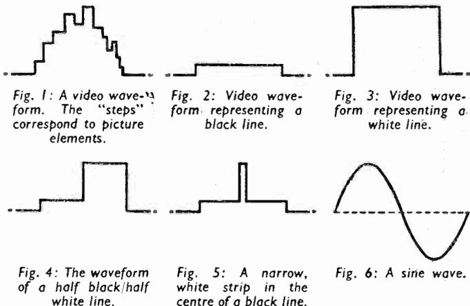
The result is a video waveform, and this is generally shown for each line of picture. The basic idea is given in Fig. 1. This represents a complex line; that is, one that has a widely changing variation of tones (between black and white).
