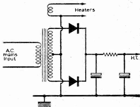
Fig. 2: A.C. only receiver mains input circuitry.
