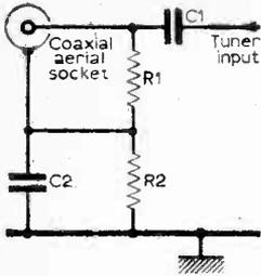
Fig. 3: Isolation of the aerial input circuit.
