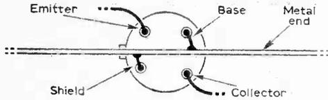
Fig. 6—This diagram identifies the transistor lead-outs and shows how the transistors are mounted.
