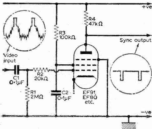
Fig. 1—The basic pentode sync separator circuit.
