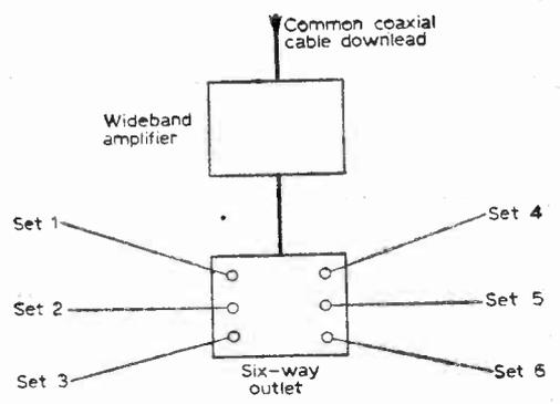
Fig. 2—The amplifier can also be employed to feed signals in all channels to six receivers, as shown.
