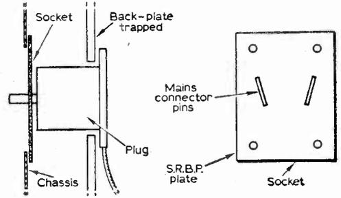
Fig. 6: Standard type mains input socket.
