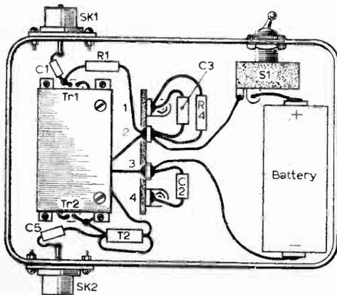
Fig. 7—Point-to-point wiring diagram of the complete unit.
