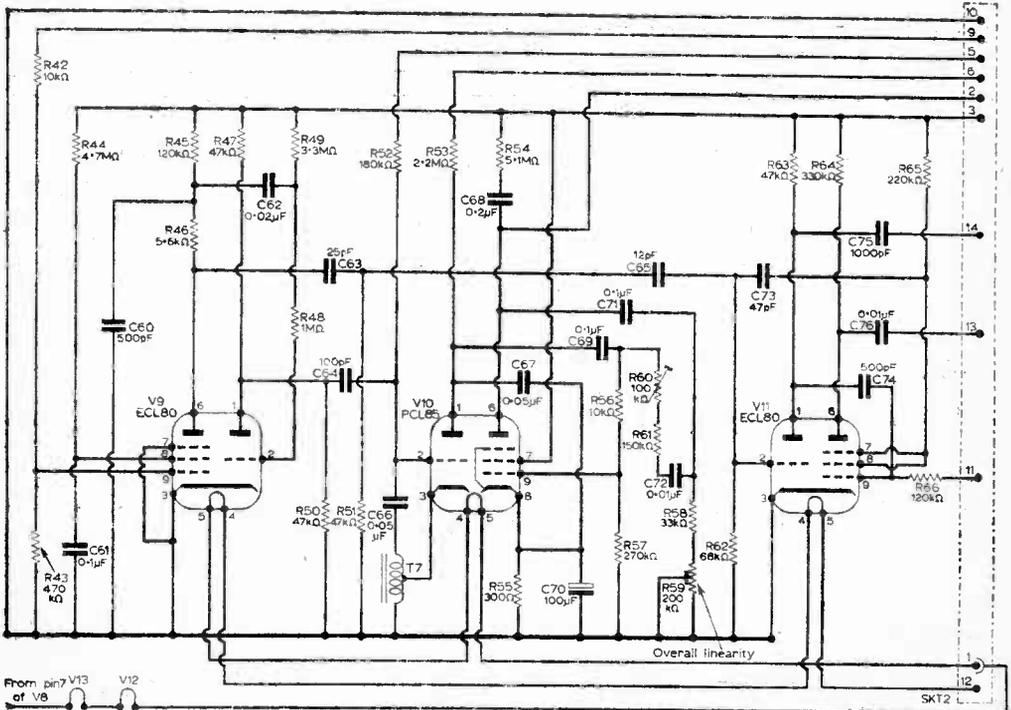
Fig. 2: Sync separator, frame oscillator and output, and line oscillator.
