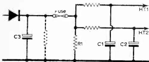
Fig. 8: Typical mains input circuitry with h.t. fuse.
