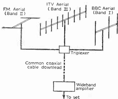
Fig. 1—The amplifier can be connected to a common downlead as shown to amplify all signals simultaneously.
