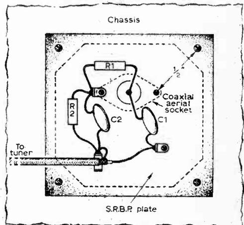
Fig. 4: Practical layout of components shown in Fig. 3.
