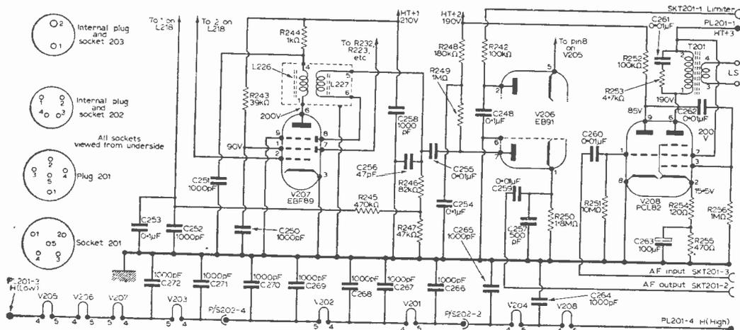
Fig. 4—Sound i.f. and output stage.
