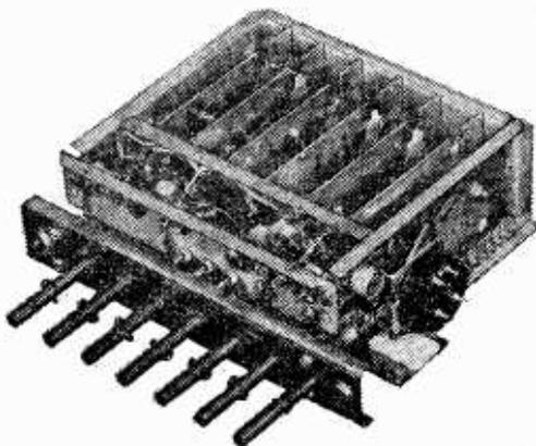
**D**URING recent times there have been many developments associated with the front ends of television receivers. In very early sets the front end consisted first of an r.f. amplifier and frequency changer built into the main chassis and fixed-tuned to one local Band I channel. Then a modification arose whereby the front end could be pretuned to any one channel in Band I.
