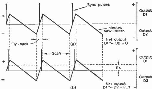
Fig. 2—Discriminator action of Fig. 1. When sync pulses coincide with points of zero voltage on the injected sawtooth waveform as at (a) the net discriminator output is zero, and the line oscillator receives no controlling voltage. If the t.b. alters its frequency so that these points fail to coincide as at (b), a positive or negative controlling voltage is developed to restore the t.b. frequency to its original state.
