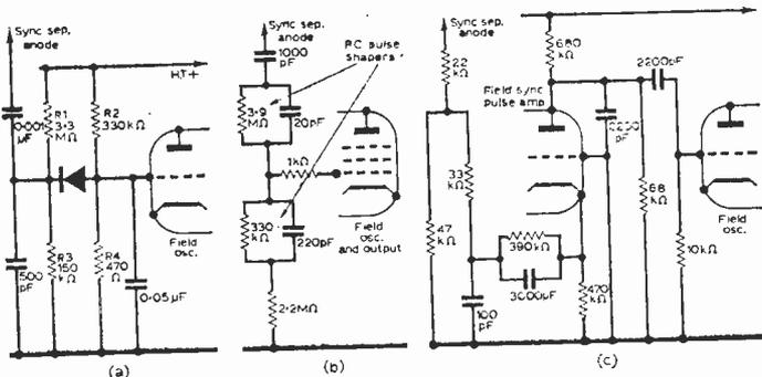
Fig. 6—Three completely contrasting field sync feed systems, (a) biased diode limiter (conducting when pulses exceed pre-determined value), (b) capacitive with two series RC pulse shaper circuits, (c) grounded-grid triode field pulse amplifier shaper.
