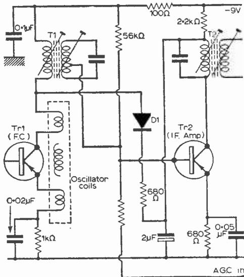
Fig. 3—Overload diode circuit as used in many Alba receivers. Normally Tr1 collector voltage exceeds Tr1 collector voltage so that D1 fails to conduct. However if a large positive-going a.g.c. voltage reduces Tr2 collector current sufficiently, Tr2 collector voltage will rise above that of Tr1 the diode will conduct and shunt the primary of Tr1 with its low forward resistance plus that of the 68-Ω series resistor. In this way, overloading on very strong signals is prevented.
