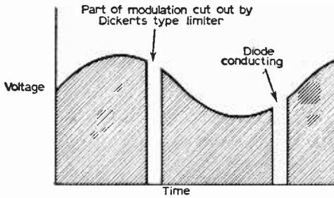
Fig. 2—Showing how part of modulation is cut out when the diode conducts.
