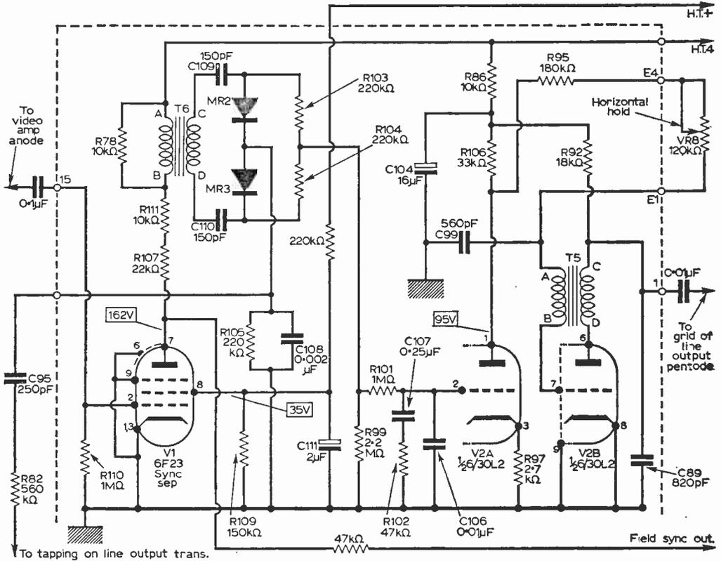
Fig. 4—Complete a.f.c. line oscillator circuit (Ekco-Ferranti) showing sync separator, discriminator, control voltage amplifier (V2A) and blocking oscillator (V2B). Control of V2B frequency is obtained by varying its grid potential by tying it to the anode of V2 instead of the h.t. rail. Sawtooth waveform sample is fed to the junction of the two diodes, with the control voltage taken from the junction of the twin 220kΩ resistors, a re-arrangement of the system shown in Fig. 1.
