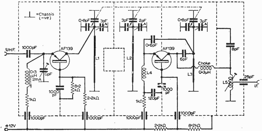
Fig. 2—Circuit diagram of a transistor u.h.f. tuner using quarter-wavelength lecher wires.
