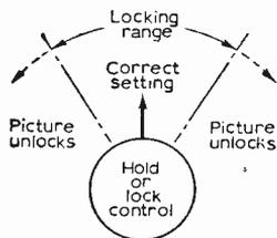
Fig. 15—The correct setting for the hold controls. Note that on dual-standard receivers there are separate lines for 405 lines and 625 lines.
