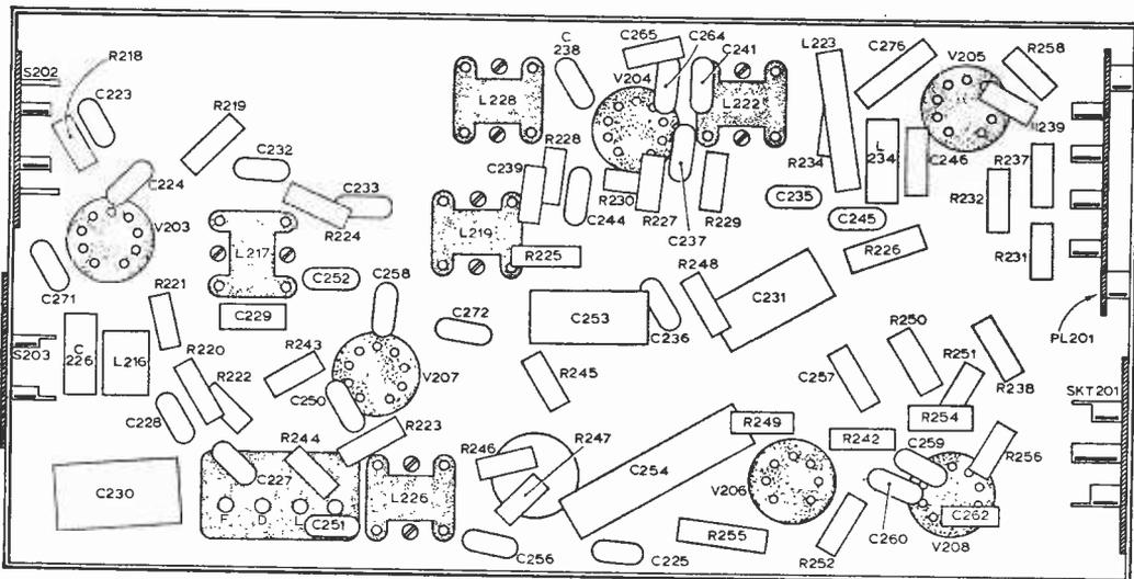
Fig. 6—Underchassis layout of sound receiver.
