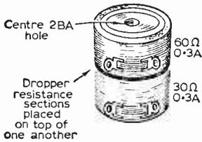
Fig. 2—Commercially made mains dropper sections (Radio Spares Ltd.).
