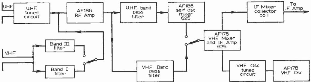
or Band III aerial filter circuit is selected, the output then feeding into the common r.f. amplifier (the presence of the u.h.f. input circuits here has no effect on the v.h.f. performance), then to the v.h.f. bandpass filter (which again is switched for Band I and III) and on to Tr3 which, on v.h.f. acts as a mixer.
