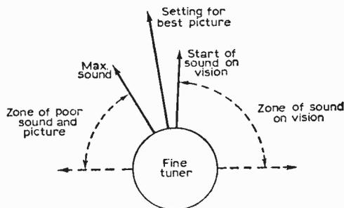
Fig. 14—This diagram shows the best setting for the fine tuning control.
