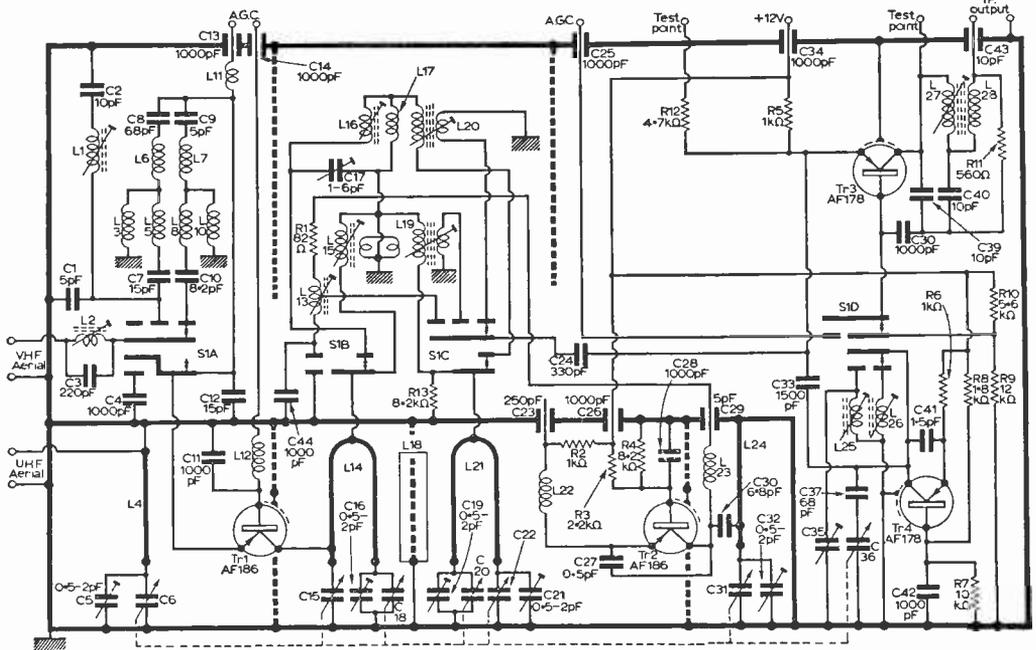
Fig. 3 (above)—Circuit diagram of the Pye "all-band" television tuner. This is fully described in the text.
