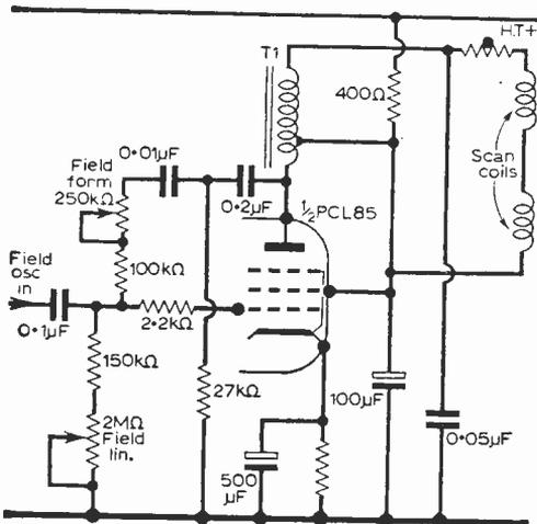
Fig. 3—Unusual field output circuit used in many Decca dual-standard receivers. Scan-coils are directly connected to auto-transformer T1 via thermistor, while  $400\Omega$  decoupling resistor feeds both anode and screen of pentode.
