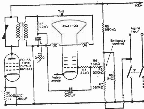
Fig. 4—Typical field flyback suppressor (GEC). On flyback a negative pulse developed across C2 is fed via C3 to the tube grid and blanks out the re-trace. Thermistor TH1 reduces in value as heat increases the resistance of the scan coil windings thus maintaining height. R7 is returned to the mains side of the mains switch to reduce duration of the "switch-off spot".
