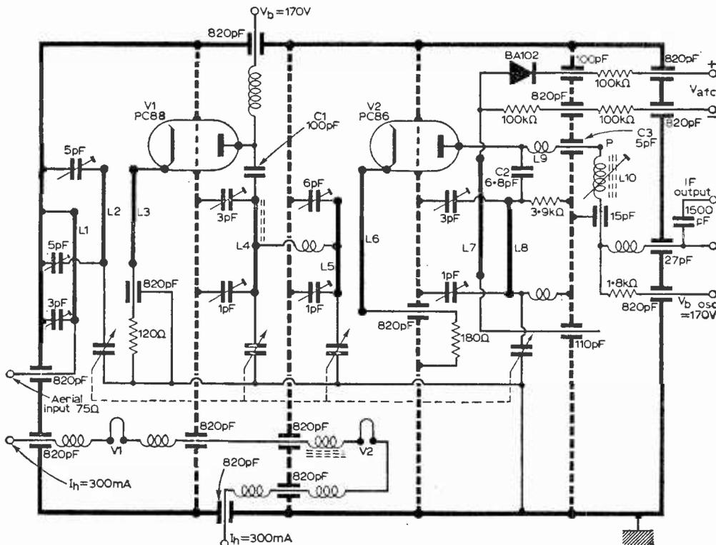
Fig. 1—Circuit diagram of Mullard u.h.f. tuner, using valves and half-wavelength lecher wires.
