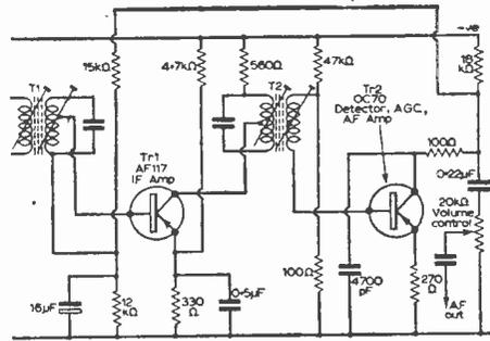
Fig. 4—STC (Regentone, KB, RGD) a.g.c. circuit. Biased to the point of max l. curvature, Tr2 performs signal rectification, a.f. amplification and also supplies a.g.c. control to i.f. amplifier Tr1. As increasing input decreases Tr2 collector voltage, Tr1 bias falls, thus reducing its emitter current and gain.
