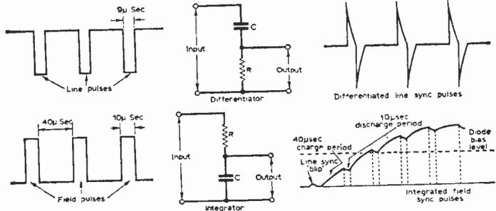
Fig. 5—Line sync pulses after differentiation have a good timebase triggering waveform. Field sync pulses after integration (essential for separation) have an inferior slowly rising front produced by the 40 $\mu$ Sec charge/10 $\mu$ Sec discharge 8 pulse train. The difficulties imposed by this waveform disparity are reflected in the more complex field sync supply systems shown in Fig. 6.
