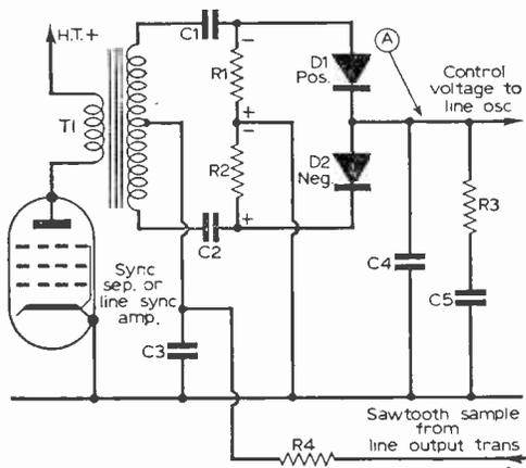
Fig. 1—Basic duo-diode discriminator circuit. T1 feeds equal but opposite polarity sync pulses to diodes D1 and D2, which develop identical value outputs across R1 and R2 but which results in a net zero output at (A).
