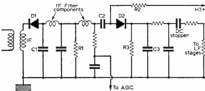
Fig. 3—Circuit containing a series limiter using germanium diodes.
