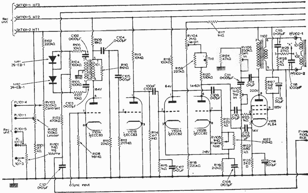
Fig. 5—Sync separator and field timebase circuits.
