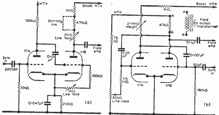
Fig. 2—The two types of field multi-vibrator circuits used in modern receivers, (a) using both capacitive and common cathode resistor coupling, (b) using purely capacitive coupling.
