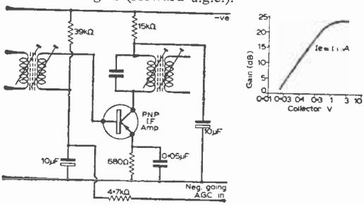
Fig. 1—Typical circuit for varying transistor gain by varying its emitter current as used in most modern receivers. The graph shows gain variation with  $I_e$  variation. With usual p-n-p. transistors, a.g.c. voltage must be positive-going. The slight negative voltage developed across R4-5 aids D1 rectifying action by giving it a slight forward bias.
