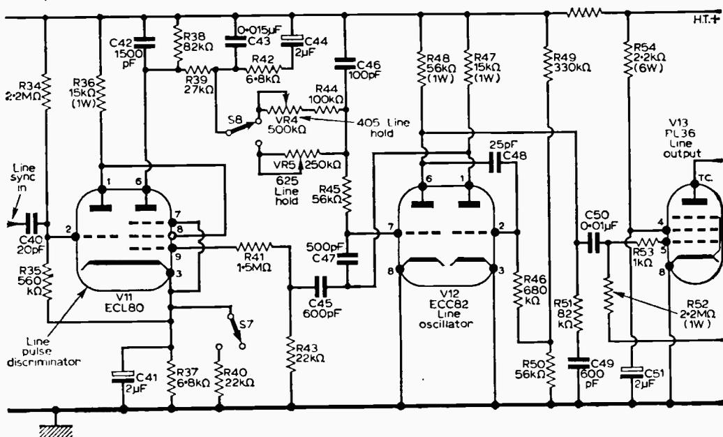
Fig. 2.—Typical line output stage (Decca) using duo-triode as line generator with PL36 line output pentode purely as power amplifier. Note cross-connected capacitors to ECC82 triodes.
