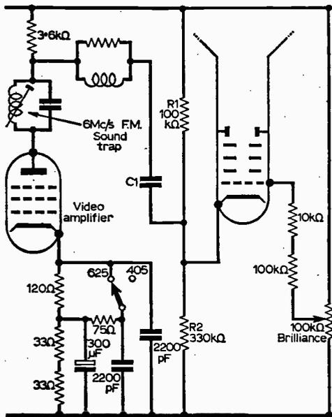
Fig. 4—"AC" tube feed as used in many dual-standard receivers. R1 and R2 form a fixed potential divider holding tube cathode at a predetermined voltage thus keeping brilliance level constant despite bias changes on 405/625 changeover.
