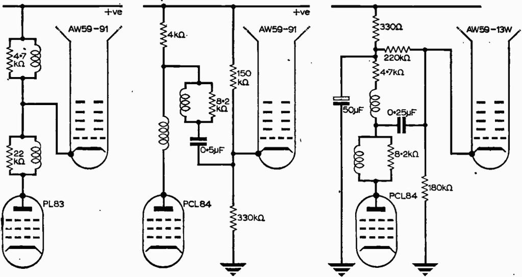
Fig. 6—Typical examples of the three types of resistive/inductive video loads. Left, parallel (Philips 23TG-122A) centre, series (Ferguson 850) right, combined series/parallel (Regentone VCI series).
