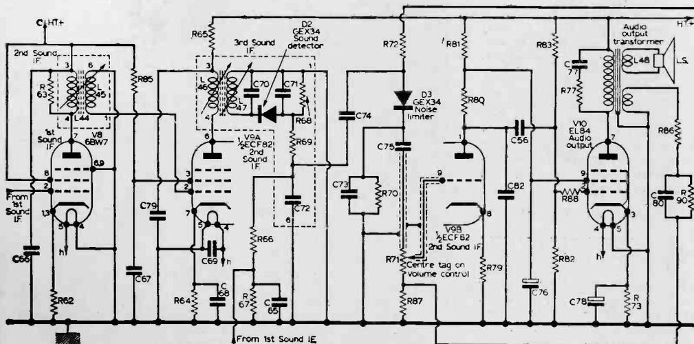
Fig. 1(a)—Sound i.f. and audio stages of the K-B NV40 and NV60 models, which are used as a basis for discussion in the text.
