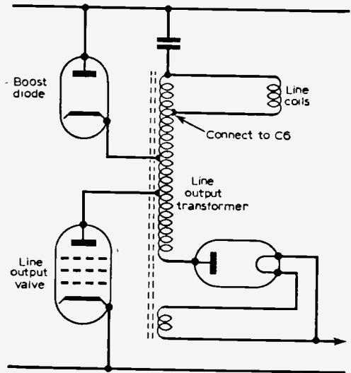
Fig. 9—Connection of Co.
