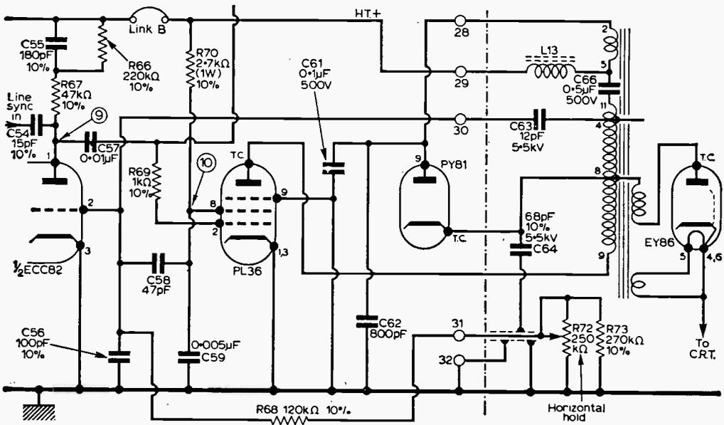
Fig. 1—Typical line output stage (Invicta 337) where line output pentode also acts as half multivibrator with ECC82 triode. Note h.w.v. capacitor from tapping on transformer to ECC82 grid for positive feedback.
