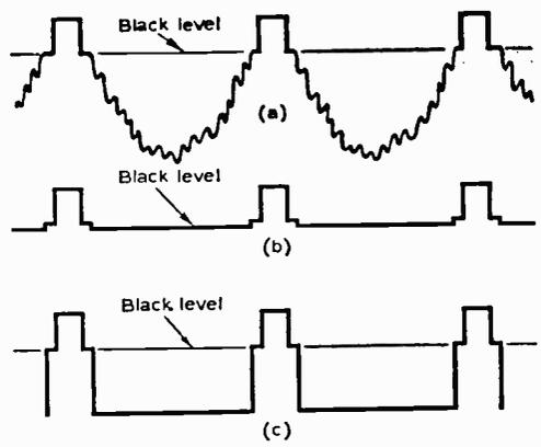
Fig. 2 (above) and 3 (top right)—(a) average picture, (b) black picture, (c) white picture. Note constant position of black level when effect of d.c. component is retained.
