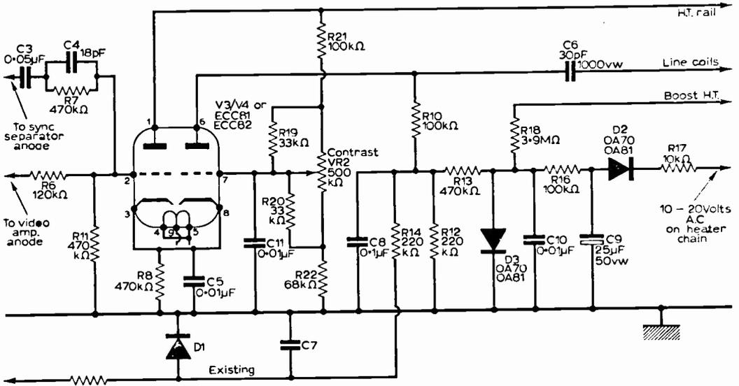
Fig. 7—Complete circuit diagram of the unit.
