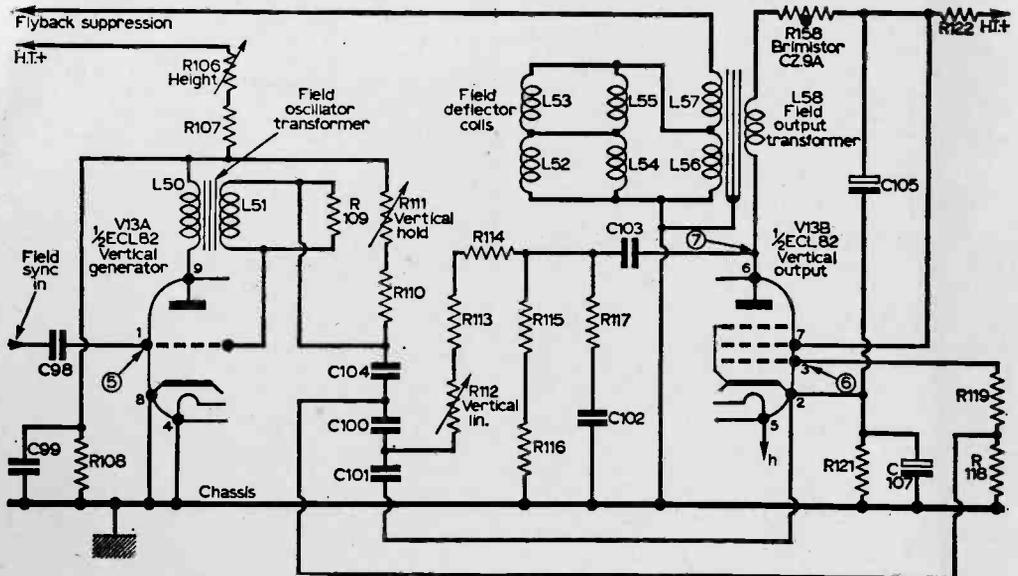
Fig. 2—Field timebase circuits of the K-B NV40/60.
