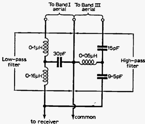
Fig. 13—Practical circuit, giving component values, of a diplexer.
