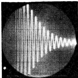
Fig. 9—Oscillogram of un-suppressed damped oscillation.
