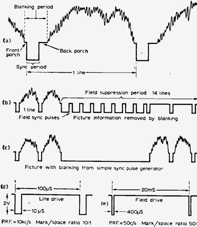
Fig. 2—Synchronising pulses required by all picture sources.
