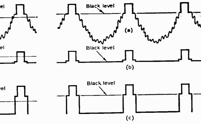
Fig. 4 (right)—(a) Low strength signal, (b) high strength signal, (c) low strength with base line redrawn, (d) high strength with base line redrawn.
