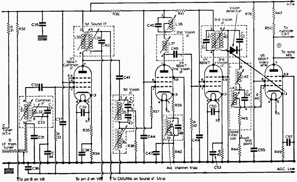
Fig. 1(b)—Common i.f. and video circuits of the K-B NV40/60
