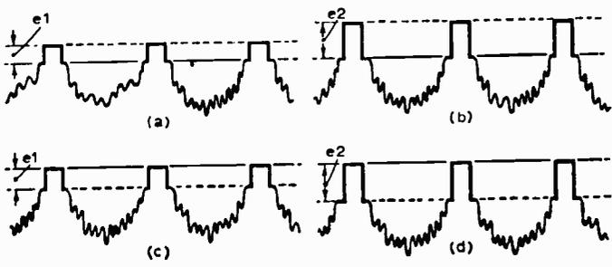
Fig. 4 (right)—(a) Low strength signal, (b) high strength signal, (c) low strength with base line redrawn, (d) high strength with base line redrawn.
