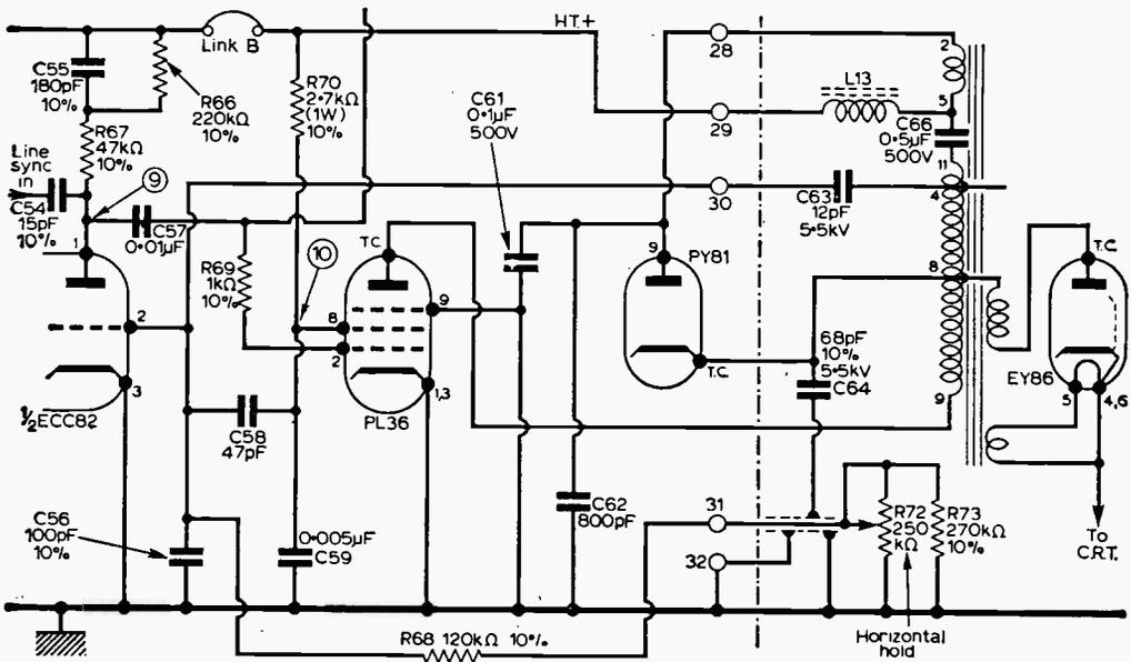
Fig. 1—Typical line output stage (Invicta 337) where line output pentode also acts as half multivibrator with ECC82 triode. Note h.v.v. capacitor from tapping on transformer to ECC82 grid for positive feedback.
