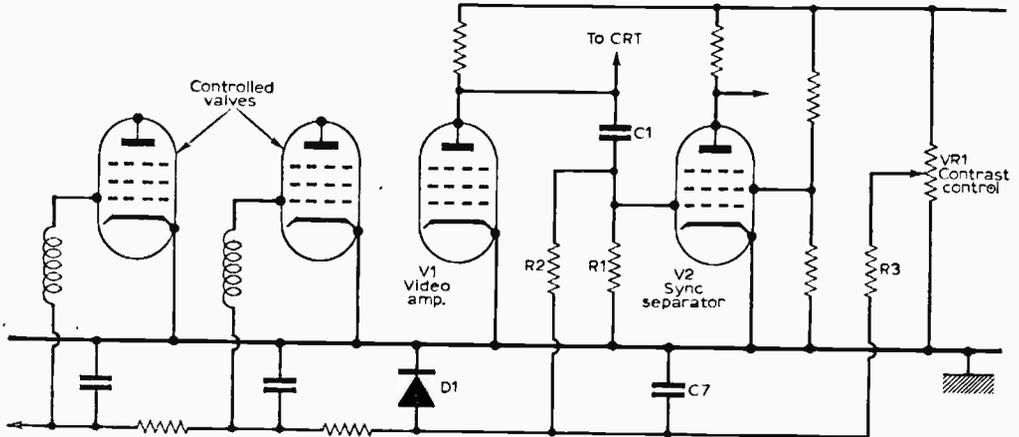
Fig. 1—Typical mean-level auto gain control circuit.
