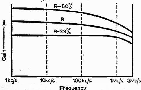
Fig. 1—Effect of increased and reduced values of load resistor on typical purely resistive video amplifier.
