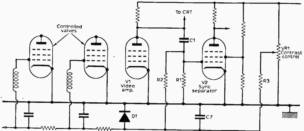
Fig. 1—Typical mean-level auto gain control circuit.
