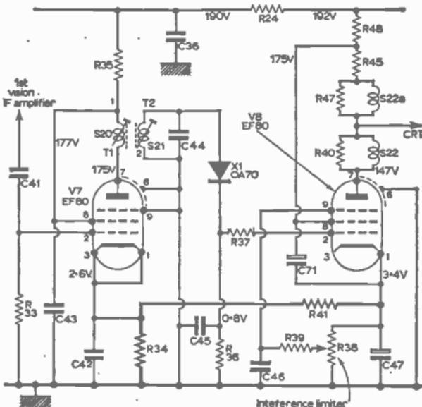
Fig. 2—Video biasing system used in many Philips models. Cathode bias resistor of second vision i.f. amplifier is common to video amplifier. As mean picture level rises so does video anode current and also voltage developed across common resistor to bias back the i.f. stage, giving a degree of a.g.c.
