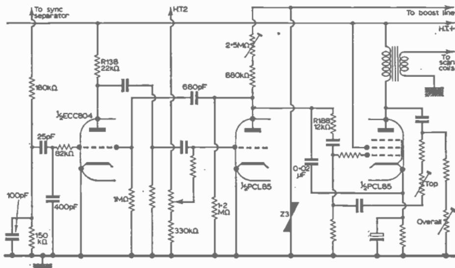
Fig. 3—Variation on the theme of Fig. 1, used in a wide range of Thorn receivers, under the Ferguson, Marconi, H.M.V and Ultra trade marks. Differences are discussed in the text.
