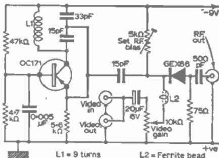
Fig. 6—Circuit of the r.f. modulator.
