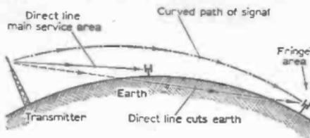
Fig. 19—Showing how the signal curves round the earth in the fringe area. This bending is influenced by the troposphere or earth's atmosphere, the conditions of which are affected by the local weather. Thus, fringe area reception can be disturbed by the weather conditions.
