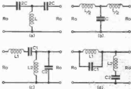
Fig. 15—(a) High-pass T-type filter. (b) Low-pass filter. (c) Band-pass filter. (d) Band-elimination filter.
