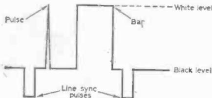
Fig. 1—Pulse and bar signal with line sync pulses.
