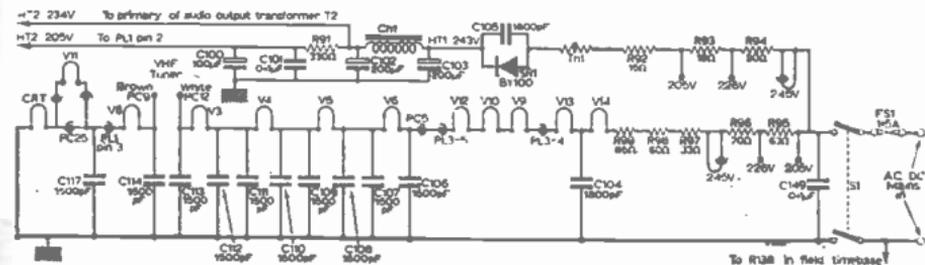
Fig. 4—Arrangement of heater and d.c. supplies.
