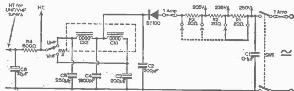
Fig. 1—H.T. smoothing and supply system used in Decca DR 101 to 606 range of receivers. Operation of system switch SW2 passes h.t. current through Ck1 on v.h.f. and Ck2 on u.h.f. These then magnetically pull over the multi-contact change-over switch to the appropriate position. R4 and C6 comprise additional smoothing for the v.h.f./u.h.f. tuners.
