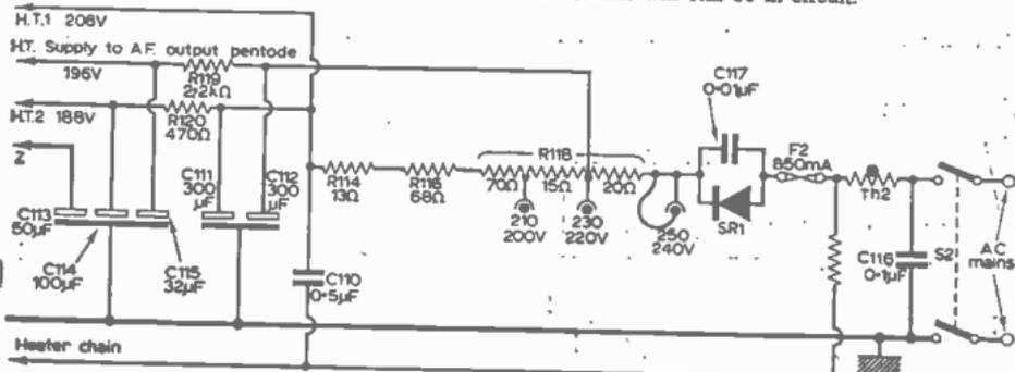
Fig. 3—Complex h.t. smoothing and supply system as used in many dual standard bush receivers. The 208V h.t. feed supplies the receiver strip while the lower voltage, but still further decoupled HT2 feed supplies the timebases and sync separator. C110 connected from the heater chain to HT1 supply feeds a small anti-phase a.c. voltage for residual hum cancellation.
