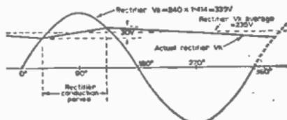
Fig. 5—An average dual-standard television receiver will require about 300 mA at 245V d.c., but as rectifier conduction occurs only during the positive half-cycle and then only when its anode voltage  $V_A$  exceeds its cathode voltage  $V_C$ , the d.c. feed to the reservoir capacitor takes the form of short heavy pulses during the brief conducting periods as indicated.
