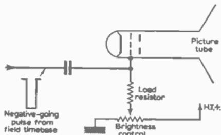
Fig. 16—Basic circuit of field flyback blanking.
