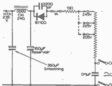
Fig. 4—Conventional h.t. smoothing filter as used in most current TV designs. (Example from KB, Regentone, RGD range). High value smoothing capacitor plus choke Ckt gives extremely low hum level with high output voltage.
