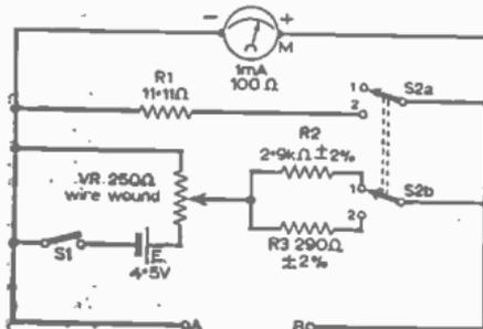
Fig. 2—Circuit of the author's ohmmeter. All component values are given on the circuit.
