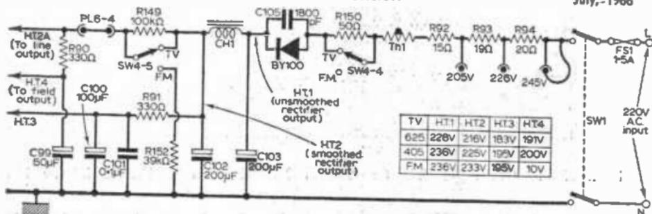
Fig. 2—Triple output h.t. smoothing and supply system used in many GEC/Sobell v.h.f./u.h.f./f.m. receivers. Note voltage variations on 625, 405 and f.m. and additional surge limiter in circuit on f.m. to reduce voltage.
