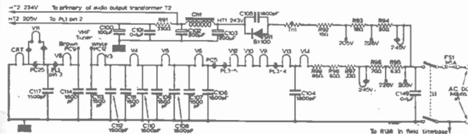
Fig. 4—Arrangement of heater and d.c. supplies.
