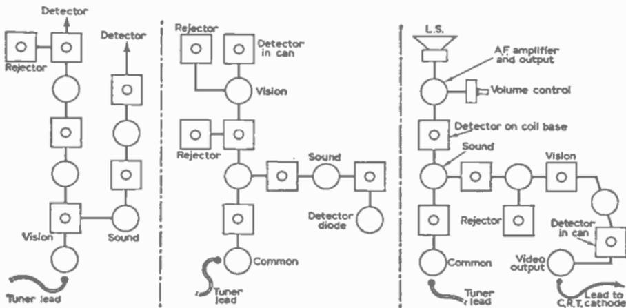
Fig. 1—Various i.f. layouts showing how sound and vision chains can be traced.
