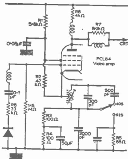
Fig. 1—Basic Ferguson dual-standard video amplifier. When R1 and R2 reduced in value thus increasing voltage drop across R3 and R4 and over-biased the video amplifier, symptoms were (a) practically zero sync lock, (b) low a.g.c. voltage, (c) i.f. overloading and (d) poor picture tonal gradation.
