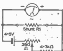
Fig. 4—Circuit for adjusting the shunt.
