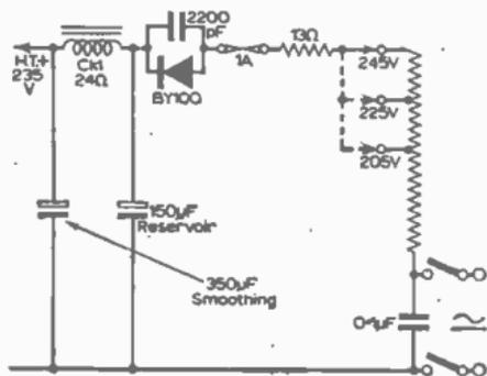
Fig. 4—Conventional h.t. smoothing filter as used in most current TV designs. (Example from KB, Regentone, RGD range). High value smoothing capacitor plus choke Ck1 gives extremely low hum level with high output voltage.
