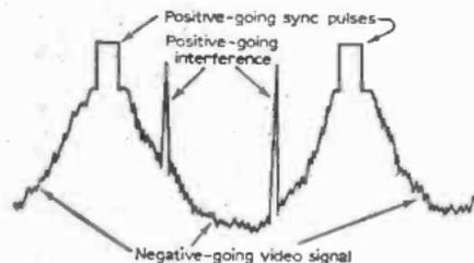
Fig. 17—Showing how interference pulses rise of a 625-line picture waveform.
