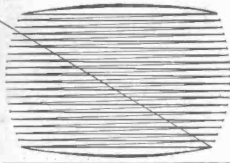
up with the control at one of its stops. Rotating the other way will only worsen the effect. Fig. 3 indicates that the line timebase is running too slowly, while Fig. 4 indicates fast running. These are indicated by the slight diagonal tilt to the left and the right of the screen respectively.
