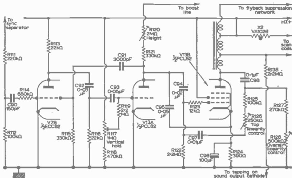
Fig. 1—Typical field oscillator and output circuit, as used by several models in the Ferguson range.
