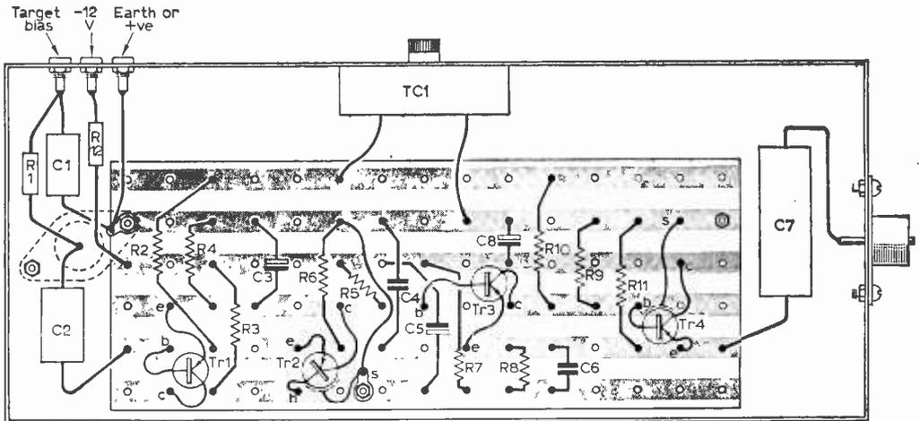
Fig. 17—Veroboard layout of the head amplifier.
