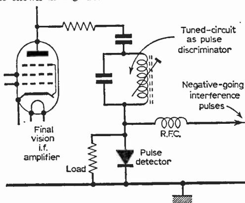
Fig. 26—Showing how the triggering interference pulses for the heptode circuit in Fig. 25 may be obtained from a tuned circuit discriminator and pulse detector, fed from the final vision i.f. amplifier anode circuit.
