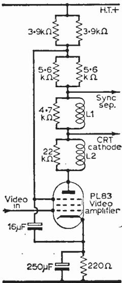
Fig. 3—Integral anode load and screen supply circuit as used in many Philips receivers to provide high-gain, linear amplification from d.c. to 6 Mc/s. Peaking coils are used to boost the h.f. response and selective negative feedback to reduce amplification at the low frequencies.
