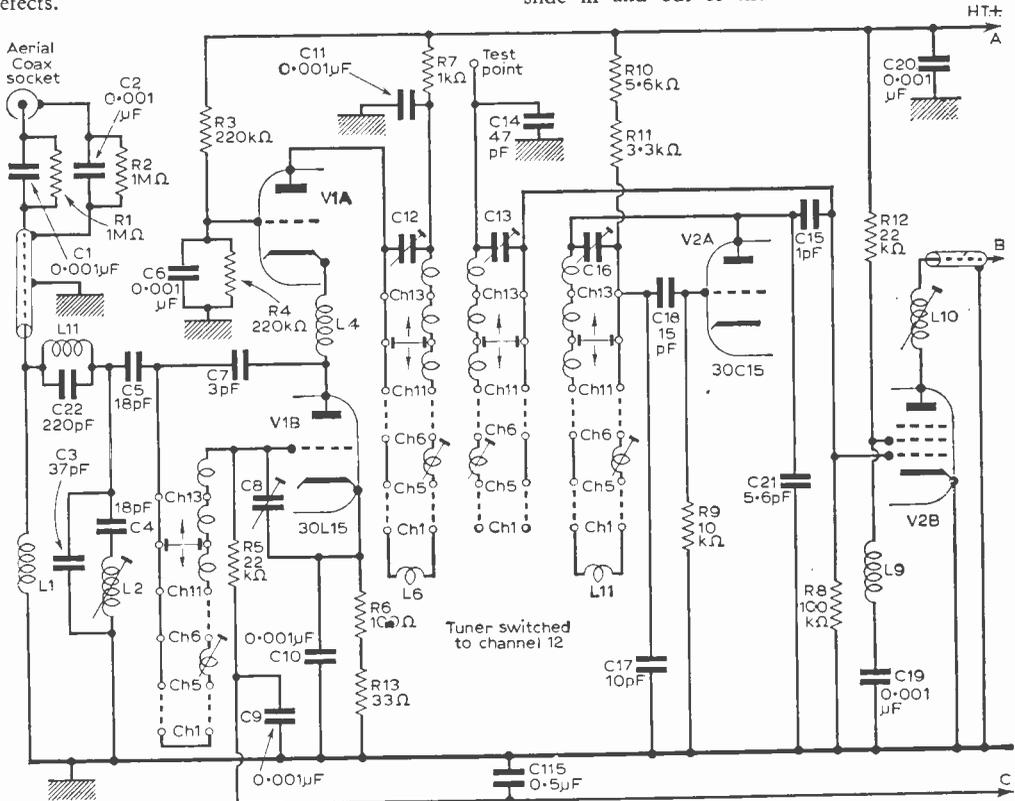
Fig. 1—Circuit of the r.f. tuner unit.
