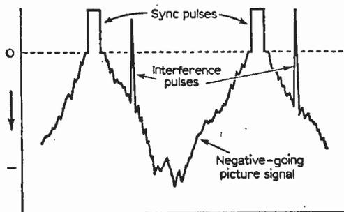
Fig. 24—Showing how pulses of interference appear on the video waveform and rise in the same direction as the sync pulses on 625-line signals with negative-going picture modulation.
