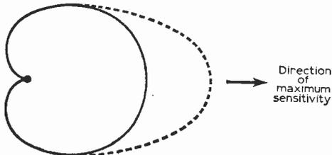
Fig. 22—A heart-shaped polar diagram. The broken-line shows emphasis due to directors in addition to a reflector on an aerial system.
