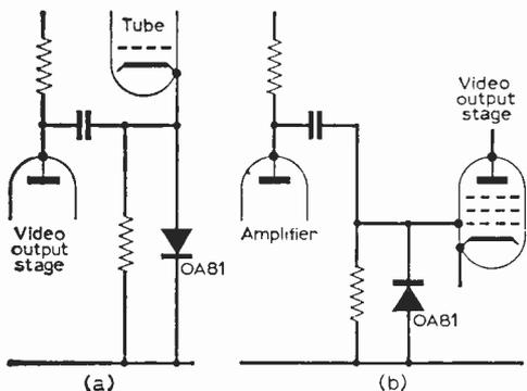
Fig. 11(a)—D.C. restoration at the c.r.t. cathode and 11(b) grid of the video detector.
