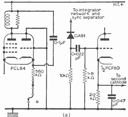
Fig. 4a (above)—Conversion of vision interference limiter triode to diode for frame sync coupling, as in (b), below.
