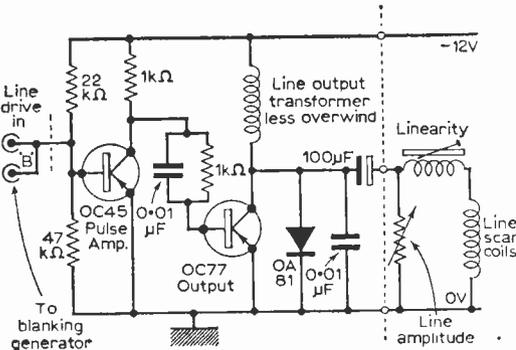
Fig. 14—The line scan circuit.
