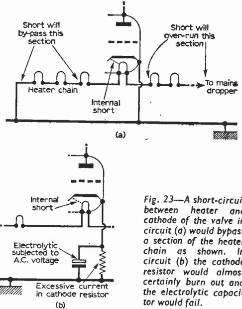
Fig. 23—A short-circuit between heater and cathode of the valve in circuit (a) would bypass a section of the heater chain as shown. In circuit (b) the cathode resistor would almost certainly burn out and the electrolytic capacitor would fail.
