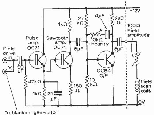
Fig. 15—The field scan circuit.
