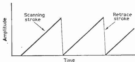
Fig. 1—A perfect, text-book sawtooth waveform on which the scanning and retrace strokes are identified.
