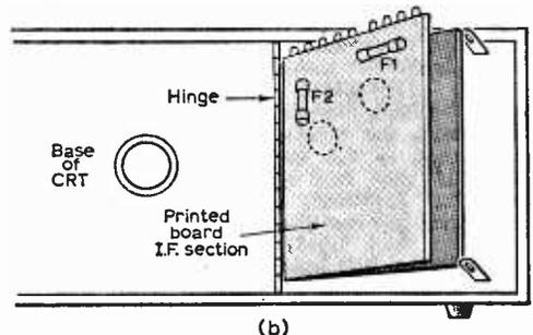
Fig. 5—Separation of h.t. lines can produce confusing symptoms. H.T. supply circuit used in many Philips models is shown (a), with physical position of fuses (b).
