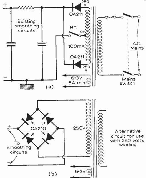
Fig. 12(a)—Power supply for parallel heater and 12(b) alternative cct.
