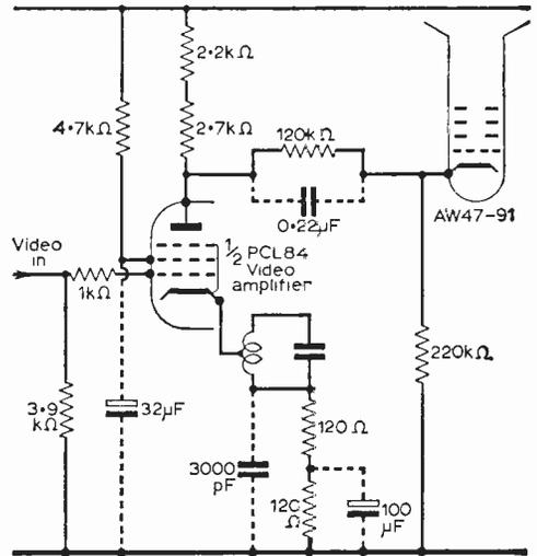
Fig. 4—The components shown connected by dotted leads will reduce the effect of negative feedback at the medium and high frequencies and thus increase gain in the upper part of the spectrum. The circuit shown is used in the Sobell ST196 receiver.
