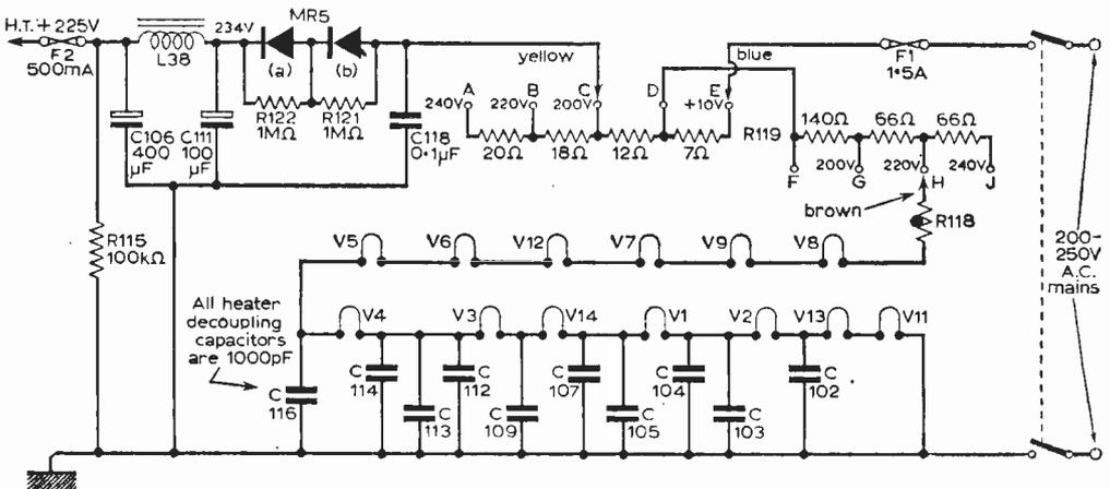
Fig. 2—The power supply and heater chain.
