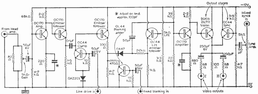
Fig. 18—Circuit of the processing amplifier.
