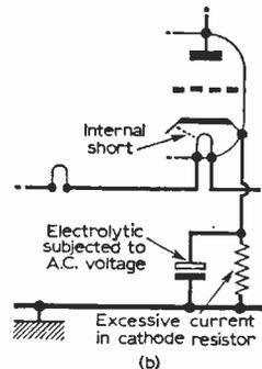
Fig. 23—A short-circuit between heater and cathode of the valve in circuit (a) would bypass a section of the heater chain as shown. In circuit (b) the cathode resistor would almost certainly burn out and the electrolytic capacitor would fail.
