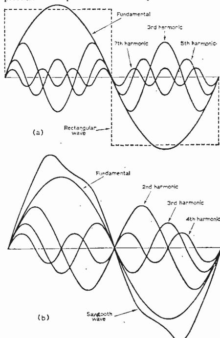
Fig. 21—Showing at (a) how a rectangular wave is produced by the addition of odd harmonics and (b) the formation of a triangular or sawtooth wave by the addition of both odd and even harmonics.
