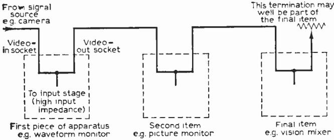
Fig. 10—Showing method of “linking” the coaxial cable between units. Note that cable terminated at one end only.
