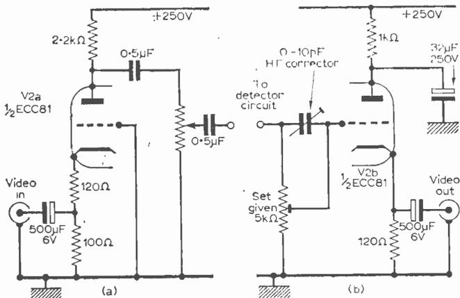
Fig. 9(a) Earthed grid amplifier and 9(b) Cathode follower.
