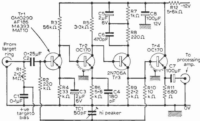
Fig. 16—The head amplifier circuit.
