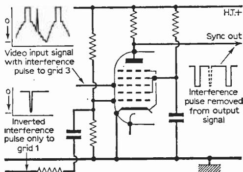
Fig. 25—Basic circuit of the heptode interference-cancelling sync separator.
