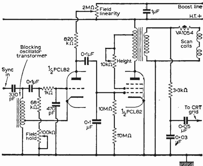
Fig. 6—Typical Pye circuit, as used in Invicta 538. Note anode feed to oscillator triode, use of variable pentode screen voltage to control height, and varistor in scan coil circuit.
