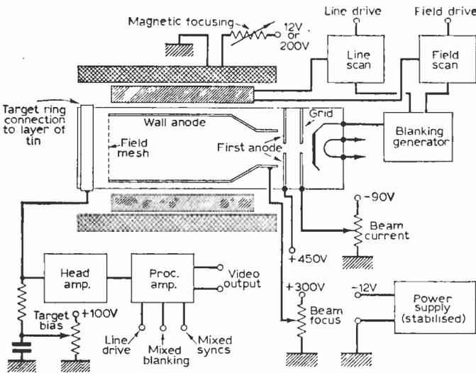
Fig. 13—The vidicon camera tube and associated circuitry.
