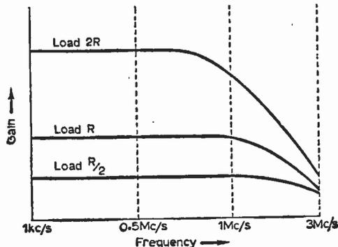
Fig. 1—This graph shows how the overall response of a video stage can be changed by varying the value of the resistive loads.
