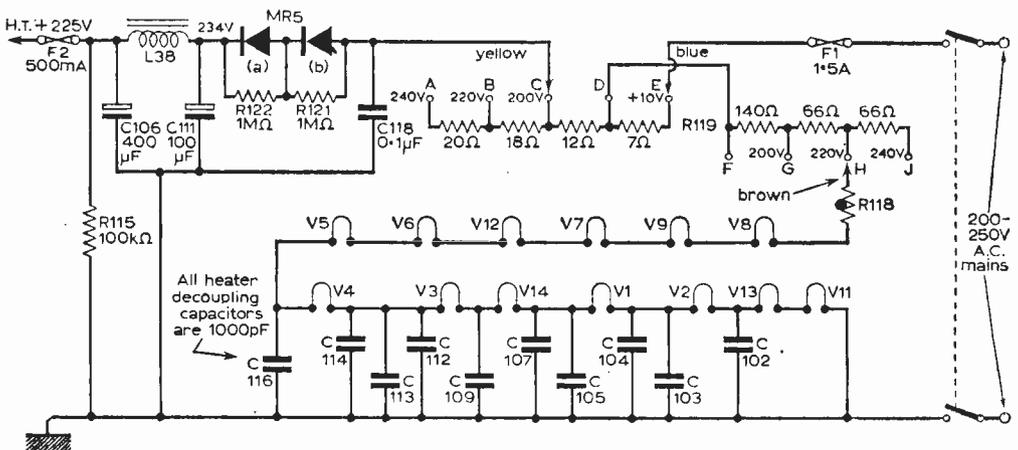
Fig. 2—The power supply and heater chain.
