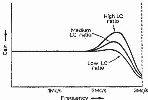
Fig. 2—Additional inductance tuned to resonate with the stray circuit capacitance can be used to peak the h.f. end of the band.
