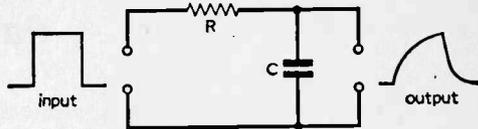
Fig. 27—Simple integrator circuit.
