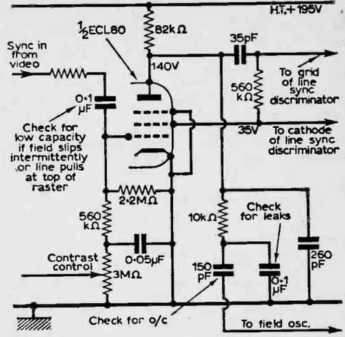
Fig. 18—Unusual regulation method for G2 voltage employed by Decca in the DM35 range.
