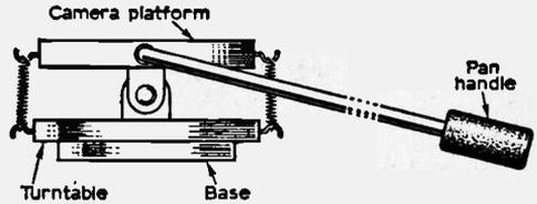
Fig. 27—Pan and tilt head assembly.
