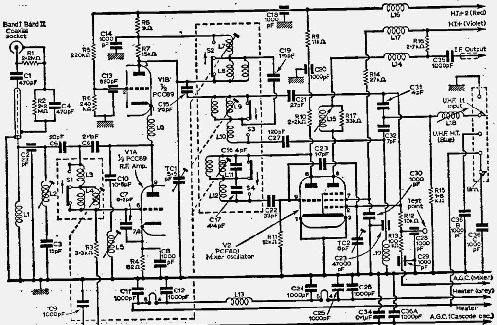
Fig. 1—The dual-standard tuner unit.
