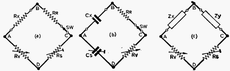
Fig. 2—The three forms of bridge used in this instrument circuit. 'a' is for resistance 'b' for capacitance and 'c' gives the ratio between two external impedances.
