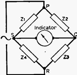
Fig. 1—Basic a.c. bridge circuit.
