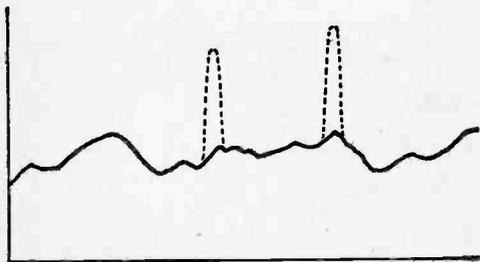
Fig. 3—Typical a.f. waveform with two random noise pulses superimposed.
