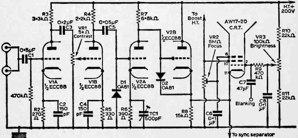
Fig. 26—Video amplifier and connections for the AW17-20 c.r.t.
