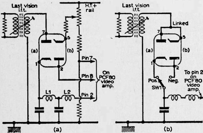
Fig. 1—Switchable diode detector (valves).
