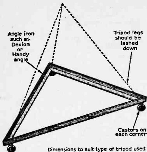
Fig. 28—'Skid' for use with a tripod.
