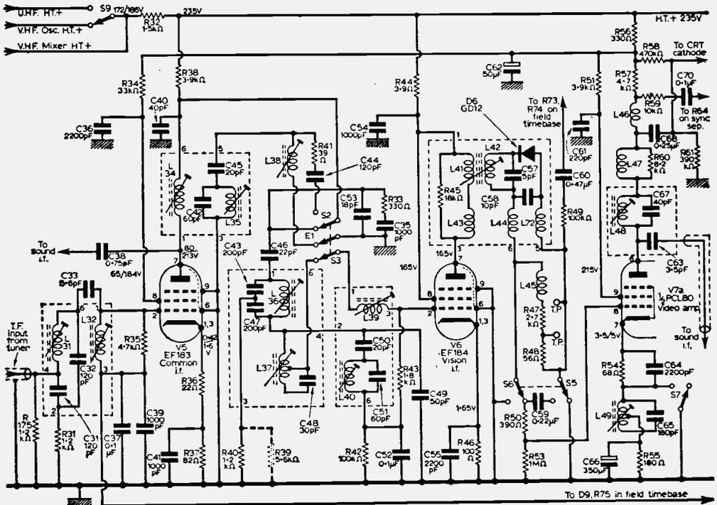
Fig. 3—Circuit of the i.f. unit.
