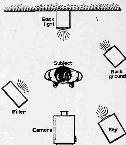
Fig. 29—Layout of studio lamps and cameras.
