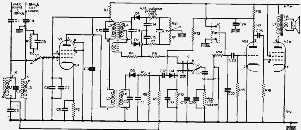
Fig. 1—Circuit diagram of the 405/625 sound system used in the STC VC2 range of receivers.
