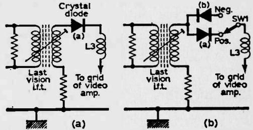
Fig. 2—Switchable diode detector (diodes).
