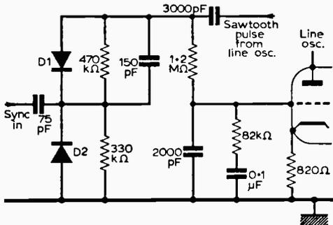
Fig. 15—Basic STC discriminator circuit used in many different models.
