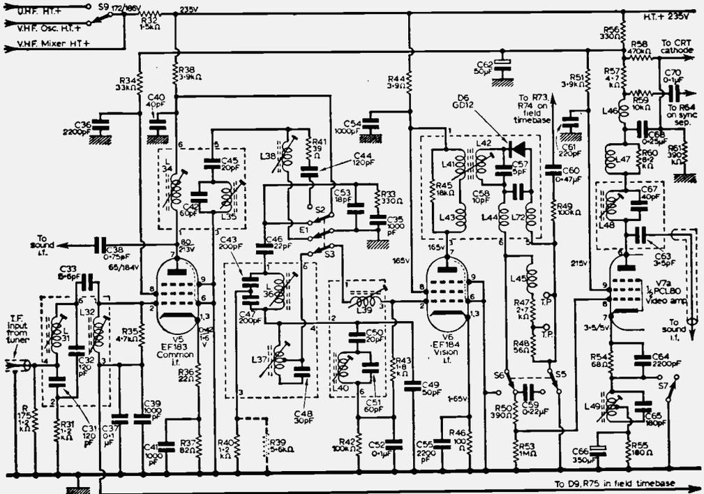
Fig. 3—Circuit of the i.f. unit.
