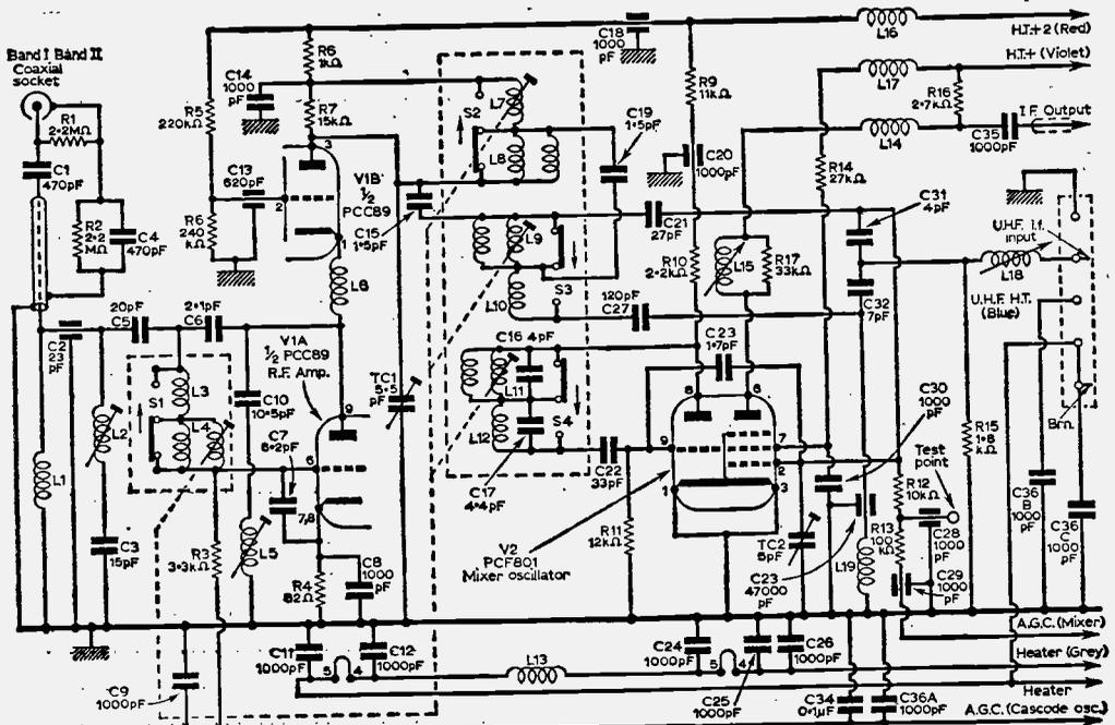
Fig. 1—The dual-standard tuner unit.
