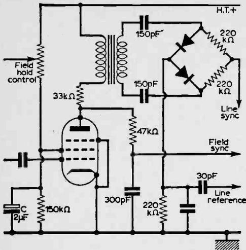
Fig. 17—Sync separator stage of Ekco T344F, using a 6F23 pentode.
