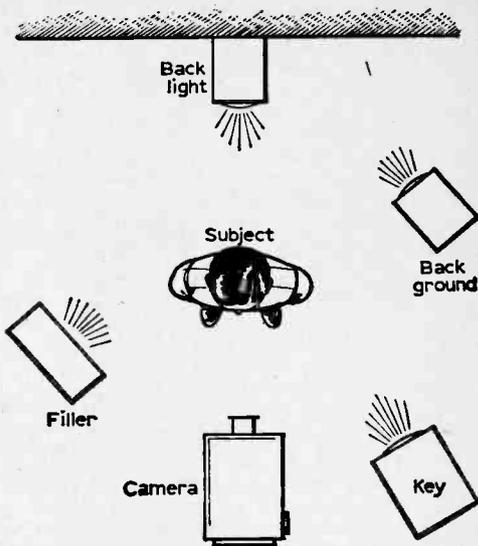
Fig. 29—Layout of studio lamps and cameras.
