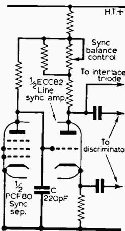
Fig. 19—Deceptively simple sync separator stage of Pye 17 and 21 groups of receivers with direct coupling from sync separator anode to line sync amplifier grid.
