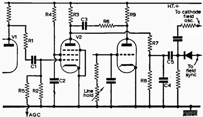
Fig. 13—Skeleton circuit of typical synchronising separator stage.
