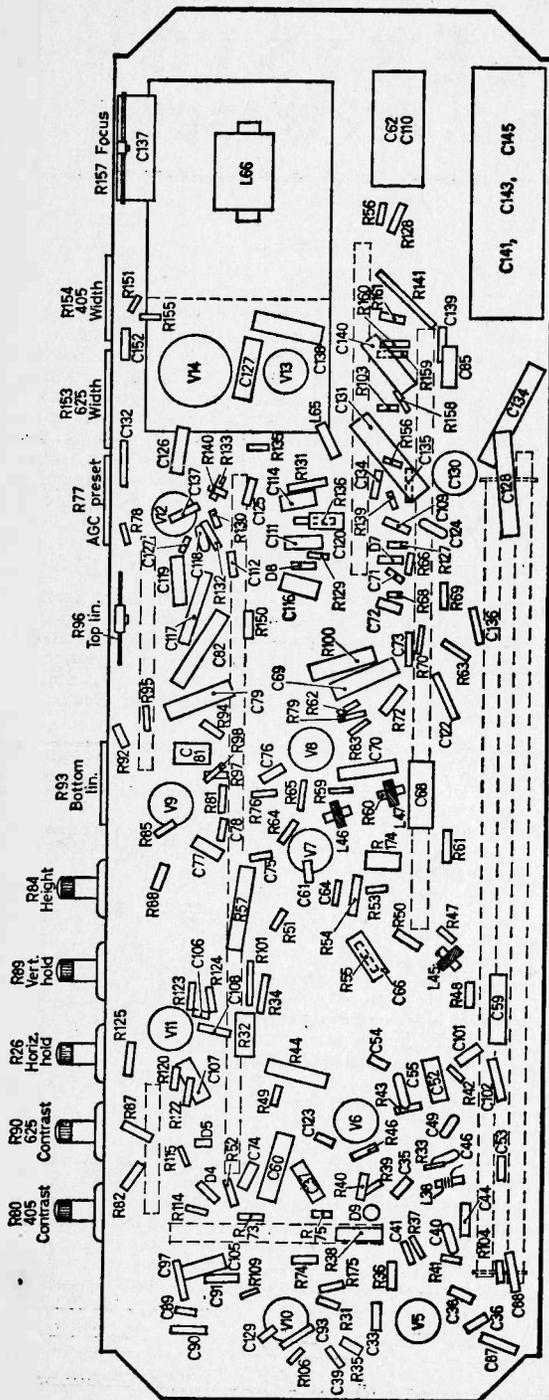
Fig. 2—Under-chassis view showing layout of components.
