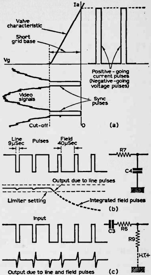
Fig. 14—What happens to the waveforms. (a) the composite signal is applied to a short grid base stage so that sync pulses cause conduction while video information cuts the valve off (positive-going sync negative-going video). (b) longer field pulses are integrated to form one larger pulse and limiter setting renders smaller line pulses ineffective. (c) passing the total sync signal through a differentiating circuit produces short steep pulses at leading and trailing edges.
