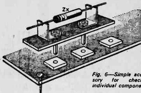
Fig. 6—Simple accessory for checking individual components.
