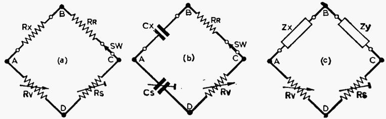
Fig. 2—The three forms of bridge used in this instrument circuit. 'a' is for resistance 'b' for capacitance and 'c' gives the ratio between two external impedances.
