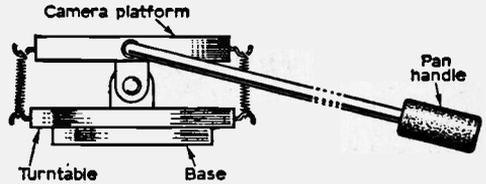
Fig. 27—Pan and tilt head assembly.
