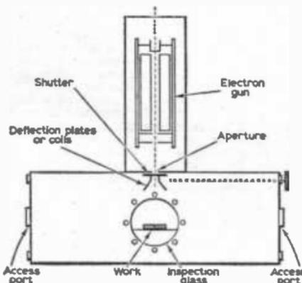
◀Fig. 1—Schematic diagram of an electron beam welder.
