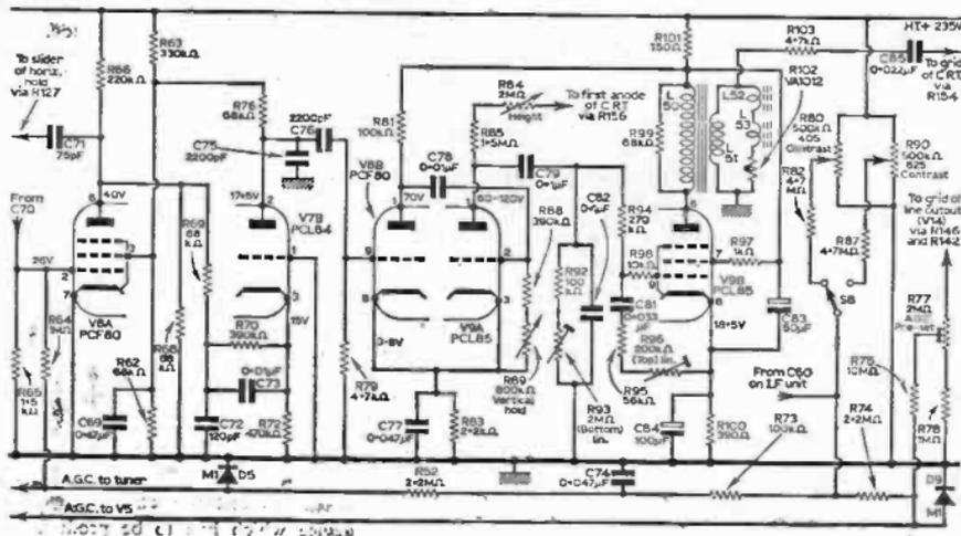
Fig 4—Field oscillator and output circuits.
