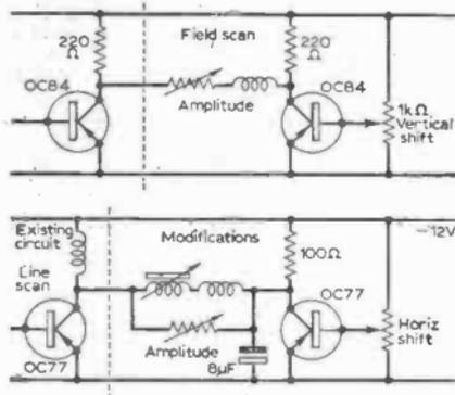
Fig. 33—Modifications to scan chassis to move shift control.
