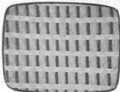
Fig. 10—An example of one of the numerous interlace patterns which will lock rigid upon slight misplacement of VR3. (Useful for checking geometry faults.)
