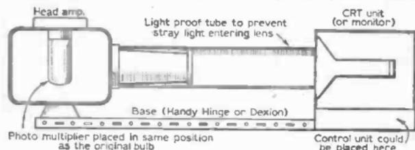
Fig. 30—Layout of flying spot scanner.
