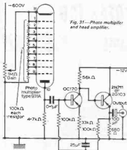
Fig. 31—Photo multiplier and head amplifier.
