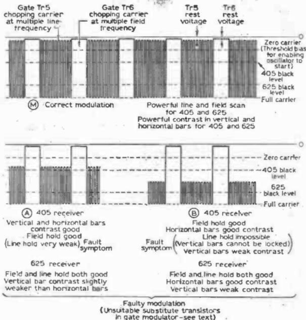
Fig. 3—Pattern modulator principles (waveforms at the slider of VR1).
