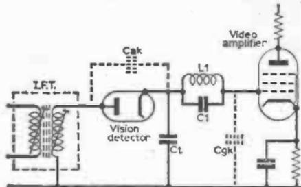
Fig. 4—The importance of small capacitances in the television detector stage. Due to C<sub>ak</sub> being comparable with C<sub>t</sub> a large i.f. content is present in the rectified signal. On 405, filter choke L1 is often designed to tune with C<sub>1</sub> as a rejector to the i.f. frequency and with the input capacity C<sub>gk1</sub> of the video pentode at 2.5-3Mc/s to boost top end response.
