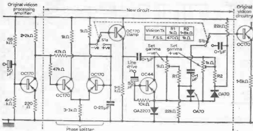
Fig. 34—Modifications to vidicon processing amplifier for use with TK screens.
