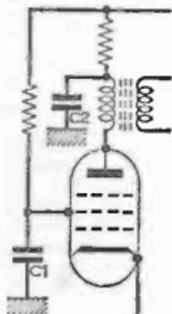
decoupling capacitors is illustrated in Fig. 5. The snag with substituting a capacitor in the normal way is that if it is held across the suspected one by hand, the presence of the hand might actually introduce instability. If a new capacitor is soldered in as a check, the long wires could also cause instability; and if the wires are cut to size, then the capacitor may be useless for further use because the wires are too short.
