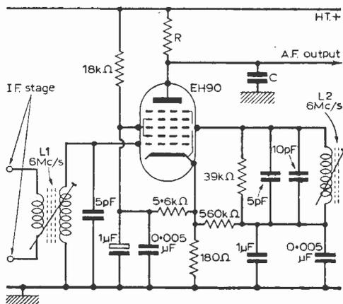
Fig. 1: Basic EH90 'Locked Oscillator' f.m. discriminator. Space charge coupling between G1 and G3 induces a replica of the input frequency on the latter but lagging by 90°. F.M. variations of the input signal then produce slight variations of this phase disparity to produce an a.f. signal across the anode load resistor.
