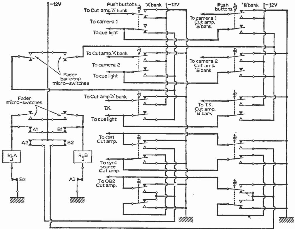
Fig. 55: A/B mixer d.c. switching.
