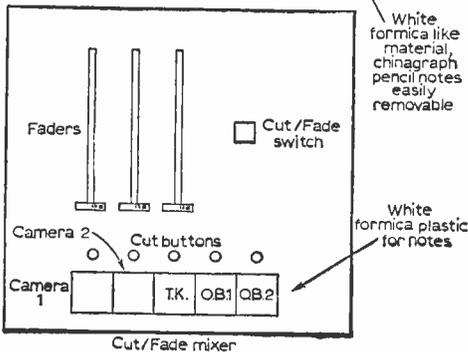
Fig. 58: Layout of mixer control panels.
