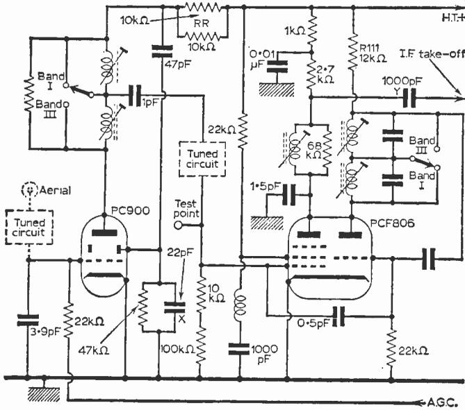
Fig. 43: Permeability tuner for Bands I and III.
