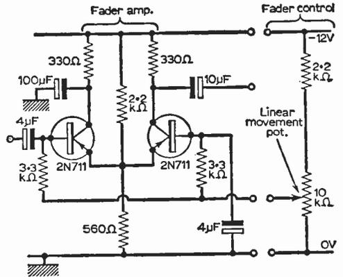
Fig. 53: Circuit of the fader amplifier.
