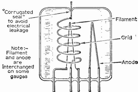
Fig. 1: Electrode structure of an ion gauge.
