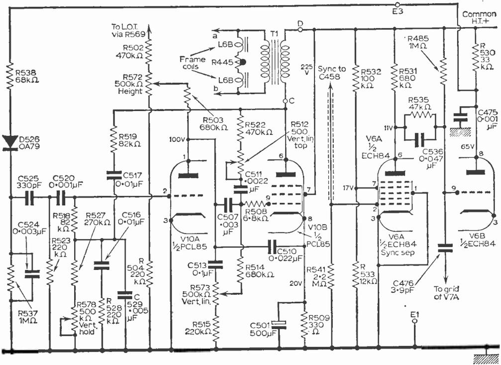
Fig. 6 (above): Field timebase circuitry.
