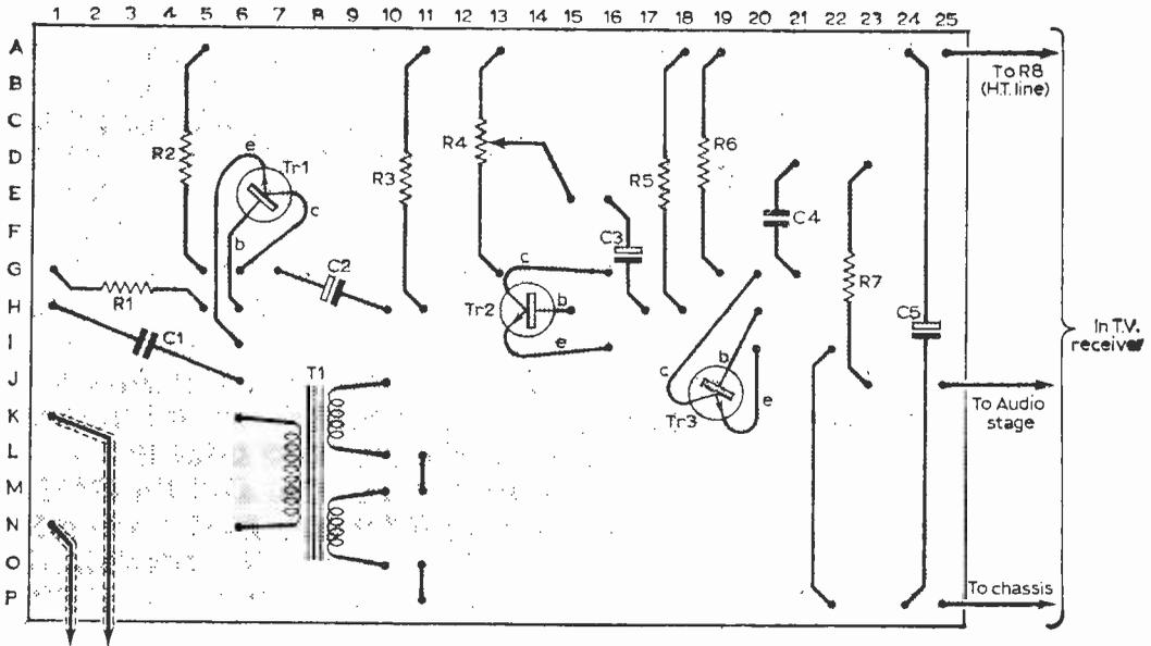
Fig. 3: Suggested component layout of the standard circuit using Veroboard
