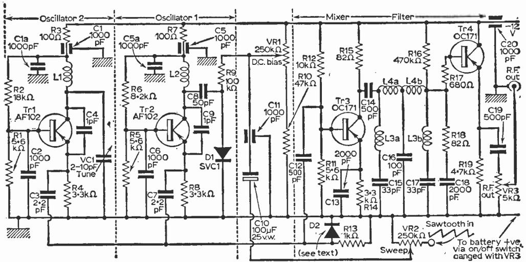
Fig. 2: Complete circuit diagram of the wide range wobblator.
