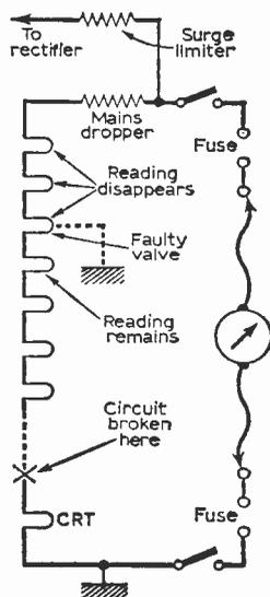
Fig. 1: Testing for heater/cathode leaks with an ohmmeter.
