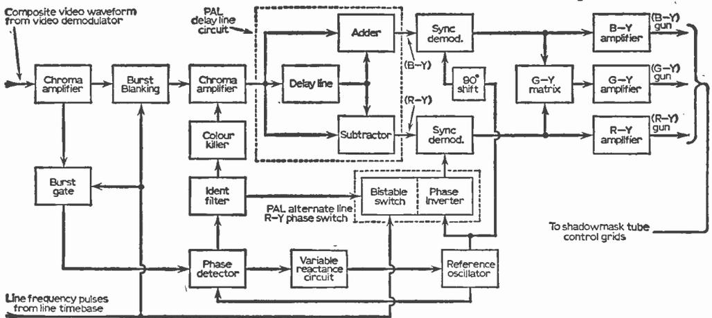
Fig. 1: Block schematic diagram of the essential features of a PAL decoder.
