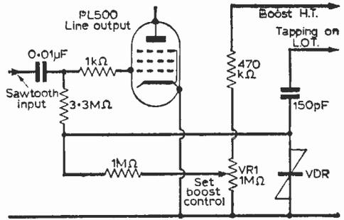
Fig. 3: GEC/Sobell/McMichael width stabilisation system. Correct picture width is obtained by setting VR1 "Set Booster Control" to give boost rail voltage of between 750-790V with full raster scan.
