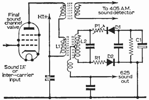
Fig. 6: Intercarrier buzz can often be reduced by carefully balancing the i.m. ratio detector by adjustment of P1.
