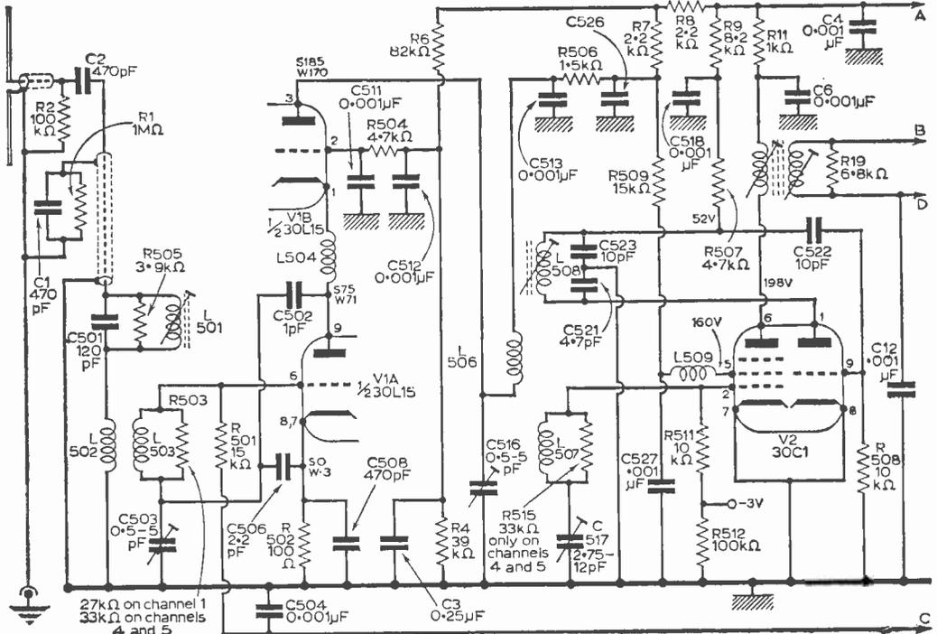
Fig. 1: Tuner circuit of the V470.
