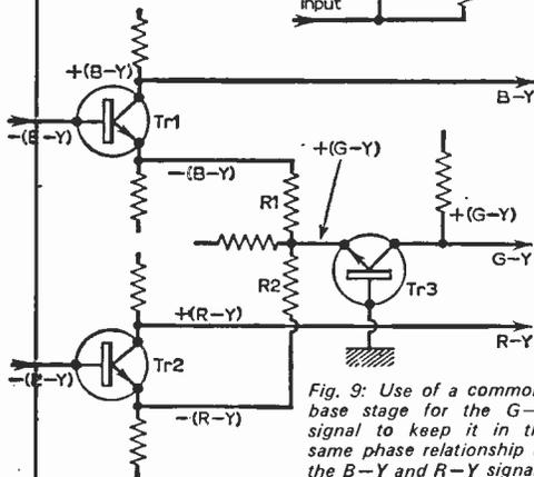
Fig. 9: Use of a common-base stage for the G-Y signal to keep it in the same phase relationship as the B-Y and R-Y signals.
