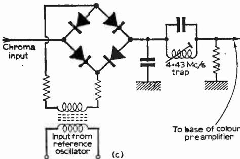
Fig. 7c: Semiconductor bridge demodulator.
