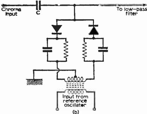
Fig. 7b: Synchronous demodulator using two diodes.
