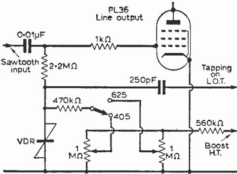
Fig. 2: Width stabilisation circuit used in many Dynatron models incorporating separate width setting potentiometers for both systems.
