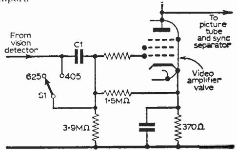
Fig. 4: Grid current in the video amplifier valve can affect the picture locking on 625-lines owing to the a.c. coupling on this standard. The relatively low grid impedance on 405-lines, due to the d.c. coupling on this standard, can often mask grid current effects (see text).
