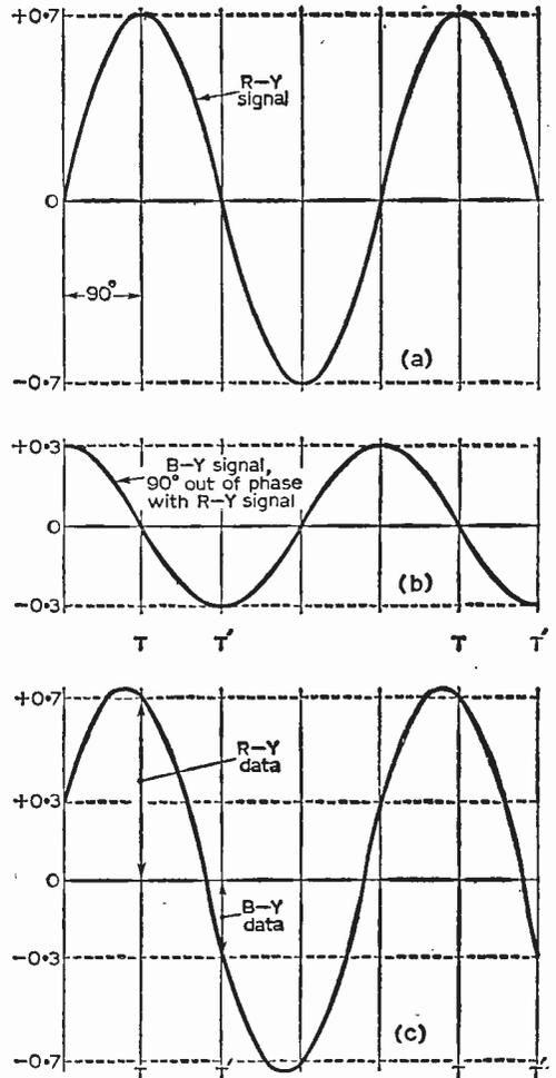
Fig. 6: The principle of synchronous demodulation.
