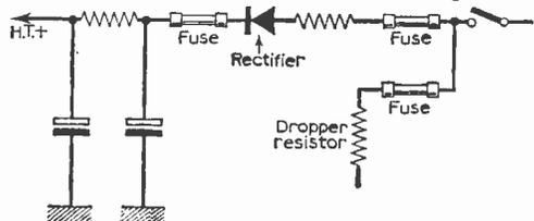
Fig. 2: Adding extra fuses is a useful way of locating a faulty section of circuitry.
