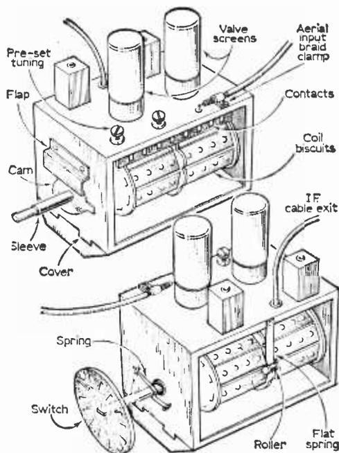
Fig. 48: Two views of old-type turret tuner, showing the trouble spots discussed in the accompanying text.
