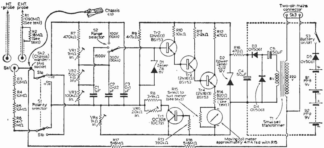
Fig. 1: Theoretical circuit diagram of the transistorized e.h.t. meter.
