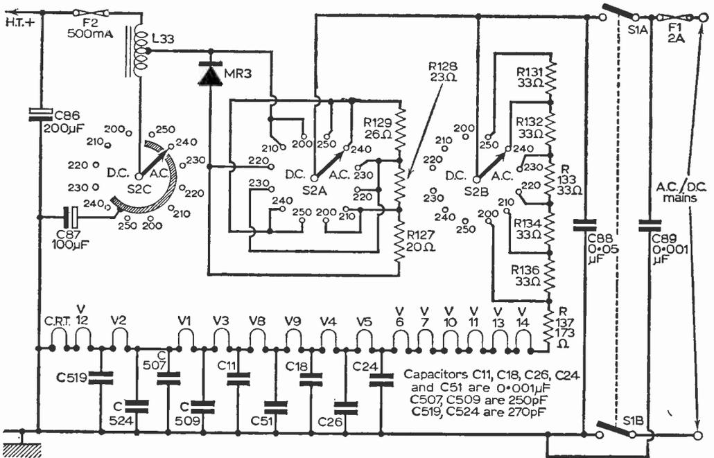
Fig. 3: Power supply circuitry for the V470 chassis.
