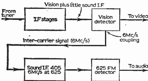
Fig. 5: The intercarrier technique employed in dual-standard sets in the 625-line condition.
