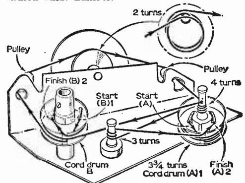
Fig. 50: An example of the fine tuner system employed for u.h.f. tuning. Exact routing of cord and freedom of pulleys is very important to avoid backlash and tuning drift.
