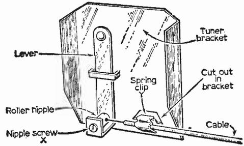
Fig. 49: System switches are often cable-operated. In some types it is important that the removal of the cable is by unhooking the clamp and releasing the nipple, but not loosening the retaining screw.
