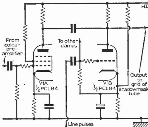
Fig. 10: Pentode colour output stage with triode clamp to clamp the output during the line flyback period to the correct zero value.
