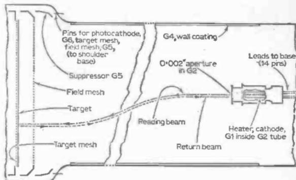
Fig. 2: The scanning section of the image orthicon.
