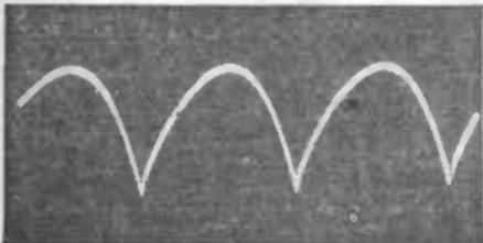
Fig. 4: This parabolic waveform is developed at the cathode of the field output valve and is used for linearity correction and for dynamic convergence in colour sets.
