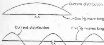
Fig. 1: Method of working of multiple  $\frac{1}{2}$ -wave aerial.
