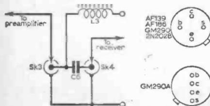
Fig. 4: Addition for line powering and key to transistor bases
