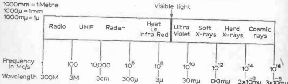
Fig. 1: Spectrum of electromagnetic waves; light waves fall between the heat and ultra-violet bands.
