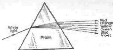
Fig. 2: A simple method of breaking up white light into its different wavelengths (different colours) is to use a prism.
