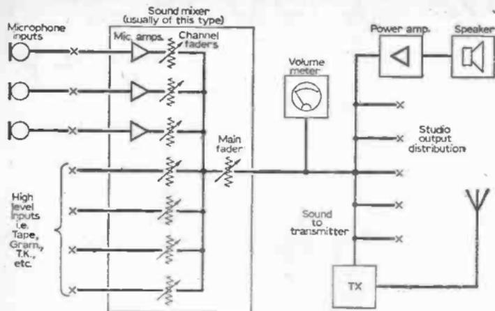
Fig. 70: Layout of the general sound system. The power amplifier and loud-speaker are used for monitoring.
