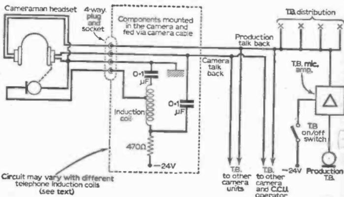
Fig. 71: Talkback schematic diagram. Production T.B. will be heard in left ear-ice. camera control in right.
