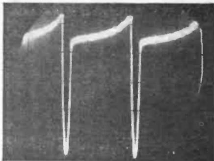
Fig. 5: The waveform at the line output stage when the Y lead is closely coupled to the insulation of the lead to the anode of the line output valve.
