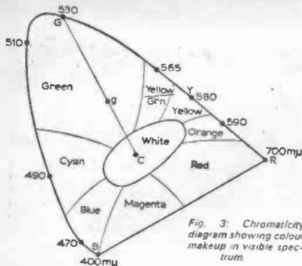
Fig. 3: Chromaticity diagram showing colour makeup in visible spectrum.
