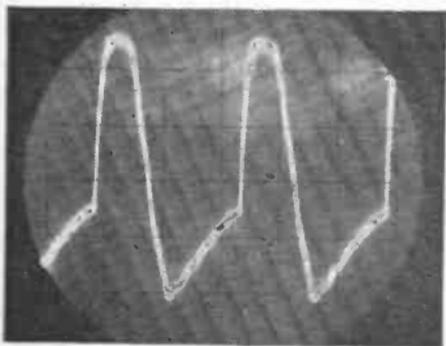
Fig. 6: Line waveform at the screen grid of the line output valve.
