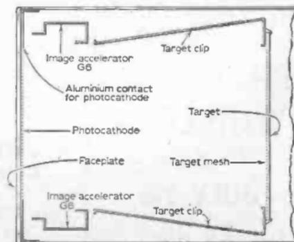
Fig. 1: The image section of the tube.
