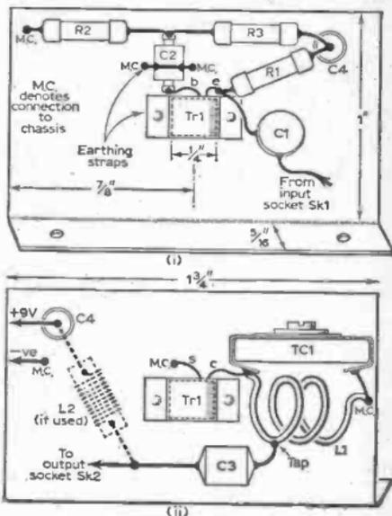
Fig. 3: Layout above and below chassis.
