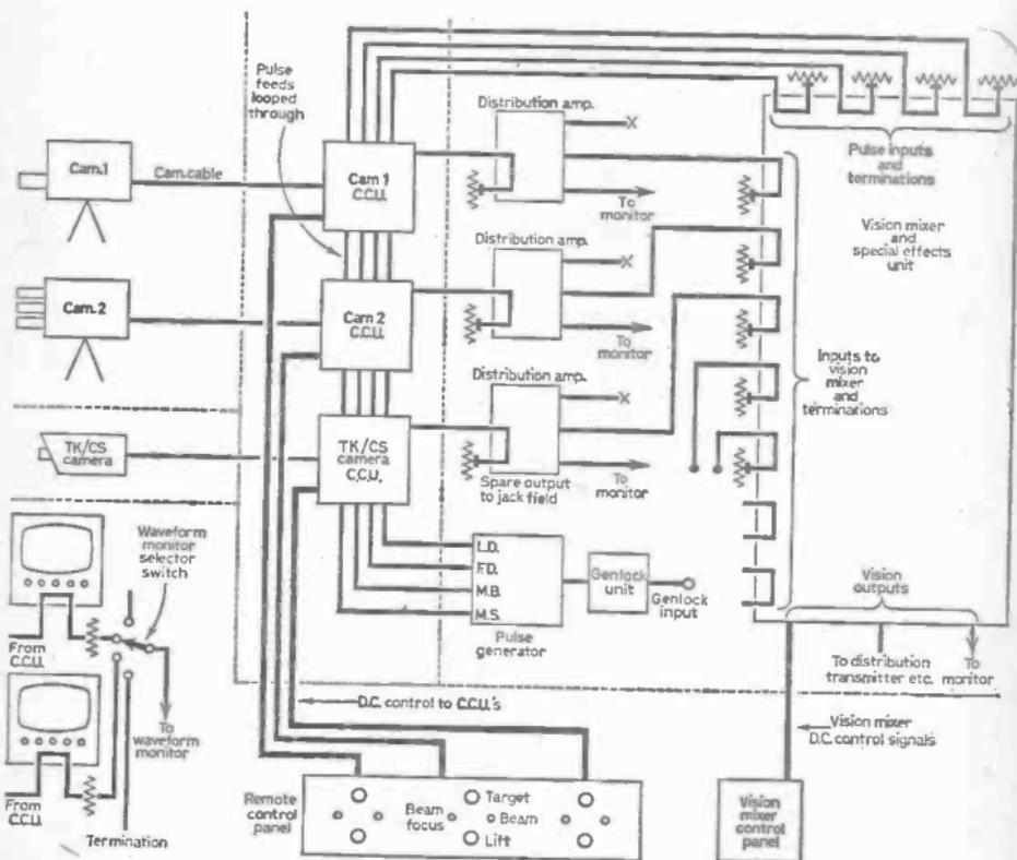
Fig. 74: Video and control schematic showing interconnection between units.
