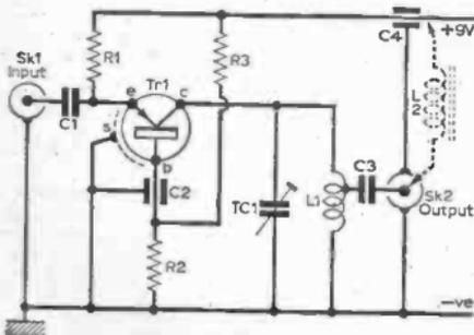
Fig. 2: Circuit diagram of the preamplifier.
