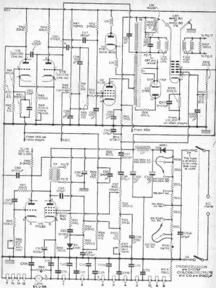
Fig. 4: Line and field timebases and power supplies.
