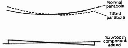
Fig. 34 Tiltting a parabola by adding a sawtooth component.
