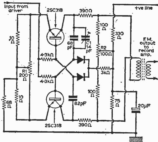
Fig. 16: The f.m. modulator stage consists of an astable multivibrator.
