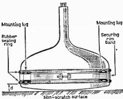
Fig. 1: When fitting replacement tubes secured by rim bands always check distance "d" as well as the location of the mounting lugs.
