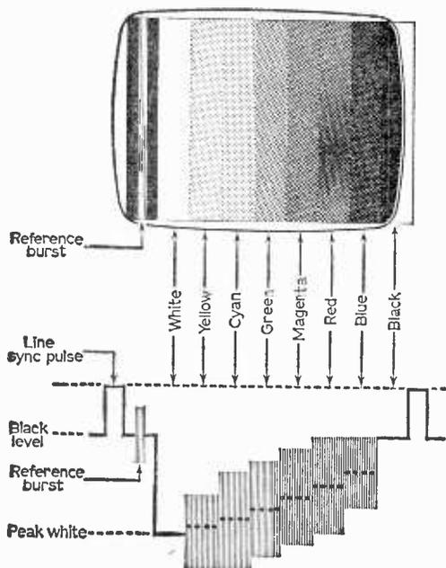
*Fig. 1 (left): The burst spotter's guide. Above is shown the colour bar test pattern as received on monochrome, displaced to the right to enable the burst signal to be observed on the left. Below is the same waveform as monitored on a good quality scope.*
