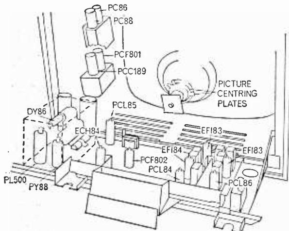
Fig. 1: Rear view of chassis in swung-down position.
