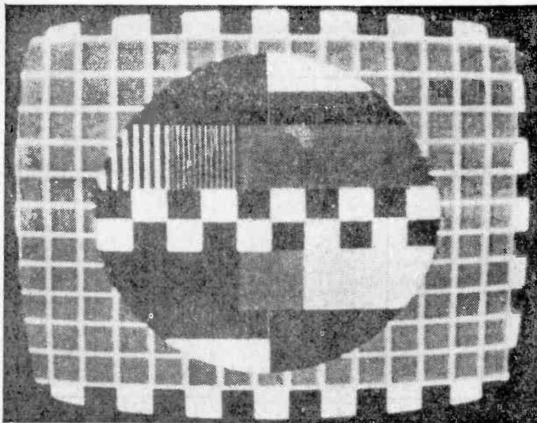
Test Card: Electronic type as photograph. As used by Lopik Ch. 27 as an alternative to Test Card as per Data Panel 12.
