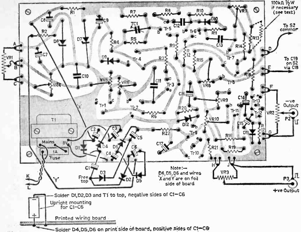
Fig. 2: Printed wiring board, shown from print side. Components on other side.
