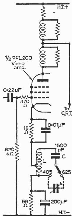
Fig. 2 (right): Notch filtering as used in recent Pye/Ekco models. L and C are switched to form a high-Q parallel-tuned retractor on 405, resonant at 3.5Mc/s. To remove subcarrier patterns on 625 a similar filter resonant at 4.43Mc/s is needed. In this case a capacitor connected across the switch as shown and of value determined by experiment would be all that is required.
