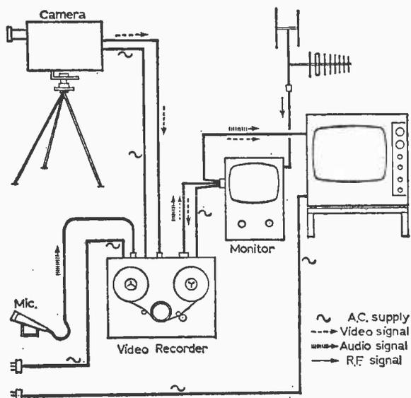
Fig. 14: Practical wiring layout of the Sony 2000 system, showing interconnection between the camera, recorder, monitor/off-air receiver and large-screen monitor, with microphone input in a conventional mode.
