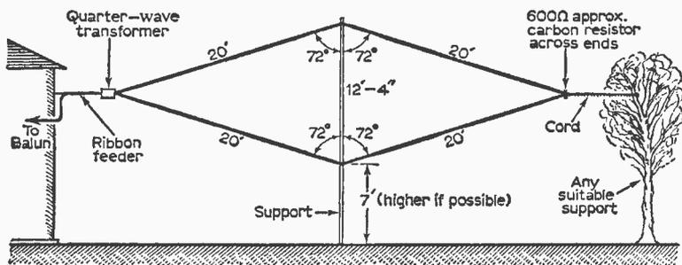
Fig. 1: General arrangement of the Band III rhombic aerial. All sides must be exactly the same length, though the length itself is not very critical. The angle of 72° shown is critical.
