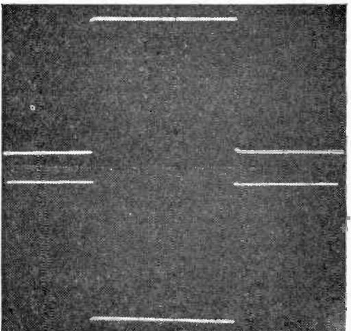
*Pulse output at field pulse width—20mS. Positive pulse at top, negative pulse at bottom.*
