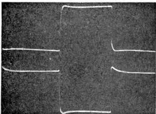
*Pulse output with pulse width equal to one line—100 $\mu$ S approximately (405-line system). Positive pulse at top, negative pulse at bottom.*
