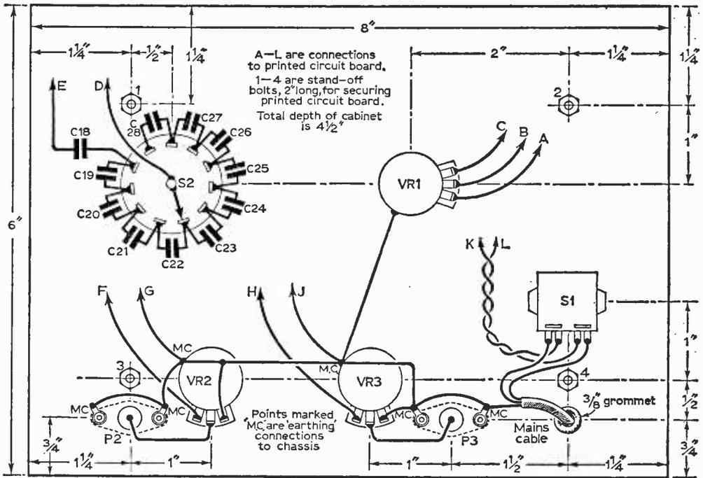
Fig. 3: Rear view of front panel layout.
