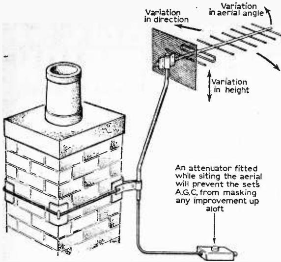
Fig. 3: The last  $\mu\text{V}$  of signal can be obtained at any location by varying aerial height, position and angle. This is most important when receiving colour since the chroma signal is much weaker than the monochrome luminance signal. The aerial may also need to be twisted on its axis for optimum results.
