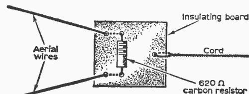
Fig. 2: Mounting for the terminating resistor.
