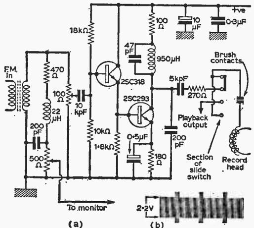
Fig. 18: (a) Circuit of the video record output stage. (b) Sample waveform at head feed.
