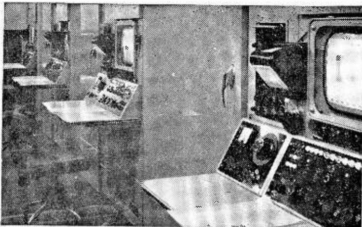
*Left: Flying-spot telecine control panels at the rear of the film transport mechanism. The operator has operational controls, intercom with the studio and hears talkback from the control room and also has a monitor and scope to help him control picture quality. Southern ITV photo.*
