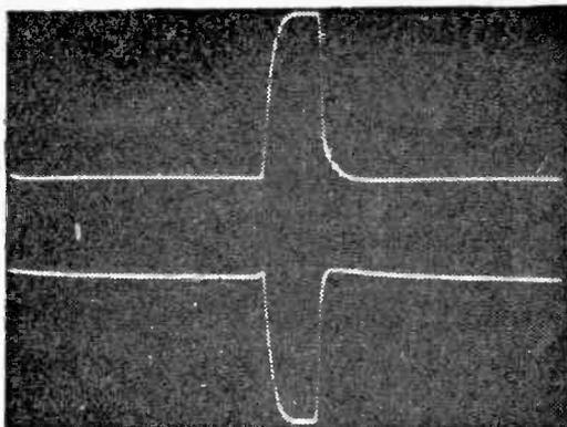
*Pulse output at shortest pulse width—10 $\mu$ S. Rise time 2 $\mu$ S, fall time 600nS. Positive pulse at top, negative pulse below*
