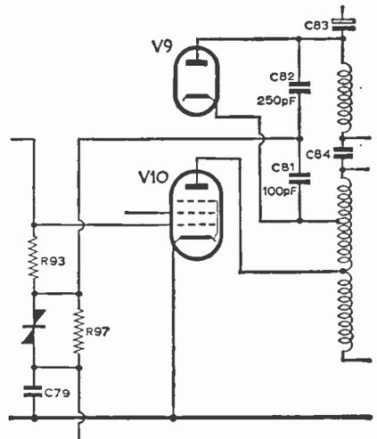
Fig. 2: Line output stage variations in early receivers (serial nos. 237001-238000 and 241001-242500).
