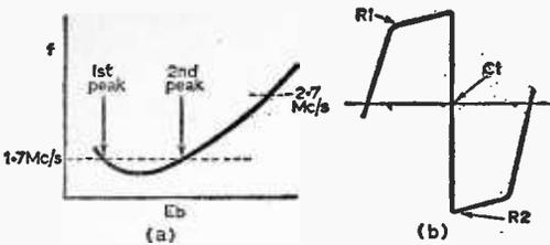
Fig. 17: (a) Output/frequency curve taken at base of video record amplifier, showing need to lock the oscillator to the second peak to avoid the bend at the bottom of the curve. (b) Symmetry waveform. Exact symmetry of the oscillator waveform is essential and three presets are provided for this purpose. After symmetry adjustment check basic frequency to ensure no offset has occurred.
