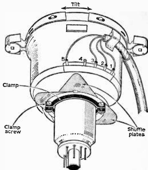
Fig. 2: Typical scan coil assembly (Philips). Slackening the clamp screw enables the assembly to be removed from the tube neck. The shuffle plates centre the picture while scan coil rotation levels the picture.
