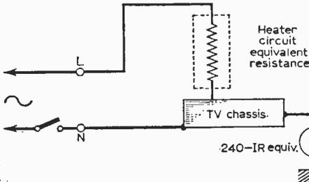
Fig. 1: With a television receiver chassis properly connected to the neutral mains supply lead it becomes live if switched off by breaking the neutral lead only.
