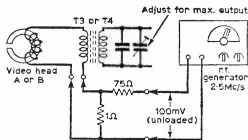
Fig. 19c: Tuning head transformer circuits requires an r.f. generator tuned to 2.5Mc/s with a matching pad in the head return lead.
