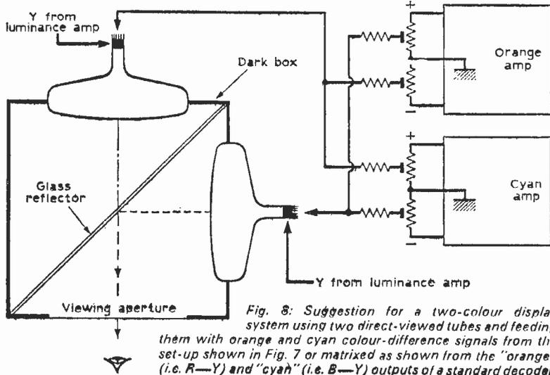
Fig. 8: Suggestion for a two-colour display system using two direct-viewed tubes and feeding them with orange and cyan colour-difference signals from the set-up shown in Fig. 7 or matrixed as shown from the "orange" (i.e. R-Y) and "cyan" (i.e. B-Y) outputs of a standard decoder.
