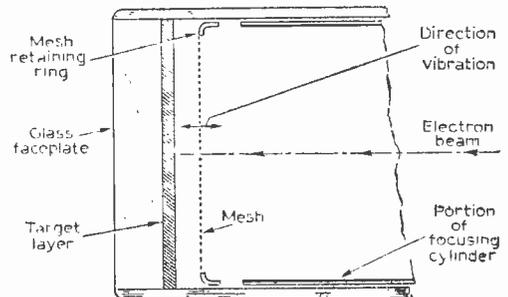
Fig. 1: Microphonic portion of vidicon tube.
