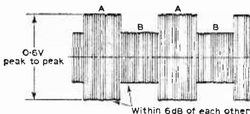
Fig. 19b: The outputs from the preamplifiers appear at TP9 as successive "blocks" which should be within 6dB of each other for correct playback conditions, with a minimum peak-to-peak voltage of 0.4V.
