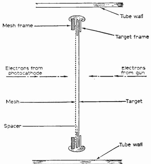
Fig. 3: Vibrating components of image orthicon.
