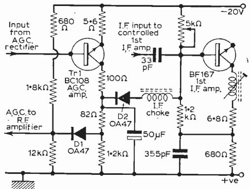
Fig. 3: Commonly used a.g.c. delay circuit providing independent control of the r.f. and i.f. stages.
