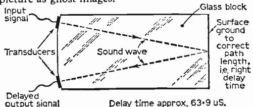
Fig. 9: The type of chrominance line-period delay line in general use in colour receivers.
