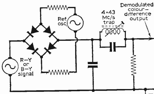
Fig. 10: A synchronous demodulator circuit in wide use. The series diode bridge detector.
