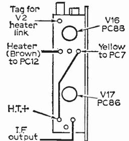
Fig. 6: Representative u.h.f. tuner unit wiring.
