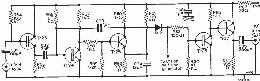
Fig. 8: The half-field generator. The same type of circuit as the half-line generator is used, with the value of the time-constant cross-coupling capacitor altered to give the required pulse repetition frequency.
