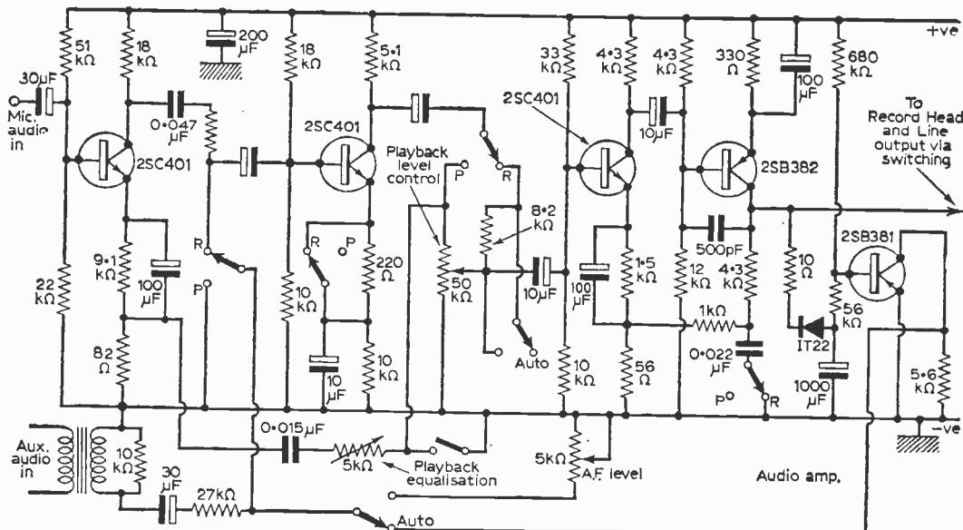
Fig. 33: The audio manual/auto circuits.
