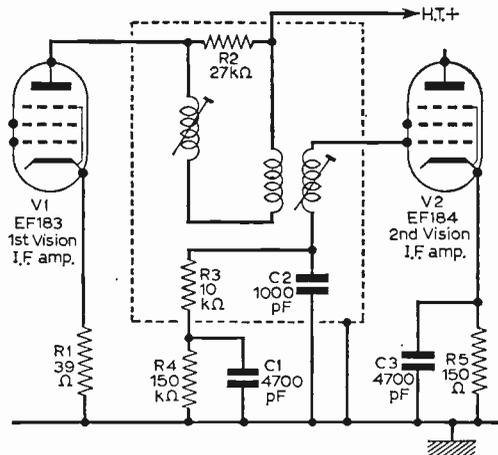
Fig. 15: Vision i.f. circuit overload protection. Should excessive inputs drive V2 into grid current R4, C1 develop additional self-bias to add to the bias provided by R5. V1 has a.g.c. applied to it R1 being left unbypassed to offset variations in input capacitance caused by a.g.c. variations.
