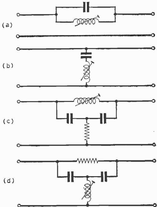
Fig. 11: Typical wavetraps used in television receiver i.f. circuits: (a) series rejector, (b) parallel acceptor, (c) and (d) bridged-T rejectors. Bridged-T filters give a much higher degree of attenuation and a more sharply tuned response than simple acceptor or rejector circuits.
