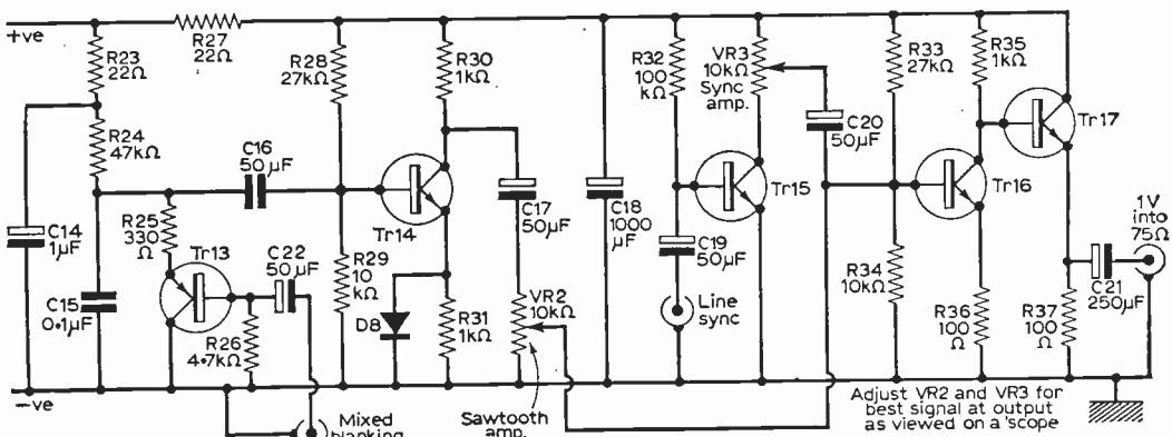
Fig. 6: The sawtooth pattern generator. The sawtooth waveform is generated by C15 charging exponentially via R24 and discharging when shorted by Tr13 being switched hard on. Tr14 acts as a linear amplifier.
