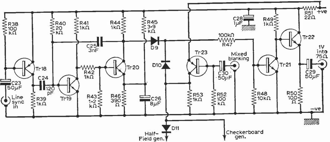
Fig. 7: The half-line generator. Tr18 inverts the input sync pulses which are used to trigger the monostable multivibrator Tr19, Tr20. The output is fed via D9 to the inverter Tr21 and emitter-follower output transistor Tr22, and via D10 to the checkerboard pattern generator to be described next month. The blanking pulses are also fed to the output to the checkerboard generator via Tr23.
