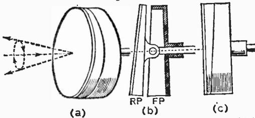
Fig. 12: Spiral scanner: (a) scanning ray sweeps widely to trace outer curve of spiral; (b) reflector plate RP separated from flange plate FP (section); (c) ray returned to centre of screen on completion of spiral trace.
