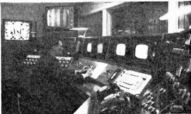
*Telecine Control Room: In the foreground the audio test selector, tone generator and channel control panels. In front of the controller are the four video monitors, camera control units and mixing panels. Beyond the controller are the intercom waveform monitor and relay selector panels. Above these can be seen the R, G, B and black-and-white terminal monitors.*
