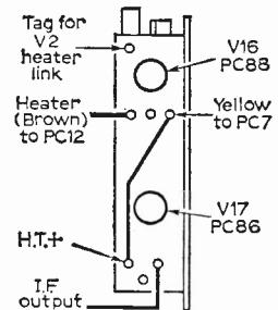
Fig. 6: Representative u.h.f. tuner unit wiring.
