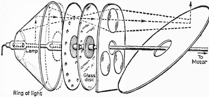
Fig. 10: Cone reflector for multi-scan: annular projection with apertured disc, bushed glass plate and circle of lenses.
