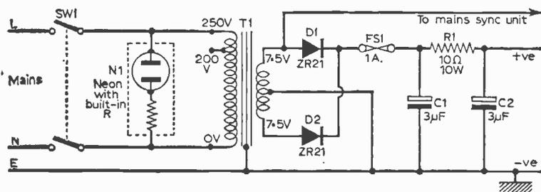
Fig. 1 (left): The power supply circuit. One of the 7.5V a.c. phases is taken to the mains lock circuit to synchronise the field generator.
