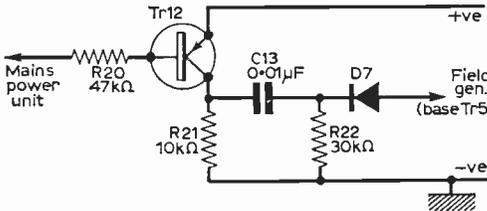
Fig. 5: The mains lock circuit. The 50 c/s sine wave input is applied to the base of Tr12 via the limiting resistor R20. The resulting square wave is differentiated by C13 and R22, clipped by D7 and used to synchronise the multivibrator Tr5, Tr6.
