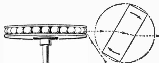
Fig. 9: Ball-bearing scanner. Line traced by reflection from each ball. Rotating glass block deflects in frame direction.
