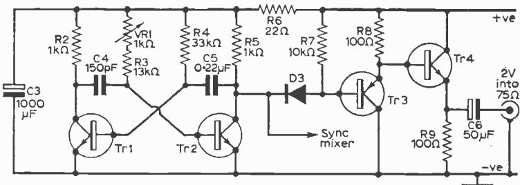
Fig. 2 (right): The line generator circuit. This consists of a standard free-running multivibrator circuit feeding a compound emitter-follower pair. VR1 enables the circuit to be set to 15,625 c/s (625 lines).
