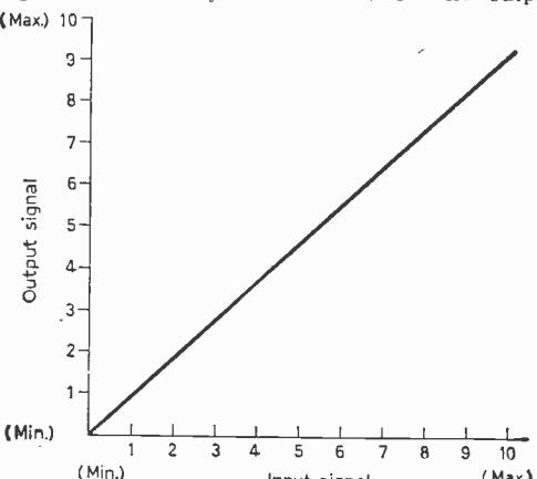
Fig. 1: The ideal transfer characteristic without non-linearity.
