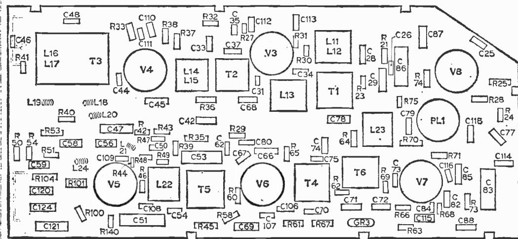
Fig. 3: Component layout of the i.f. printed board.
