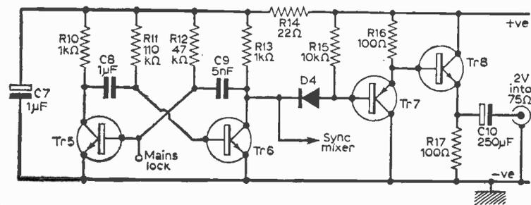
Fig. 3 (left): The field generator circuit. Apart from the time-constants of the multivibrator this is identical to the line generator. Tr5 base is synchronised to the mains frequency via the mains lock circuit.
