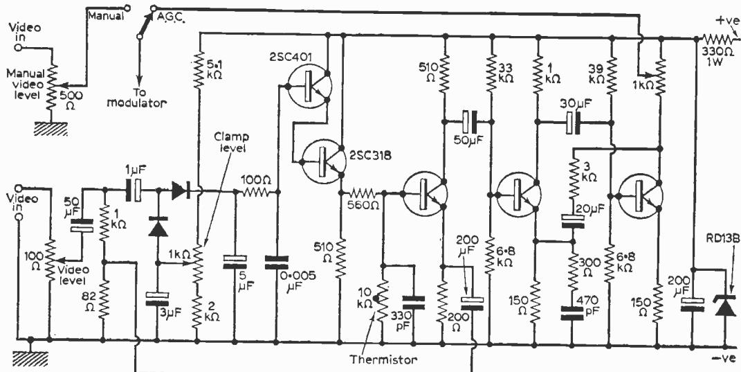
Fig. 32: The video manual/auto circuits.
