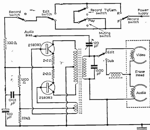
Fig. 31 (left): Additional switching is incorporated in the power supply circuits and in the erase head section of the latest machines to enable editing and dubbing of vision and sound to be carried out. Note that while editing, i.e. insertion of new video material, causes erasure of both vision and sound, dubbing switches in the sound erase winding only via a loading coil.
