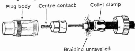
*Fig. 1: Better way of fixing a coaxial plug*
