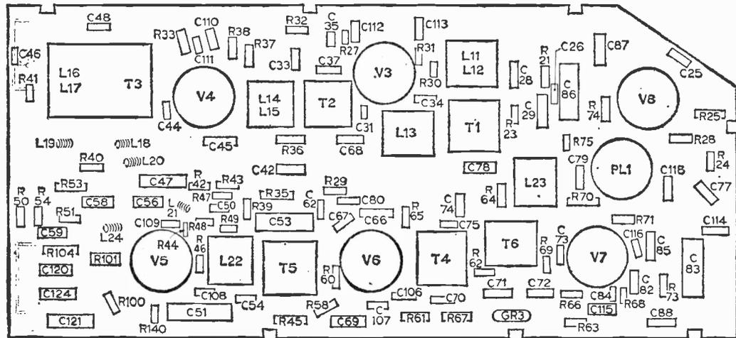
Fig. 3: Component layout of the i.f. printed board.
