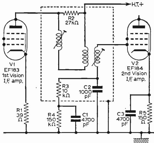
Fig. 15: Vision i.f. circuit overload protection. Should excessive inputs drive V2 into grid current R4, C1 develop additional self-bias to add to the bias provided by R5. V1 has a.g.c. applied to it R1 being left unbypassed to offset variations in input capacitance caused by a.g.c. variations.
