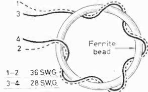
Fig. 3: T1, T2 and T3 winding details.
