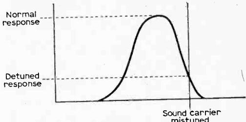
**Fig. 6:** When the tuning of a 405-line set is in error the sound carrier moves away from the sound response curve as shown. This reduces the sound sensitivity and encourages sound-on-vision interference. On the 625-line standard the 6Mc/s intercarrier signal remains exactly at that frequency in spite of mistuning within the passband.
