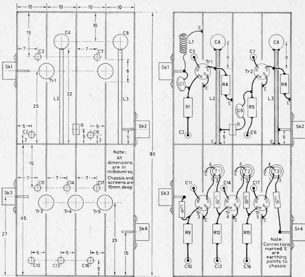
Fig. 5: Under-chassis layout and dimensions
