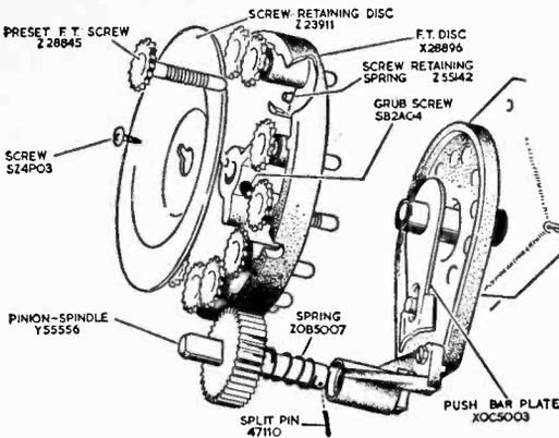
Fig. 3: Preset fine tuning mechanism.
