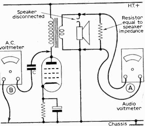
*Fig. 2: Ways of indicating the amount of signal present at the output of the sound channel.*
