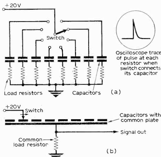
Fig. 4: Extracting the video signal from the vidicon.
