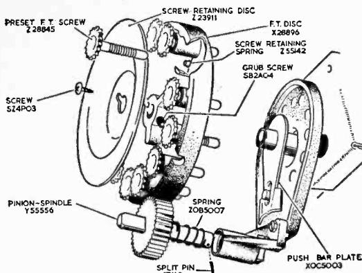
Fig. 3: Preset fine tuning mechanism.
