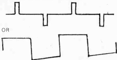
Fig. 12: Two typical ident pulse trains.
