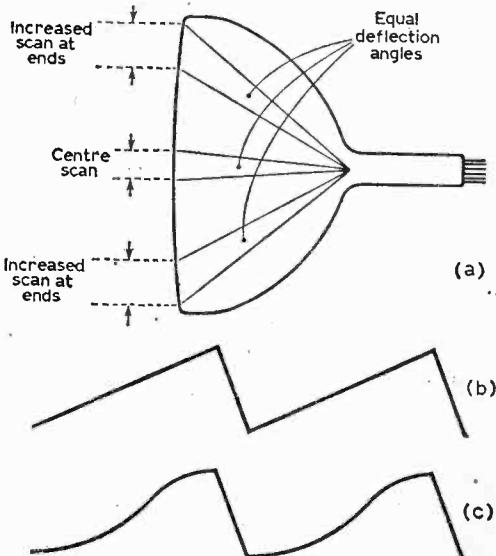
Fig.1: (a) Showing increased sweep obtained at end of scan compared to that at centre for equal deflection angle. (b) Sawtooth scan waveform. (c) Sawtooth waveform modified by S-capacitor in series with scan coils, introducing a parabolic component
