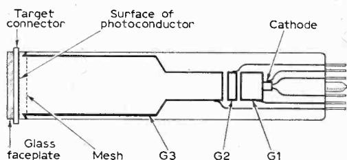
Fig. 3: Main parts of the vidicon camera tube.
