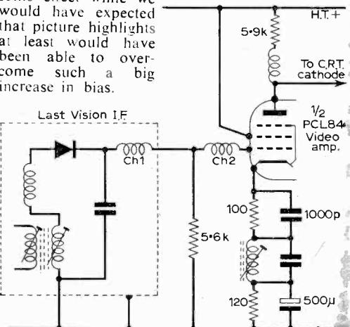
Fig. 2: Typical 405-only video circuit. The positive-going output from the diode detector produces an increased voltage at the video amplifier cathode as contrast is advanced. In one case of vision failing after 20 minutes coincident increase in this voltage indicated the probable cause.
