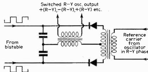
Fig. 16: A PAL R-Y switch circuit.
