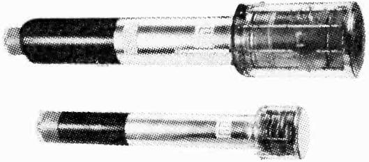
The large and small models of the EEV Image Isocons—the camera tubes that "see in the dark".
