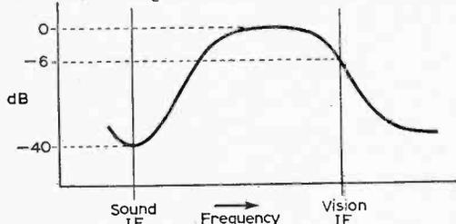
Fig. 5: Basic response curve in the vision i.f. channel of a 625-line set or on the 625-line position of a dual-standard set. Note that the sound i.f. falls in a trough at about 40dB down from the top of the curve, while the vision carrier is about 6dB down on the other side of the curve. Adjusting the u.h.f. tuning causes both carriers to move along the response, thereby resulting in the sound i.f. rising from its trough and the vision i.f. changing from its correct -6dB position.
