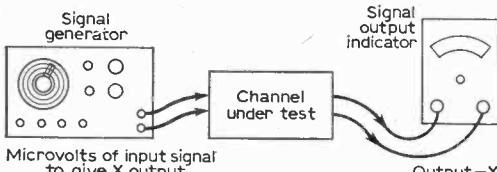
Fig. 1: The basic concept of sensitivity. The idea is to find the input signal (sound and vision) required to produce a specified standard output.
