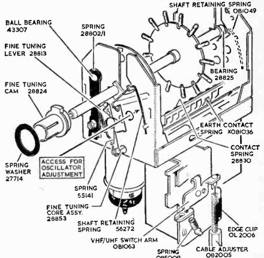
Fig. 4: Rotary tuner with fine manual tuning.
