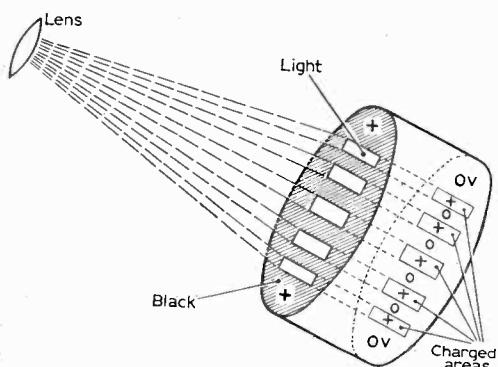
Fig. 2: Action of vidicon photoconductive layer.
