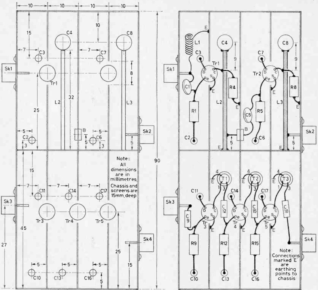
Fig. 5: Under-chassis layout and dimensions
