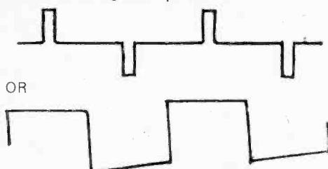
Fig. 12: Two typical ident pulse trains.
