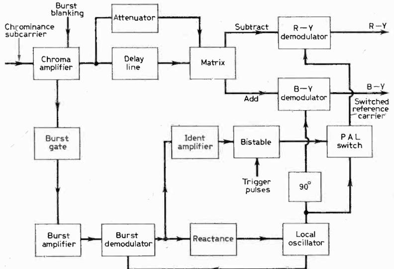
Fig. 14: Block diagram of a PAL decoder.
