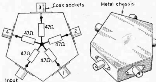
Fig. 7: Four-way resistive splitter network.
