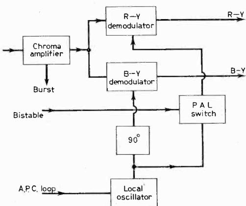
Fig. 15. Showing how the chrominance signal path is simplified in a PALs decoder.
