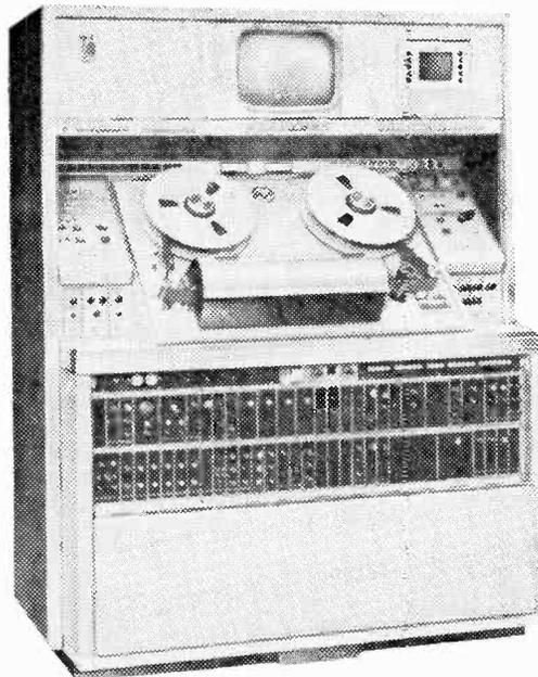
Colour video tape recorder TR70 which is suitable for use with either PAL or NTSC systems.
