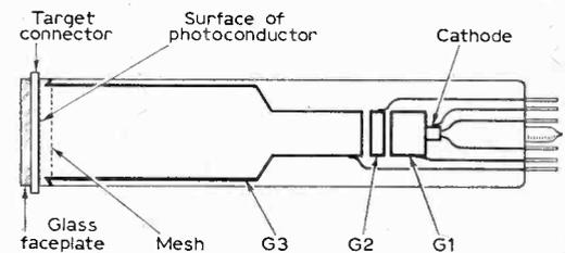
Fig. 3: Main parts of the vidicon camera tube.
