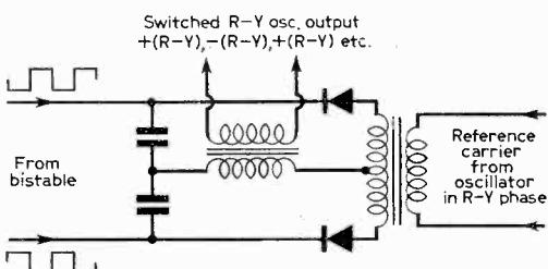
Fig. 16: A PAL R-Y switch circuit.
