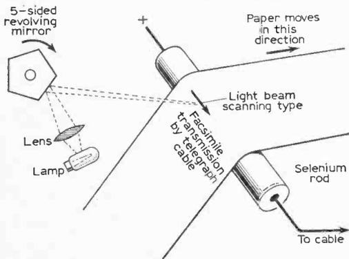
Fig. 1: Use of photoconductive selenium rod for newspaper picture telegraphy.
