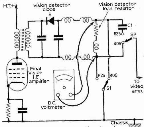
*Fig. 3: Metering sensitivity in the vision channel.*
