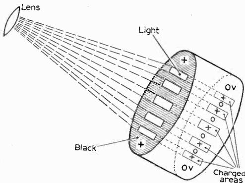
Fig. 2: Action of vidicon photoconductive layer.
