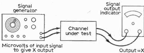
Fig. 1: The basic concept of sensitivity. The idea is to find the input signal (sound and vision) required to produce a specified standard output.
