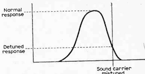
Fig. 6: When the tuning of a 405-line set is in error the sound carrier moves away from the sound response curve as shown. This reduces the sound sensitivity and encourages sound-on-vision interference. On the 625-line standard the 6Mc/s intercarrier signal remains exactly at that frequency in spite of mistuning within the passband.
