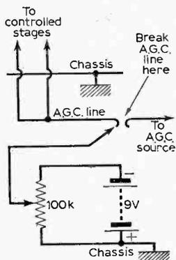
Fig. 4 (left): It is possible to cut the a.g.c. line as shown and adjust the bias on the controlled valves by means of a potentiometer connected across a battery. Take care to observe the correct polarity or the controlled valves will be fed with a positive bias instead of the correct negative bias.
