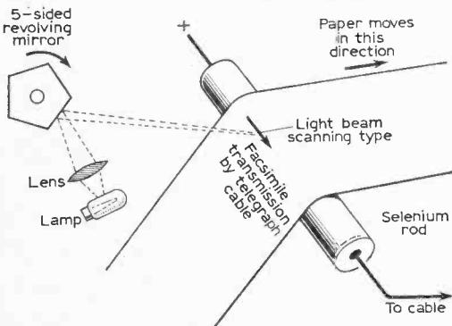
Fig. 1: Use of photoconductive selenium rod for newspaper picture telegraphy.
