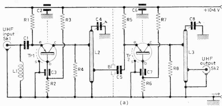
Fig. 1 (left) : Circuit diagram of (a) the u.h.f. amplifier, (b), the v.h.f. amplifier and (c) the power supply with stabilisation.
