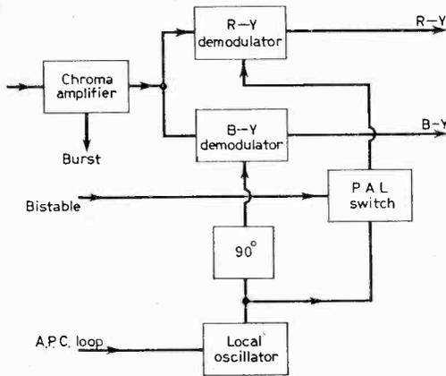
Fig. 15: Showing how the chrominance signal path is simplified in a PALs decoder.
