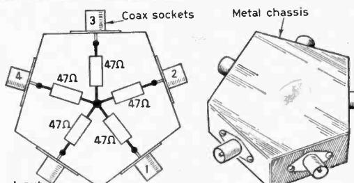
Fig. 7 : Four-way resistive splitter network.
