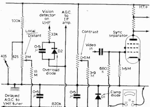
Fig. 1: Typical modern a.g.c. system (Thorn 900 Series). Simultaneous contrast and a.g.c. increase indicates a receiver section fault. Contrast increase with a.g.c. decrease is caused by a fault in the a.g.c. circuit.
