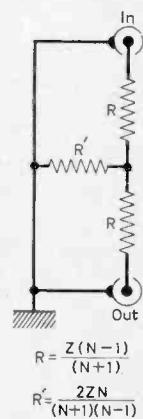
Fig. 6: General formulae for voltage attenuators.  $Z$  is the feeder impedance and  $N$  the attenuation ratio.
