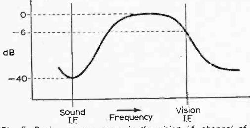
**Fig. 5:** Basic response curve in the vision i.f. channel of a 625-line set or on the 625-line position of a dual-standard set. Note that the sound i.f. falls in a trough at about 40dB down from the top of the curve, while the vision carrier is about 6dB down on the other side of the curve. Adjusting the u.h.f. tuning causes both carriers to move along the response, thereby resulting in the sound i.f. rising from its trough and the vision i.f. changing from its correct -6dB position.
