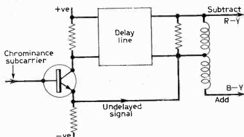
Fig. 13: Chrominance matrixing in the decoder to separate the B-Y and R-Y signals.
