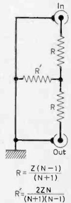
Fig. 6: General formulae for voltage attenuators. Z is the feeder impedance and N the attenuation ratio.
