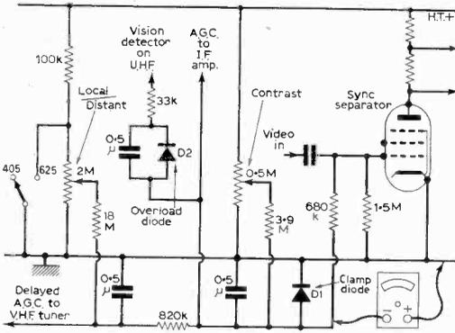
Fig. 1: Typical modern a.g.c. system (Thorn 900 Series). Simultaneous contrast and a.g.c. increase indicates a receiver section fault. Contrast increase with a.g.c. decrease is caused by a fault in the a.g.c. circuit.
