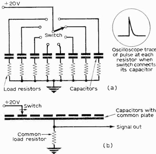
Fig. 4: Extracting the video signal from the vidicon.
