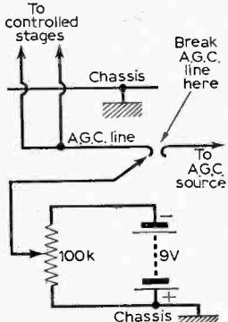
**Fig. 4 (left):** It is possible to cut the a.g.c. line as shown and adjust the bias on the controlled valves by means of a potentiometer connected across a battery. Take care to observe the correct polarity or the controlled valves will be fed with a positive bias instead of the correct negative bias.
