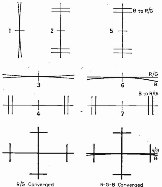
Fig. 14: Complete dynamic convergence procedure step-by-step. Adjust each error in sequence 1-7.
