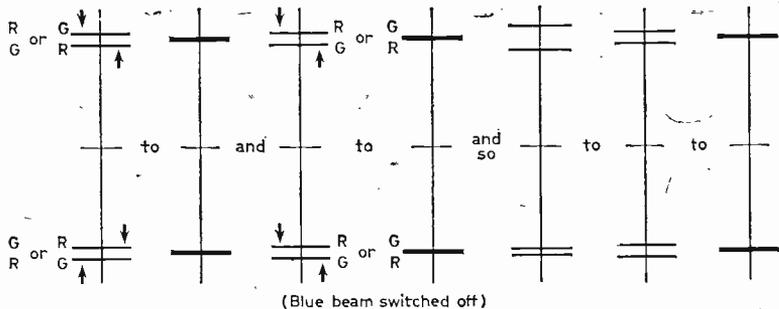
Fig. 7 (right): Dynamic convergence of field R/G horizontal lines.
