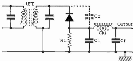
Fig. 22: Basic signal rectifier circuit. For high detection efficiency diode forward resistance must be low compared to  $R_L$  and its internal capacitance must be low compared with  $C_L$ .
