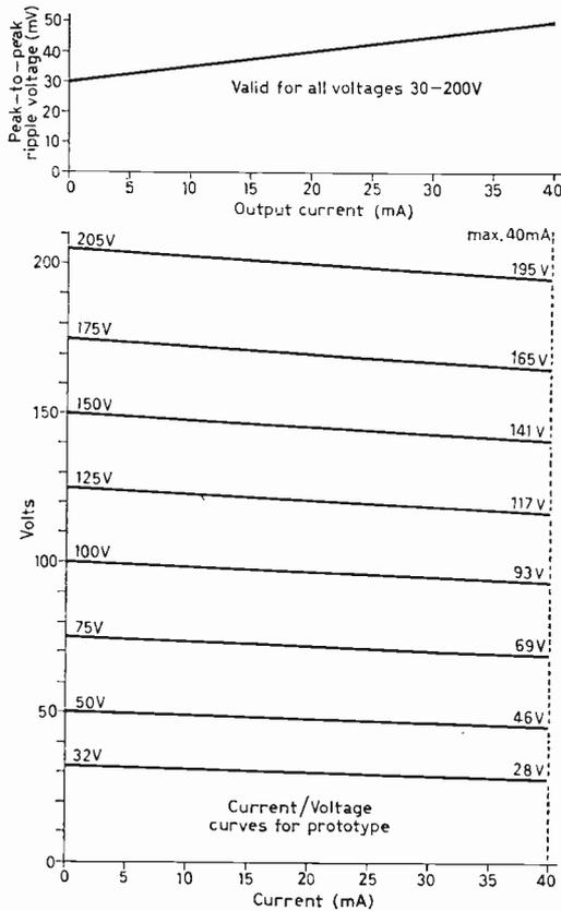
Fig. 6: Performance of the H.T.1 30-200V output. To preset the output from this circuit proceed as follows. With zero output current drain (open-circuit) alternately adjust VR1 for 32V output and VR3 for 205V output between P5 and P6, with VR2 at its left- and right-hand stops respectively. The final adjustment is of VR3 for 205V output with VR2 at its right-hand stop. Then calibrate the scale of VR2.
