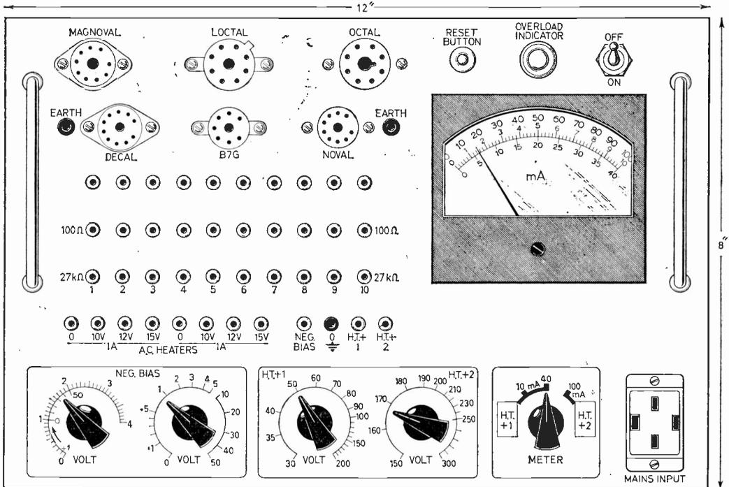
Fig. 8: Front panel layout. The front panel and chassis form an integrated drawer unit which pushes into the 6 1/2 in.-deep cabinet.
