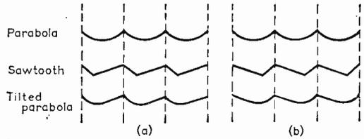
Fig. 5: Tilting a parabola: (a) Parabola tilted by a negative-going sawtooth waveform; (b) Parabola tilted by a positive-going sawtooth waveform.
