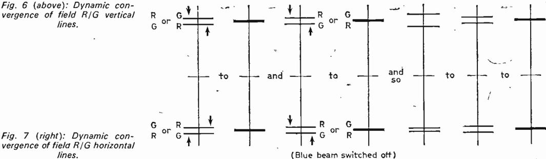
Fig. 7 (right): Dynamic convergence of field R/G horizontal lines.
