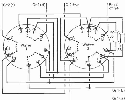
Fig. 5: Wiring of the meter switch S2. The contact wipers of the switch must be narrow so that make-before-break operation is ensured. A 3-way, 6-pole switch is used: connect the sixth pole in parallel with section E to reduce variable contact resistance in the meter shunting circuit.
