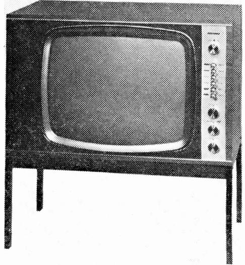
The 22 in. Murphy colour receiver model CV2210D features an integrated circuit for signal processing in the decoder, providing R, G, B drive outputs.
