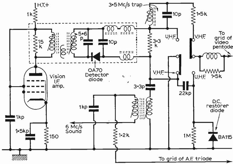
Fig. 23 (left): Typical single diode dual-standard vision detector circuit. This example is taken from the Philips Style 70 series of receivers. The output is direct coupled to the video amplifier grid on v.h.f. On u.h.f. however a.c. coupling is used, with d.c. restoration by the BA115 diode.
