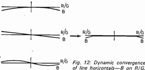
Fig. 12: Dynamic convergence of line horizontals—B on R/G.
