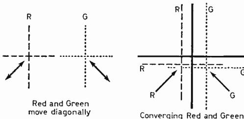
Fig. 3: Procedure for correcting static convergence errors. First converge the red and green horizontal and vertical centre lines. This is achieved by diagonal movements. Then converge blue on the converged red and green (yellow) lines. Vertical and lateral movement of the blue beam is required for this.
