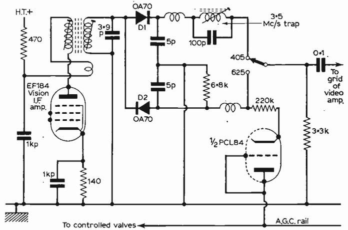
will be more clearly defined than a following equivalent reduction. However in practice this effect may well be masked by the receiver's overall frequency response so that the detector time constant is always taken to be the product of load resistance and shunting capacitance. Assuming an average load resistor of  $5k\Omega$  and total shunt capacitance, strays plus that of the reservoir, of  $10pF$ , the time constant will be:
