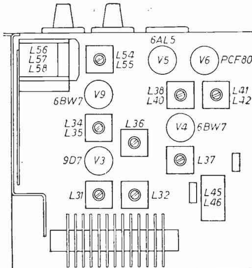
Fig. 2: Above chassis layout of the i.f. stages.
