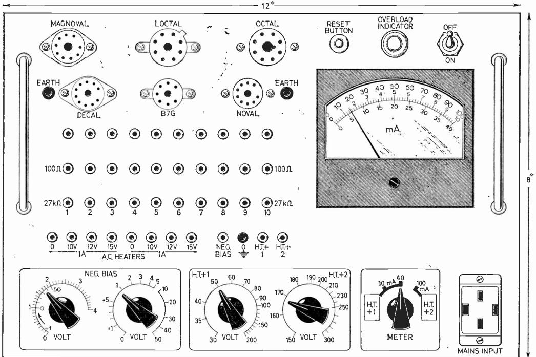
Fig. 8: Front panel layout. The front panel and chassis form an integrated drawer unit which pushes into the 6 1/4 in.-deep cabinet.
