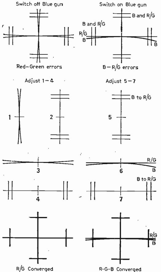
Fig. 14: Complete dynamic convergence procedure step-by-step. Adjust each error in sequence 1-7.
