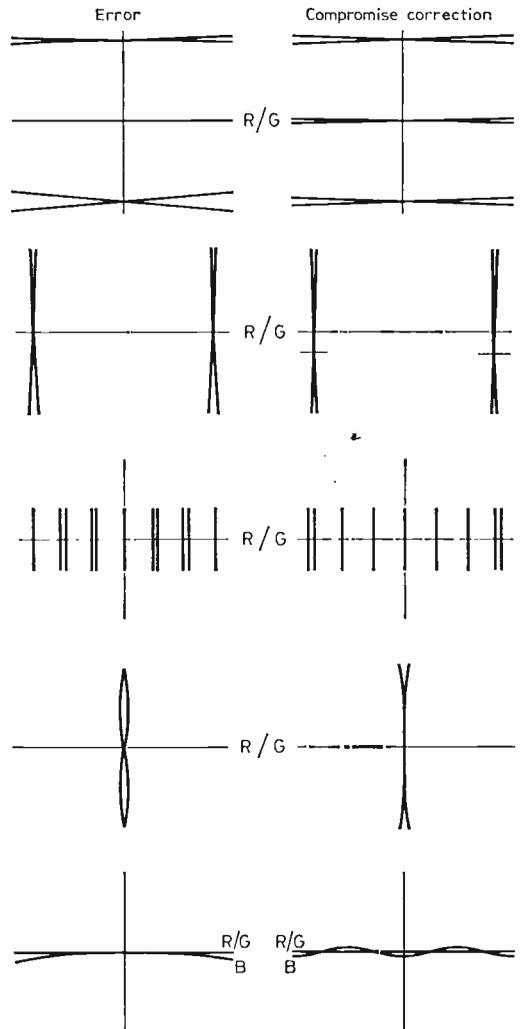
Fig. 16: Spreading the residual errors to produce a better overall effect. Only a small amount of compromise is permissible.
