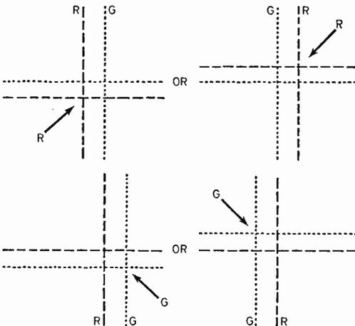
Fig. 4: Static convergence of the red and green beams—the final move.
