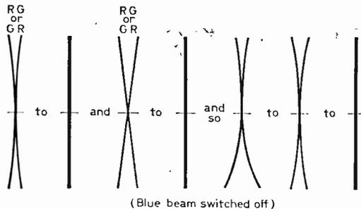
Fig. 6 (above): Dynamic convergence of field R/G vertical lines.
