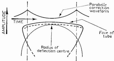
Fig. 3: The basic correction waveform required to compensate for the difference between the geometry of the tube face and the radius of the deflection centres is the parabola.
