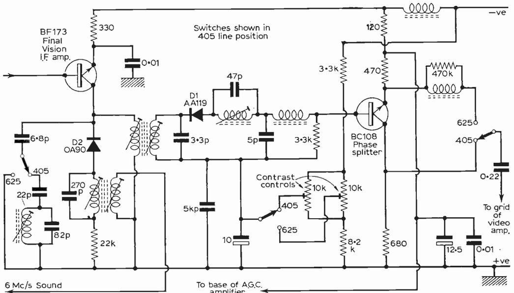
Fig. 25: Single diode (D1) u.h.f./v.h.f. vision detector as used in the Pye group 1967-68 hybrid chassis. A separate detector (D2) is used for the 6Mc/s sound signal on u.h.f. The video phase splitter stage Tr2 provides a positive-going output at its collector on v.h.f. and a negative-going output at its emitter on u.h.f.
