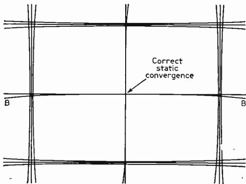
Fig. 5: Typical dynamic convergence errors.
