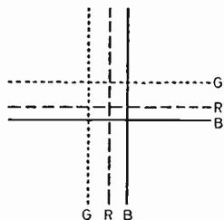
Fig. 2 (left): Typical static convergence errors (magnified).
