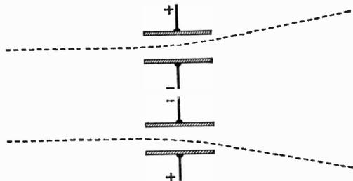
Fig. 1: The principle of electrostatic deflection. A beam of electrons is attracted by a positive potential and repelled by a negative one.
