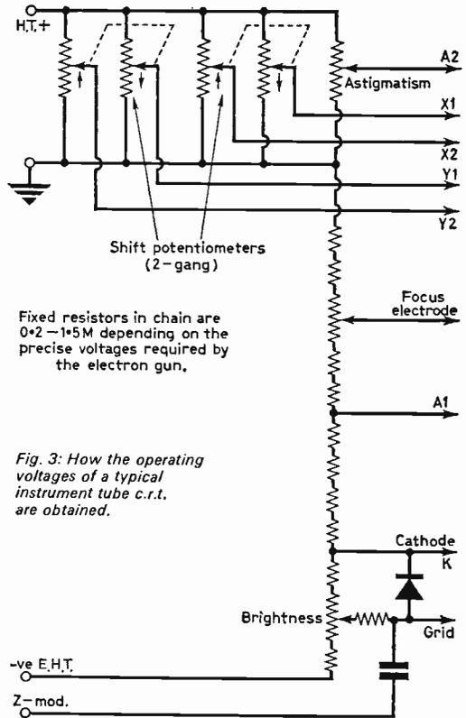
Fixed resistors in chain are 0.2-1.5M depending on the precise voltages required by the electron gun.
