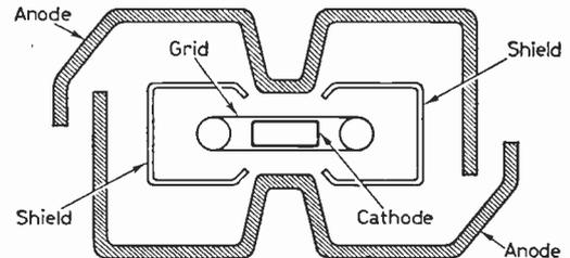
Fig. 2: Construction of a beam triode using shaped anodes and earthed shields to reduce anode-grid capacitance to a minimum.
