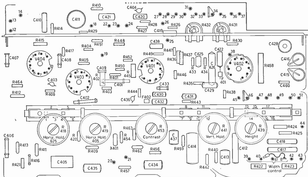
Fig. 4: Layout of the timebase printed board, viewed from the component side.
