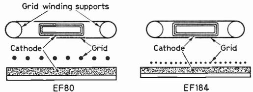
Fig. 1: How frame-grid construction (EF184) reduces grid-cathode spacing.
