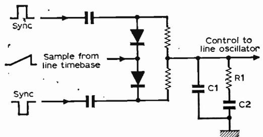
Fig. 3: A simple type of flywheel line sync discriminator; C1, R1, C2 are the flywheel components.
