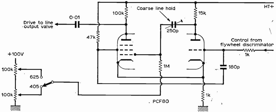
Fig. 4: Representative line generator circuit. This multivibrator employs both cathode and anode-to-grid cross-coupling. To reduce the load on the oscillator, feedback to the triode is from the screen grid instead of the anode of the pentode section of the valve.
