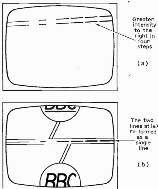
Fig. 4: Slow field retrace will show the BBC test pulses at the top of the picture as at (a). They are normally present between fields as at (b).
