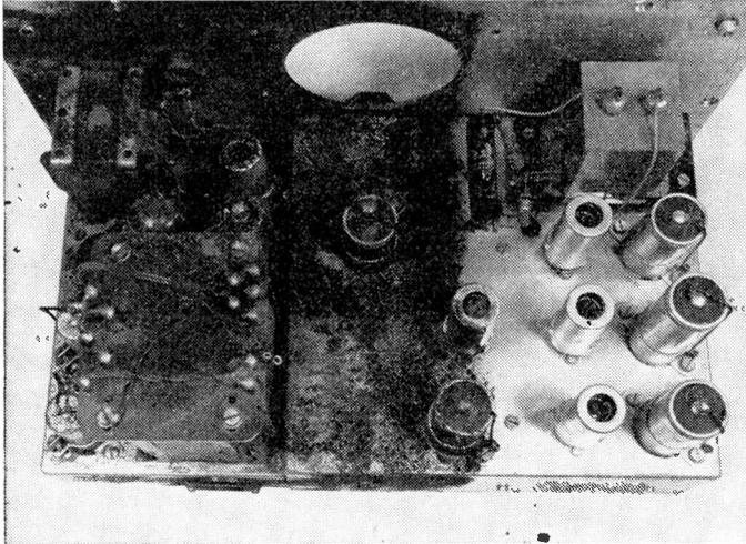
THE above photograph, sent to us by Dawe Instruments Ltd., shows how a chassis has been cleaned by one of their ultrasonic cleaning machines.
