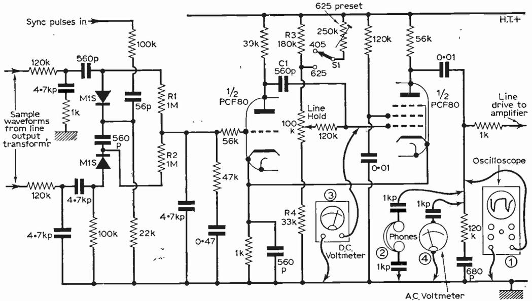
Fig. 1: Basic tests to make in the line oscillator stage. The stage shown uses a cathode-coupled multivibrator with flywheel line sync.
