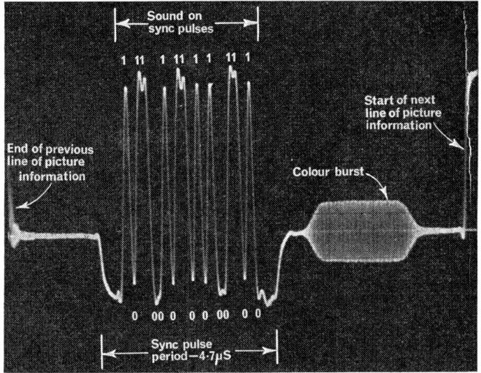
Fig. 2: BBC sound-in-vision signal. Two ten-digit binary signals are inserted in each sync pulse period. The pulses here read 101100101101010011010.
