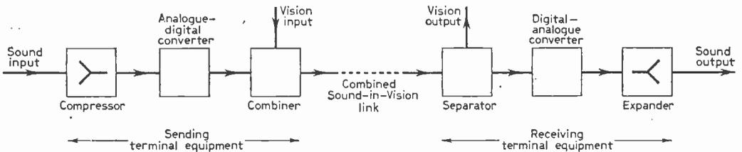
Fig. 3: Block diagram of the BBC sound-in-vision distribution system.
