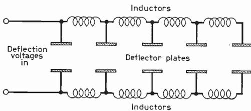
Fig. 4: The principle of travelling wave deflection whereby bandwidths of 1500Mc/s have been obtained.
