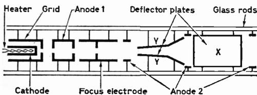
Fig. 2: Cross-section of the electron gun of a typical instrument c.r.t.
