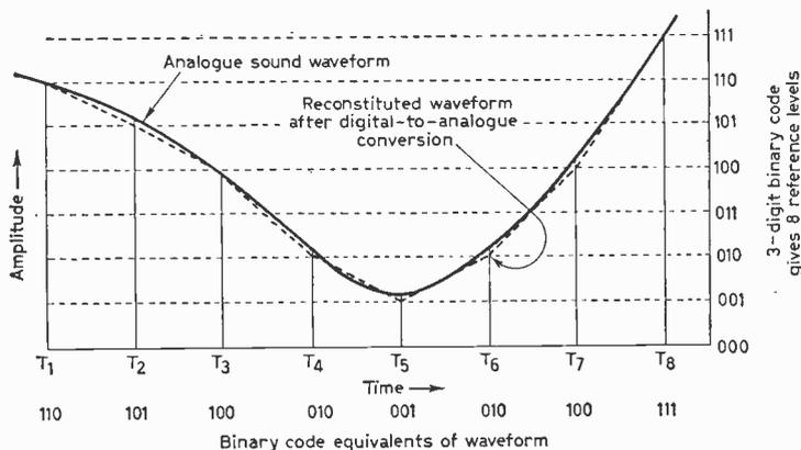
Fig. 1: Basic principle of sampling a sound waveform and converting the samples into binary form.
