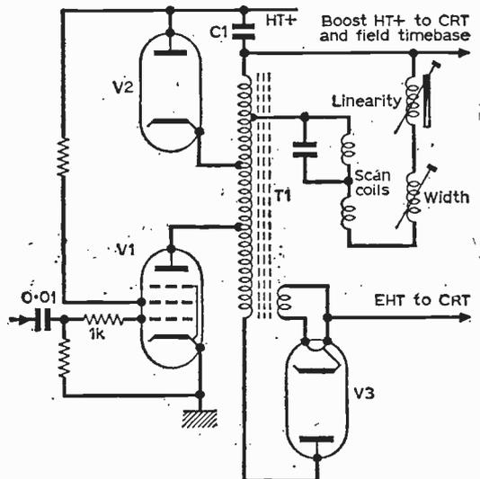
Fig. 1: Typical line output stage. V1 line output pentode, V2 efficiency or boost diode, V3 e.h.t. rectifier. T1 is the output transformer and C1 the boost reservoir capacitor.
