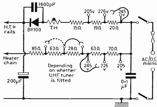
Fig. 1: Unconventional connection of the thermistor in the h.t. rectifier surge limiter circuit instead of in the heater chain in the GEC 2000DS series.
