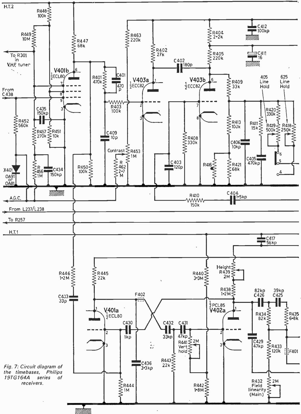
Fig. 7: Circuit diagram of the timebases, Philips 19TG164A series of receivers.
