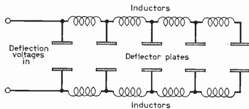
Fig. 4: The principle of travelling wave deflection whereby bandwidths of 1500Mc/s have been obtained.
