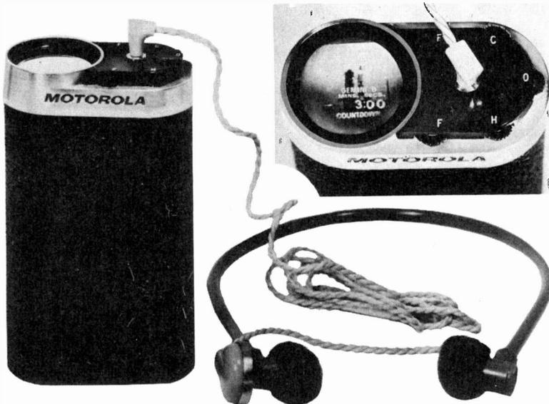
picture tube, power supply and batteries, the actual receiver circuits taking up only one cubic inch. Altogether 43 Motorola transistors and diodes are employed in the receiver which is at present designed for single channel operation. The set has a 3-transistor tuner, 3-stage i.f. amplifier, 2-stage video amplifier, ratio-detector type intercarrier sound demodulator and automatic gain control.
