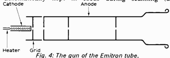
Fig. 4: The gun of the Emitron tube.
