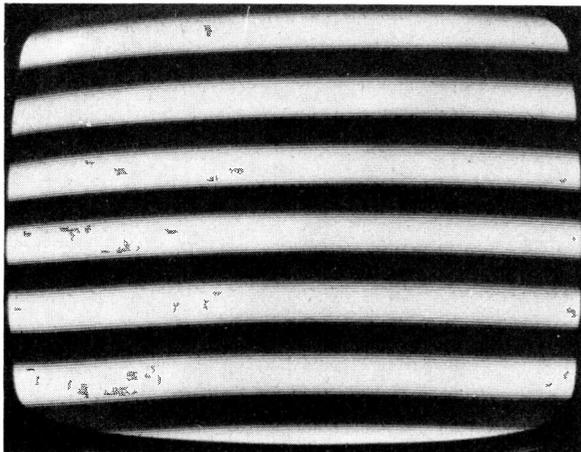
Fig. 2: Low-frequency screen test tone display.
