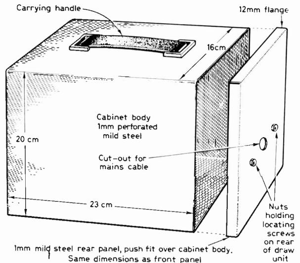
Fig. 7: Details of the case.
