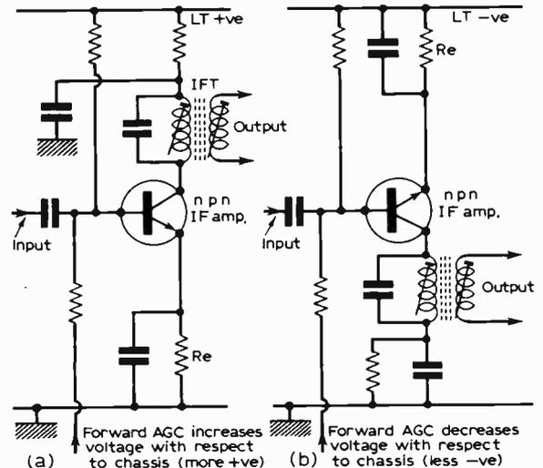
Fig. 3: Application of forward a.g.c. to transistor i.f. amplifier stages.
