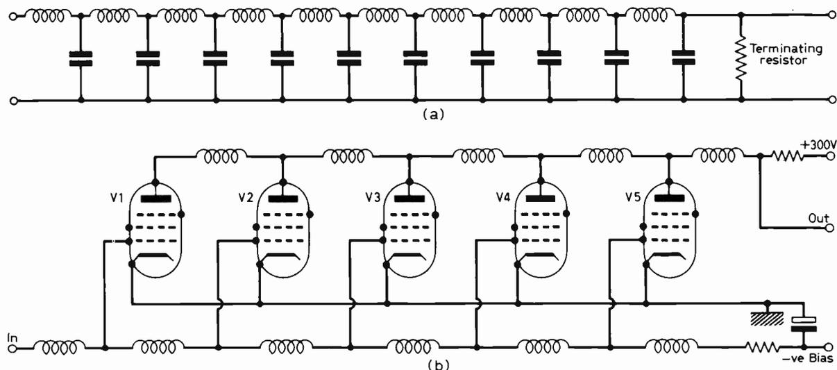
Fig. 14: The travelling-wave or distributed amplifier.
