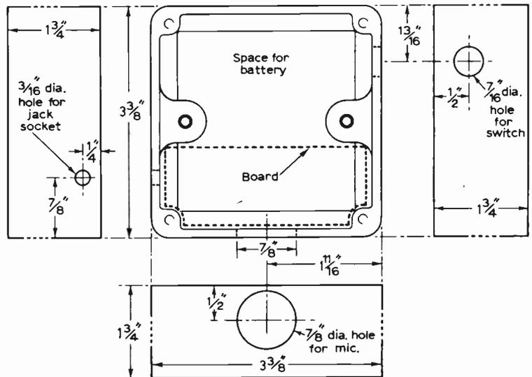
Fig. 3: Detailed plans for drilling the MK box (half scale).
