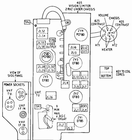
Fig. 4: Above chassis view of the receiver unit.
