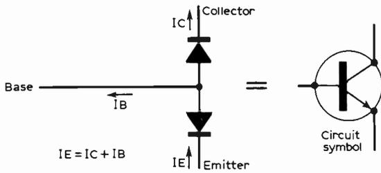
Fig. 28: A transistor looks like a pair of diodes connected back-to-back. For low-power silicon npn transistors  $V_c$  cannot be less than  $V_e + 0.1$  volts approximately because of the clamping action of the cb junction. Similarly  $V_b$  cannot exceed  $V_e + 0.6$  volts approximately.
