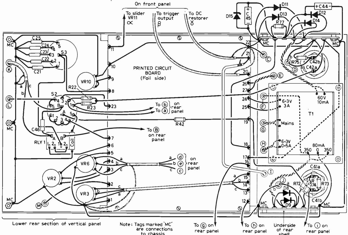
Fig. 5: Underside wiring diagram.
