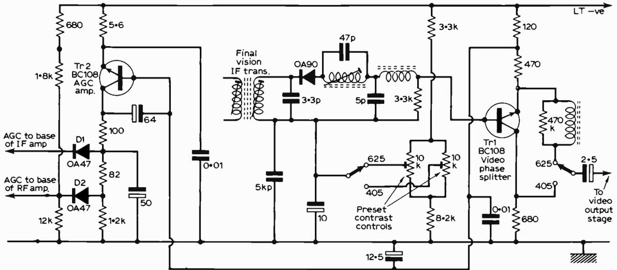
Fig. 4: Transistor a.g.c. system used in many Pye/Ekco models.
