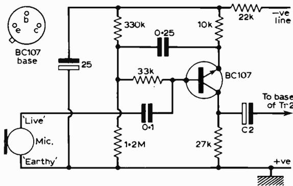
Fig. 5: Alternative front-end using a bootstrapped BC107.
