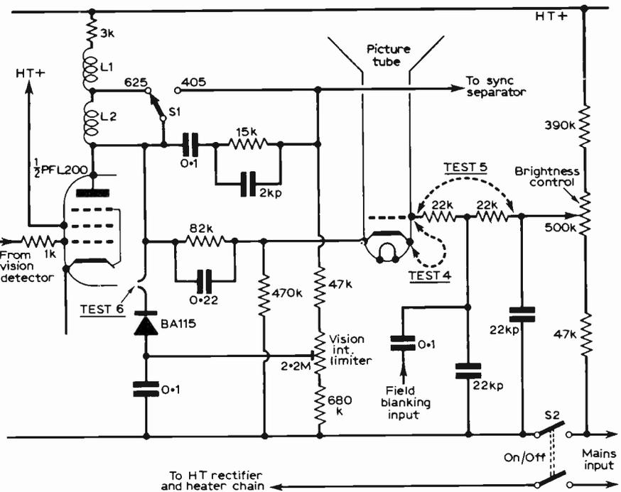
Fig. 4: Circuit with video amplifier direct coupled to the tube, showing test points. A vision-interference limiter is also incorporated in this circuit.
