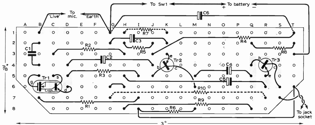
Fig. 4: Veroboard layout. Note that f.e.t.s. are very sensitive to static discharged through the device via the gate electrode and to avoid the possibility of damage to the gate oxide layer due to this cause the leads of the TAA320 are shorted by a clip when supplied. The clip is arranged so that it need not be removed until the i.c. has been mounted on the Veroboard. R7, R10 and C6 are on the conductor side of the board.
