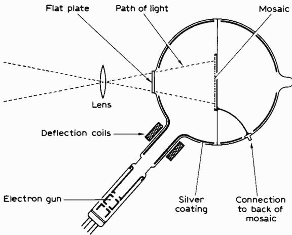
Fig. 3: Construction of the Emitron tube.
