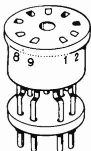
Fig. 1: Valve adaptor which can be used in these circumstances is the valve plug-holder.
