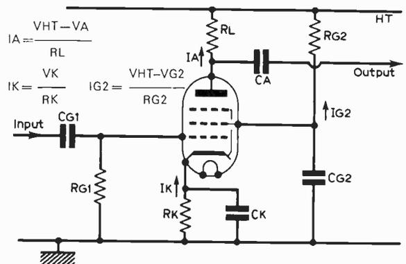
Fig. 27: A simple pentode valve amplifier stage, illustrating d.c. operating conditions.
