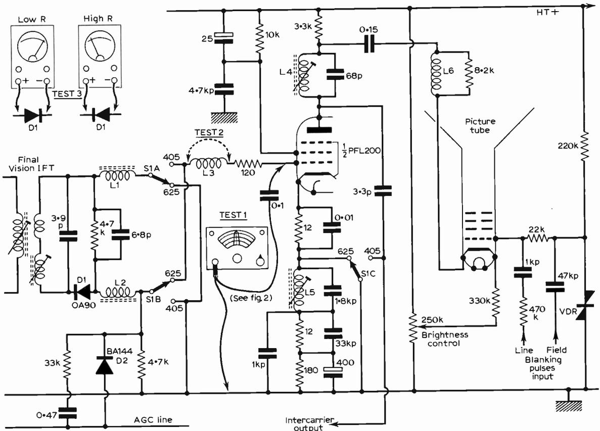
Fig. 1: The detector, video amplifier and tube biasing circuits of a recent model, showing test points.
