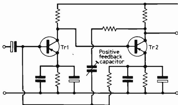
Fig. 13: The use of selective positive feedback with a pair of transistors to boost h.f. gain.
