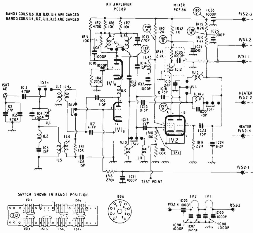
Fig. 3: V.H.F. tuner circuit and interconnections.
