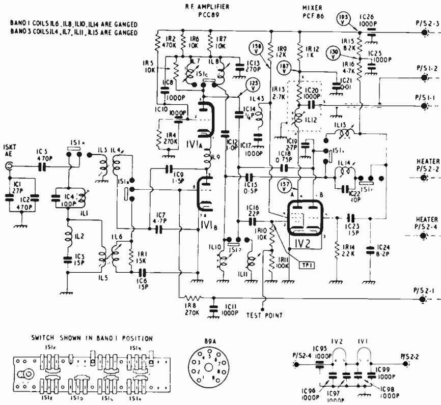
Fig. 3: V.H.F. tuner circuit and interconnections.
