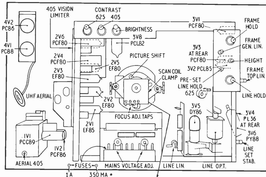
Fig. 1: Rear view of chassis assembly showing valve and control positions.
