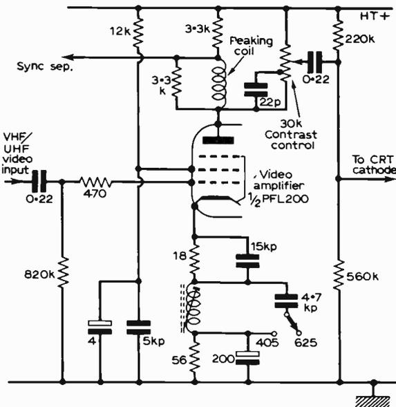
Fig. 2: High-level contrast control system as used in many valve-only and hybrid Pye/Ekco models.
