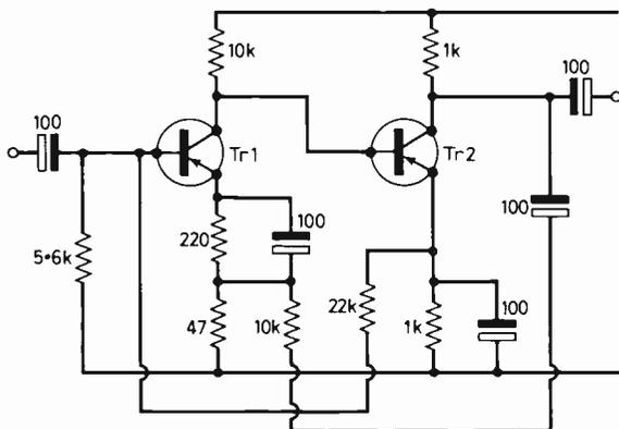
Fig. 12: Video amplifier (30dB gain up to 10MHz) using negative feedback. The 22 kΩ resistor between  $Tr_2$  emitter and  $Tr_1$  base is for d.c. stabilisation only.  $Tr_1$  and  $Tr_2$  can be any r.f. transistor (OC171, AF119 etc.) and the line voltage should be close to the maximum permissible. Bypass each of the 100 μF electrolytics with a 1,000 pF mica capacitor.
