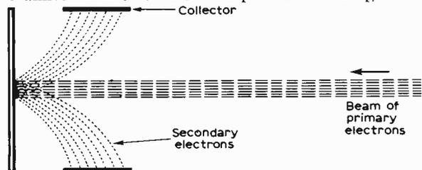
Fig. 1: Secondary emission from a surface.
