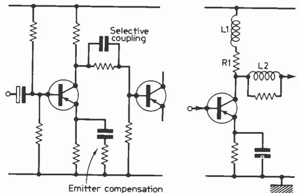
Fig. 9 (left): Use of selective coupling and decoupling. Fig. 10 (right): Use of peaking coils. The inductance of the coils is given by the formulae
