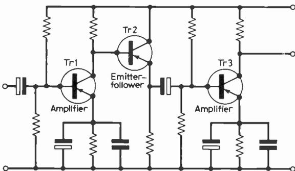
Fig. 8: Use of an emitter-follower stage to couple two common-emitter amplifier stages.
