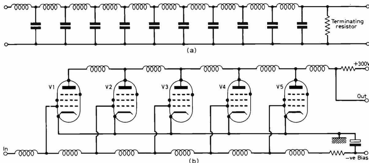
Fig. 14: The travelling-wave or distributed amplifier.
