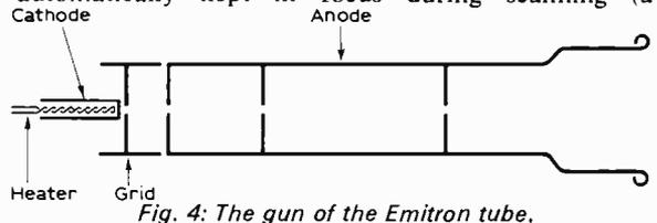
Fig. 4: The gun of the Emitron tube.
