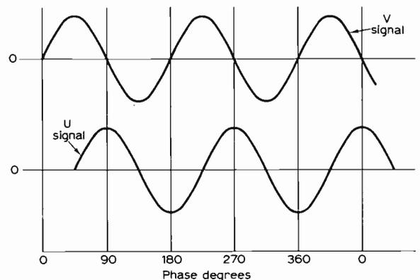
Fig. 4: Two sine wave signals, marked V and U, with the same frequency but a phase difference of 90°.
