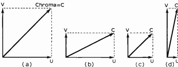
Fig. 7: The composite signal shown in Fig. 5 (i.e. the chroma signal) has amplitude and phase characteristics governed by the lengths (amplitudes) of the V and U signals, the C signal being obtained by completing the vector diagram shown in Fig. 6. Notice that both the amplitude and phase of the C signal are related to the V and U signals.
