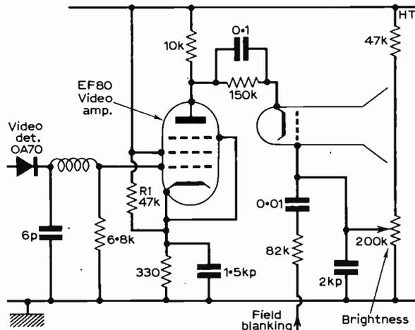
Fig. 2: See video bias stabiliser resistor.
