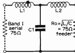
Fig. 2: Low-pass filter.
