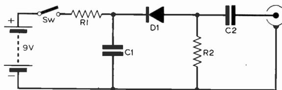
Fig. 3: Simple noise generator circuit.
