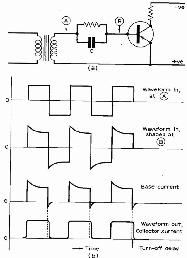
Fig. 2: (a) The input pulse can be sharpened by the use of low-impedance input loading and by a speed-up capacitor C at the base input. (b) The waveforms at A and B above, showing the pulse sharpening effect of the speed-up capacitor. The resultant base and collector current waveforms are also shown.
