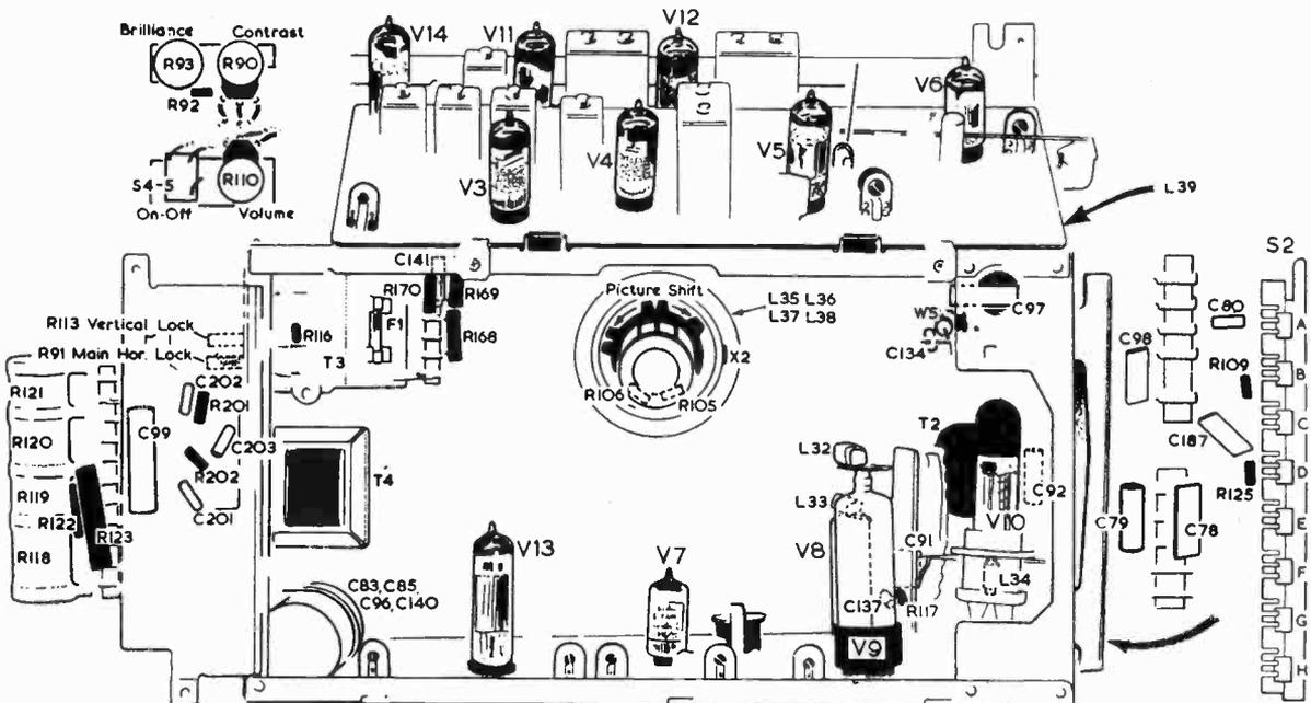
Fig. 1: Rear chassis view. In some versions the mains dropper R118-R121 is mounted horizontally at the rear centre.
