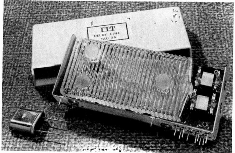
Our photograph above shows two newly introduced piezoelectric components for PAL decoders. The crystal type CTV on the left is for use in the reference oscillator circuit and is housed in an HC-6/U holder with flying leads. The other component, on the right, is a PAL-D line-duration delay line, type TAU20, which is complete with input and output matching transformers.
