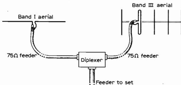
Fig. 1: Use of a diplexer with separate Band I and III aeriels so that a common download can be employed.
