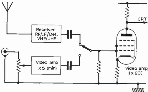
Fig. 1: The requirements of a "Schools" receiver able to accept a 1V peak-to-peak local video input.
