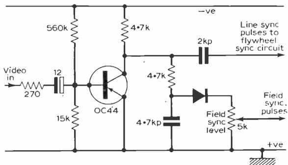
Fig. 6: The Perdio Portarama all-transistor portable model used an OC44 in another of the simple input-charge type of circuit. For all these circuits regulation of the rail voltage is essential as the circuit operating conditions are as important as the component values.
