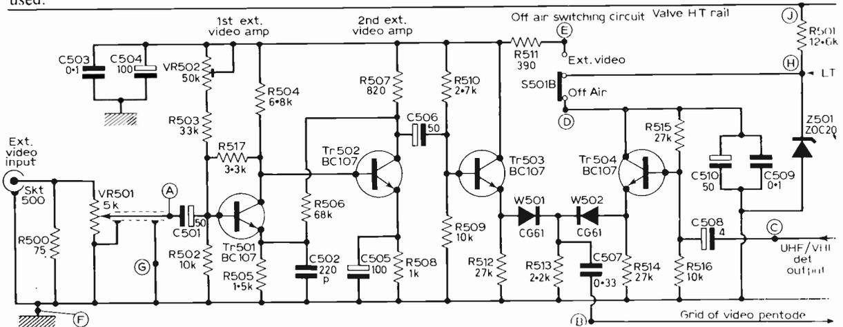
Fig. 5: The two-stage video amplifier for external inputs (Tr 501 and Tr 502) plus the electronic switching circuit for changing over from broadcast to local video as used in the BRC schools model.
