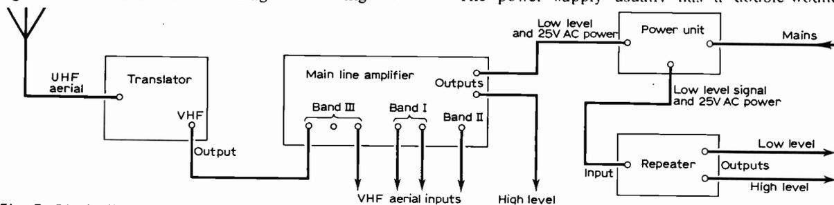
Fig. 5: Block diagram of a typical v.h.f. television line distribution system.
