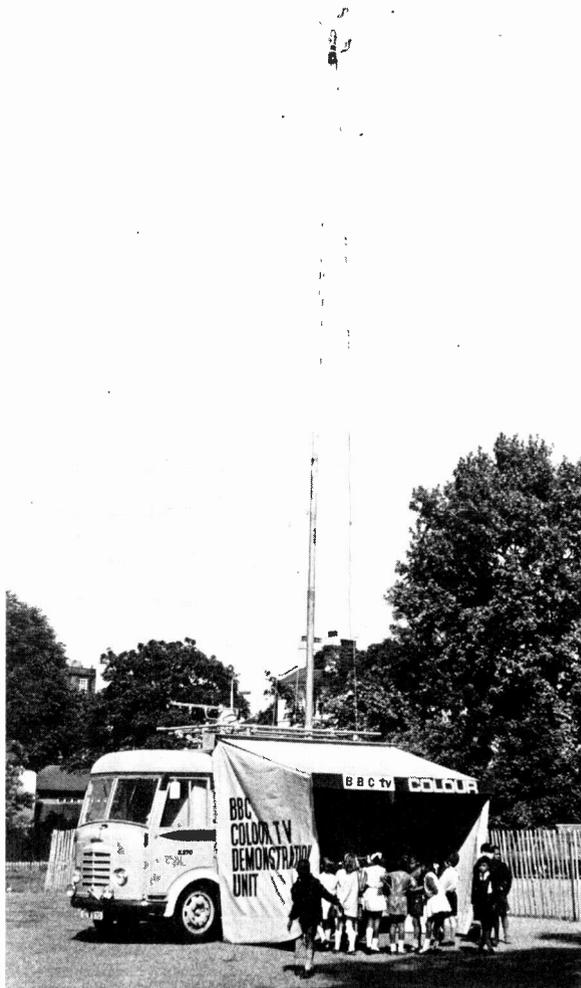
General view of the BBC's mobile colour demonstration unit with aerial mast extended and side awning out.
