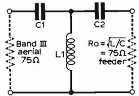
Fig. 3: High-pass filter
