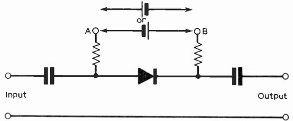
Fig. 2: Biased diode used as a switch between a.c. input and output.
