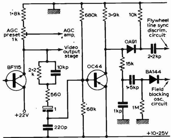
Fig. 4: In the Philips T-Vette portable television model the OC44 sync separator stage is driven by the video emitter-follower stage, a.c. coupling being used. The emitter-follower also drives the a.g.c. amplifier stage and provides peak signal clipping to reduce the effects of noise on the sync separator under weak signal conditions.
