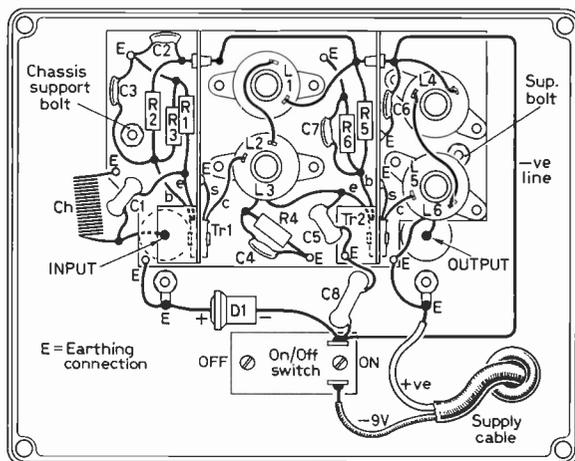
Fig. 2: Layout of the preamplifier.
