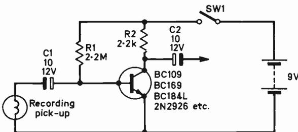
Fig. 1: Suggested preamplifier circuit.
