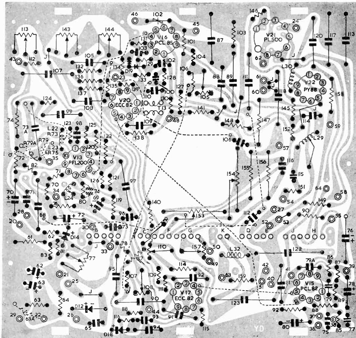
Fig. 3: Layout of the timebase printed panel, viewed from the print side.
