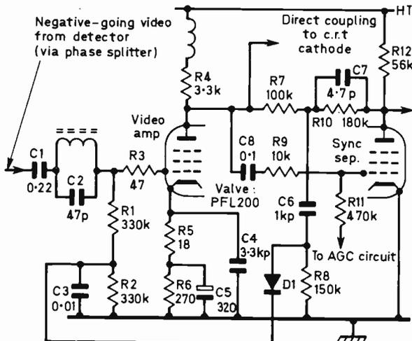
Fig. 3: Video stage (Bush-Murphy) incorporating a brightness-compensation circuit. D1 is type BA144 in the Bush-Murphy chassis.
