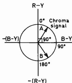
Fig. 1: Basic PAL principle.
