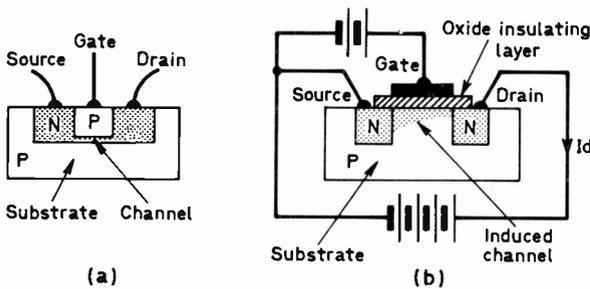
Fig. 4: (a) Diffused n-channel junction-gate f.e.t. (b) N-channel insulated-gate f.e.t., with biasing.
