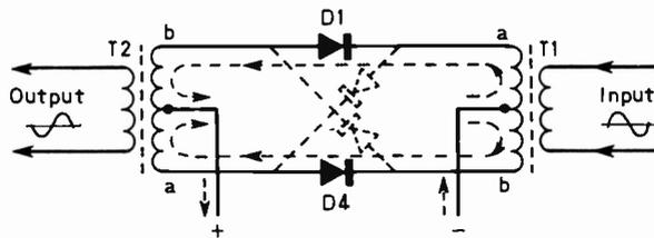
Fig. 4: (a) Ring modulator circuit used as the PAL switch in the Beovision Model 3000. (b) and (c) show how inversion of the signal occurs through reversing the direction of current flow around the circuit.
