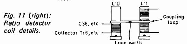
Fig. 11 (right): Ratio detector coil details.
