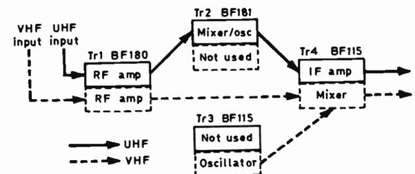
Fig. 3: Block diagram of the all-band tuner used in the BRC 2000 chassis.
