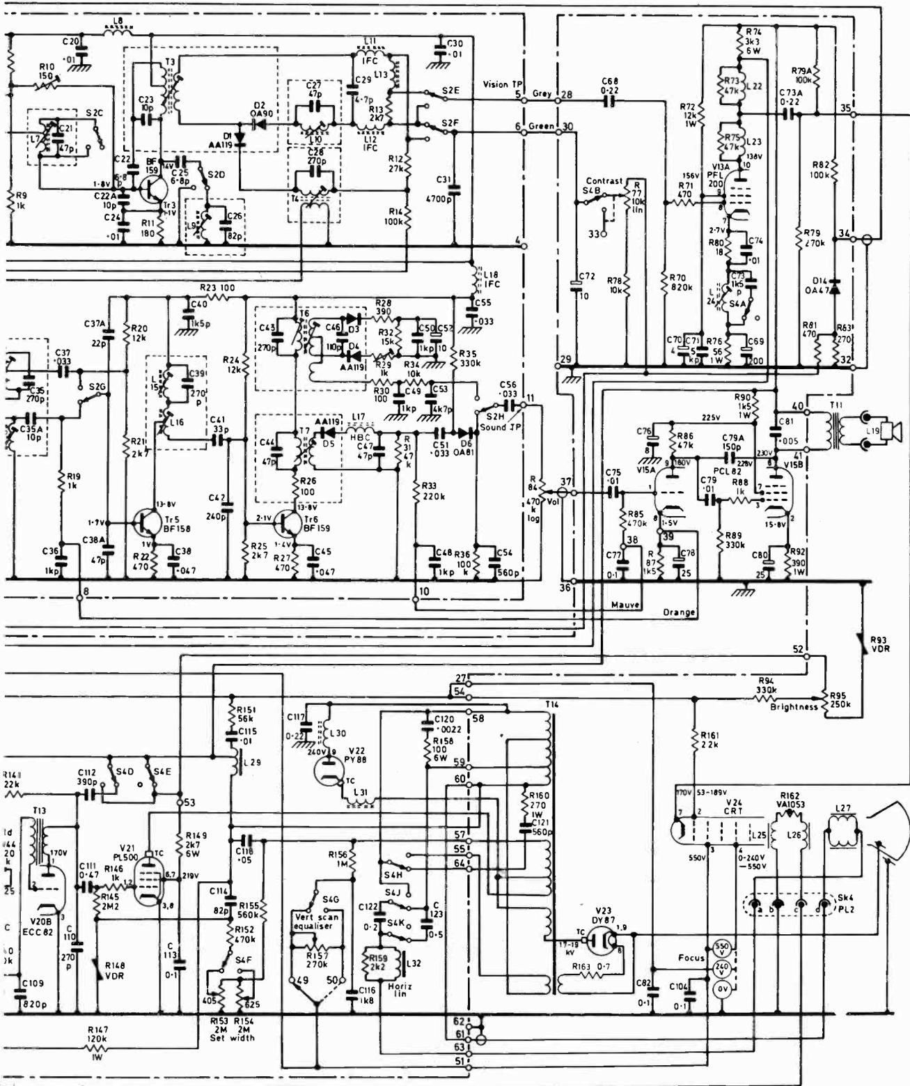
*V1 is a 1A anti-surge type. The valve voltage readings were taken with signal input, 240V a.c. mains input, volume control 0. E.H.T. is 17-19kV, measured with an electrostatic voltmeter and zero beam current. Transistor voltages taken with no signal, centre-tapped, a 47Ω resistor was fitted in Tr3 collector-lead, C12 was 22pF, C25 4.7pF, C32 25µF, C40 1,000pF, C72 followed the component value convention now used by most setmakers, i.e. 2k7 = 2.7kΩ, 3M3 = 3.3MΩ etc.*
