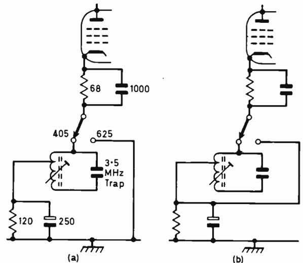
Fig. 4: Video amplifier cathode circuit with 3.5MHz trap. Typical component values shown.
