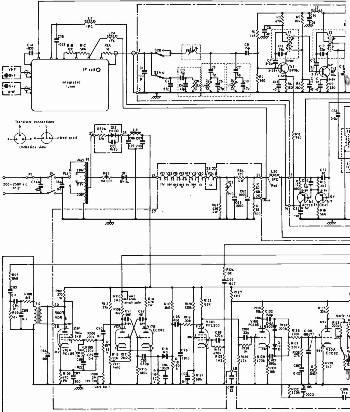
Fig. 2: Circuit diagram of the Pye Model 40F. The system switching is shown in the 405-line position. The mains fuse F at minimum and all other controls set for normal operation and the set switched to 405, using an Avo Model 8 (20,000Ω/V; signal and contrast control at maximum. In early models C1A, C1B, C73A, C34A and R79A were not fitted, L24 was 25μF, R79 470kΩ, or not fitted, R84 1MΩ, R102 33kΩ and R112 75kΩ. We have in this diagram fol.
