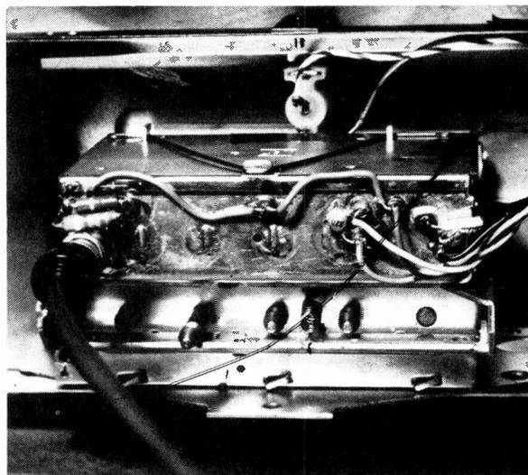
Fig. 5: The u.h.f. tuner wired into a recent Decca single-standard colour receiver.
