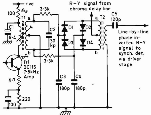
Fig. 5: A diode ring circuit is also used in ITT-KB models. This however is switched by the high-amplitude iden signal and is used to invert the R-Y chroma signal.
