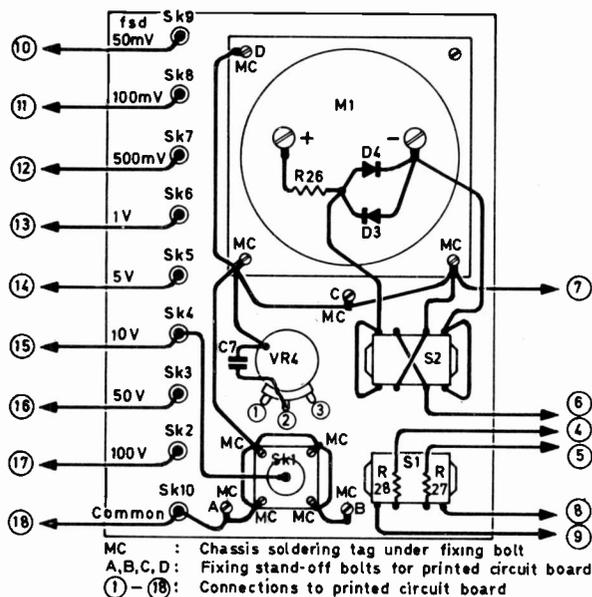
Fig. 3: Rear view of the front panel assembly. The panel is approximately 4 x 6 in.
