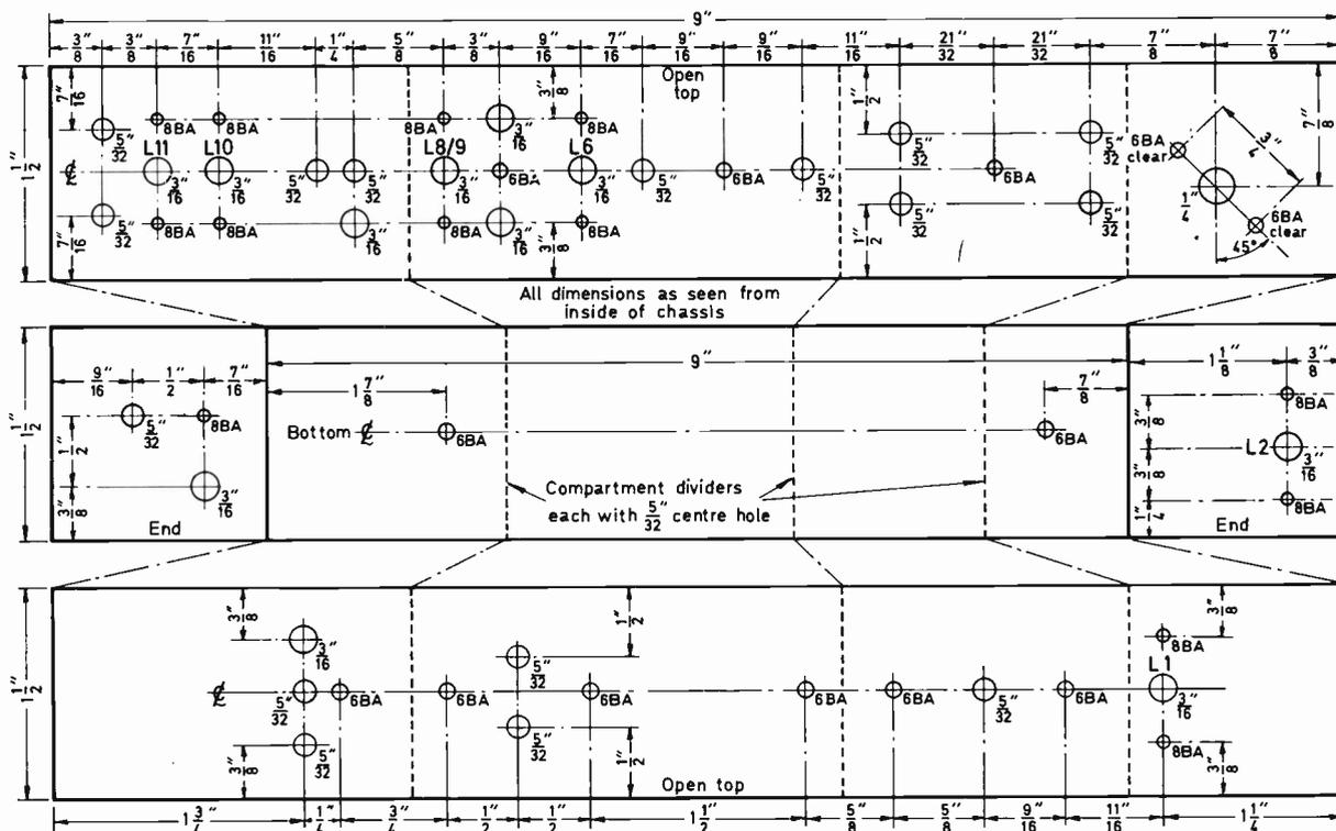
Fig. 12: Drilling details and dimensions of the chassis for the constructor's i.f. strip.
