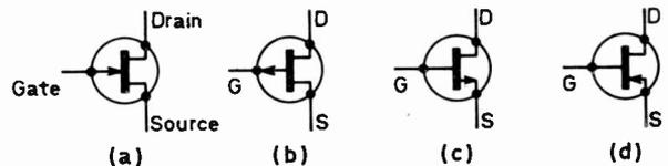
Fig. 3: Junction-gate f.e.t. circuit symbols. (a) and (c) n-channel, (b) and (d) p-channel types.
