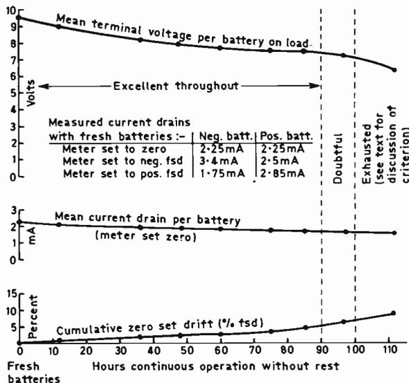
Fig. 2: Battery life, current drain and zero drift of the i.c. millivoltmeter.
