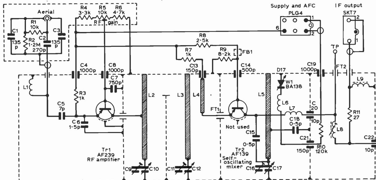
Fig. 4: U.H.F. tuner used in the BRC 3000 single-standard chassis.
