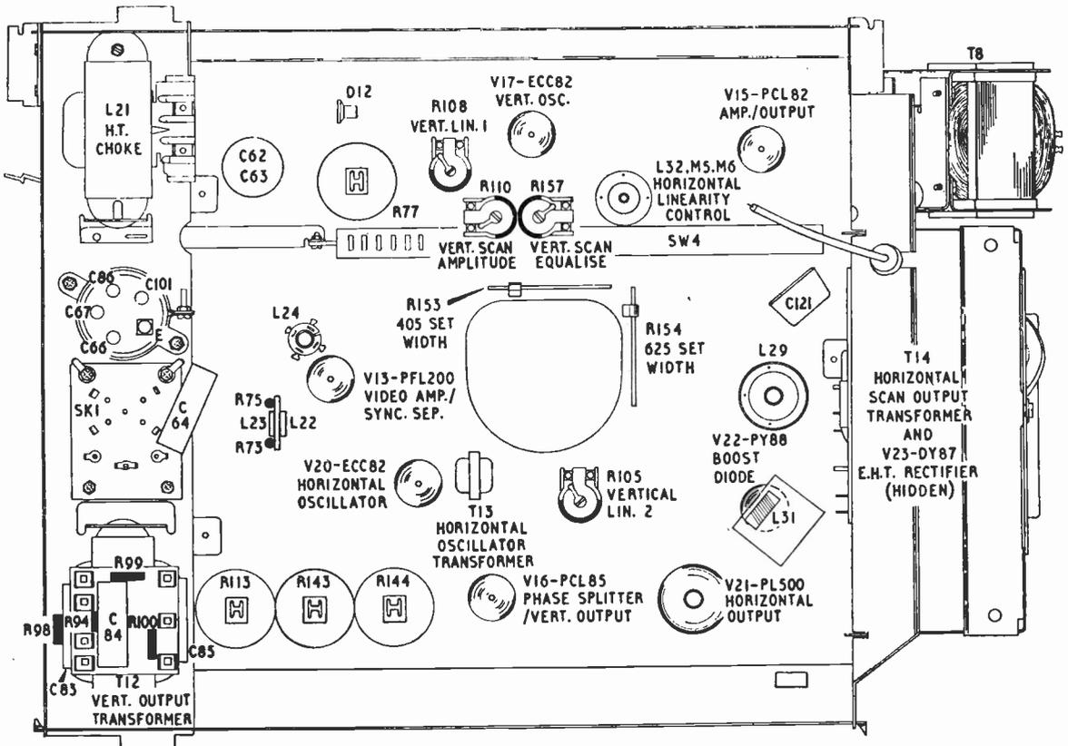
Fig. 1: Pye 40F main chassis layout—shown here in lowered position.
