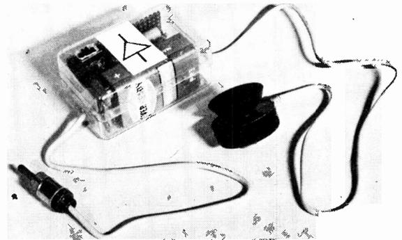
box which also holds the battery and on/off switch. Construction is simple as the layout is in no way critical. The screened lead from the pickup coil can be wired directly on to the circuit board and the output taken via a second screened lead to the type of plug used on your recorder—DIN, phono, etc.
