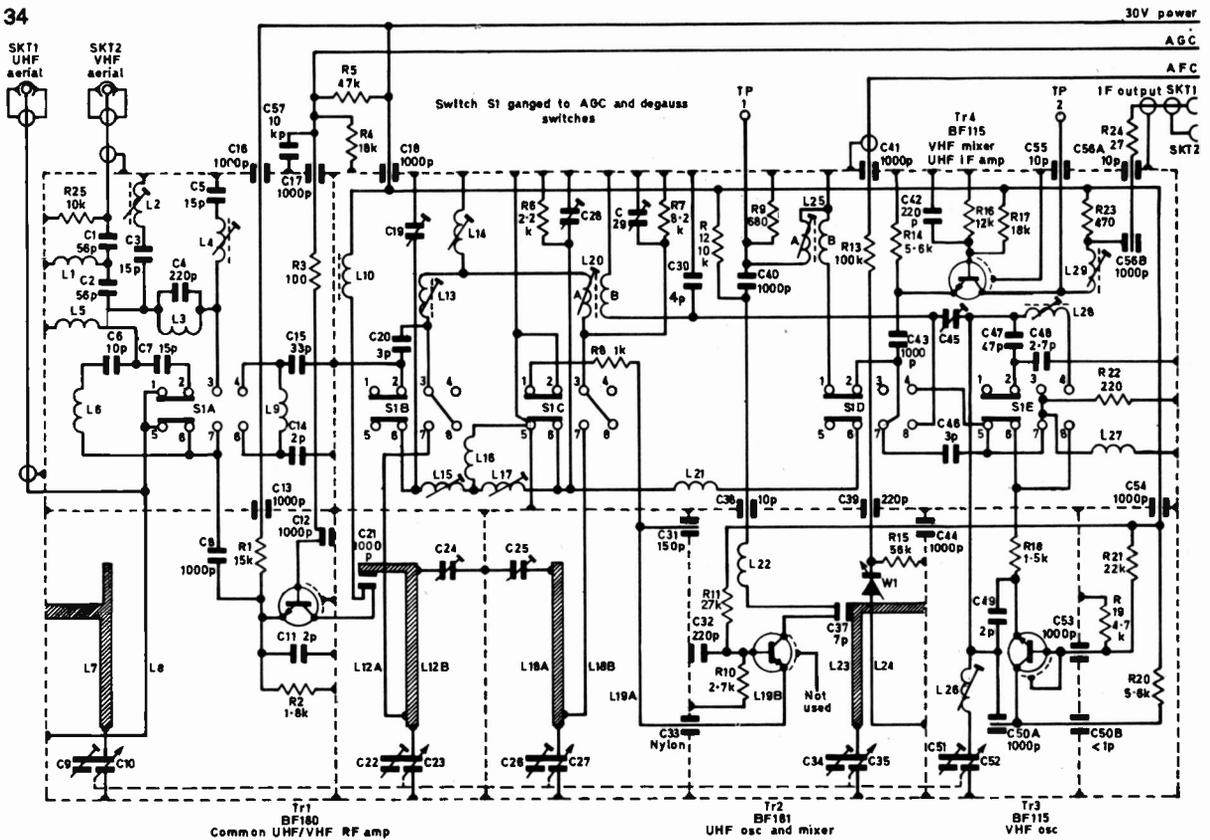
Fig. 2: All-band tuner unit used in the BRC 2000 dual-standard chassis. S1 shown in u.h.f. position. Contacts 2, 3 and 6, 7 closed on Band III, 3, 4 and 7, 8 closed on Band I.
