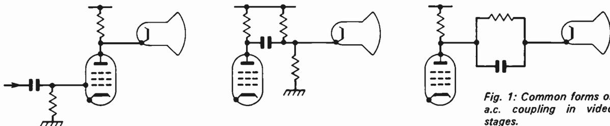
Fig. 1: Common forms of a.c. coupling in video stages.
