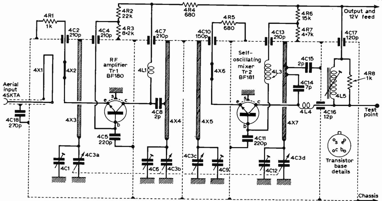
Fig. 1: U.H.F. tuner unit used in the Rank-Bush-Murphy dual-standard colour chassis (a separate tuner is used for v.h.f.). A modified version of this tuner is used in the later single-standard chassis.
