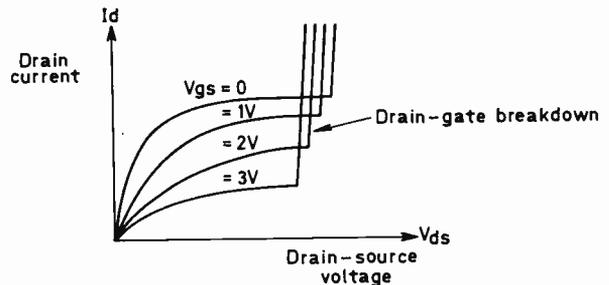
Fig. 2: Typical set of j.u.g.f.e.t. characteristics.
