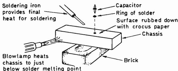
Fig. 4: Method of soldering feedthrough capacitors.
