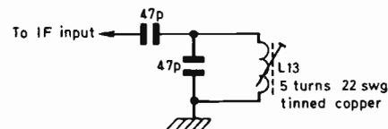
Fig. 10 (left): 41.5MHz trap.
