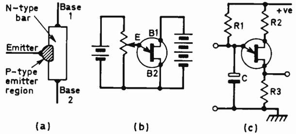
Fig. 6: The unijunction transistor, (a) construction, (b) principle of operation, (c) basic oscillator circuit.
