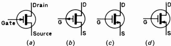
Fig. 5: Insulated-gate f.e.t. symbols. (a) and (c) n-channel, (b) and (d) p-channel types.
