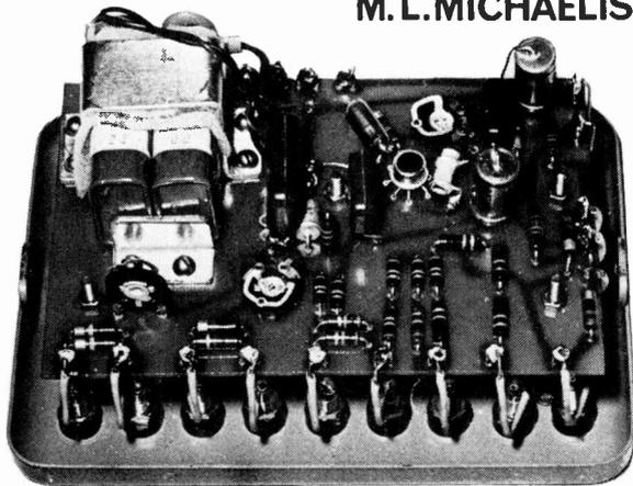
The complete theoretical circuit of the i.c. millivoltmeter is shown in Fig. 1 and is simple to understand in the light of the detailed discussion of operational amplifiers given in the August issue. A high input impedance is required so the voltage from the input bleeder network is taken to IP. VR3 is  $R_{FB}$  and its ratio with respect to R19 determines the operating gain factor which is adjustable with VR3 to set the overall sensitivity of this electronic voltmeter.
