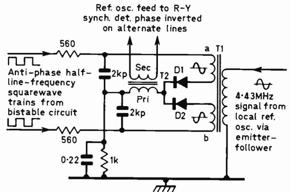
Fig. 3: Representative PAL switch, used to reverse the local oscillator feed to the R-Y synchronous detector.
