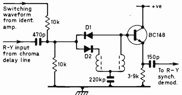
Fig. 6: Simple Decca PAL switch circuit.
