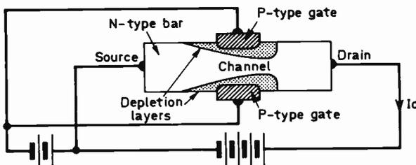
Fig. 1: Alloy n-channel junction-gate f.e.t.
