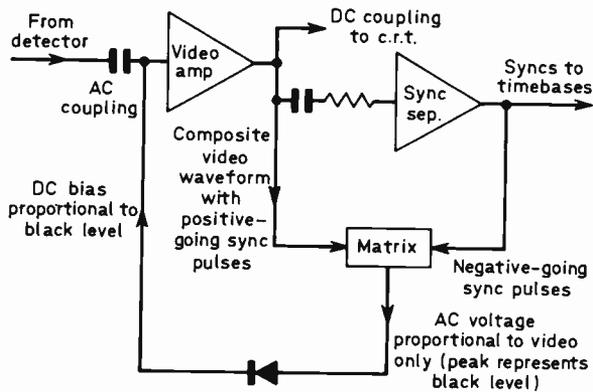
Fig. 2: Block diagram of the brightness-compensation system.
