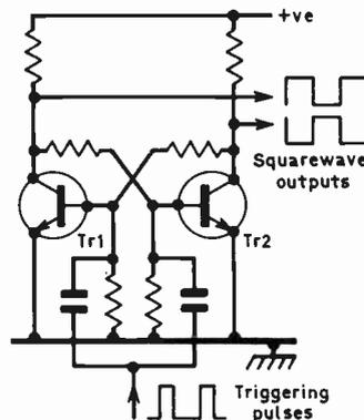
Fig. 2: Basic bistable switching circuit, using transistors.
