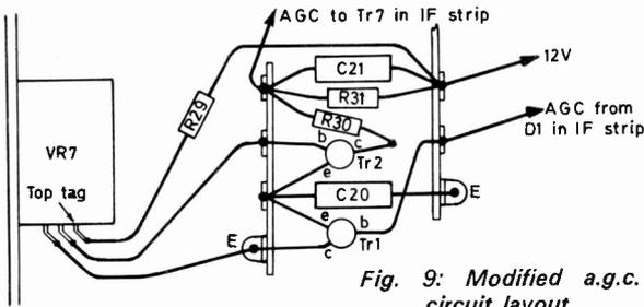
Fig. 9: Modified a.g.c. circuit layout.
