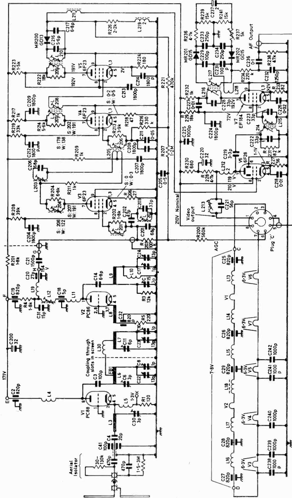
Fig. 2: Complete circuit of the Murphy 625-line conversion unit.
