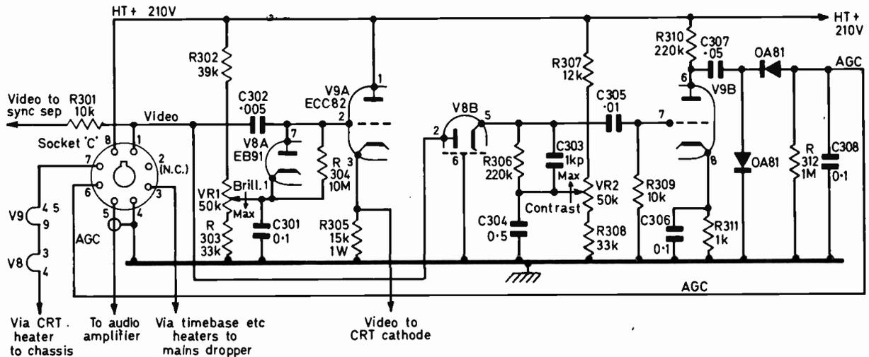
Fig. 3: Circuit of the add-on unit which forms a link between the Murphy unit and the rest of the set.
