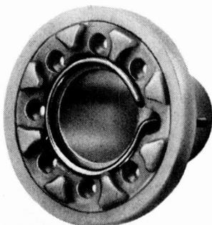
Left: Ringtrap type tube base to provide flashover protection for a monochrome tube. The wire ring forms a sparkgap to each tube pin. (Photograph courtesy of Mullard Ltd.)
