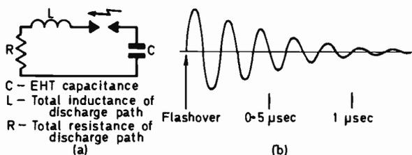
Fig. 6: (a) The equivalent circuit of a flashover path at the instant of discharge. (b) The waveform of the flashover current.
