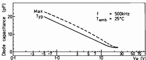
Fig. 1: The capacitance/reverse bias characteristic of a Mullard variable-capacitance diode.
