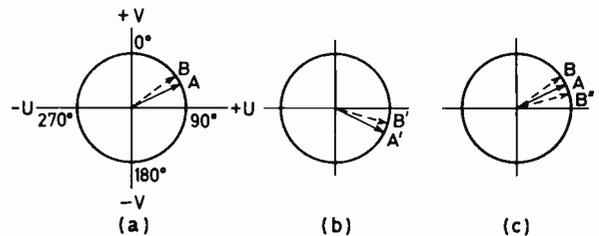
Fig. 3: Principle of phase-error cancellation in the PAL system.
