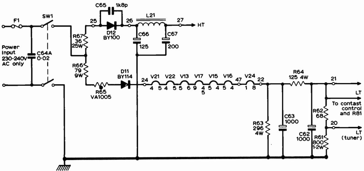
Fig. 8: Power supply circuits of the Pye 36, 37 series.
