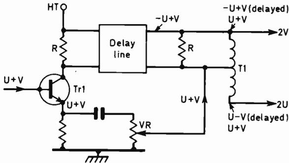
Fig. 2: Commonly used PAL delay line circuit.
