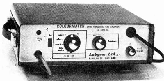
The Labgear CM6010/RG colour pattern generator.
