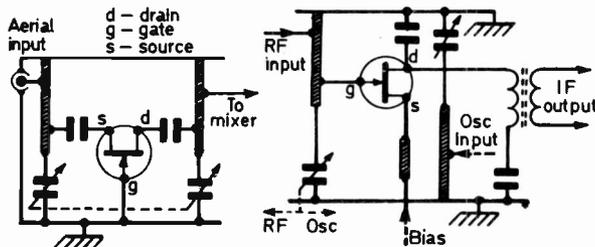
Fig. 5 (left): Basic f.e.t. u.h.f. amplifier circuit. Fig. 6 (right): Basic f.e.t. u.h.f. mixer circuit.
