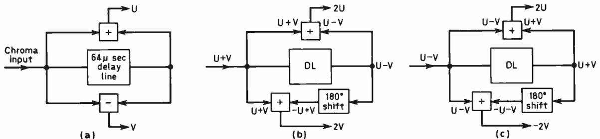
Fig. 1: Principle of operation of the chroma delay-line circuit in a PAL-D receiver.
