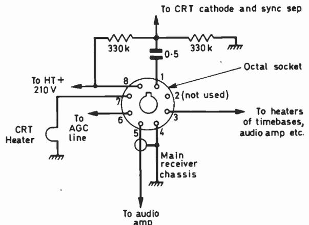
Fig. 1: Socket connections for initial testing.
