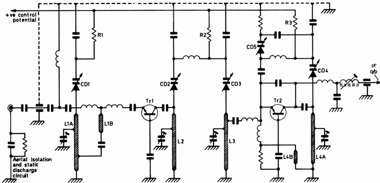
Fig. 3: Skeleton circuit of the Philips capacitance-diode tuner unit.
