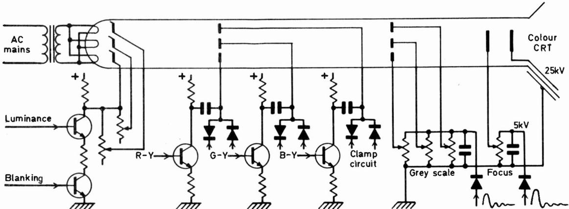
Fig. 3: How much damage would be caused by a flashover to each electrode in turn? Answer, one transformer, four high-voltage power transistors, one low-level transistor, eight diodes (one a 6kV type), six potentiometers and several miscellaneous components!
