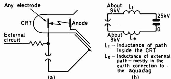
Fig. 7: (a) The basic protection circuit. (b) The equivalent circuit of the flashover path of (a). The e.h.t. voltage is divided between the two inductances.
