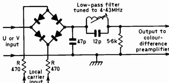
Fig. 5: Diode bridge synchronous detector. The resistors R bias the diodes so that they conduct only on the tips of the sinewave carrier.
