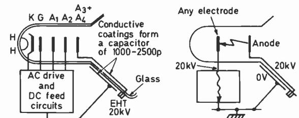
Fig. 1 (left): A highly diagrammatic and simplified representation of a c.r.t. drive and feed circuit with no flashover protection.
