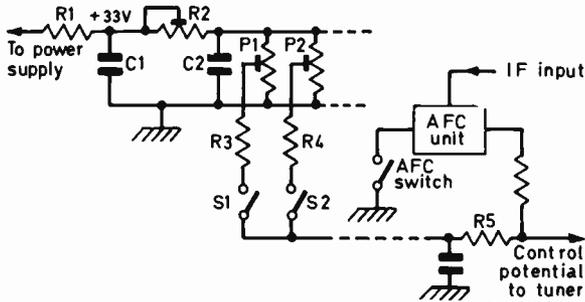
Fig. 4: Basic control arrangement used with the Philips capacitance-diode tuner.
