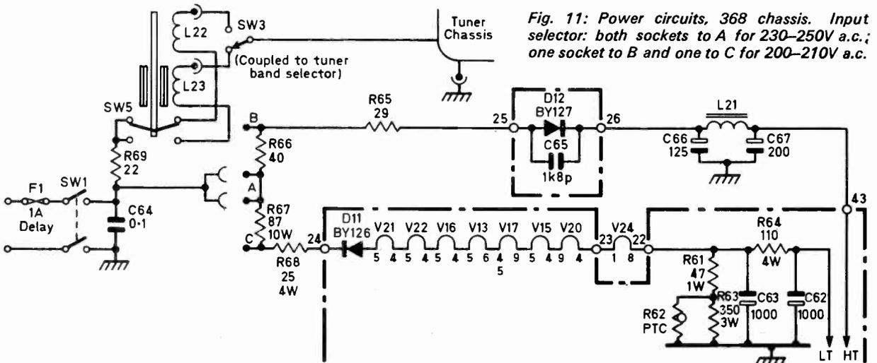
Fig. 11: Power circuits, 368 chassis. Input selector: both sockets to A for 230-250V a.c.; one socket to B and one to C for 200-210V a.c.
